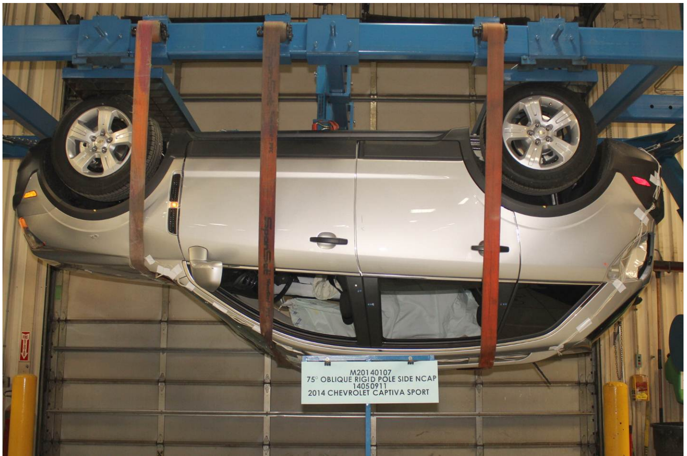
FMVSS No. 301 Static Rollover 180 Degrees
