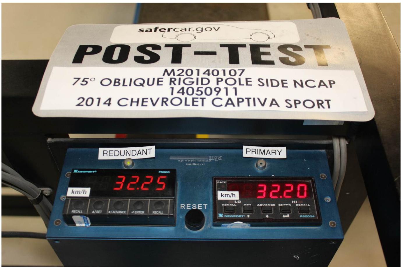
Post-Test Primary and Redundant Speed Trap Read-Out
