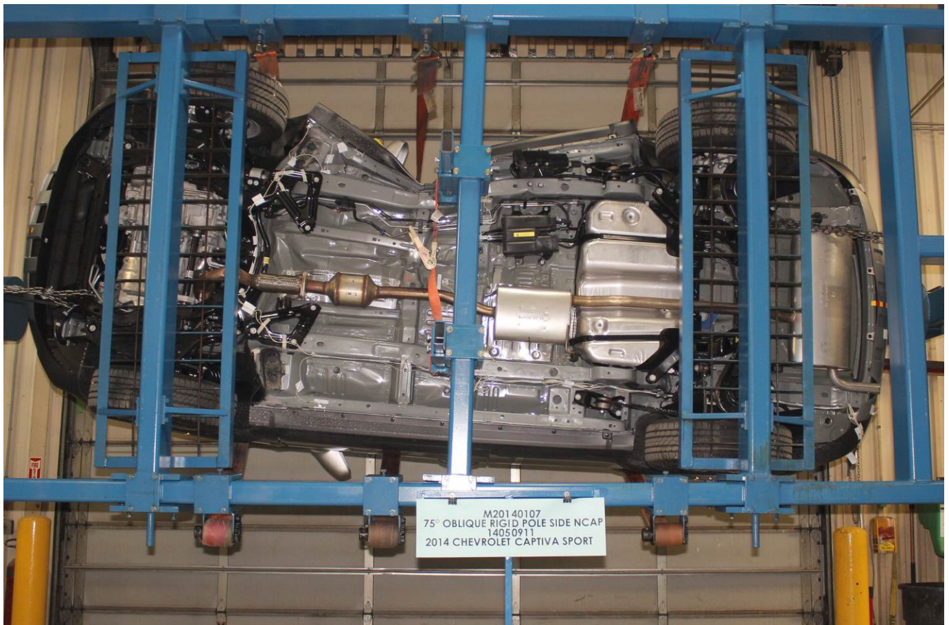
FMVSS No. 301 Static Rollover 270 Degrees
