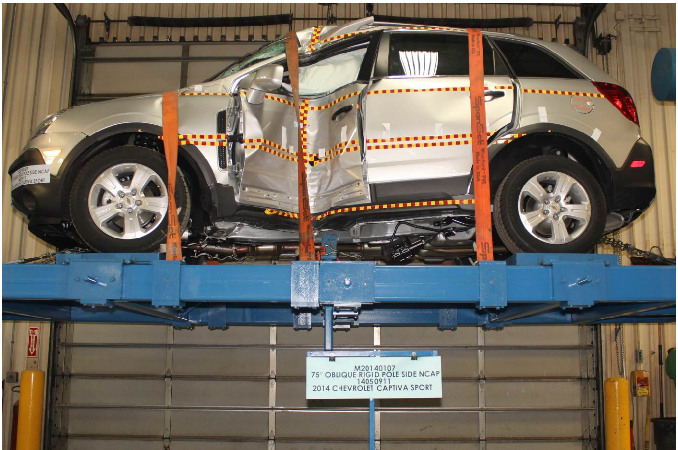
FMVSS No. 301 Static Rollover 0 Degrees
