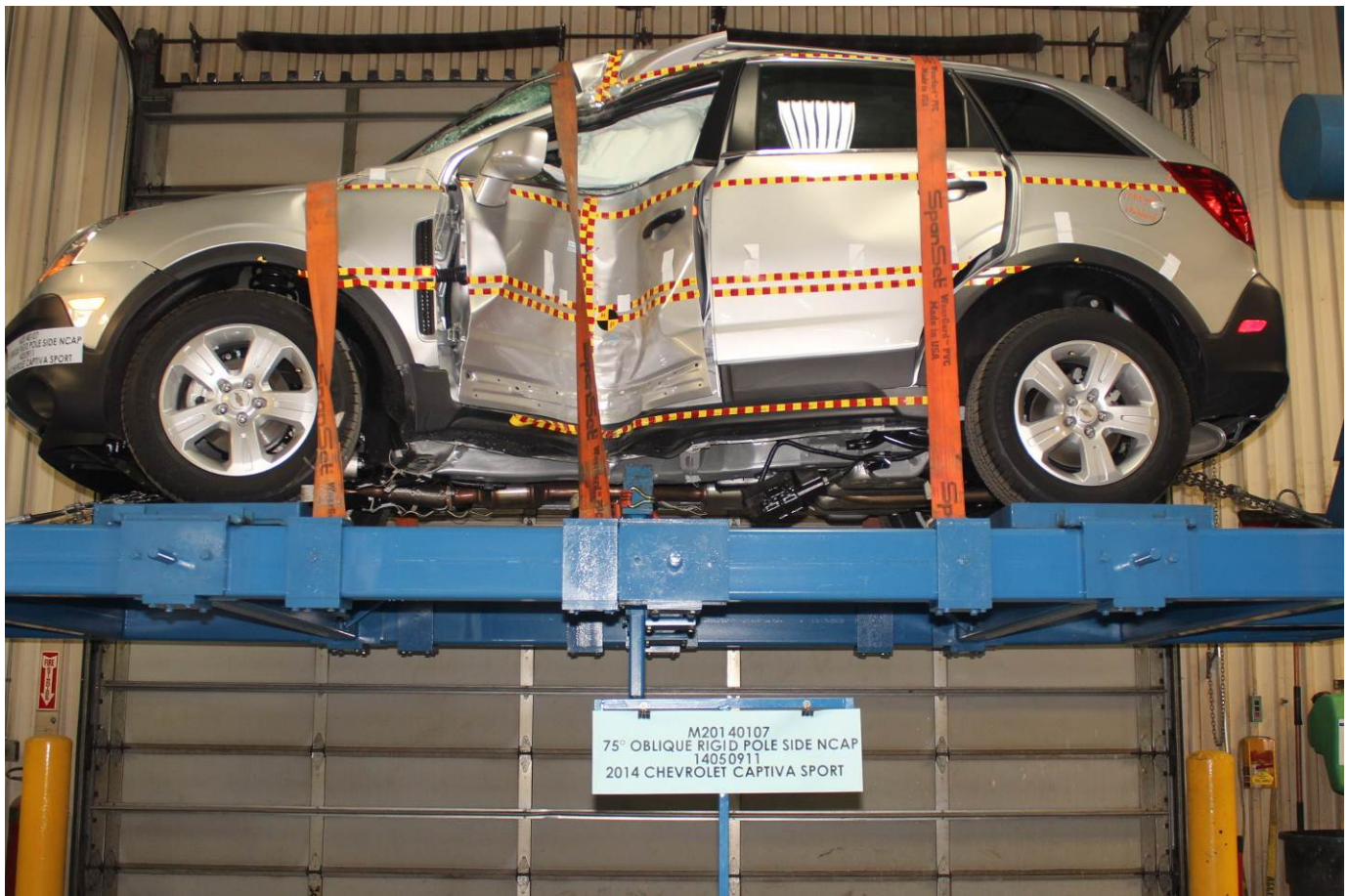
FMVSS No. 301 Static Rollover 360 Degrees
