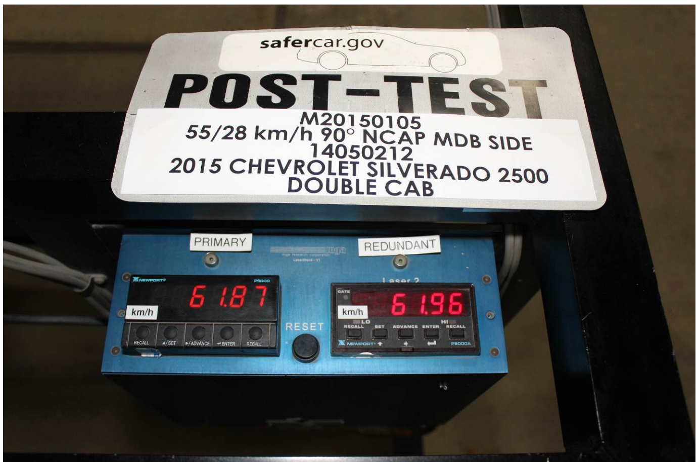
Post-Test Primary and Redundant Speed Trap Read-Out
