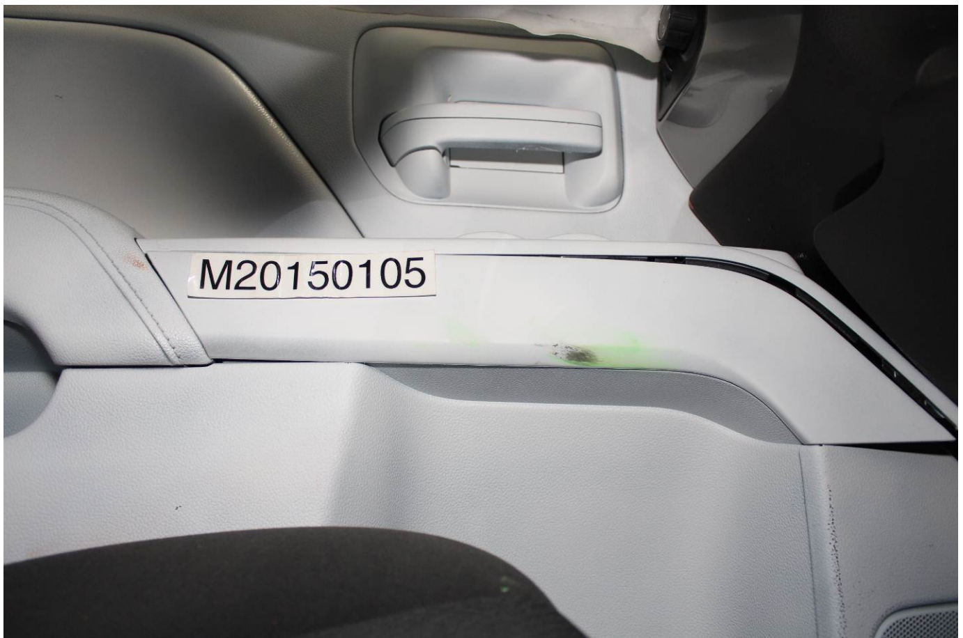
Post-Test Driver Dummy Close-up Knee Contact View
