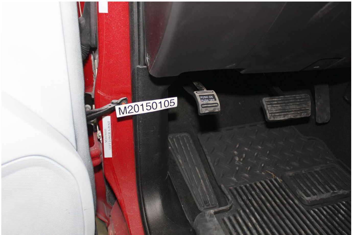
Pre-Test View of Disengaged Parking Brake
