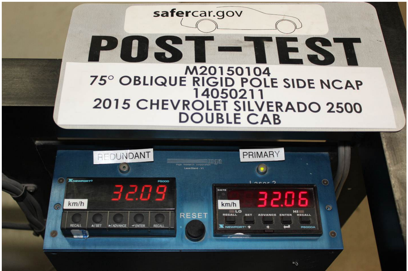
Post-Test Primary and Redundant Speed Trap Read-Out
