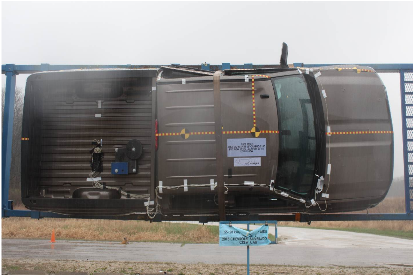
FMVSS No. 301 Static Rollover 270 Degrees
