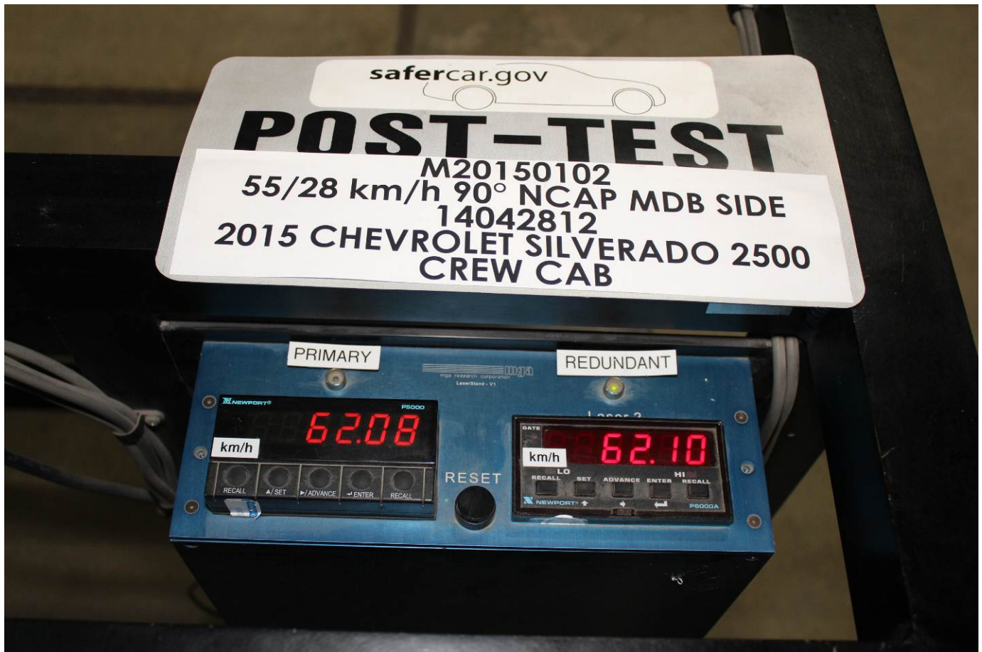
Post-Test Primary and Redundant Speed Trap Read-Out
