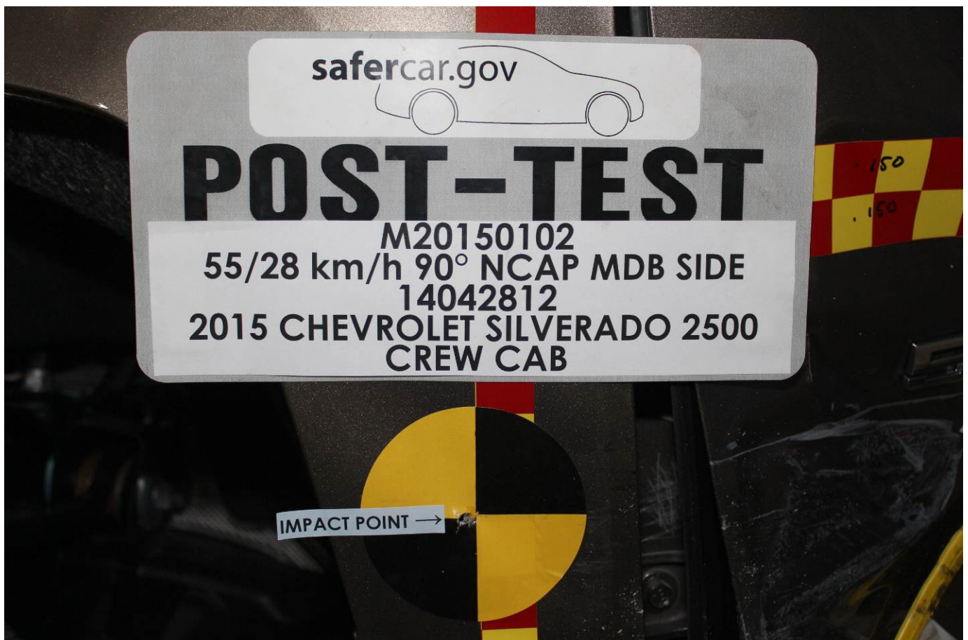
Post-Test Close-Up View of Impact Point Target
