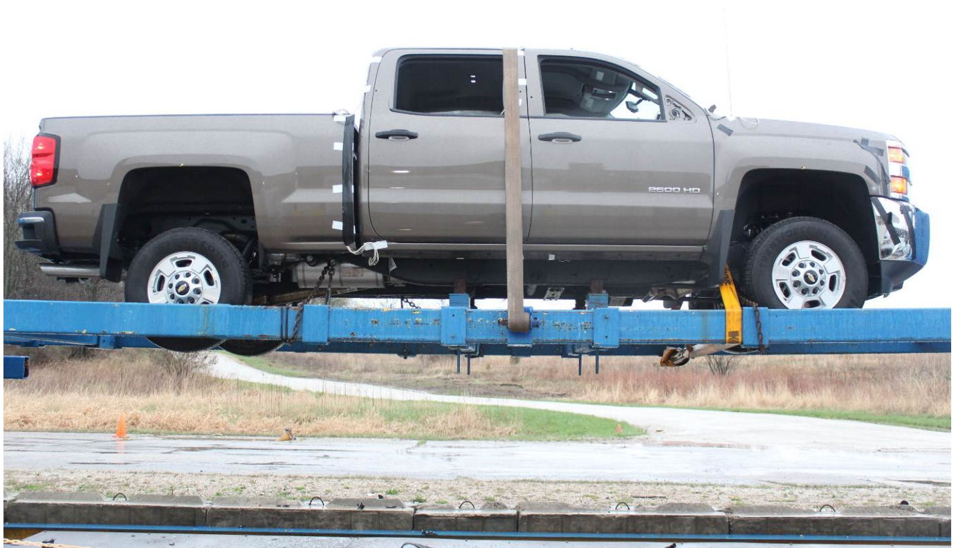
FMVSS No. 301 Static Rollover 360 Degrees
