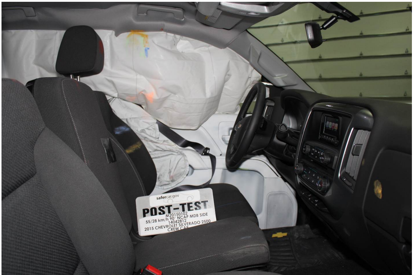
Post-Test Driver Inner Door Panel View
