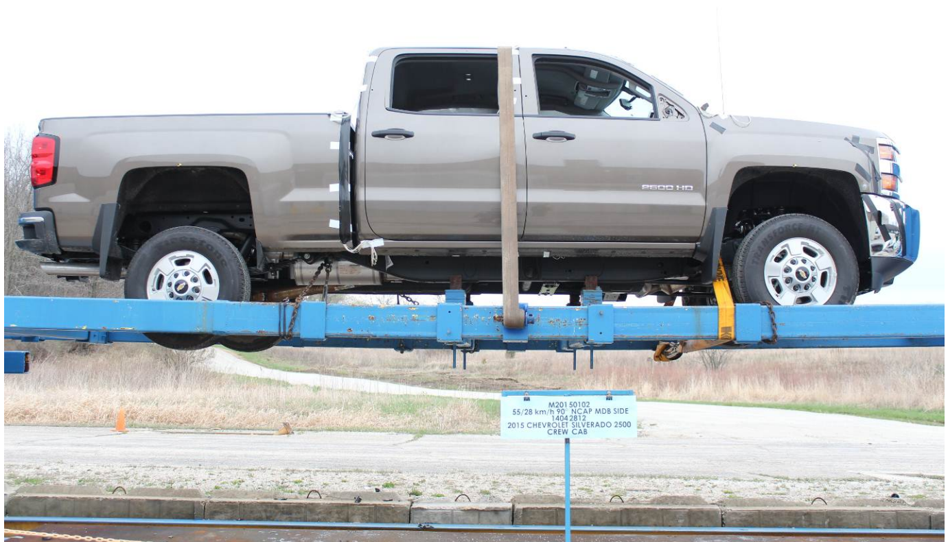
FMVSS No. 301 Static Rollover 0 Degrees
