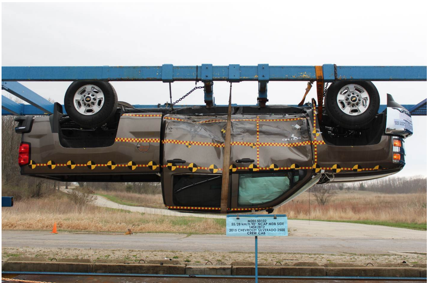
FMVSS No. 301 Static Rollover 180 Degrees
