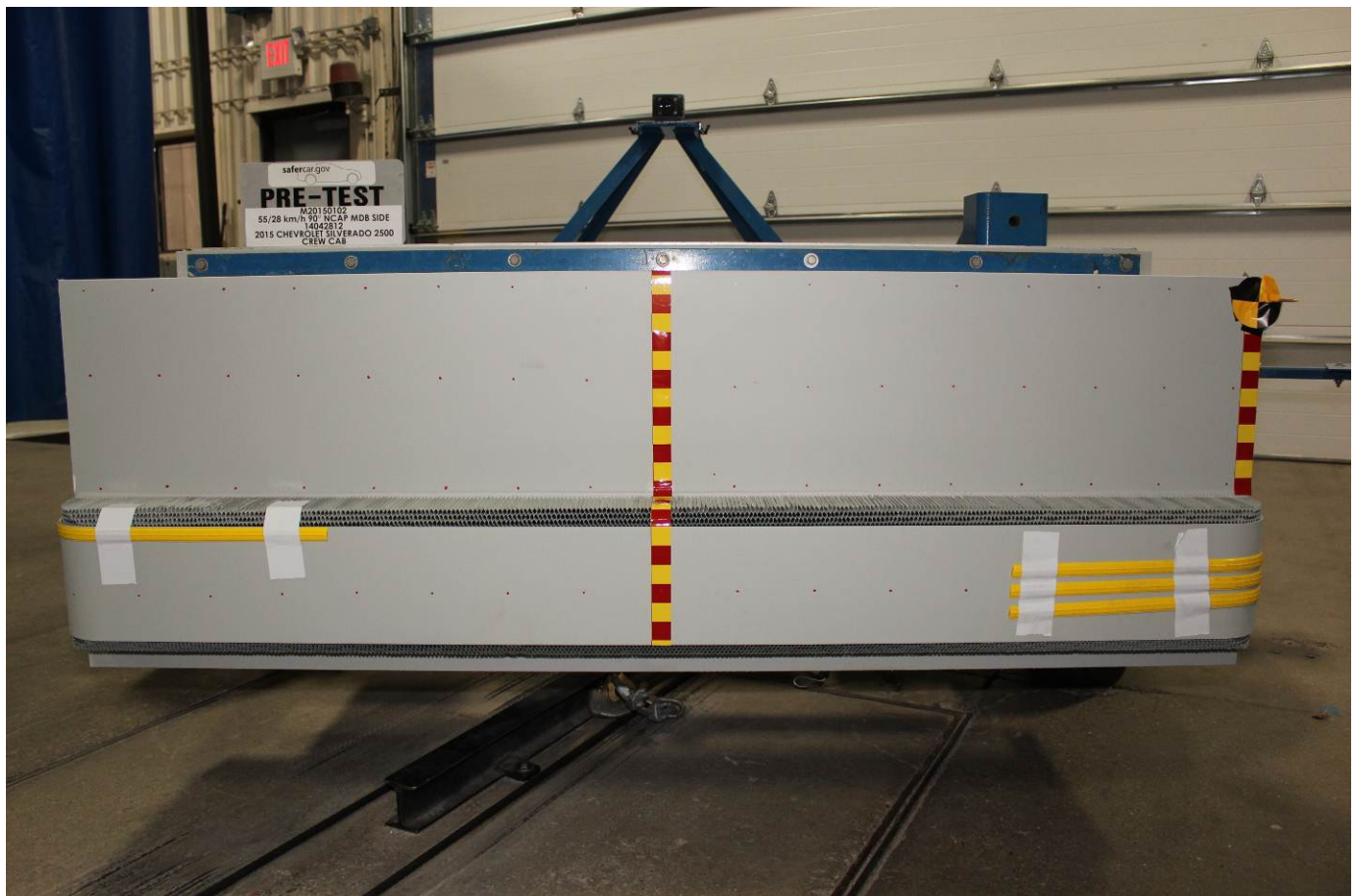
Pre-Test Front View of MDB Impactor Face
