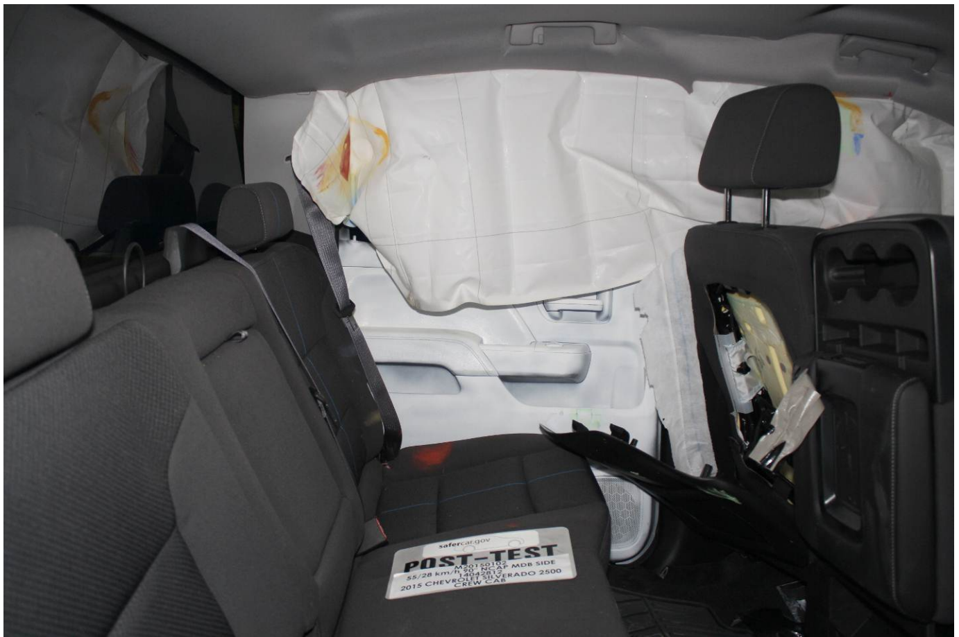
Post-Test Rear Passenger Inner Door Panel View
