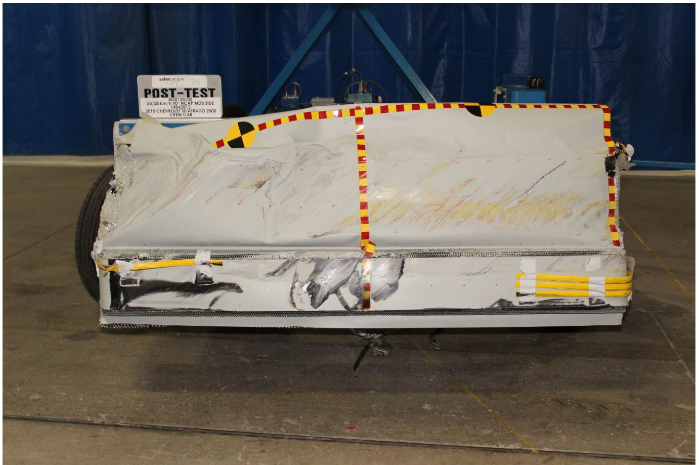
Post-Test Front View of MDB Impactor Face
