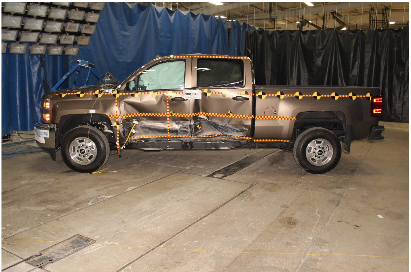
Post-Test Left Side View of Test Vehicle
