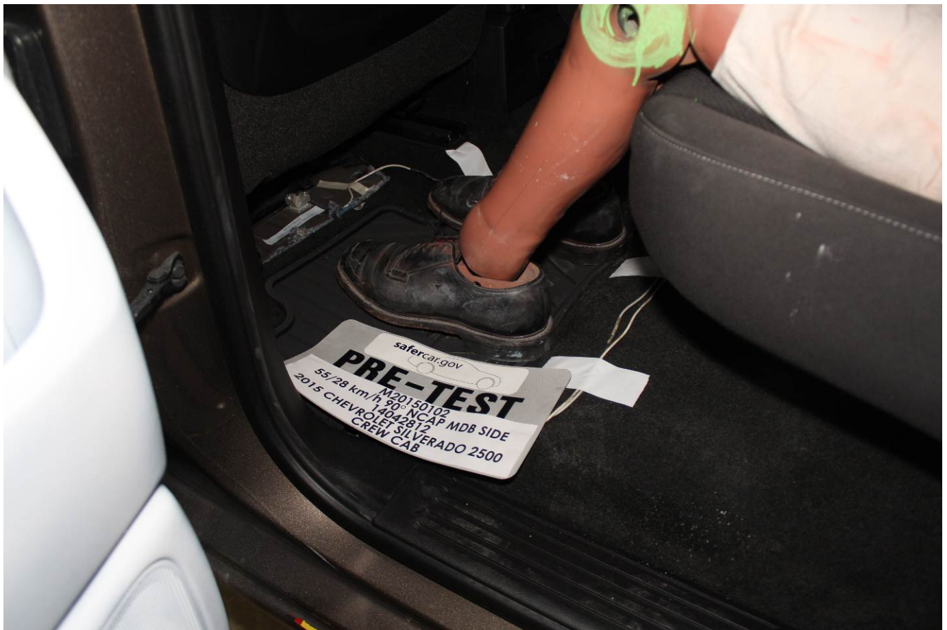
Pre-Test Placement of Rear Passenger Dummy's Feet
