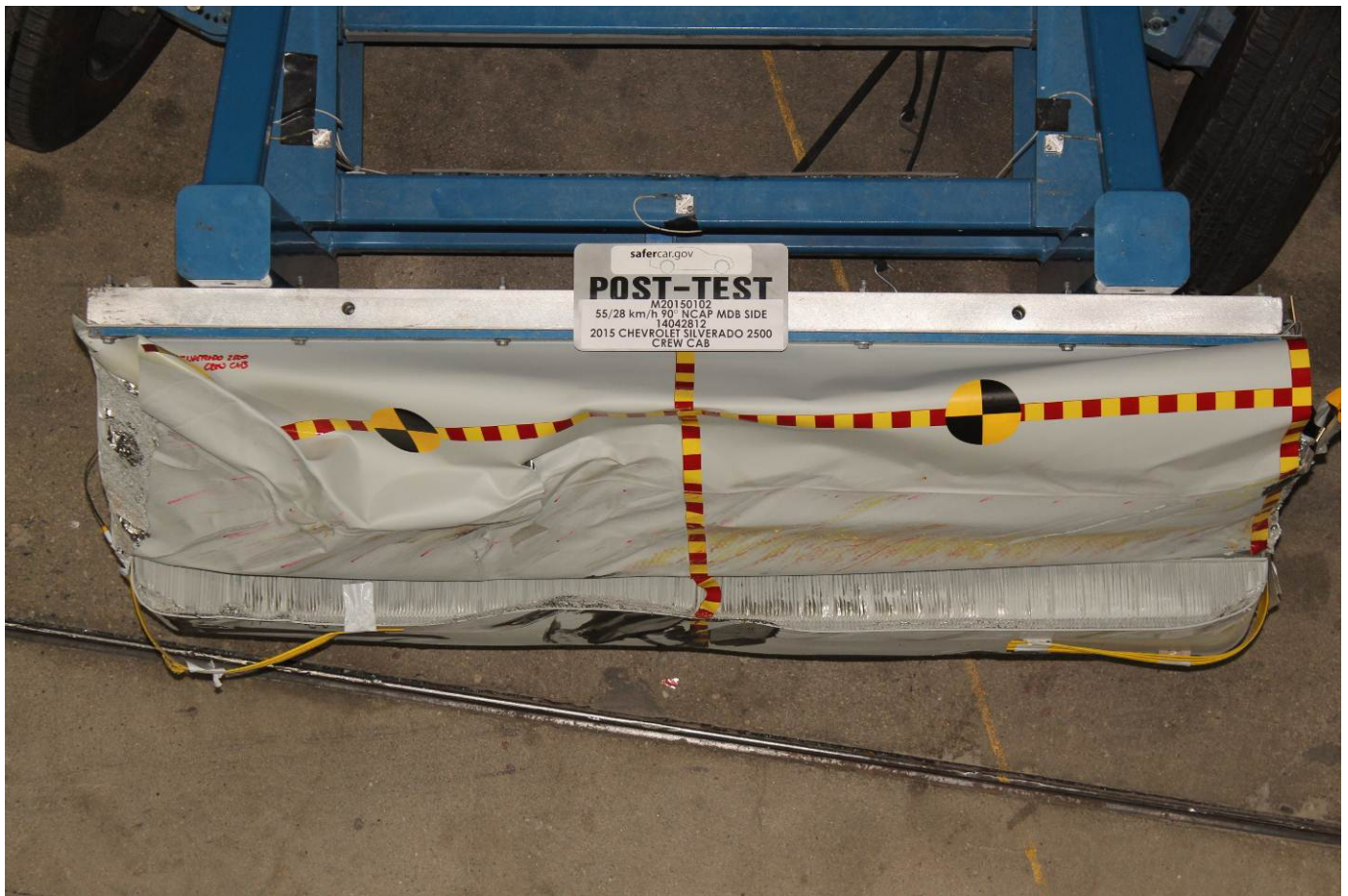
Post-Test Top View of MDB Impactor Face
