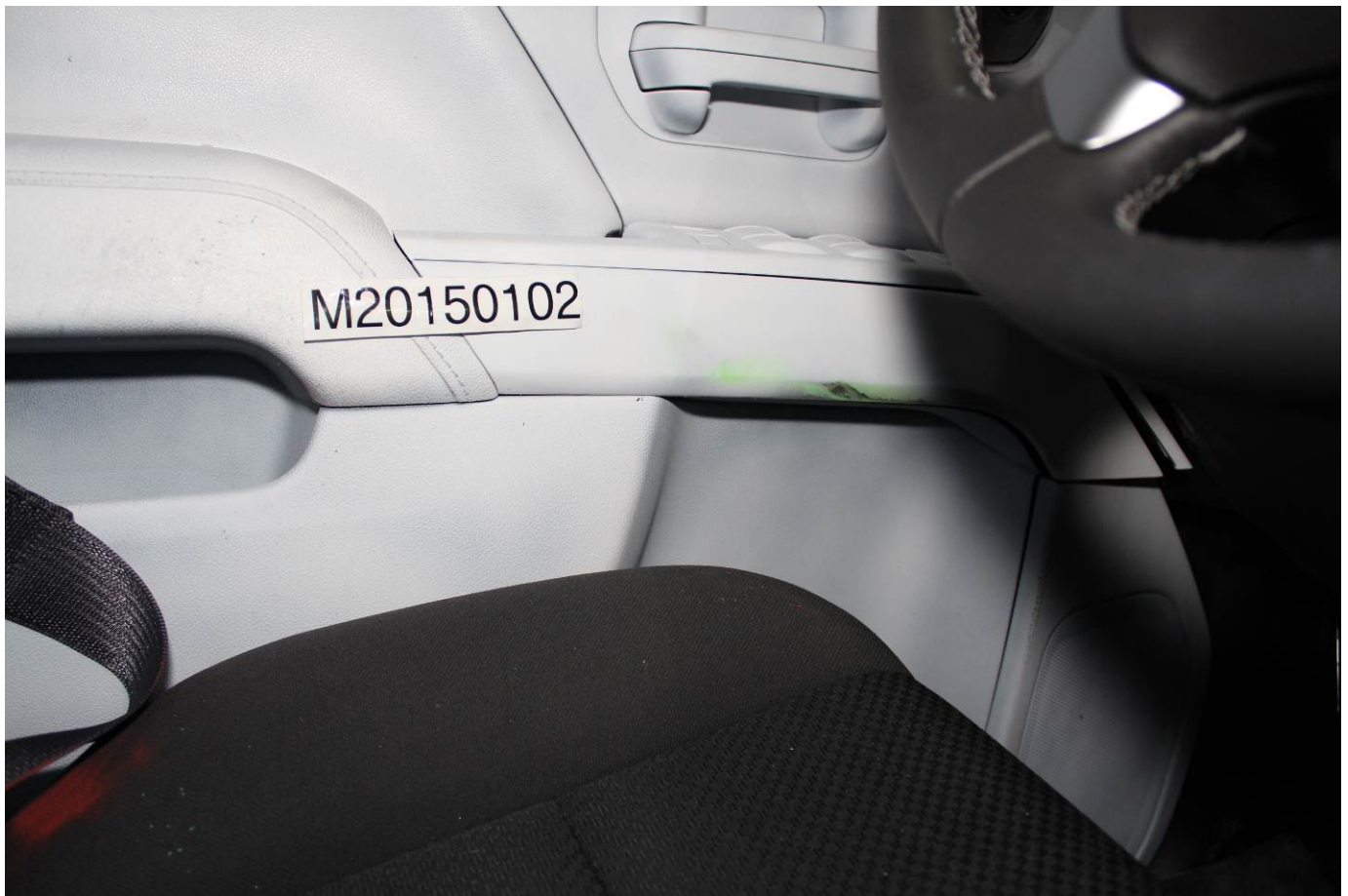
Post-Test Driver Dummy Close-up Knee Contact View
