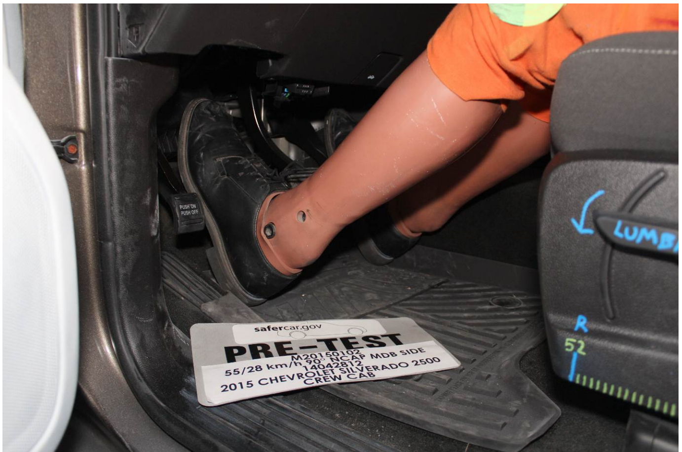
Pre-Test Placement of Driver Dummy's Feet
