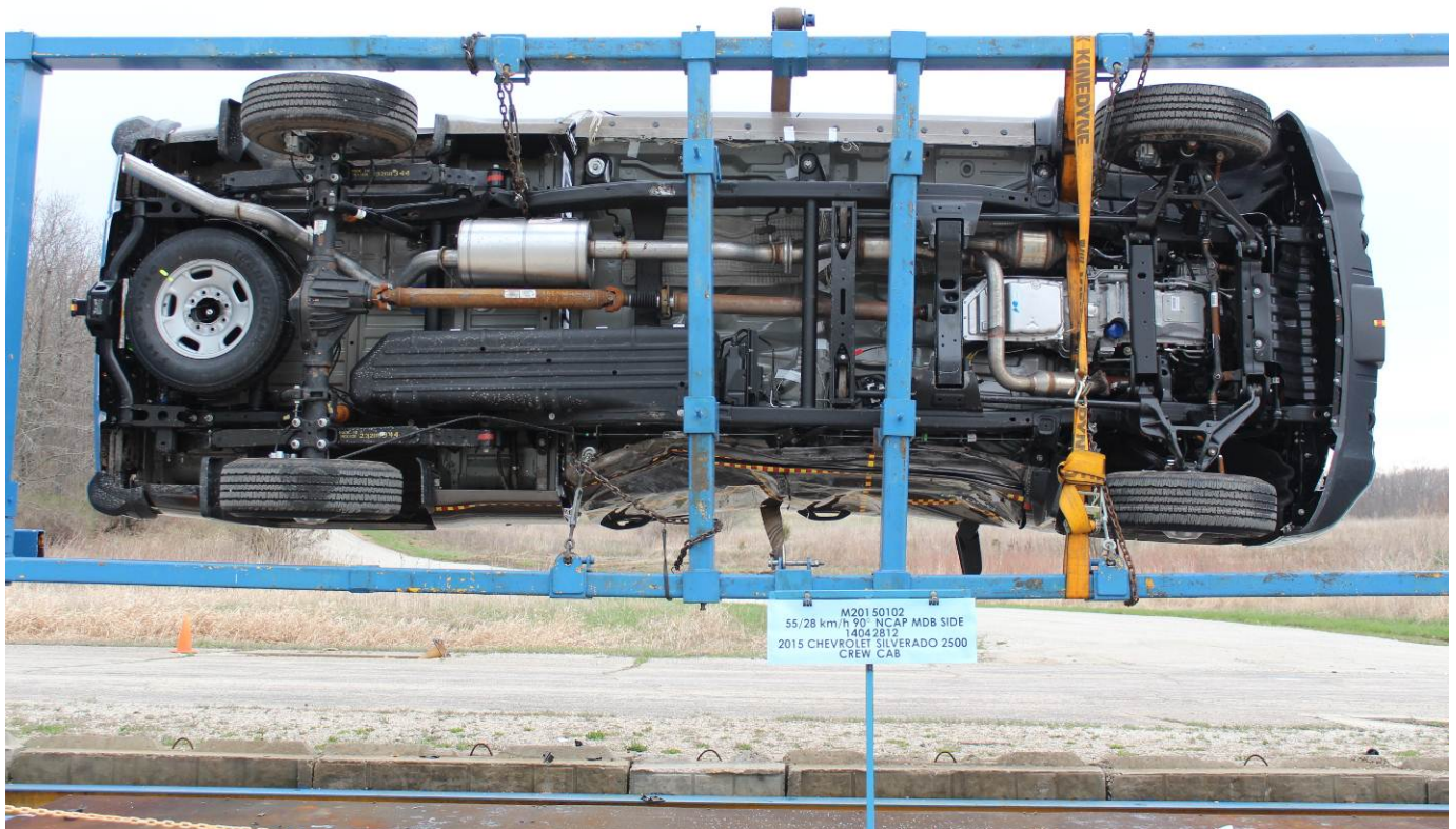
FMVSS No. 301 Static Rollover 90 Degrees
