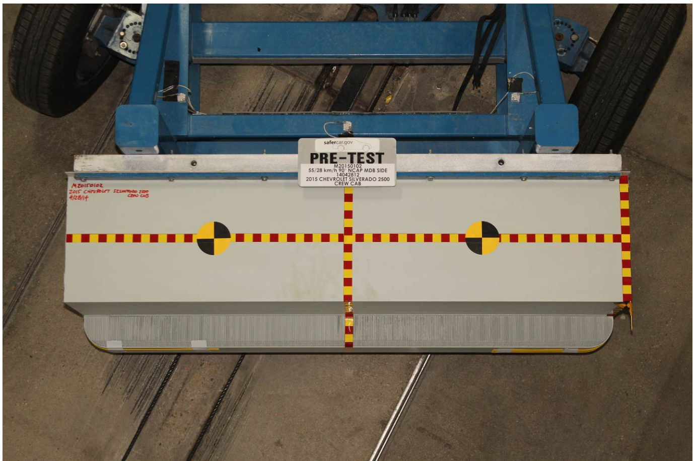
Pre-Test Top View of MDB Impactor Face
