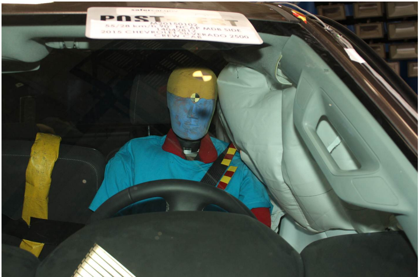
Post-Test Front Close-Up View of Driver Dummy
