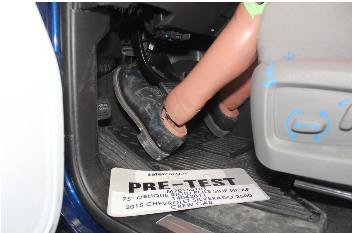
Pre-Test Placement of Dummy's Feet
