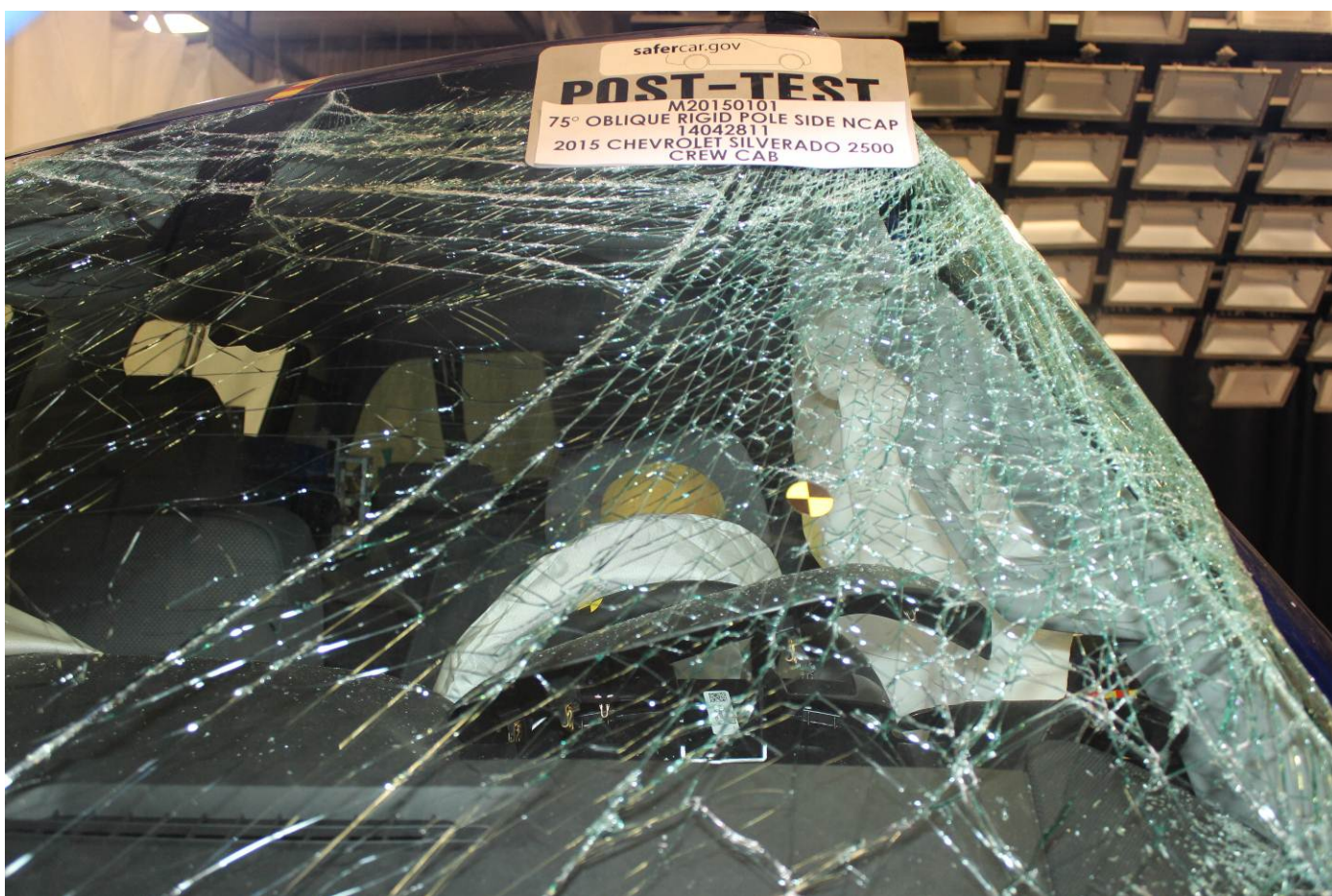
Post-Test Front Close-Up View of Dummy
