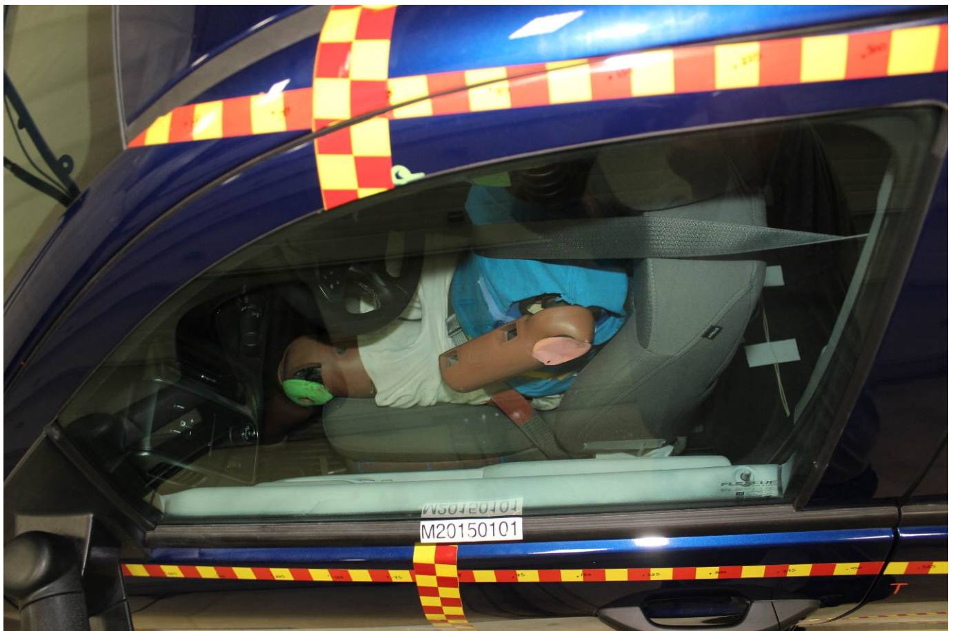
Pre-Test Dummy and Door Clearance View
