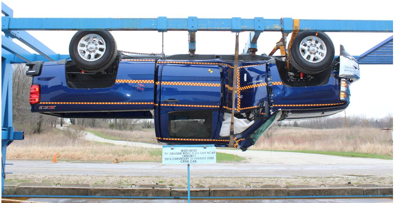
FMVSS No. 301 Static Rollover 180 Degrees
