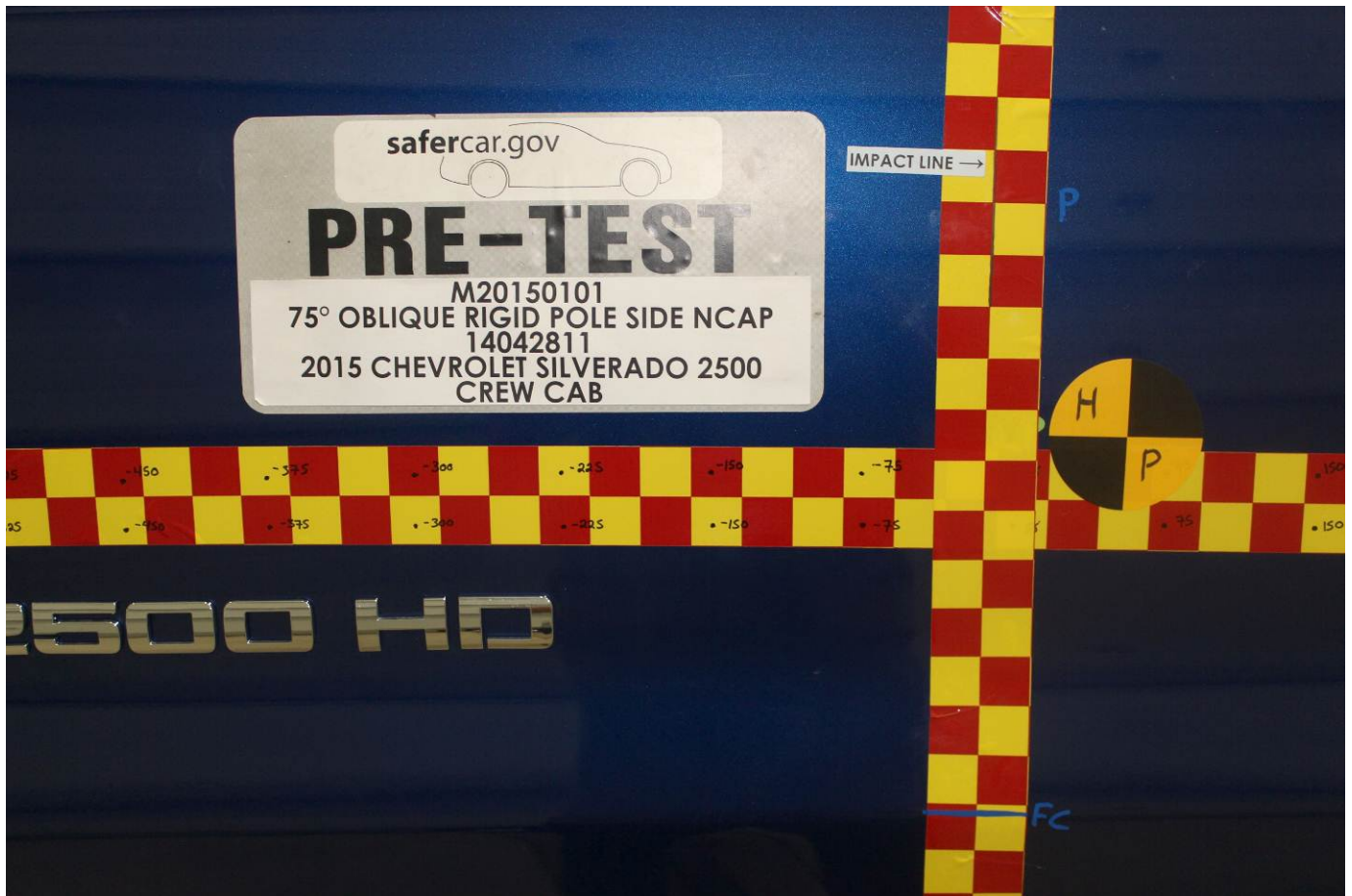
Pre-Test Close-Up View of Impact Point Target
