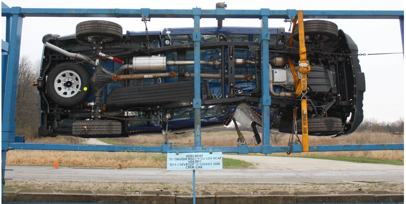
FMVSS No. 301 Static Rollover 90 Degrees
