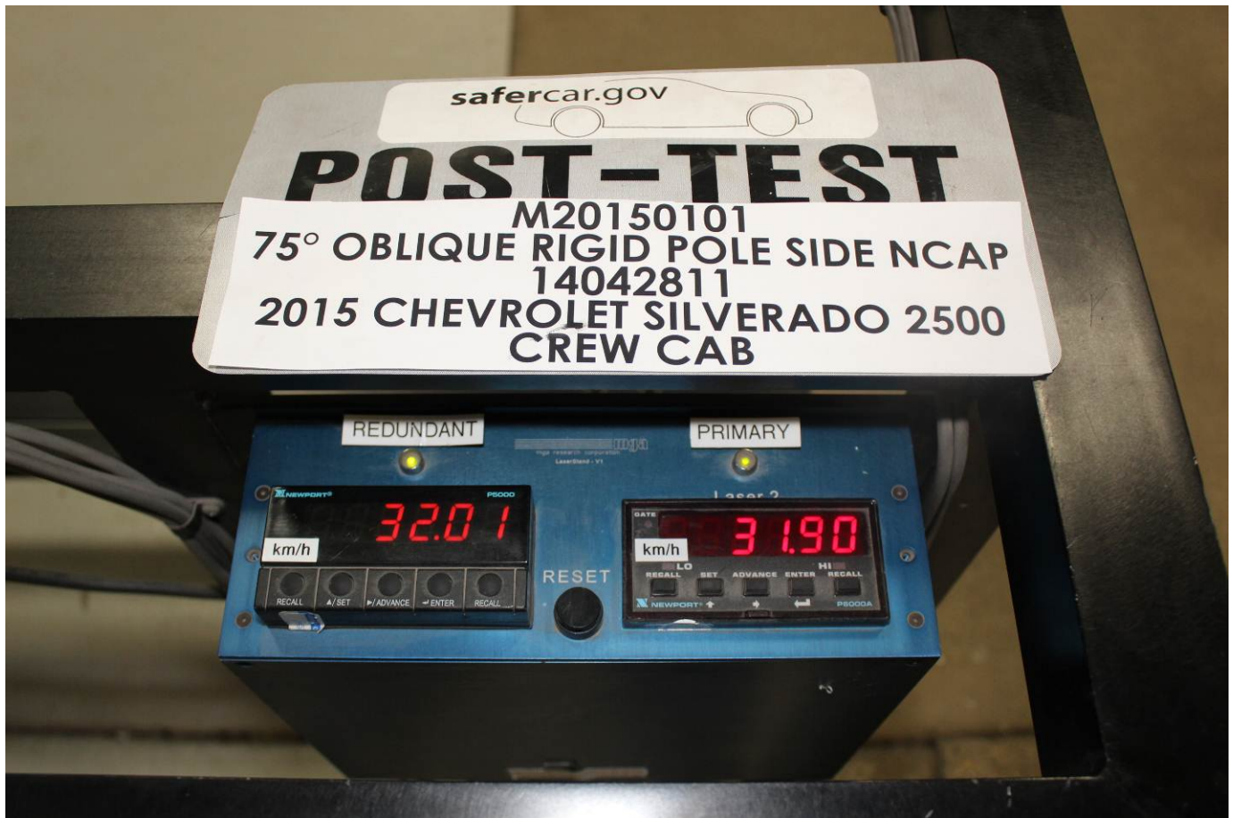
Post-Test Primary and Redundant Speed Trap Read-Out
