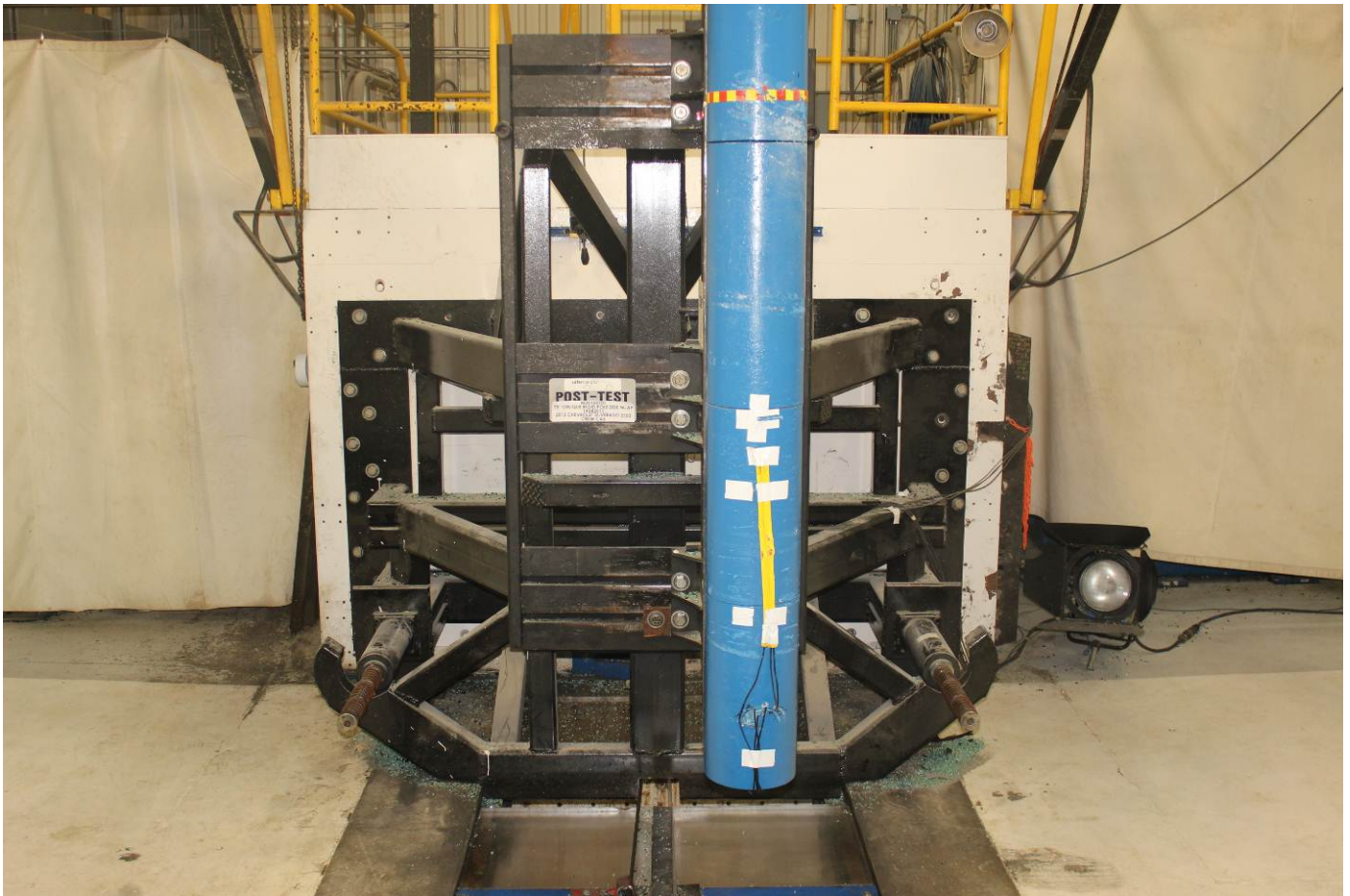
Post-Test Pole Barrier Front View
