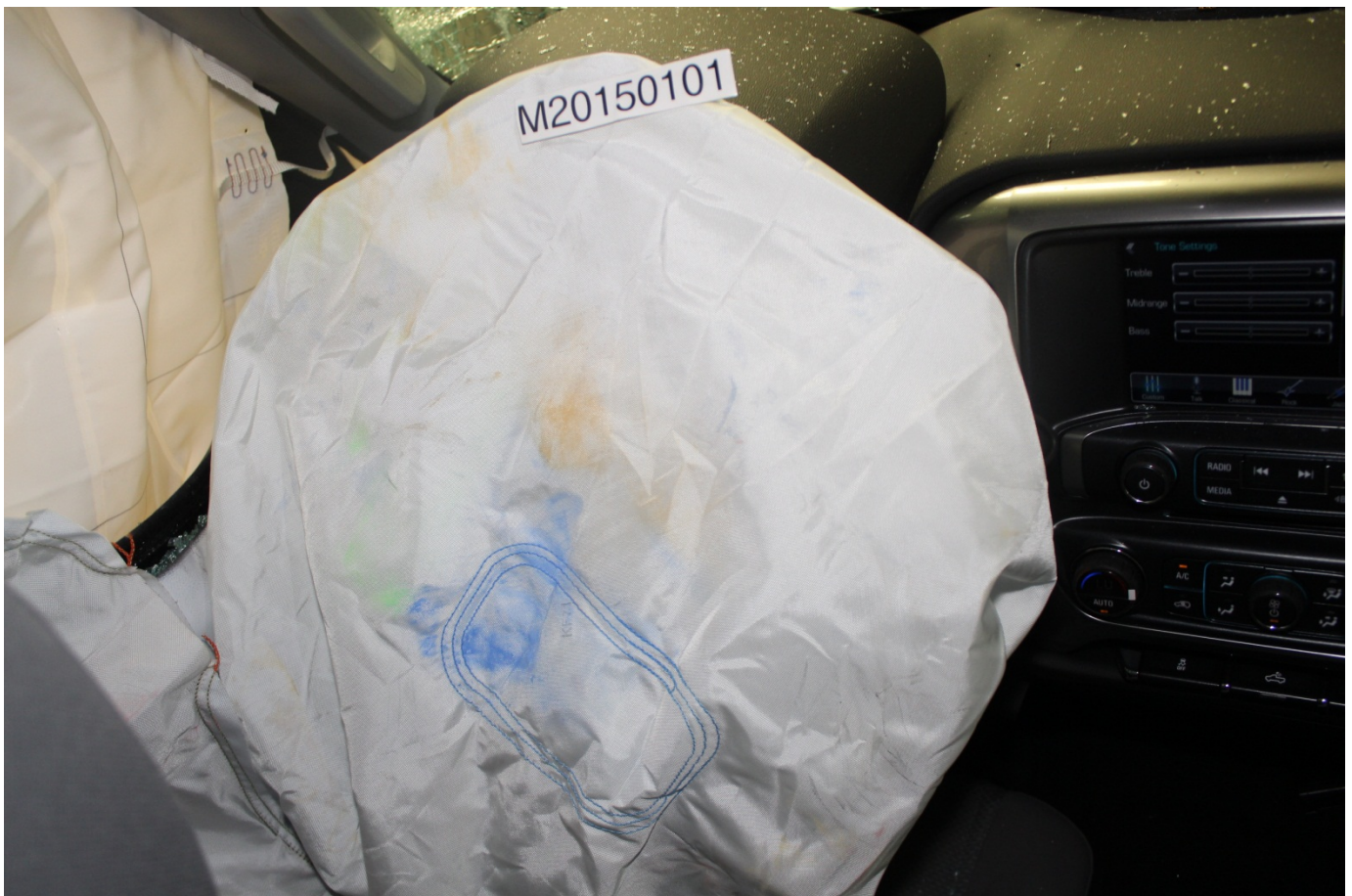
Post-Test Dummy Close-Up Head Contact with Frontal Air Bag View
