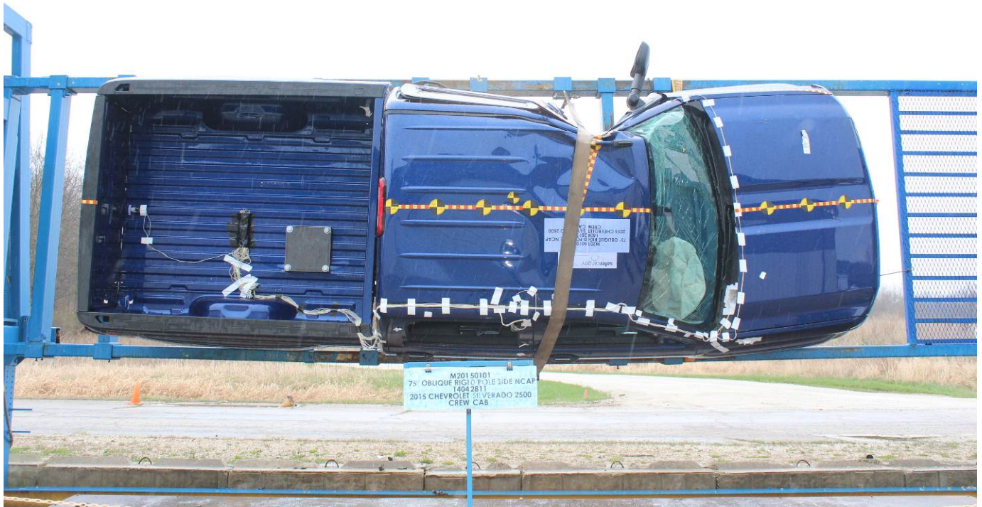
FMVSS No. 301 Static Rollover 270 Degrees
