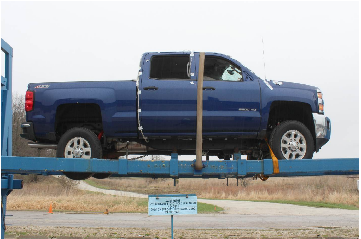
FMVSS No. 301 Static Rollover 0 Degrees
