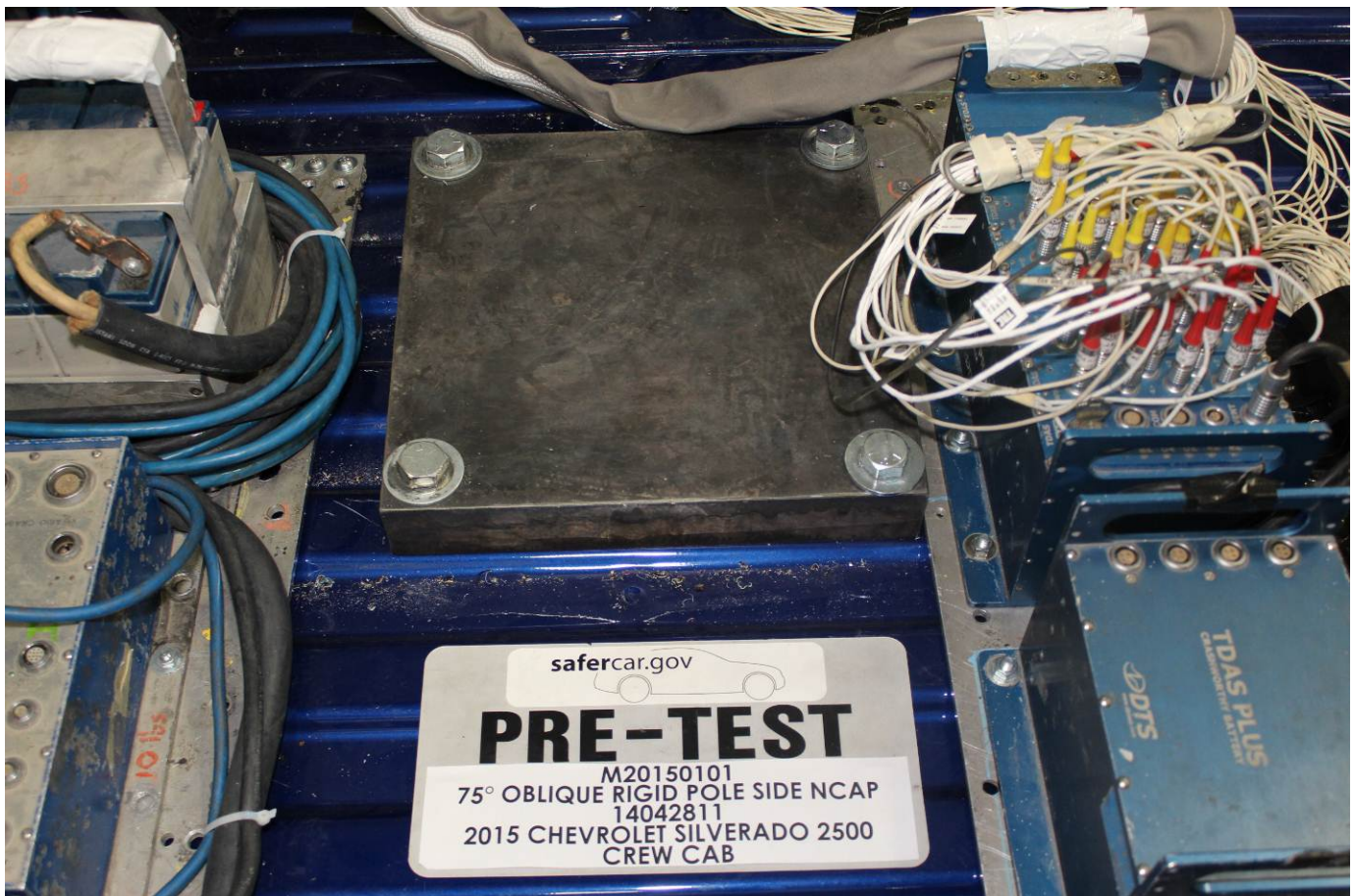
Pre-Test Ballast View
