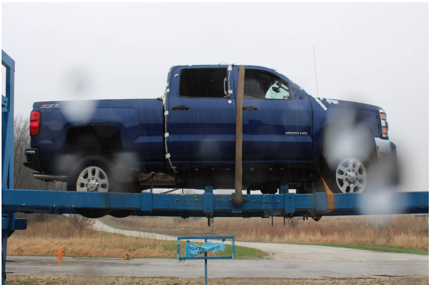
FMVSS No. 301 Static Rollover 360 Degrees
