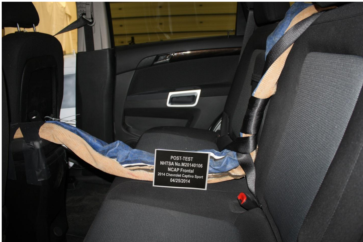
Figure A-28: Post-Test Dummy Cable Routing
