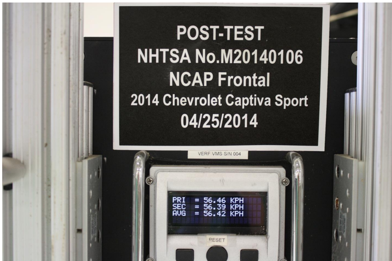
Figure A-71: Post-Test Speed Trap Read-Out
