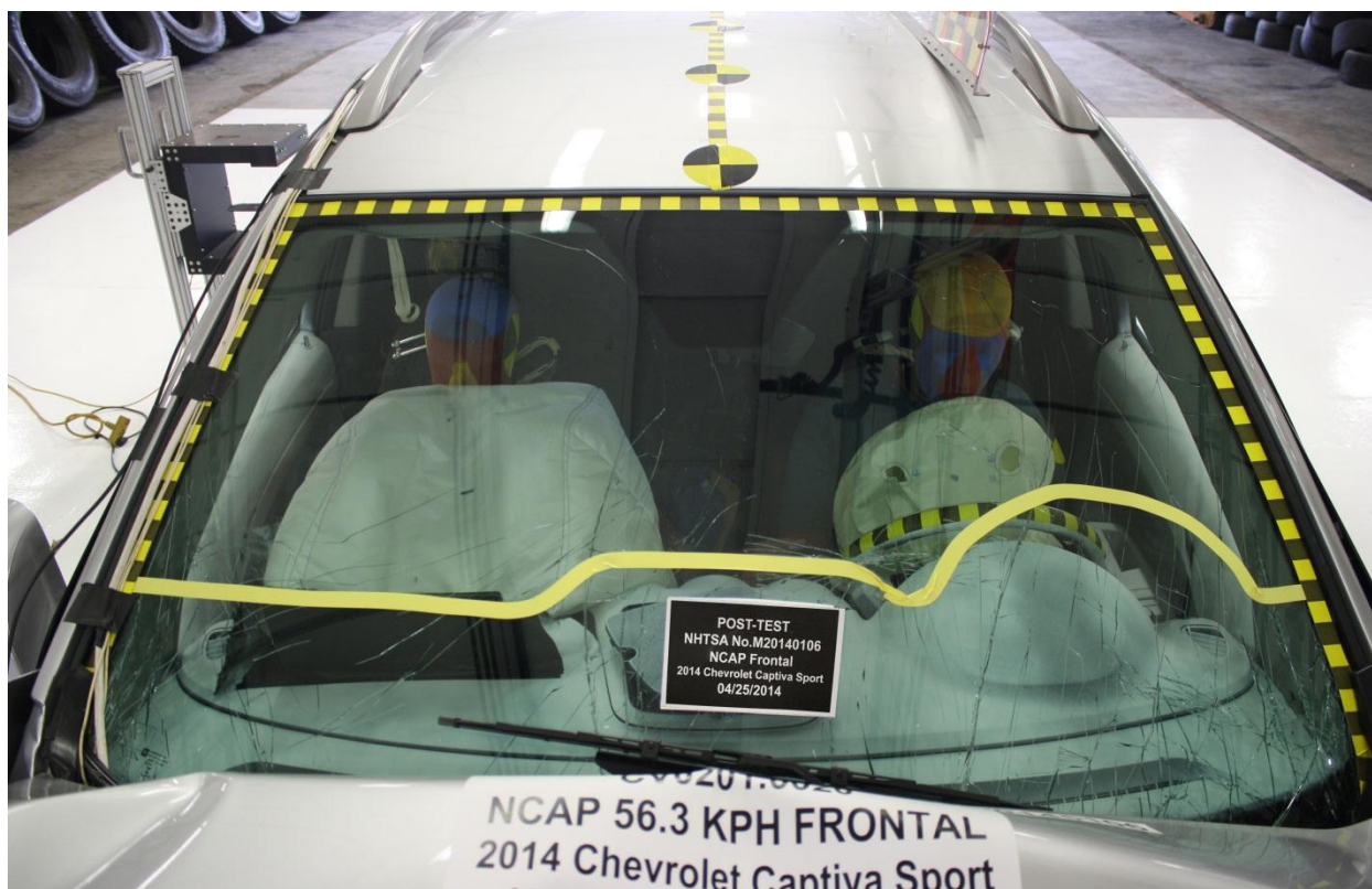
Figure A-18: Post-Test Windshield View
