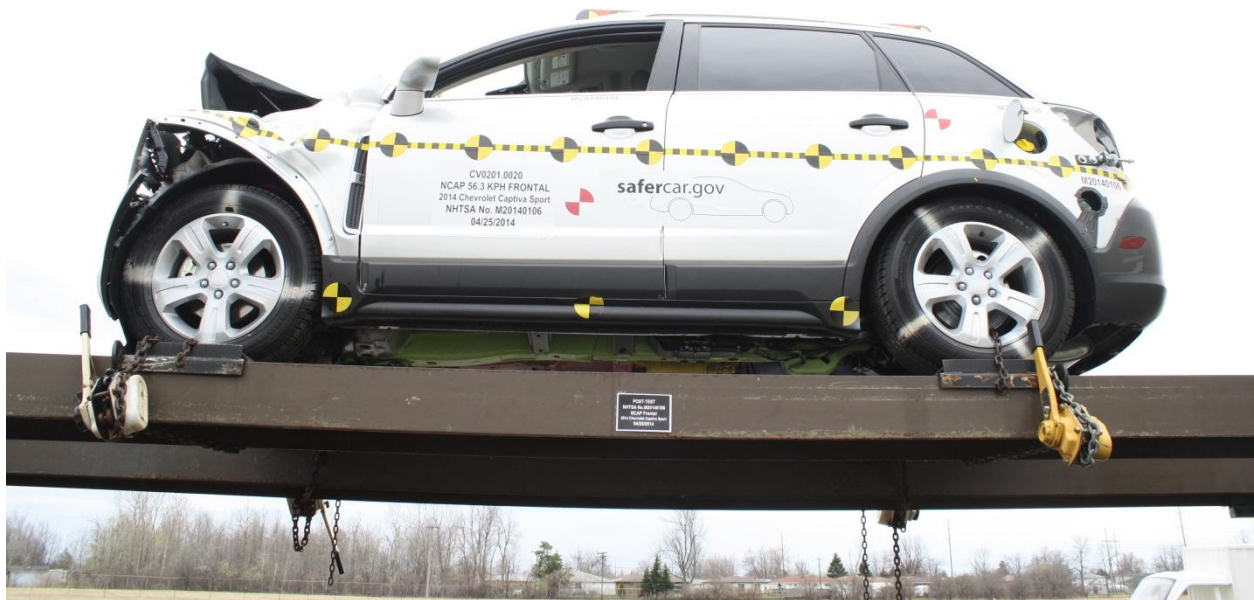
Figure A-76: Vehicle at 360° on Static Rollover Device
