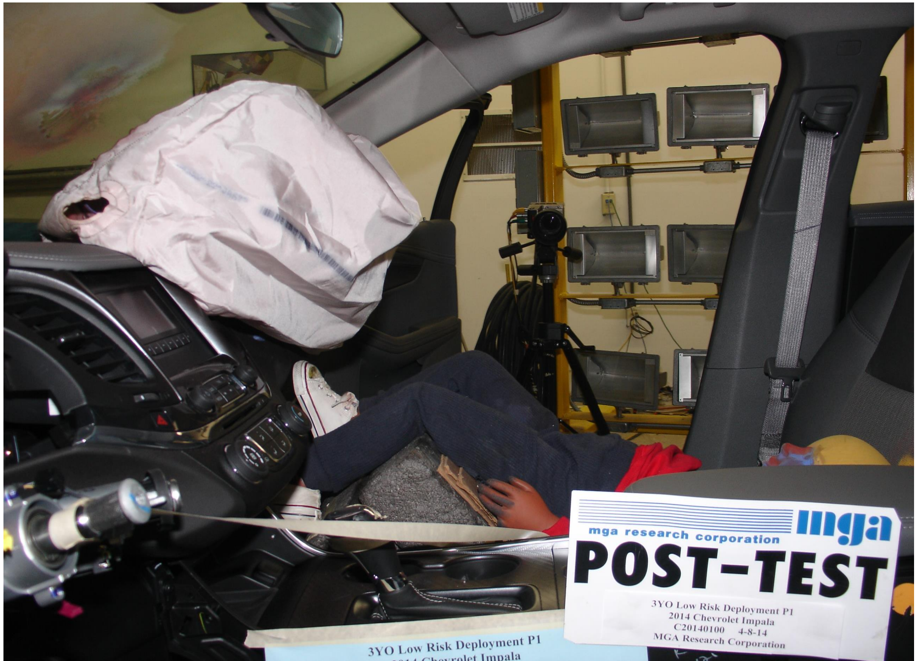
Post-Test 3YO P1 Passenger Dummy Left Side View
