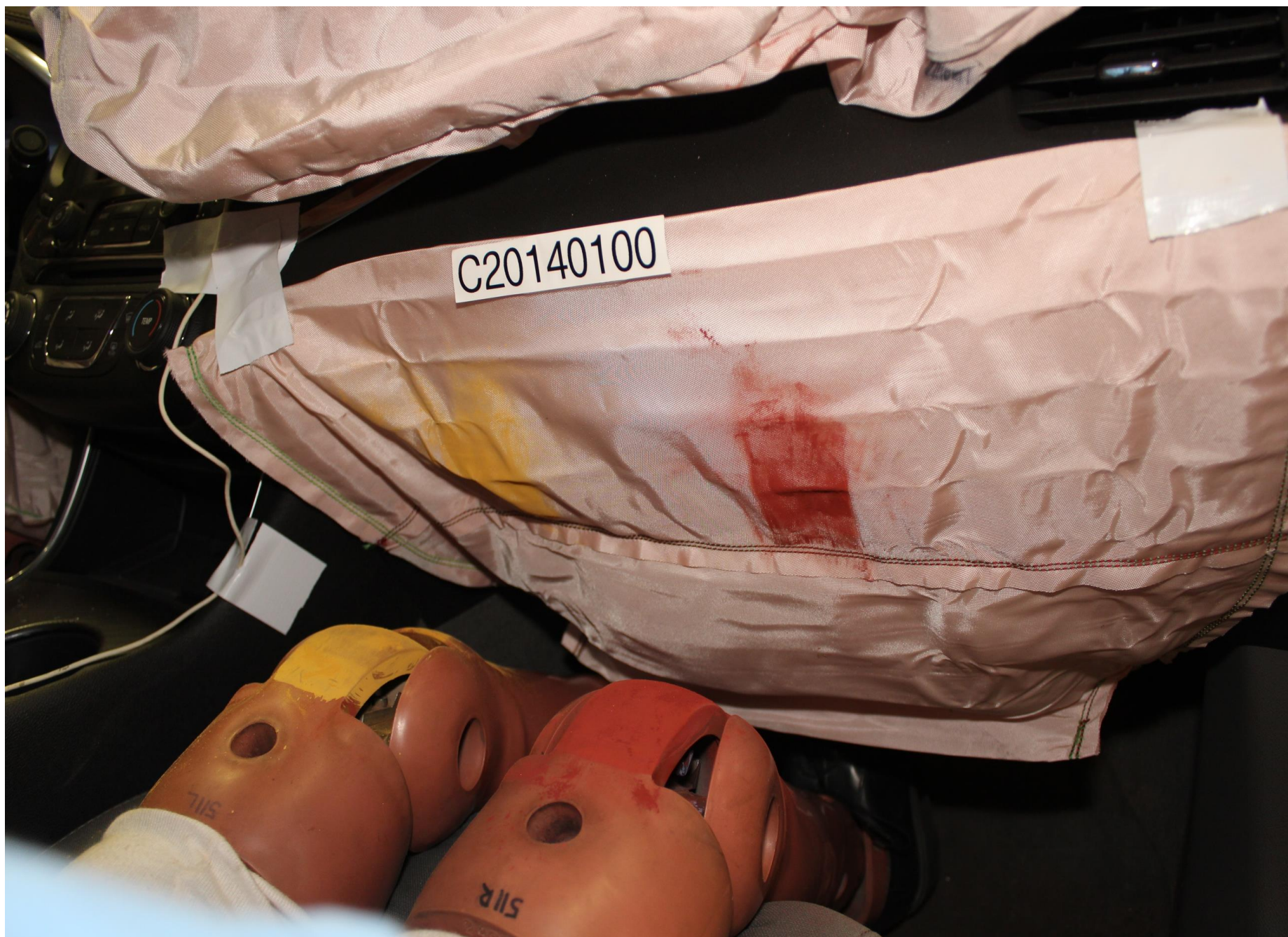
Post-Test Passenger Dummy Knee Contact
