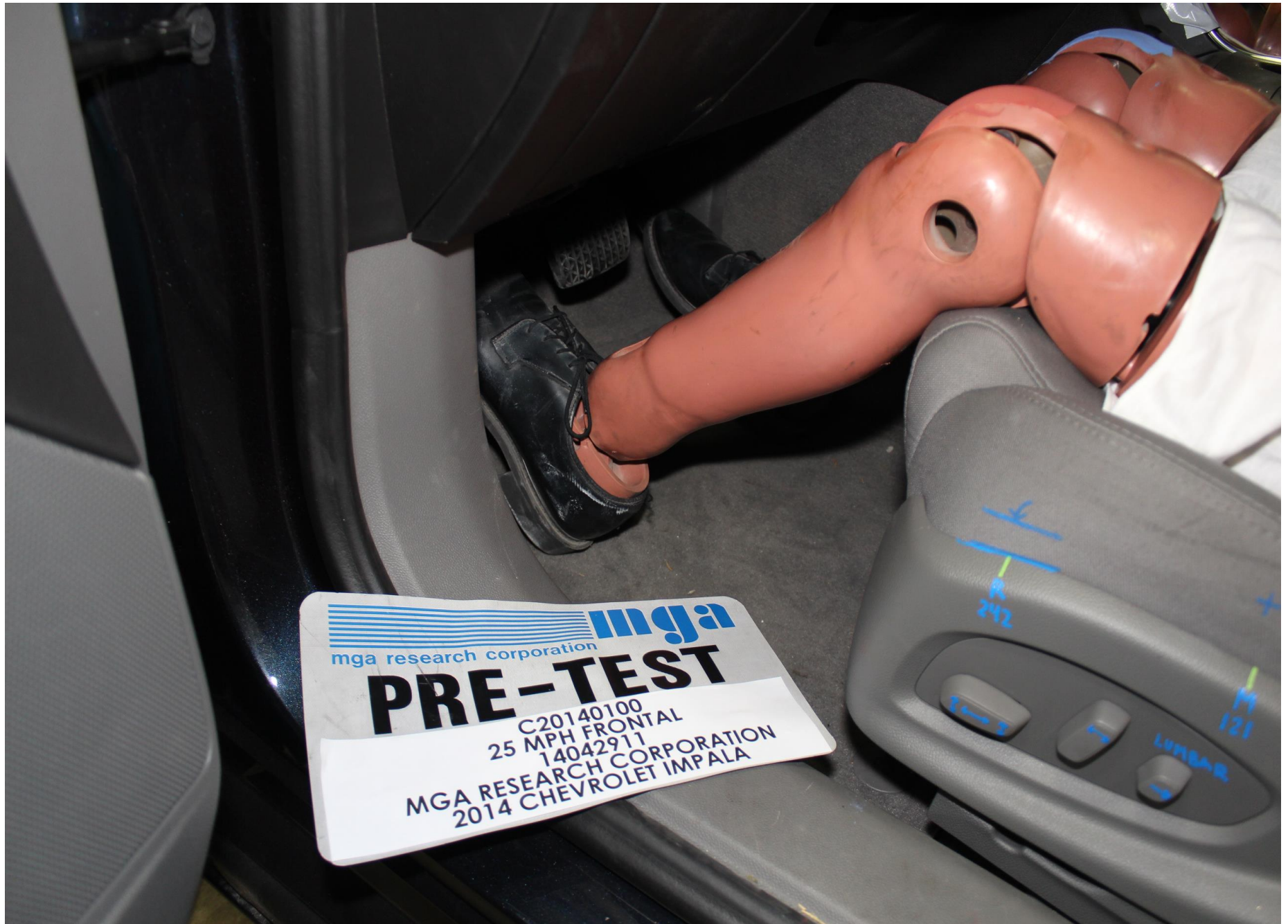
Pre-Test Driver Dummy Feet Position
