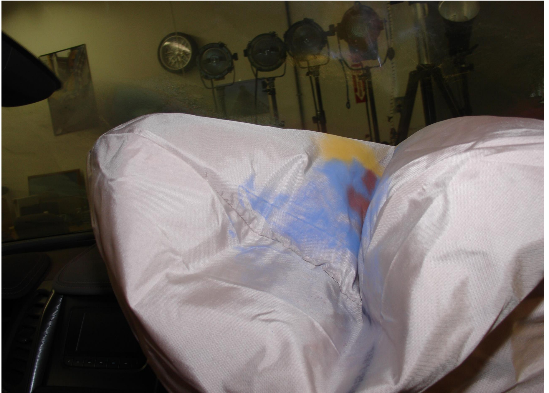
Post-Test 6YO P1 Passenger Dummy Airbag Right Side View
