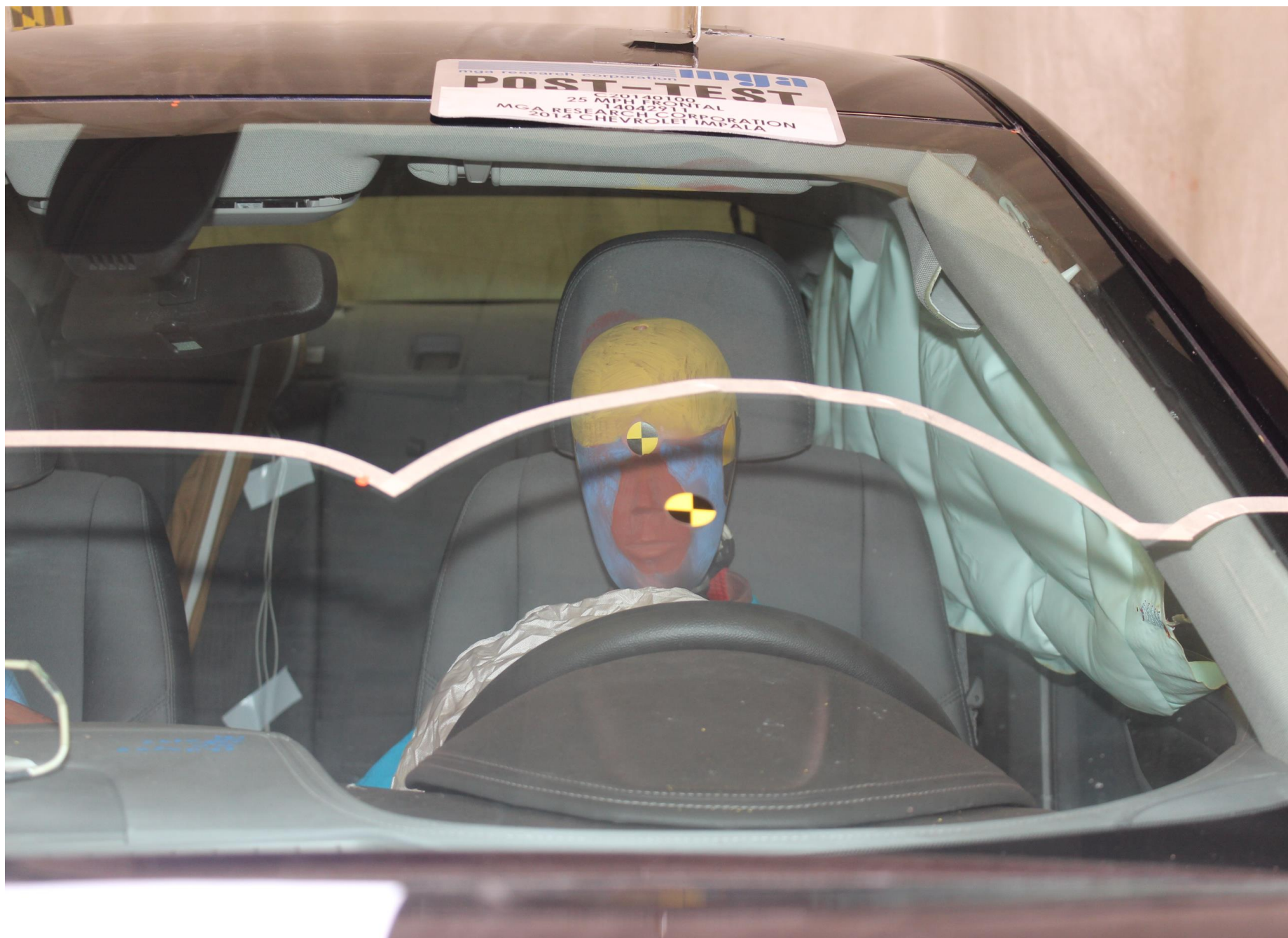
Post-Test Driver Dummy Front View (head position)
