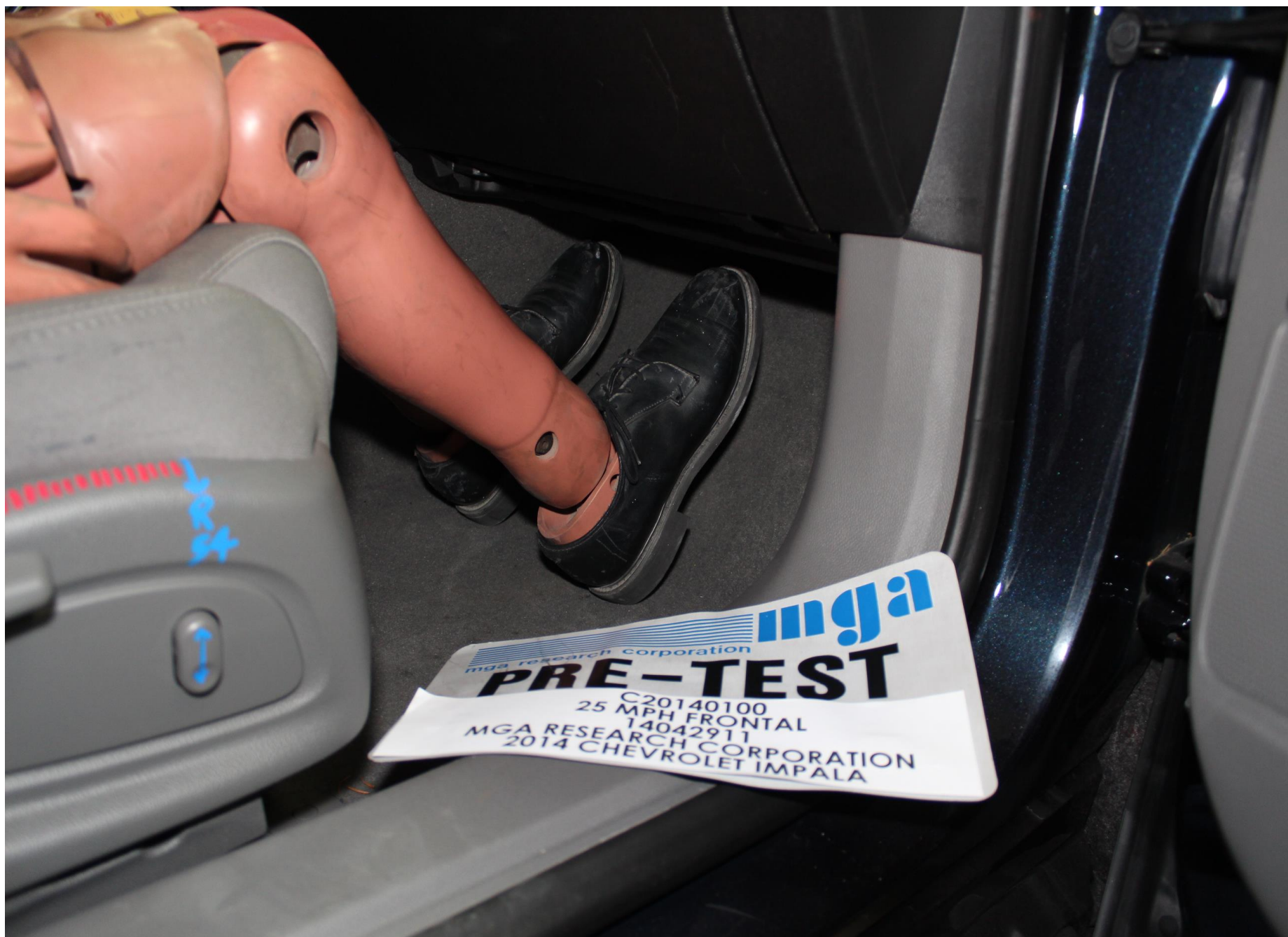
Pre-Test Passenger Dummy Feet Position
