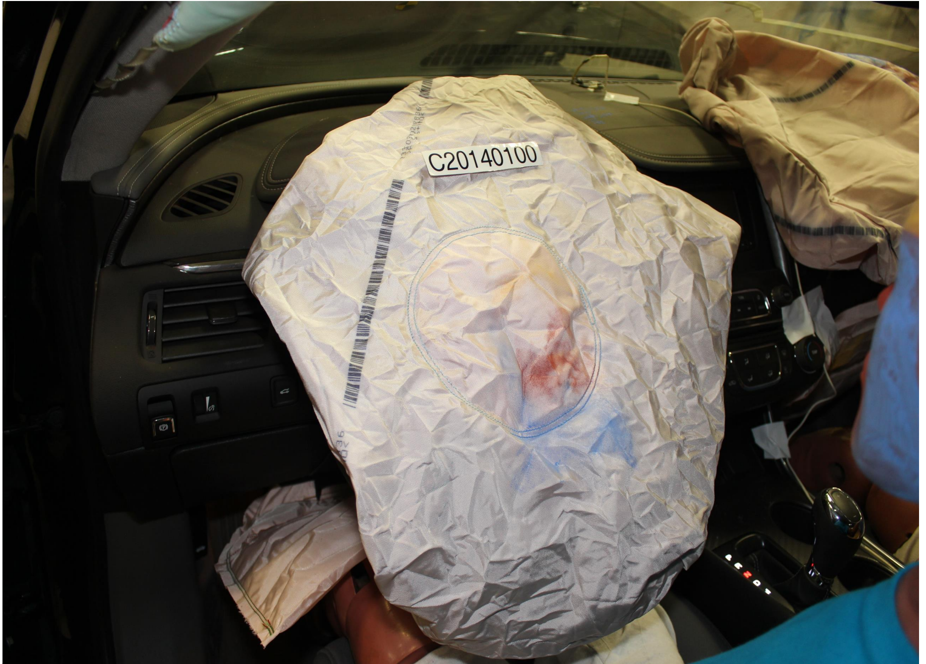
Post-Test Driver Dummy Airbag Contact
