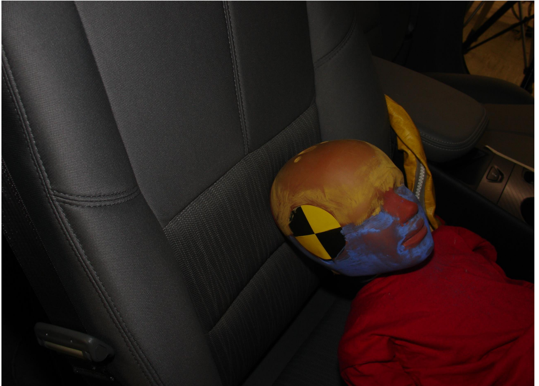
Post-Test 3YO P2 Passenger Dummy Head Contact (seat back)
