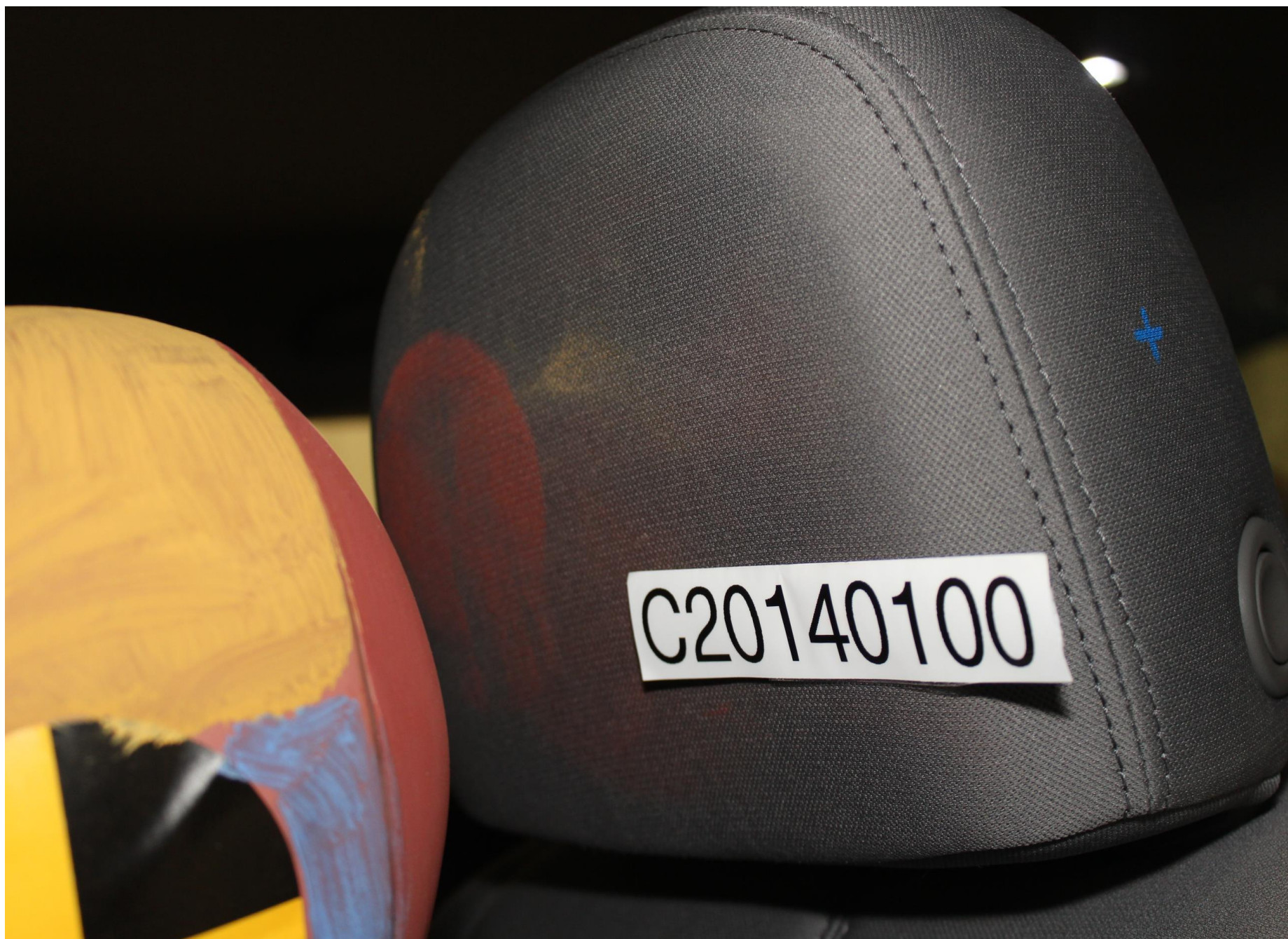
Post-Test Driver Dummy Head Contact (headrest)
