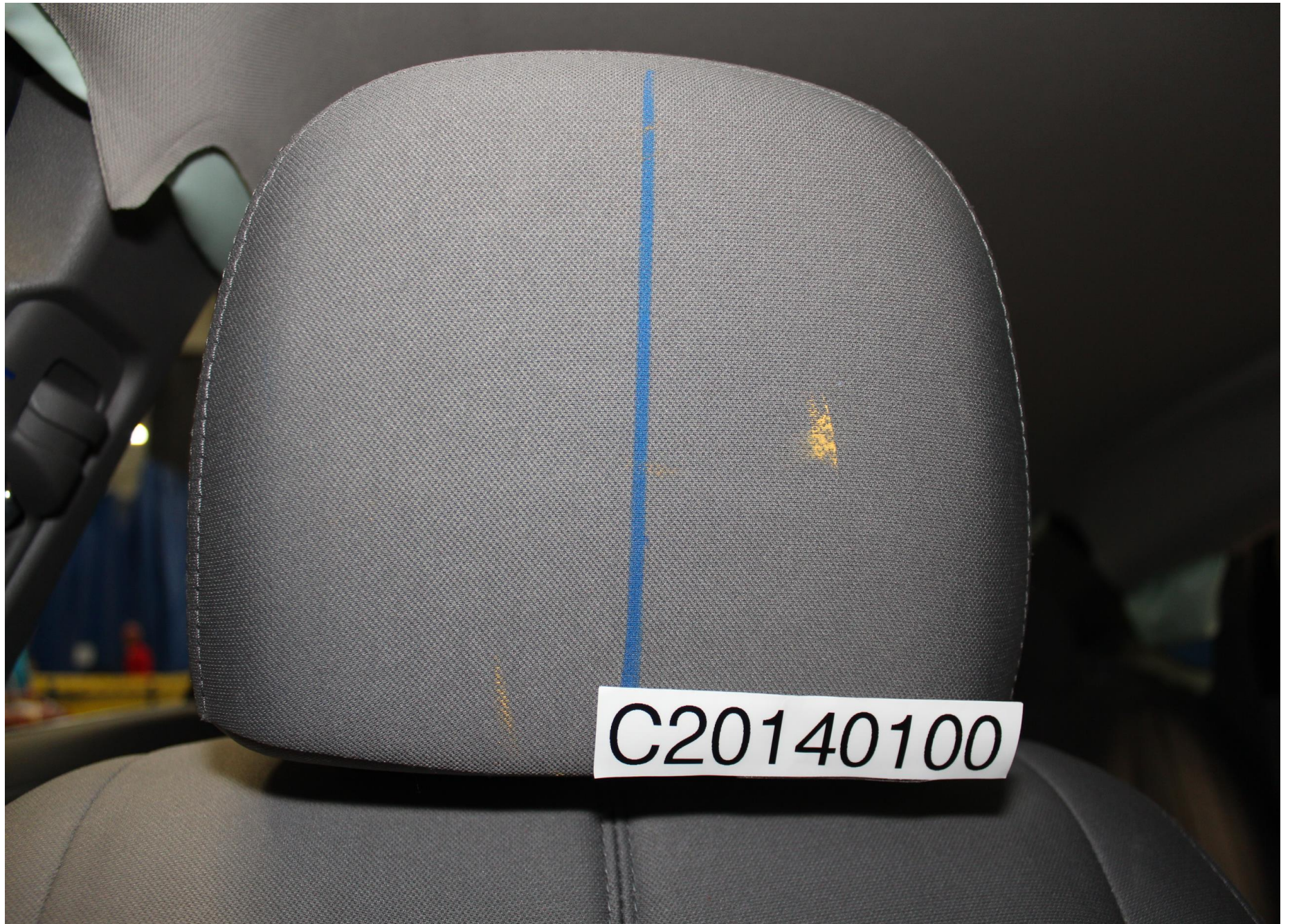
Post-Test Passenger Dummy Head Contact (headrest)
