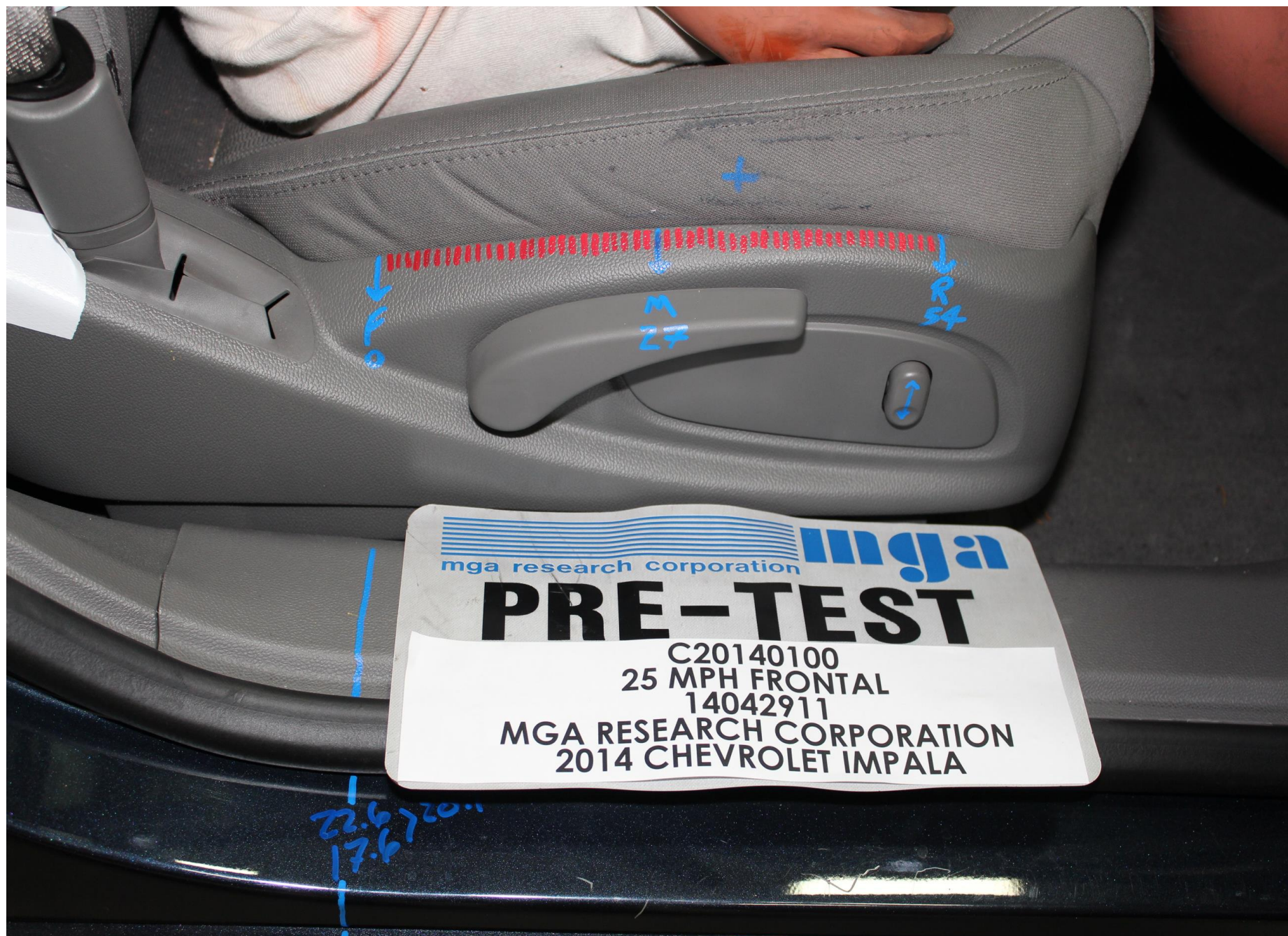
Pre-Test Passenger Dummy Seat Position
