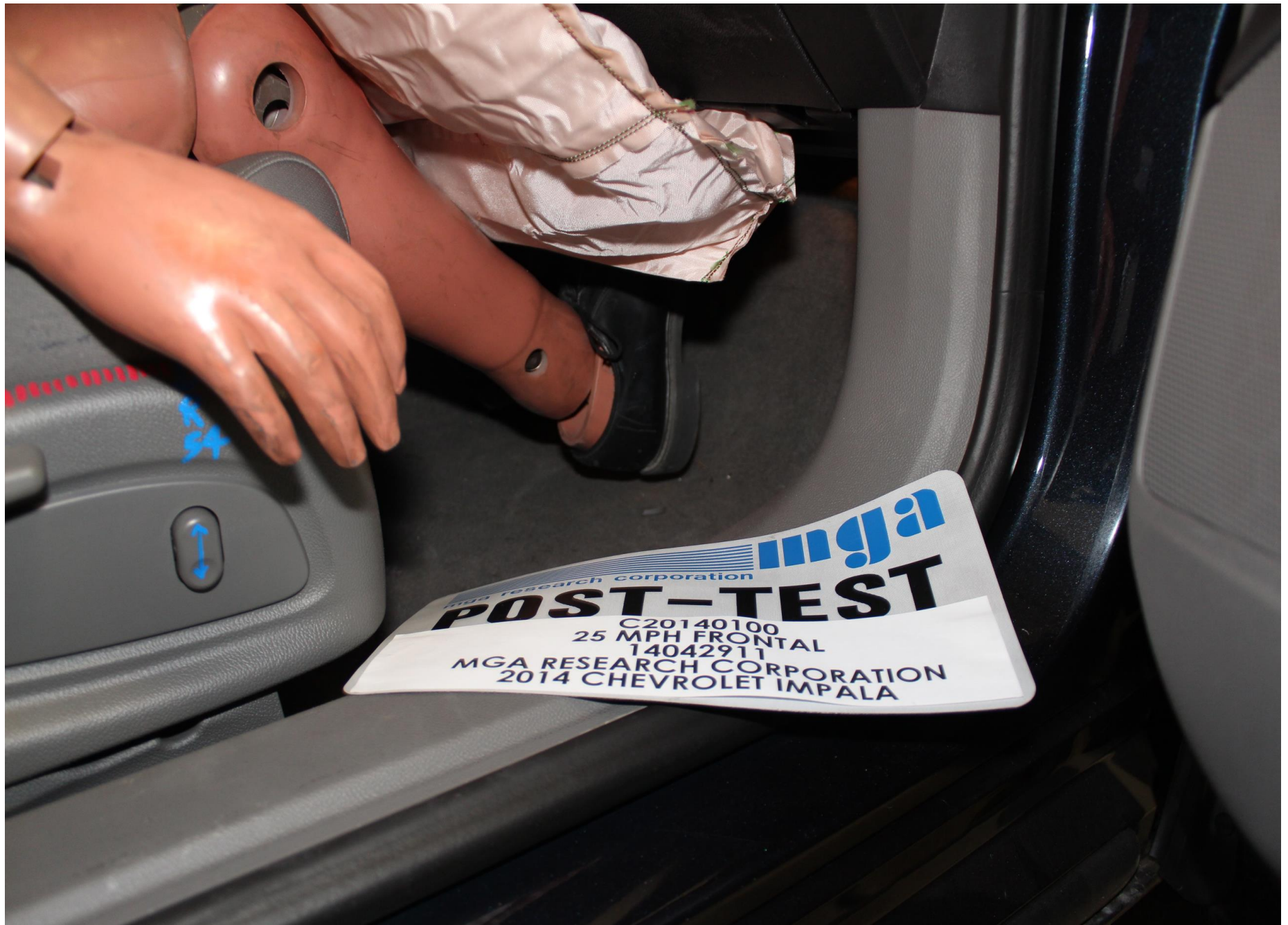
Post-Test Passenger Dummy Feet Position
