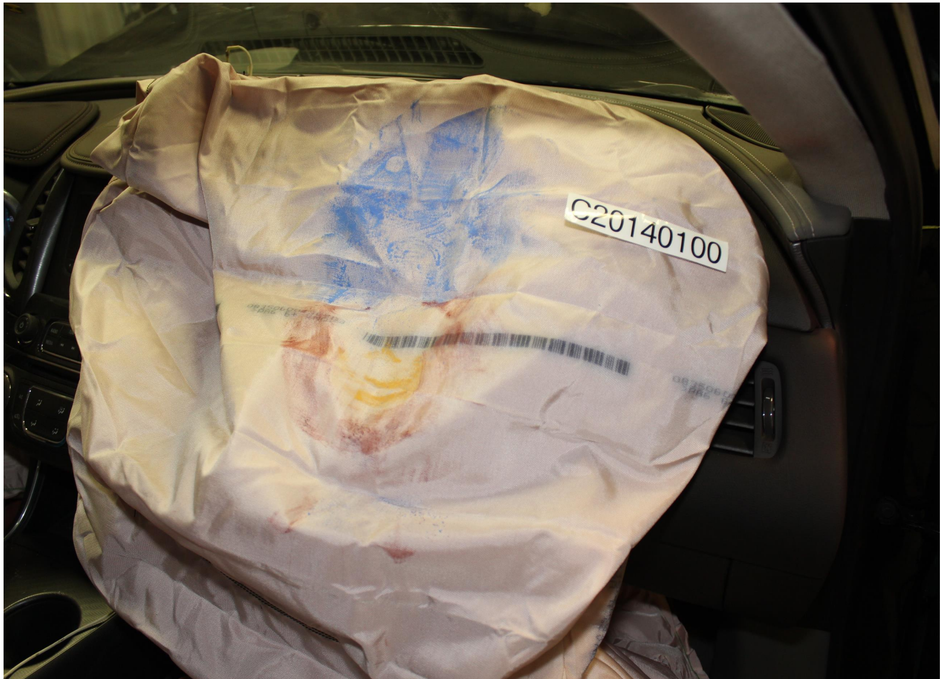
Post-Test Passenger Dummy Airbag Contact
