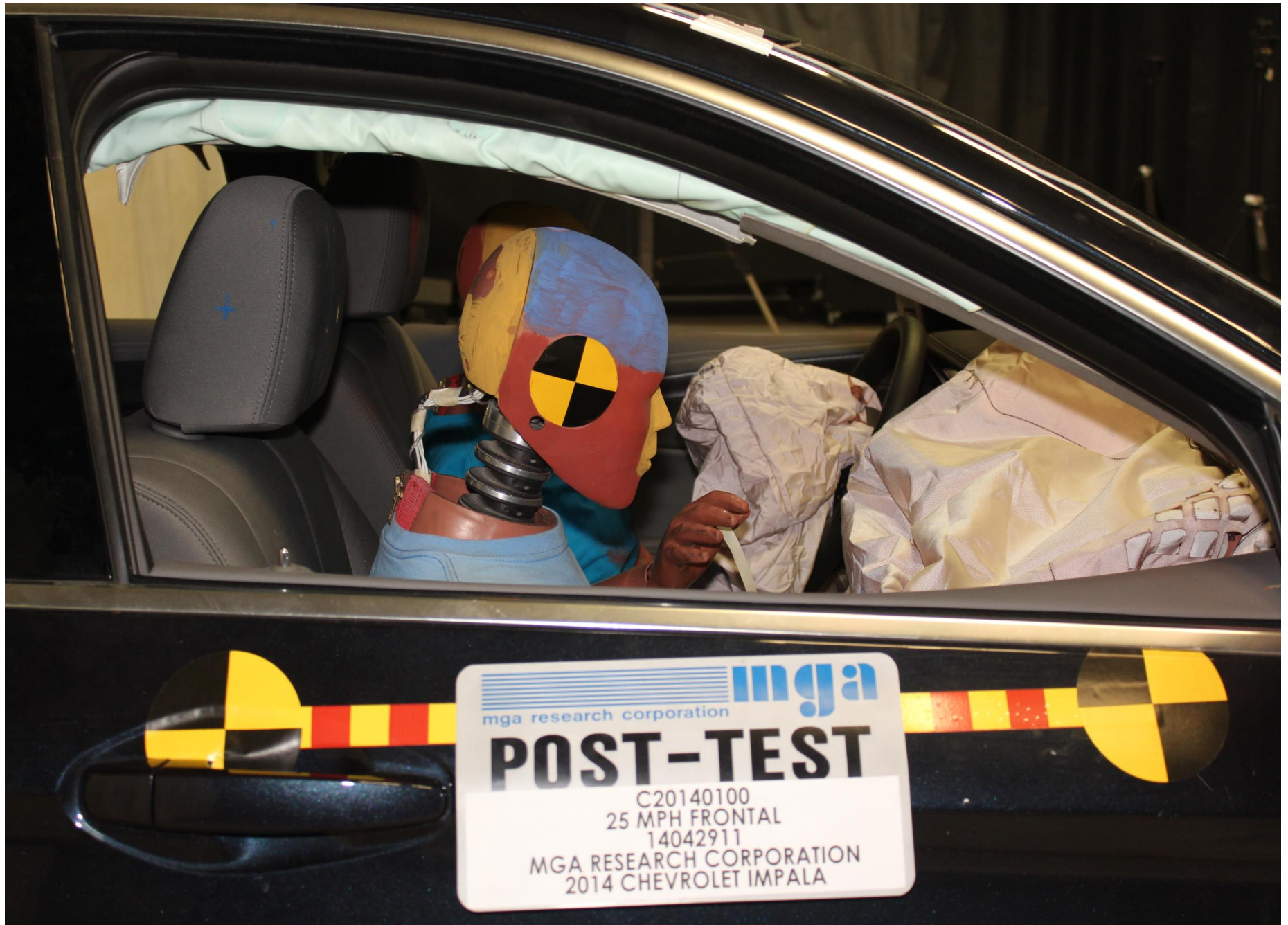
Post-Test Passenger Dummy Position Right Side View
