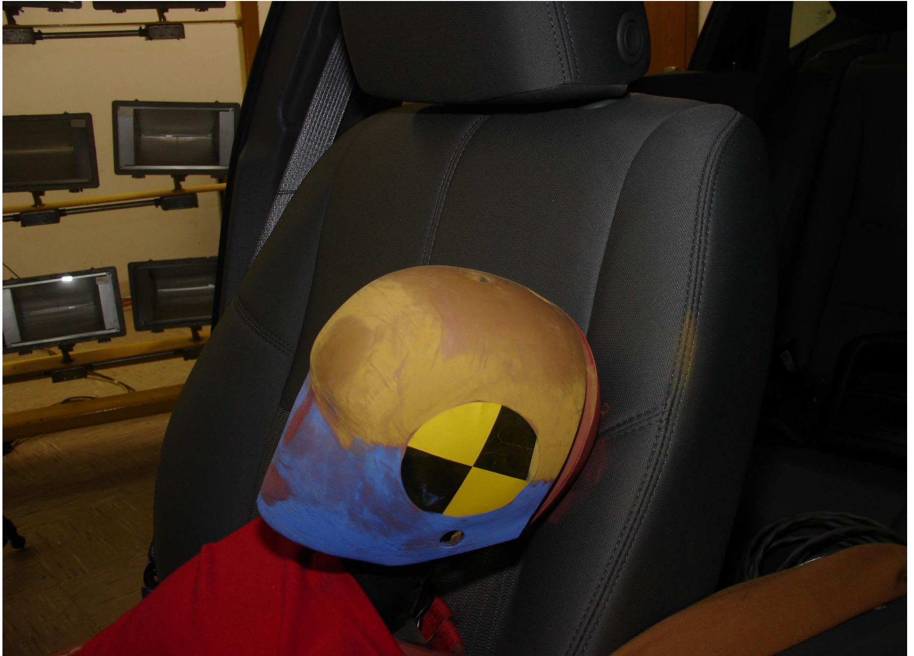
Post-Test 6YO P2 Passenger Dummy Head Contact (seat back)
