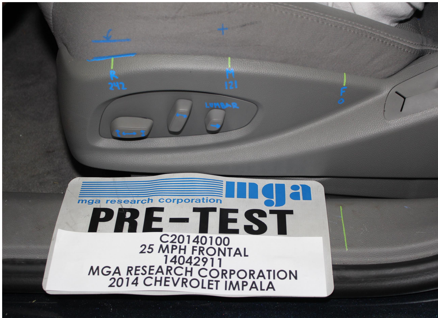
Pre-Test Driver Dummy Seat Position
