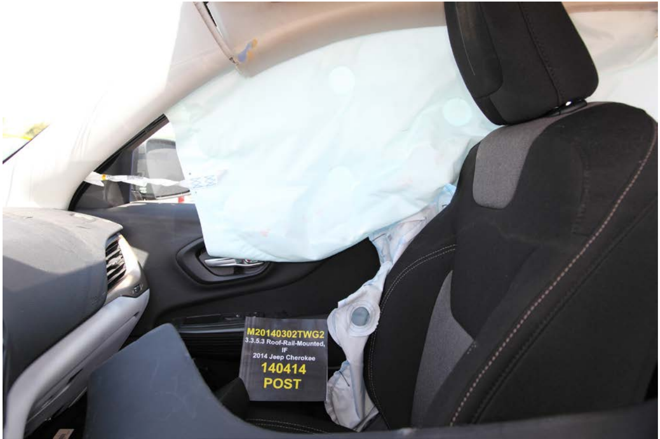
Figure A-12 Post-Test Front Passenger Airbags – Left Side View
