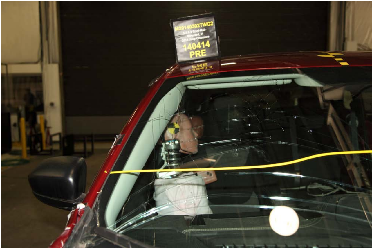
Figure A-7 Pre-Test Front Right Dummy Position – Front View
