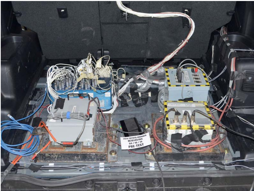
FIGURE 61. Pre-Test Ballast View
