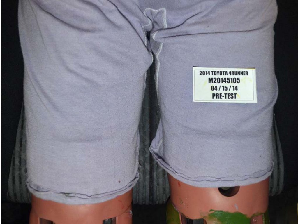
FIGURE 61. Pre-Test Overhead View of Rear Passenger Dummy Thighs on Seat Pan
