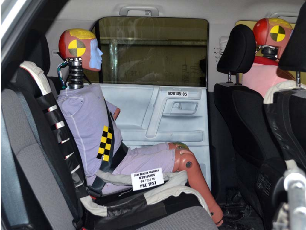
FIGURE 71. Pre-Test Right Side View of Rear Passenger Dummy and Rear Seat of Occupant Compartment
