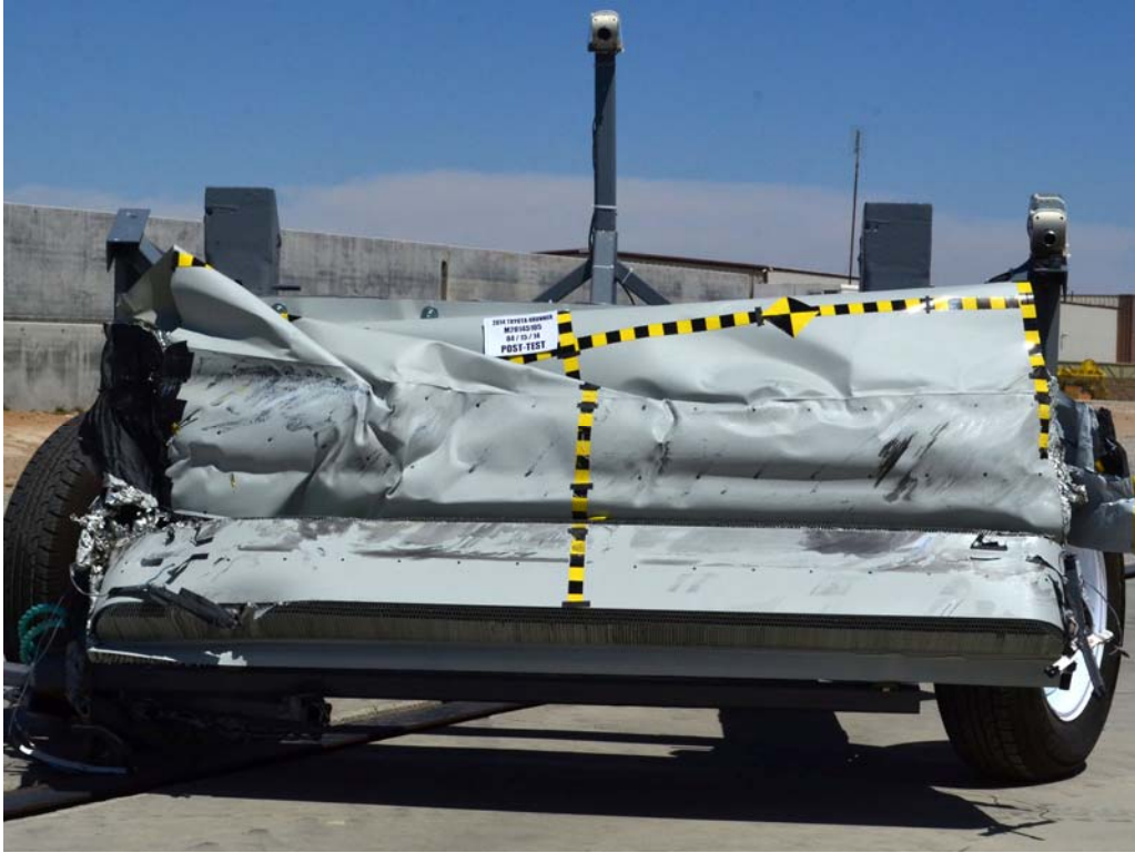
FIGURE 85. Post-Test Front View of MDB Impactor Face
