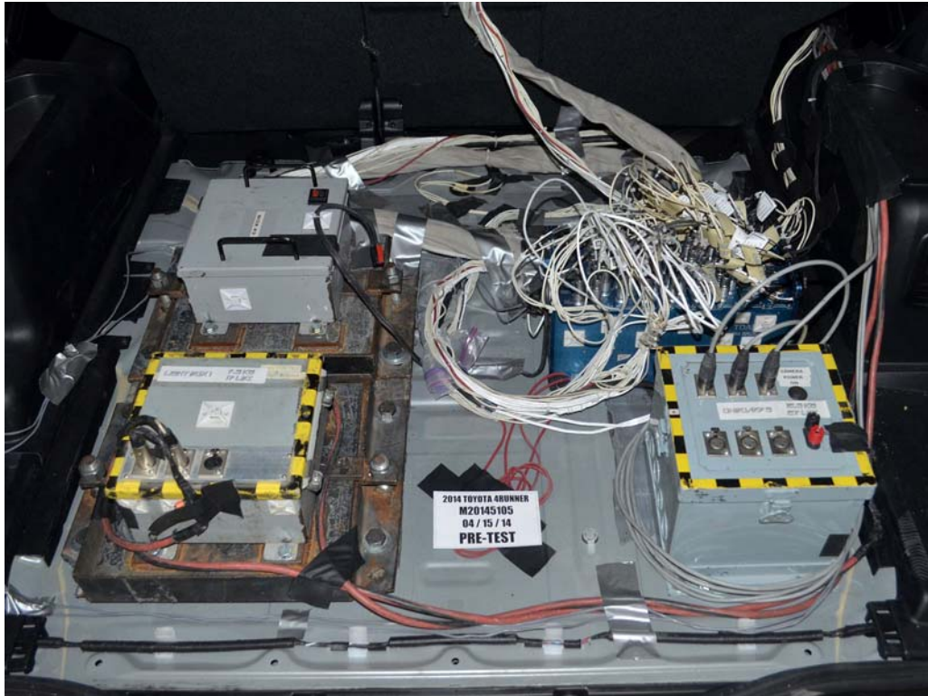
FIGURE 94. Pre-Test Ballast View
