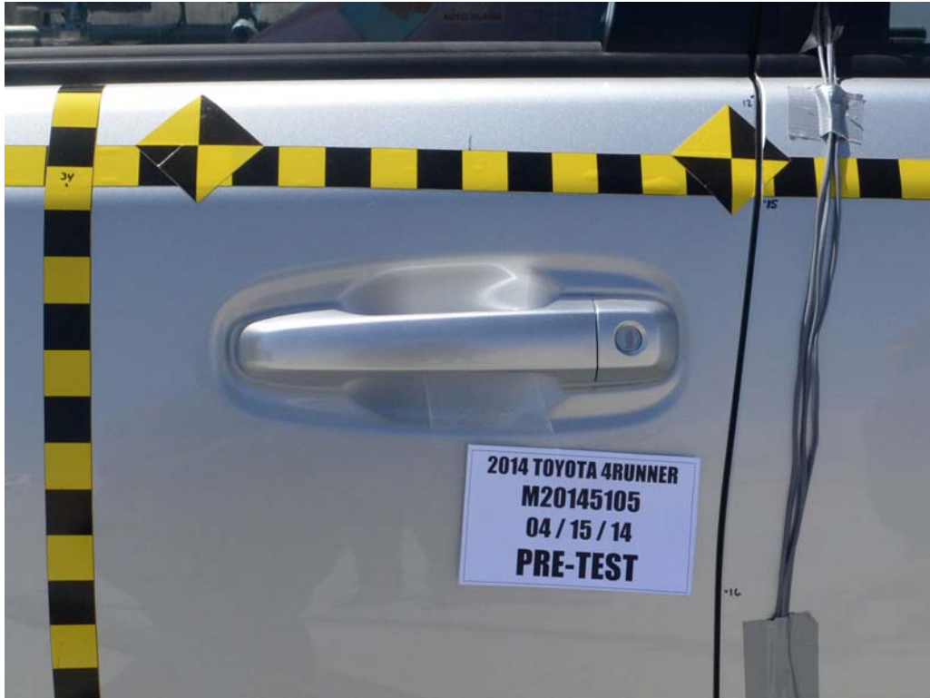
FIGURE 21. Pre-Test Left Front Door Latch Close-Up
