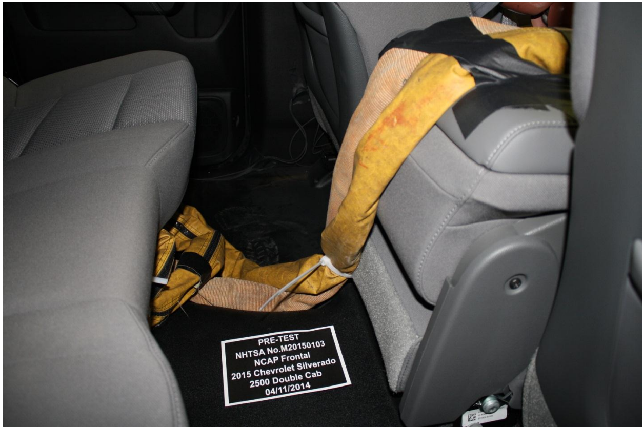
Figure A-27: Pre-Test Dummy Cable Routing
