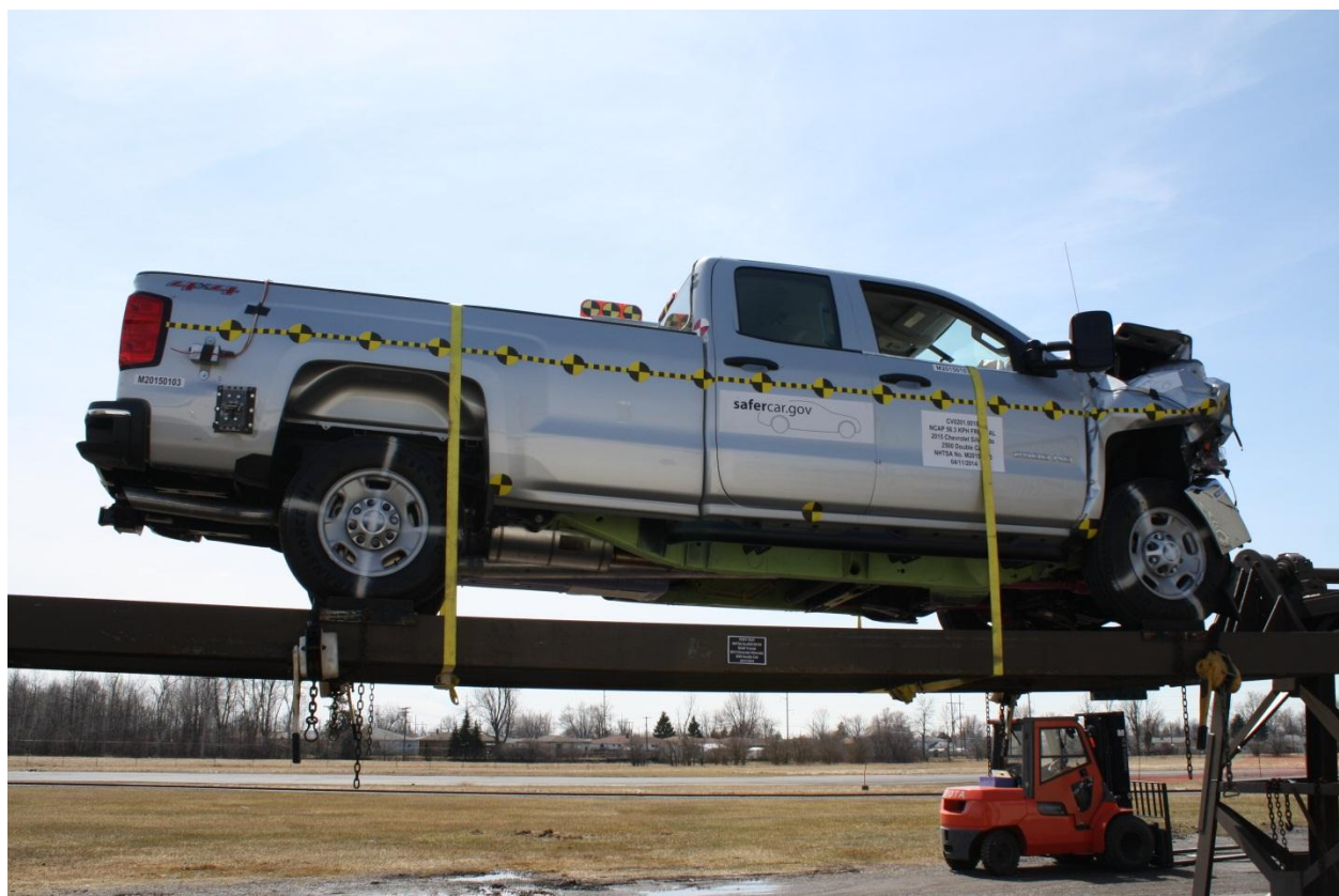
Figure A-72: Vehicle at 0° on Static Rollover Device
