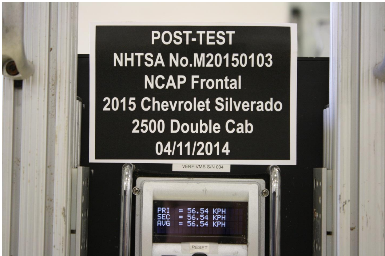
Figure A-71: Post-Test Speed Trap Read-Out
