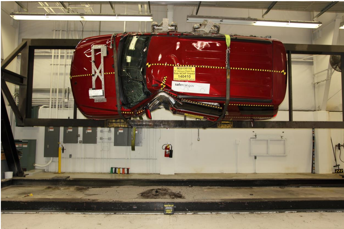
064 FMVSS No. 301 Static Rollover 90 Degrees
