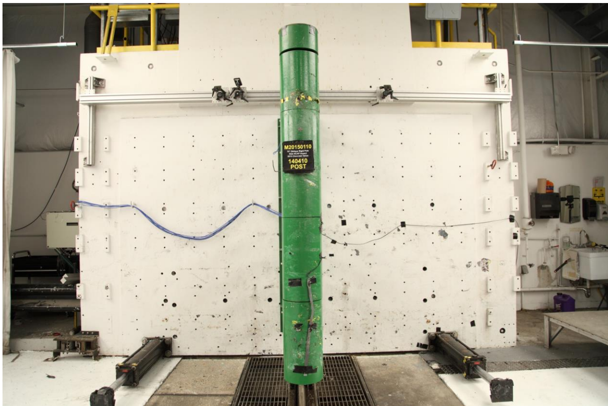
058 Post-Test Pole Barrier Front View
