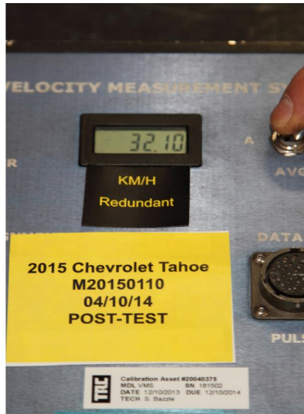
062 Post-Test Primary and Redundant Speed Trap Read-Out
