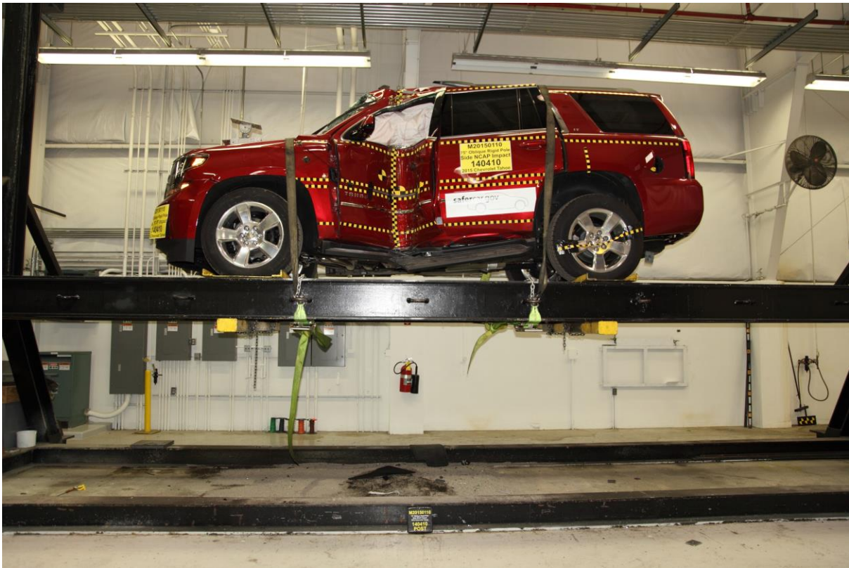
067 FMVSS No. 301 Static Rollover 360 Degrees
