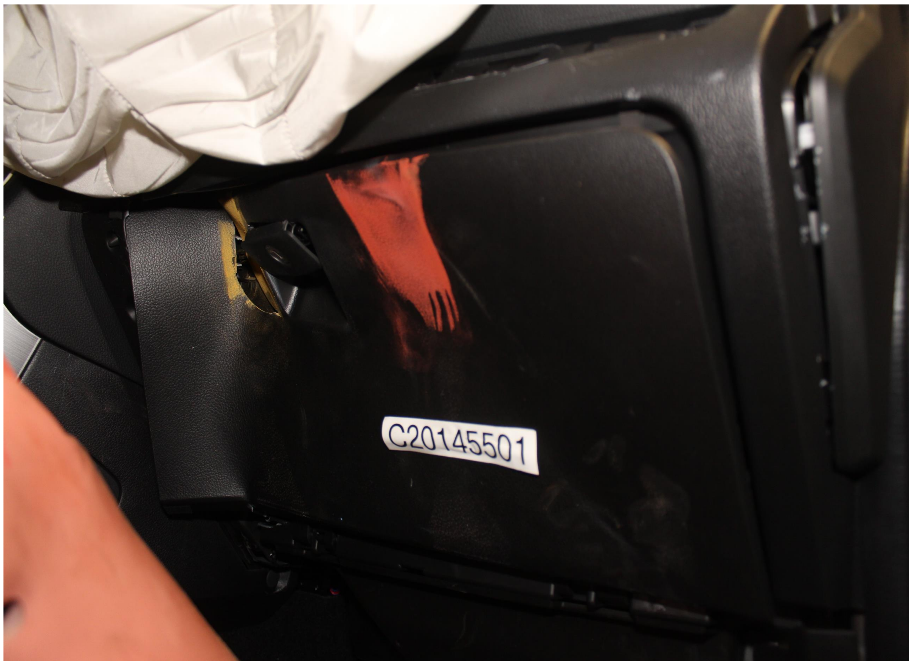
Post-Test Passenger Dummy Knee Contact
