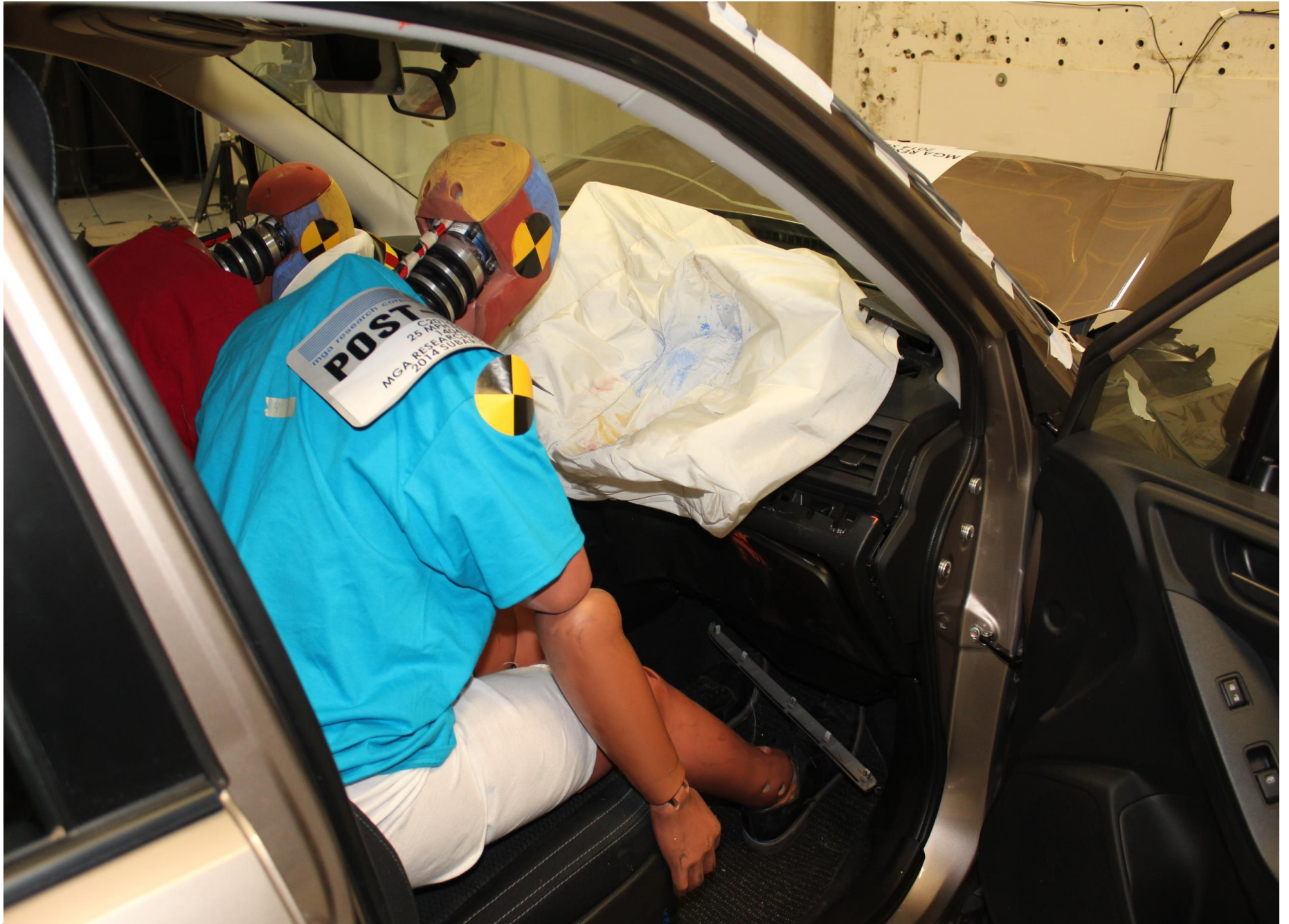
Post-Test Passenger Dummy Airbag Contact
