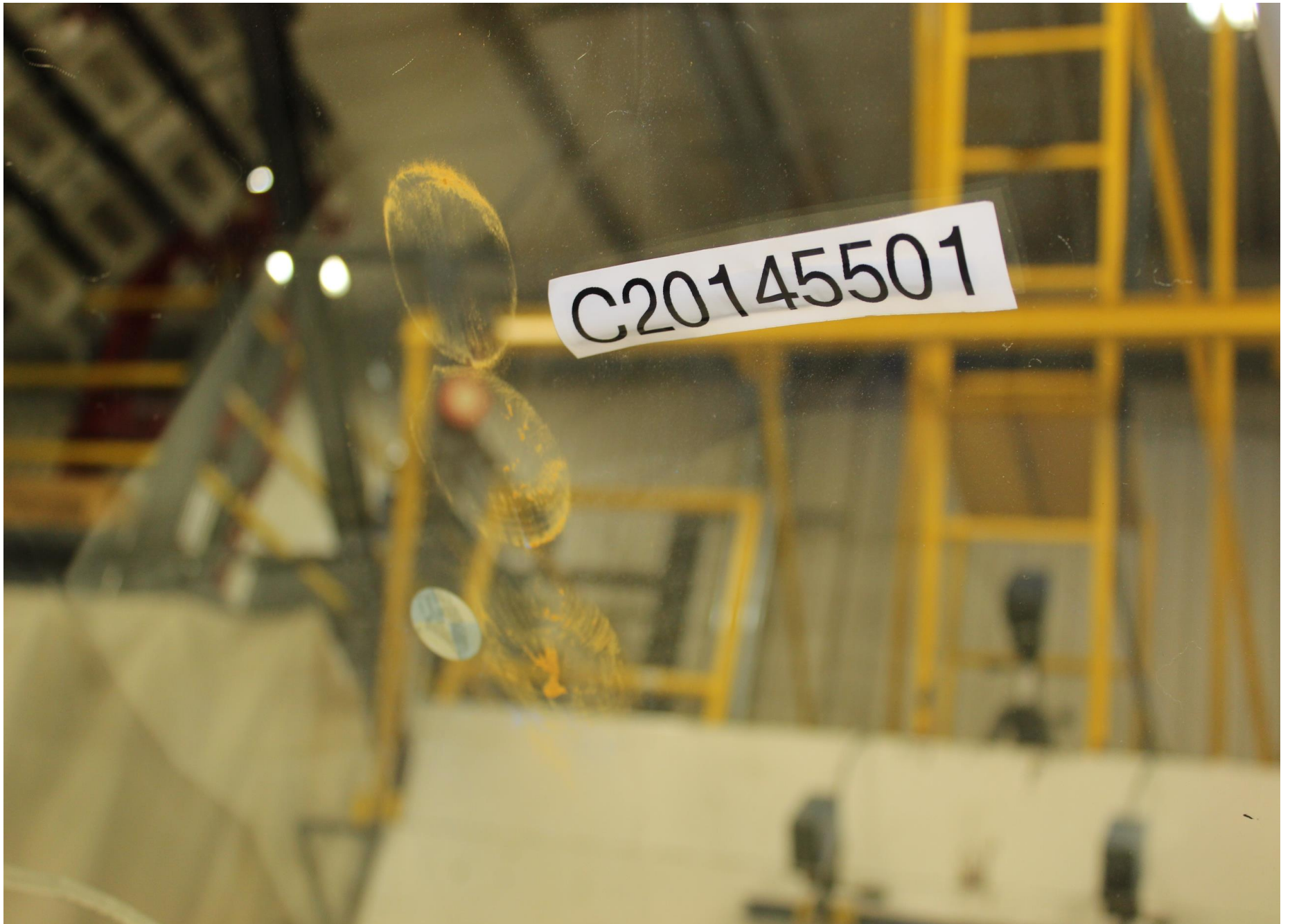
Post-Test Passenger Dummy Head Contact (windshield)
