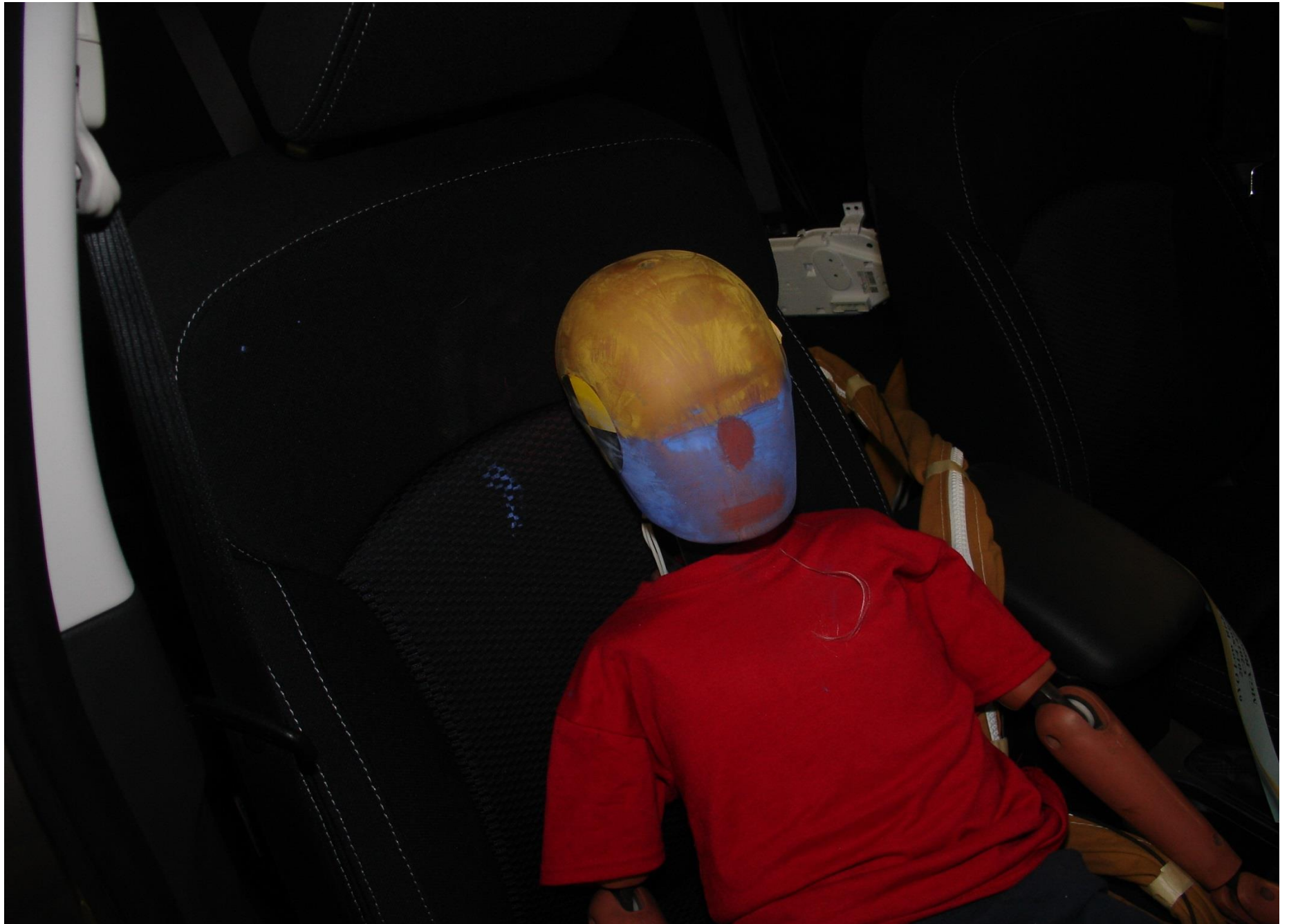
Post-Test 6YO P1 Passenger Dummy Head Contact (seat back)
