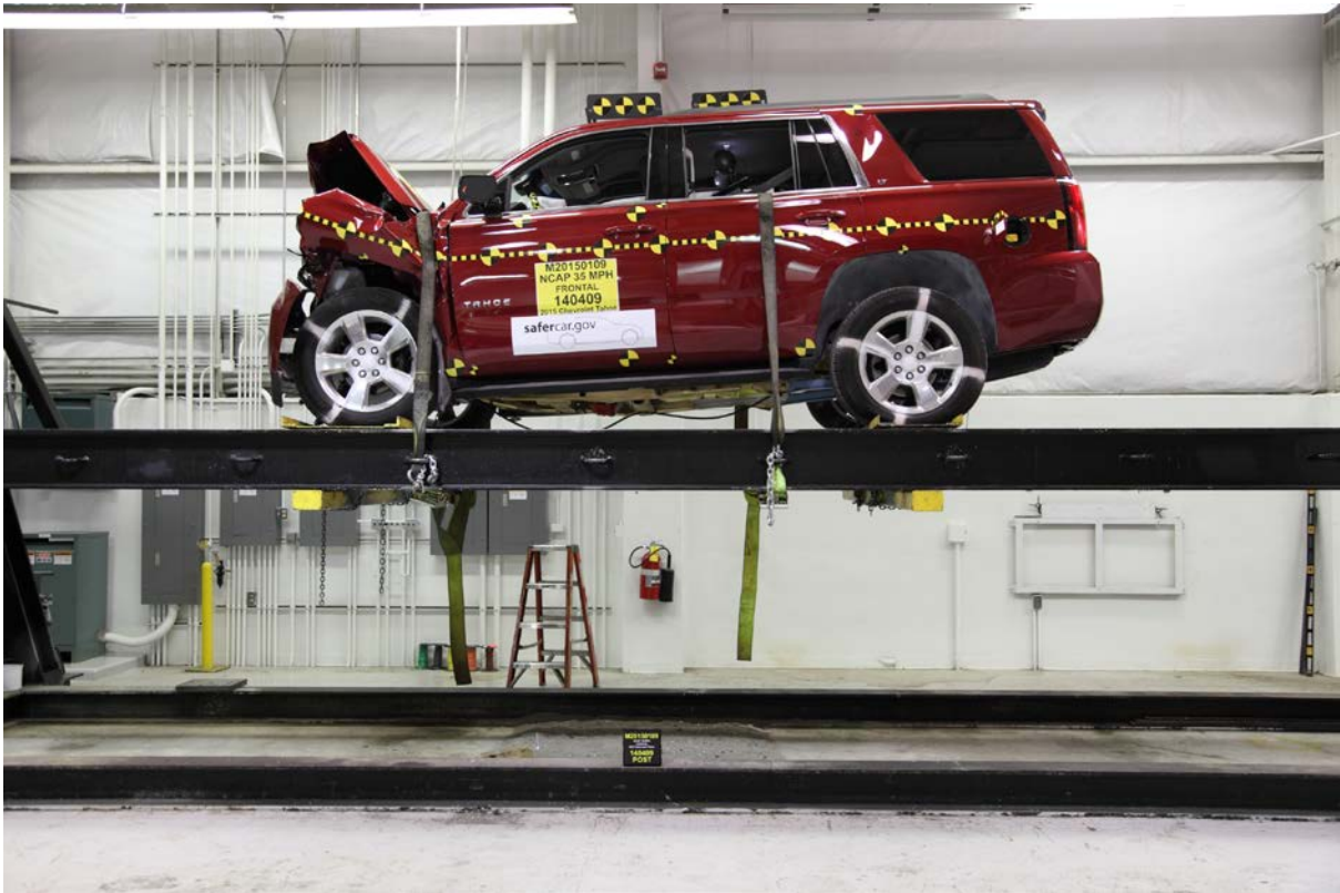
070 Vehicle at 0° on Static Rollover Device
