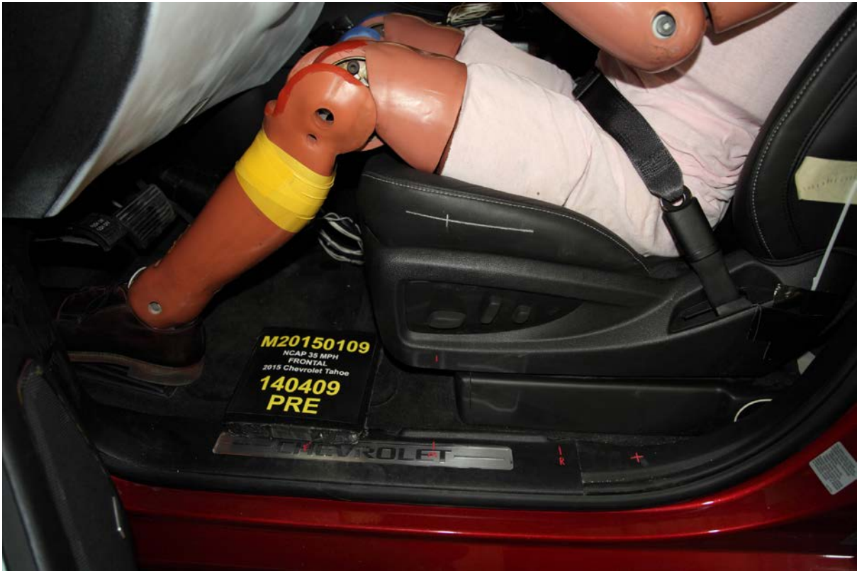
035 Pre-Test Driver's Seat Fore-Aft Markings
