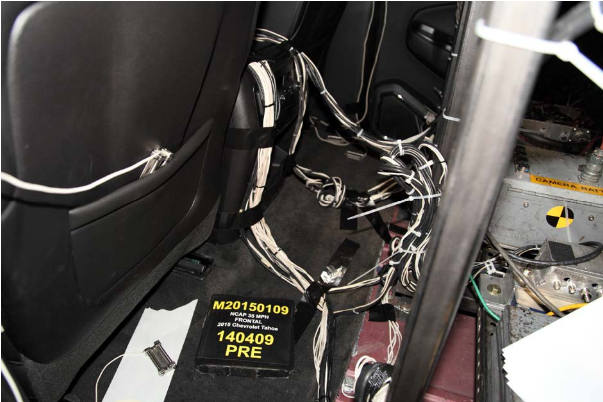
027 Pre-Test Dummy Cable Routing
