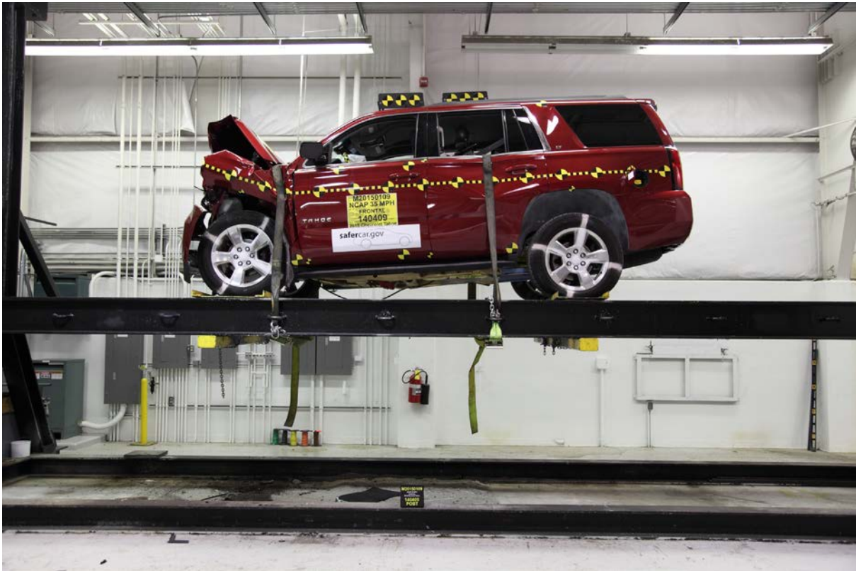
074 Vehicle at 360° on Static Rollover Device
