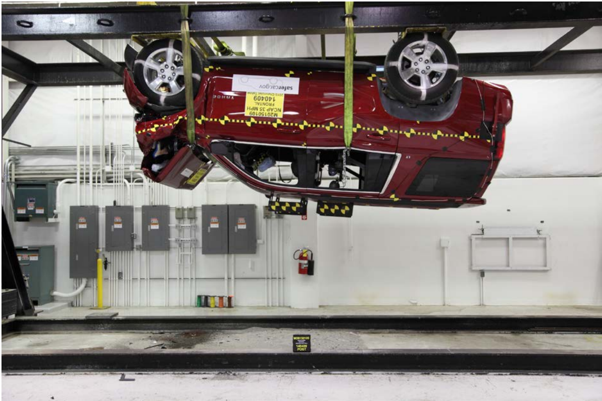
072 Vehicle at 180° on Static Rollover Device
