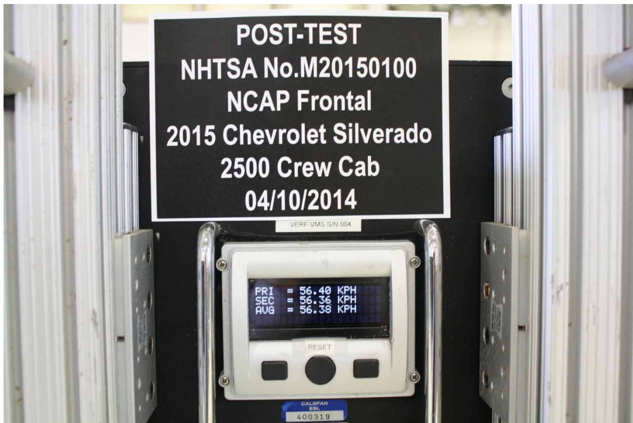
Figure A-71: Post-Test Speed Trap Read-Out
