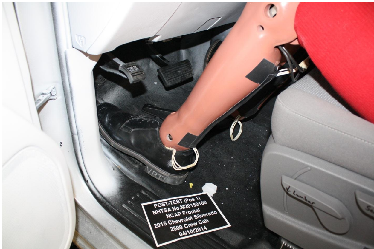
Figure A-40: Post-Test Driver Dummy Feet
