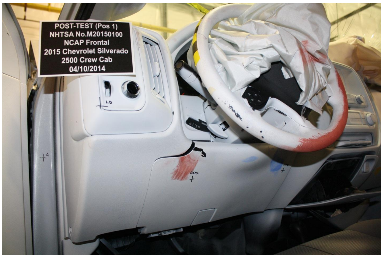
Figure A-42: Post-Test Driver's Side Knee Bolster
