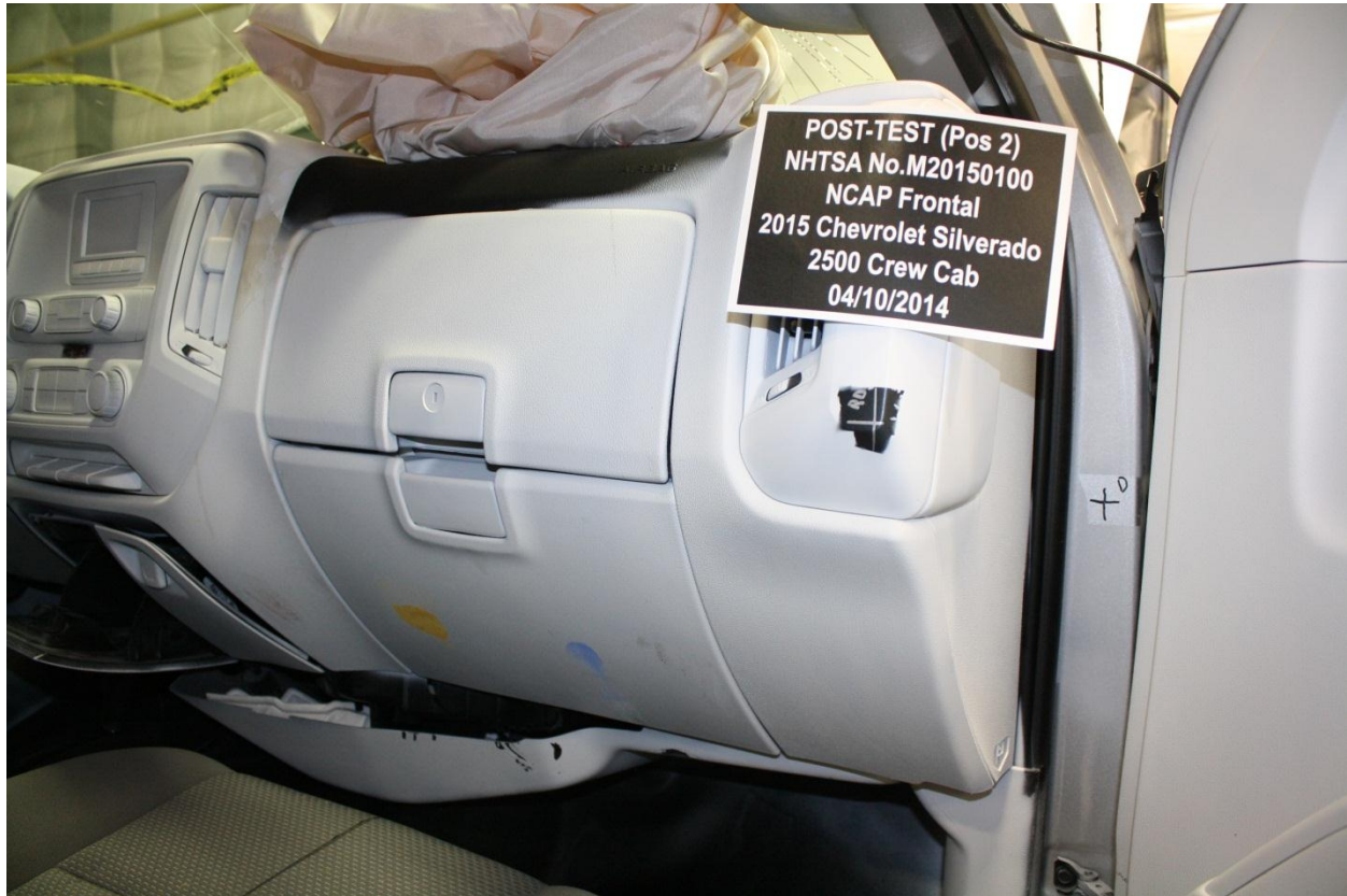
Figure A-63: Post-Test Passenger's Side Knee Bolster
