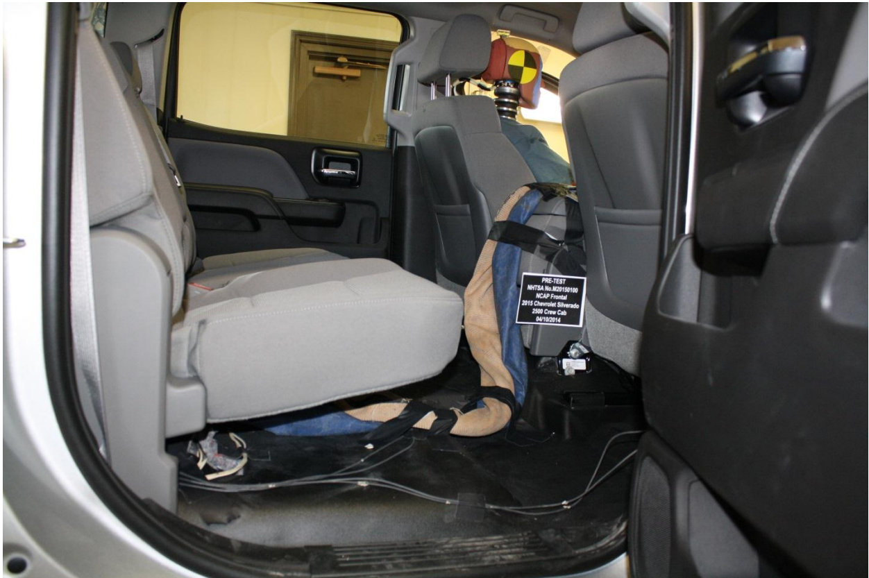
Figure A-27: Pre-Test Dummy Cable Routing
