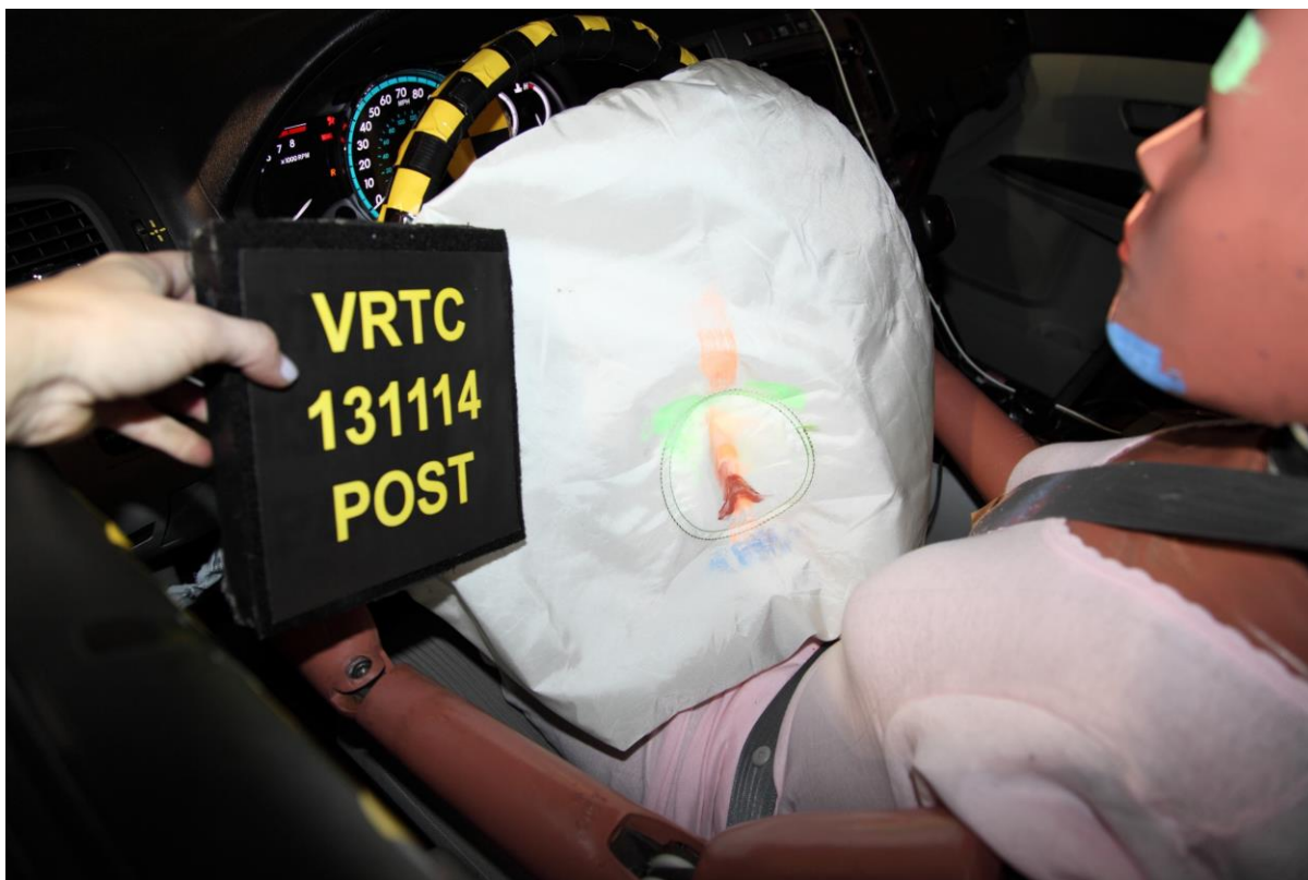
Figure A-33 Post-Test Driver Dummy Contact – View 1
