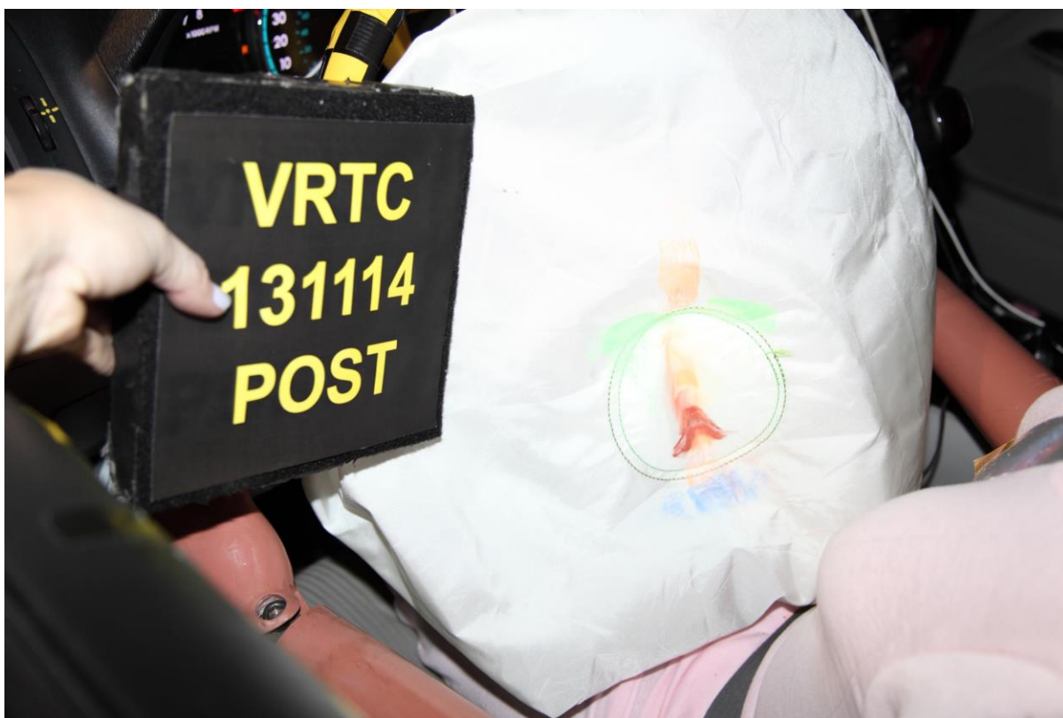
Figure A-34 Post -Test Driver Dummy Contact – View 2
