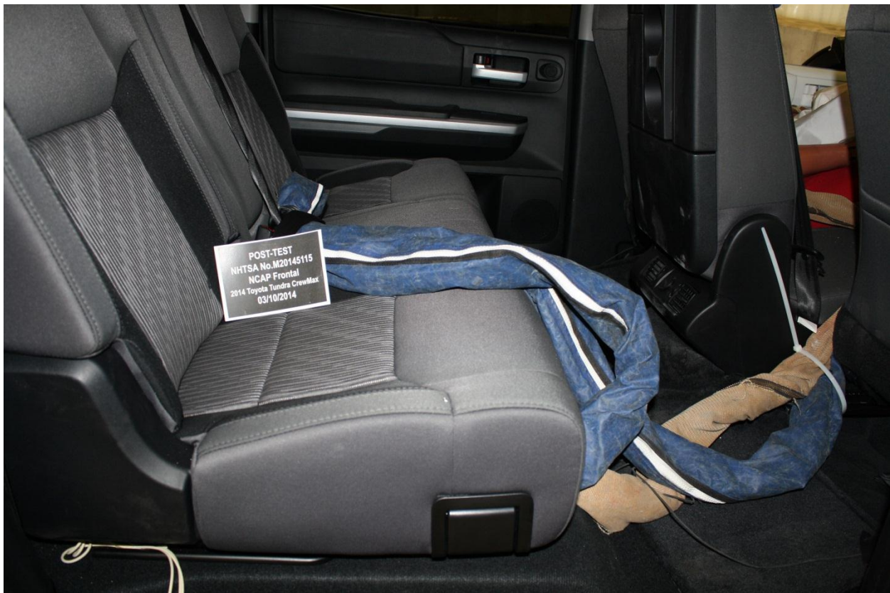
Figure A-28: Post-Test Dummy Cable Routing
