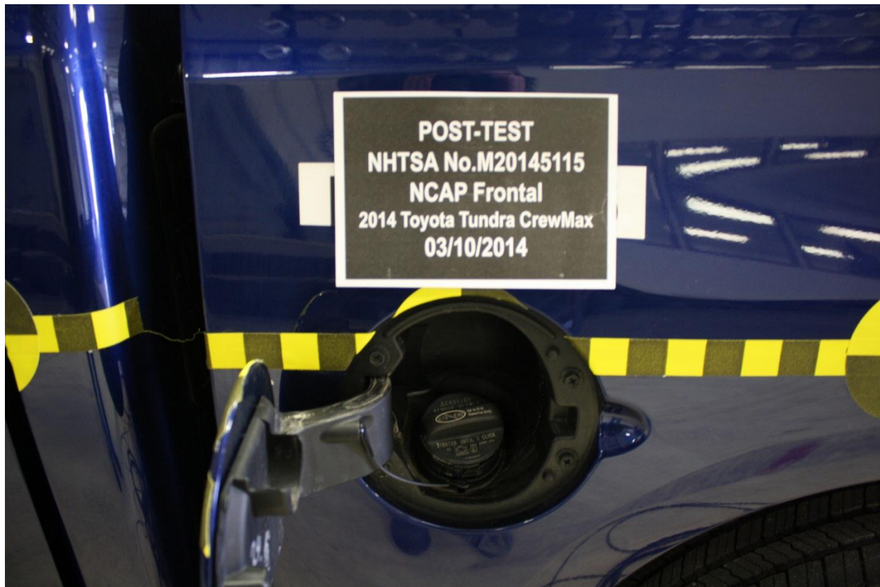
Figure A-22: Post-Test Fuel Filler Cap View
