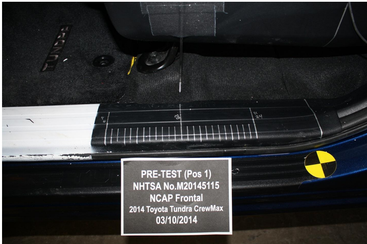
Figure A-35: Pre-Test Driver's Seat Fore-Aft Markings
