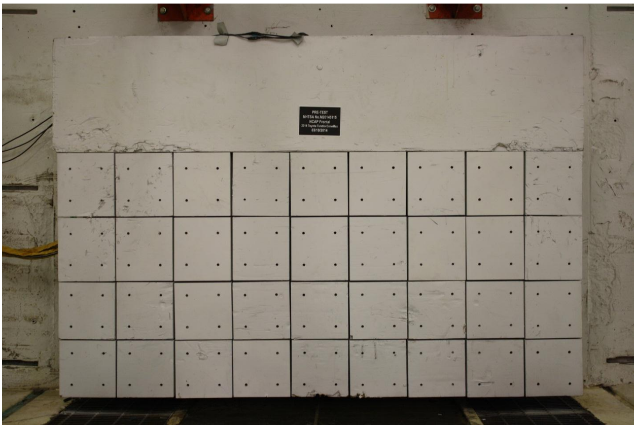
Figure A-2: Load Cell Wall
