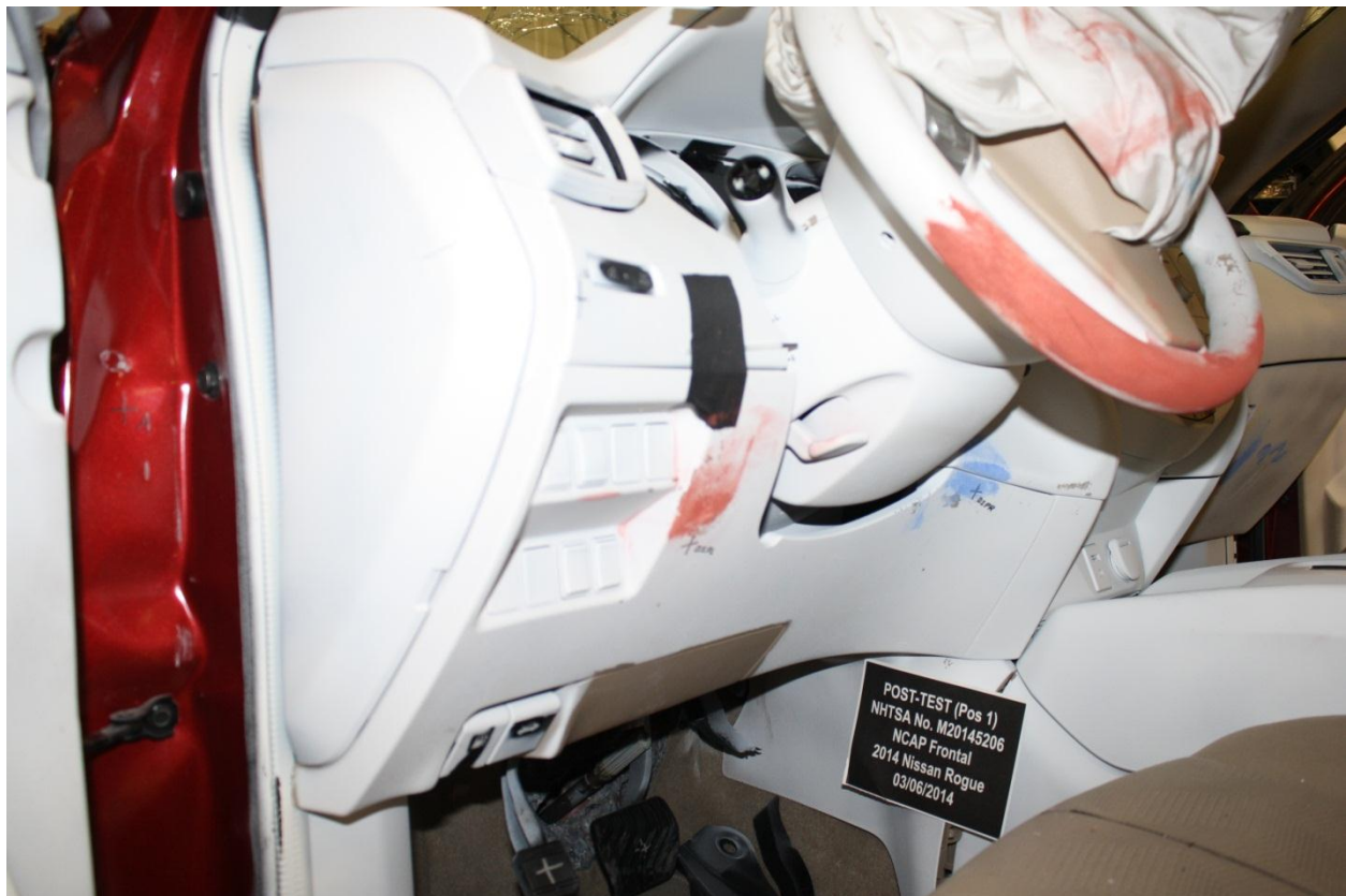
Figure A-42: Post-Test Driver's Side Knee Bolster
