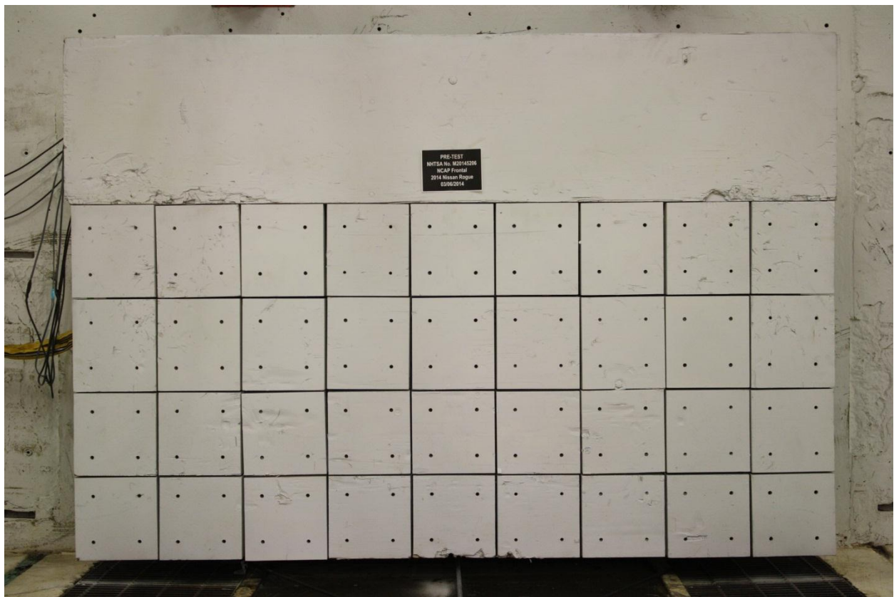
Figure A-2: Load Cell Wall
