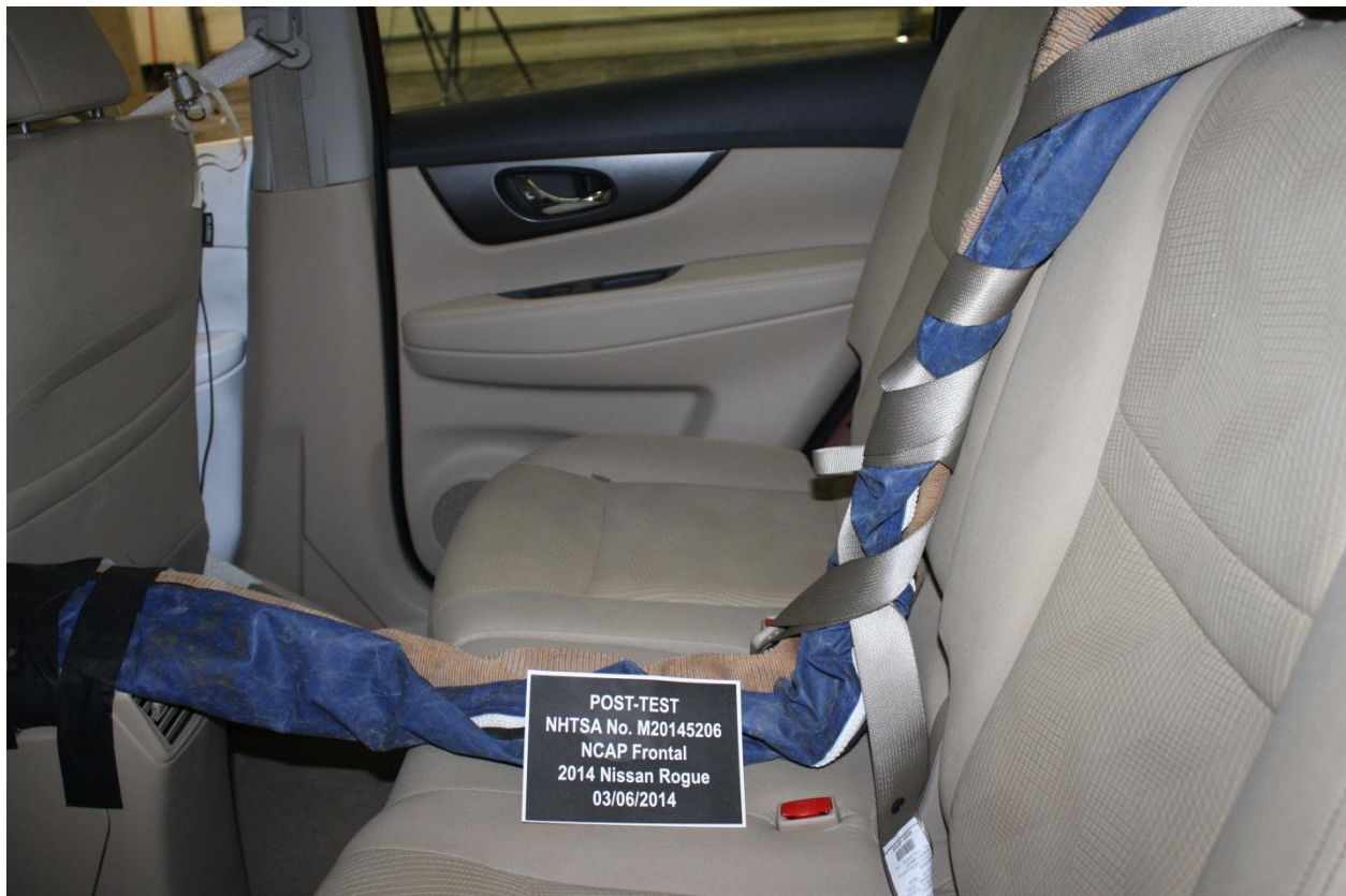
Figure A-28: Post-Test Dummy Cable Routing
