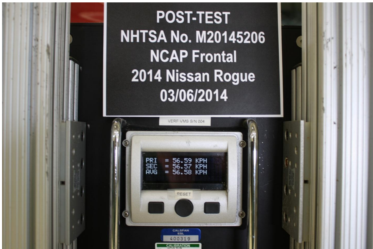
Figure A-71: Post-Test Speed Trap Read-Out
