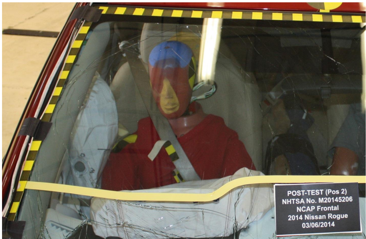
Figure A-51: Post-Test Passenger Dummy Front View
