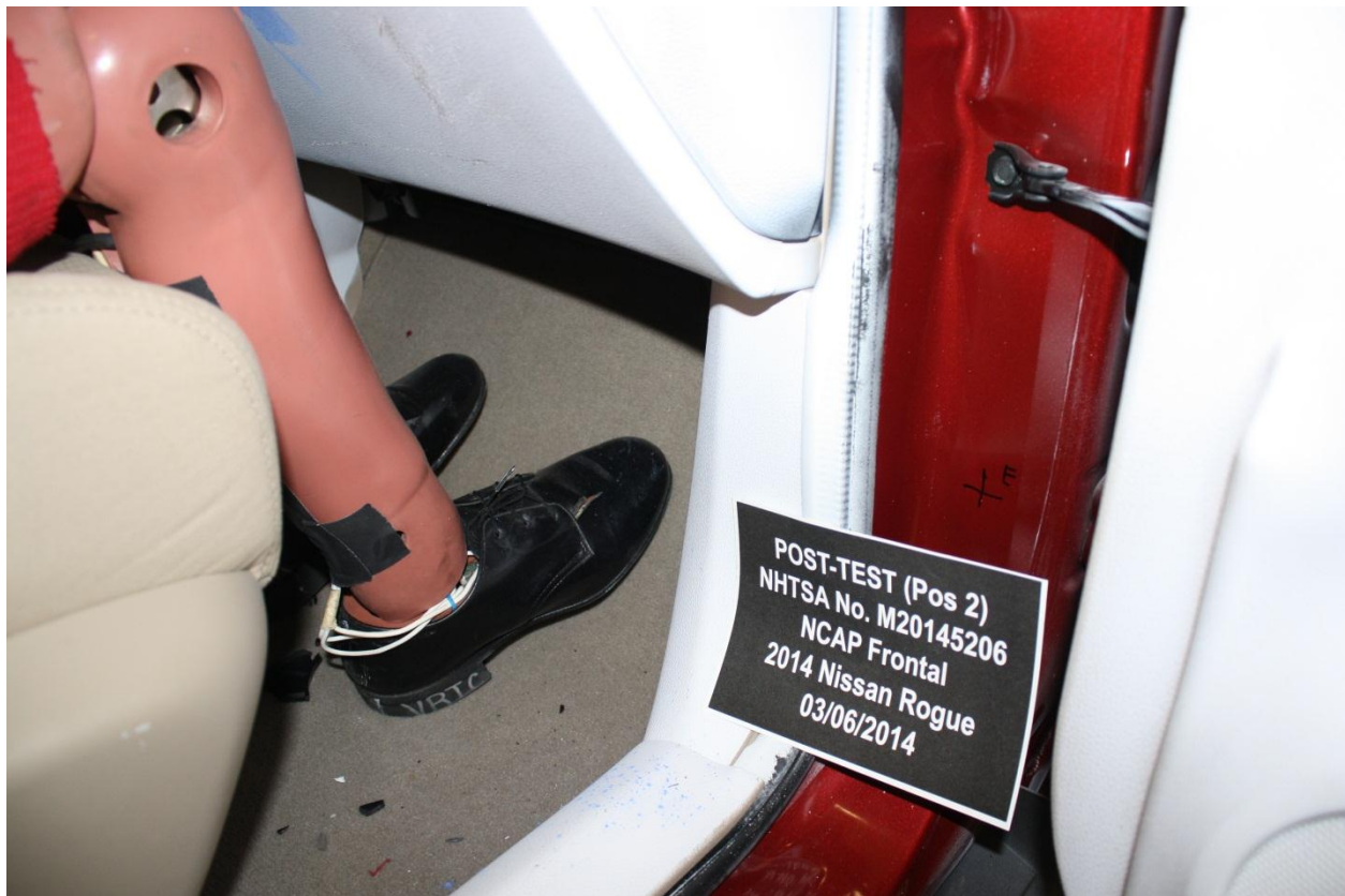
Figure A-61: Post-Test Passenger Dummy Feet
