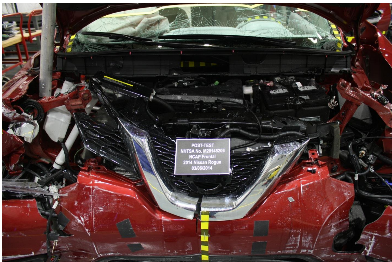
Figure A-20: Post-Test Engine Compartment View
