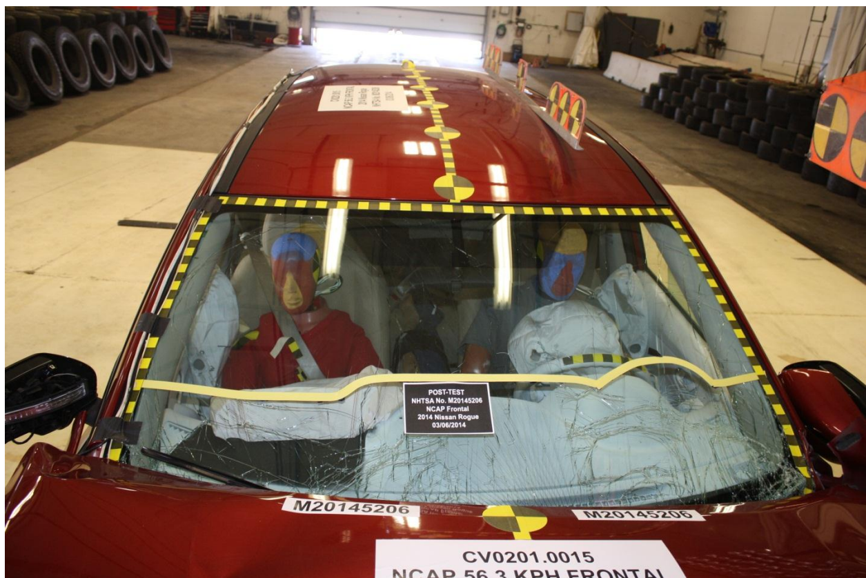
Figure A-18: Post-Test Windshield View
