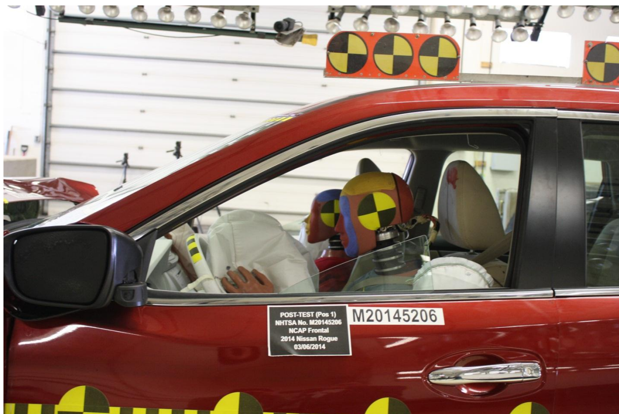
Figure A-32: Post-Test Driver Dummy Window View
