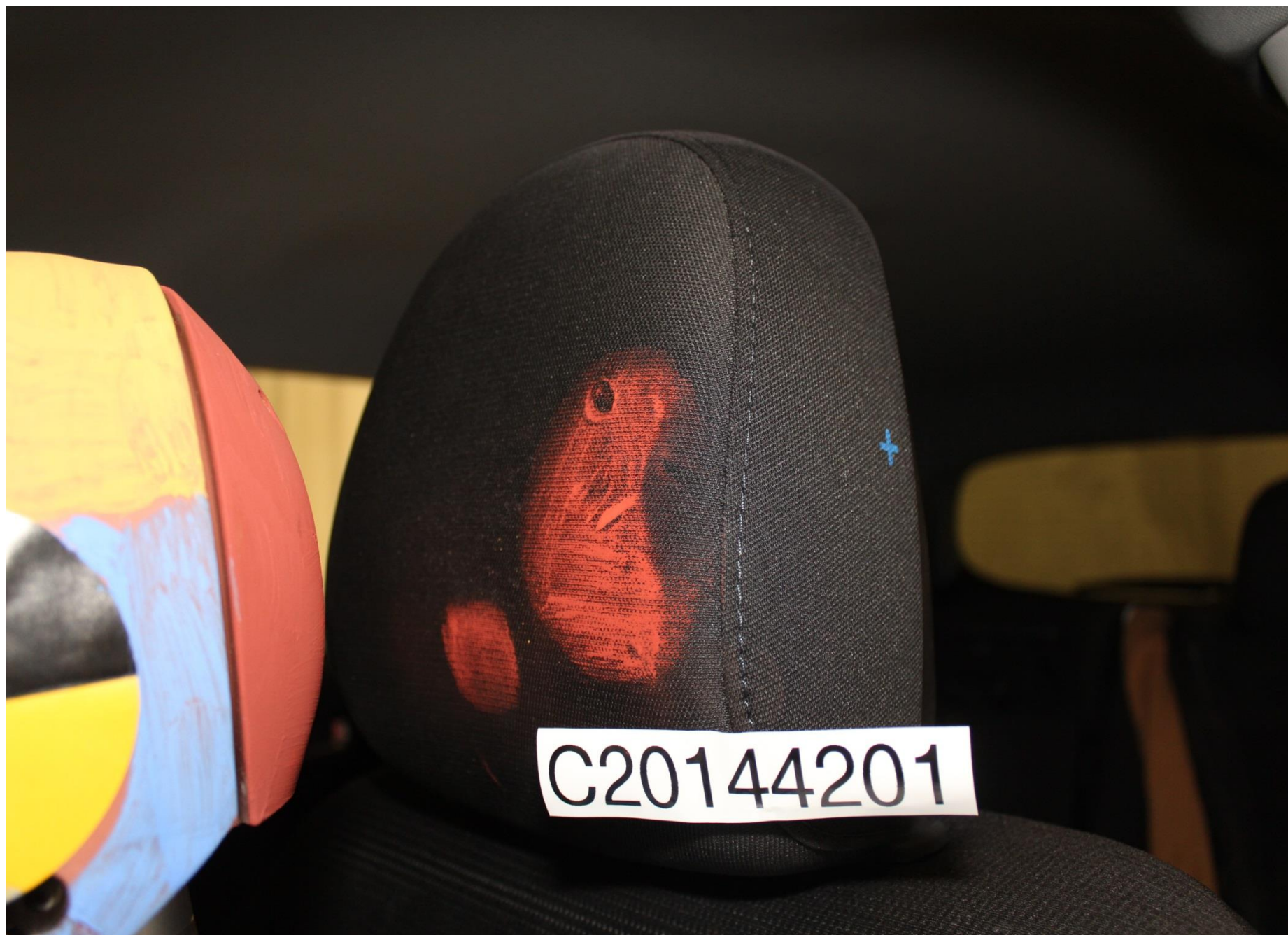
Post-Test Driver Dummy Head Contact (head rest)
