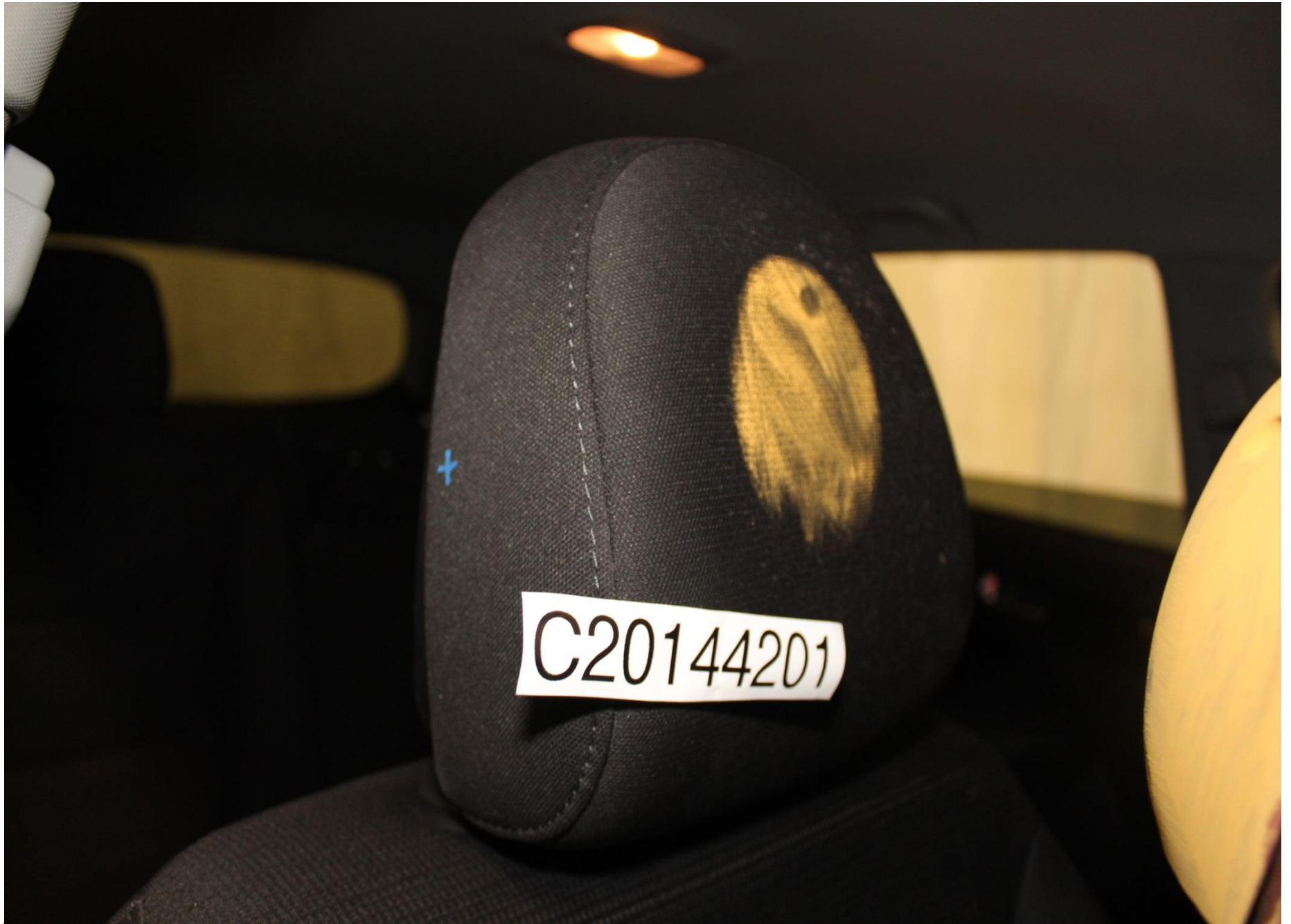
Post-Test Passenger Dummy Head Contact (headrest)
