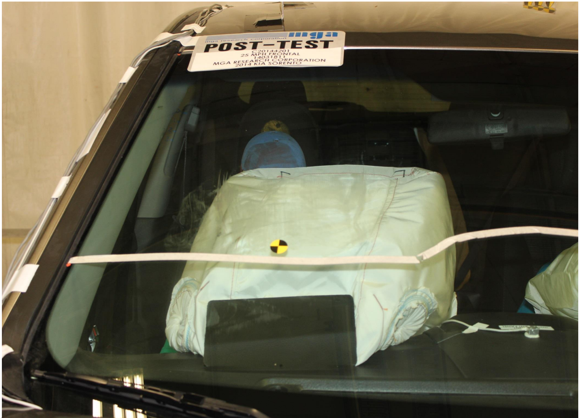
Post-Test Passenger Dummy Front View (head position)
