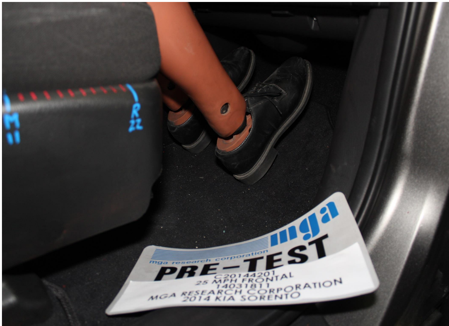
Pre-Test Passenger Dummy Feet Position
