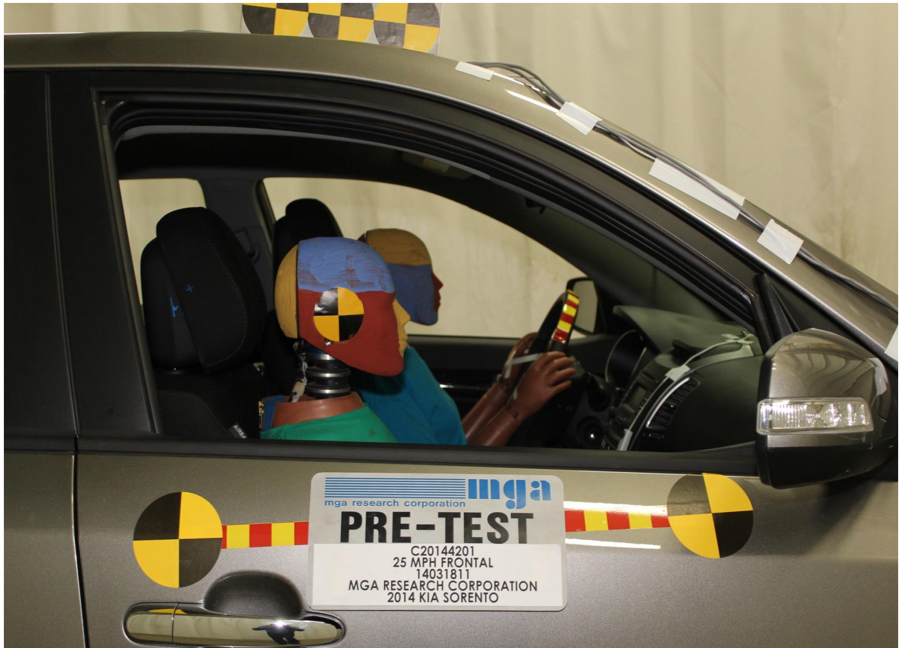
Pre-Test Passenger Dummy Position Right Side View
