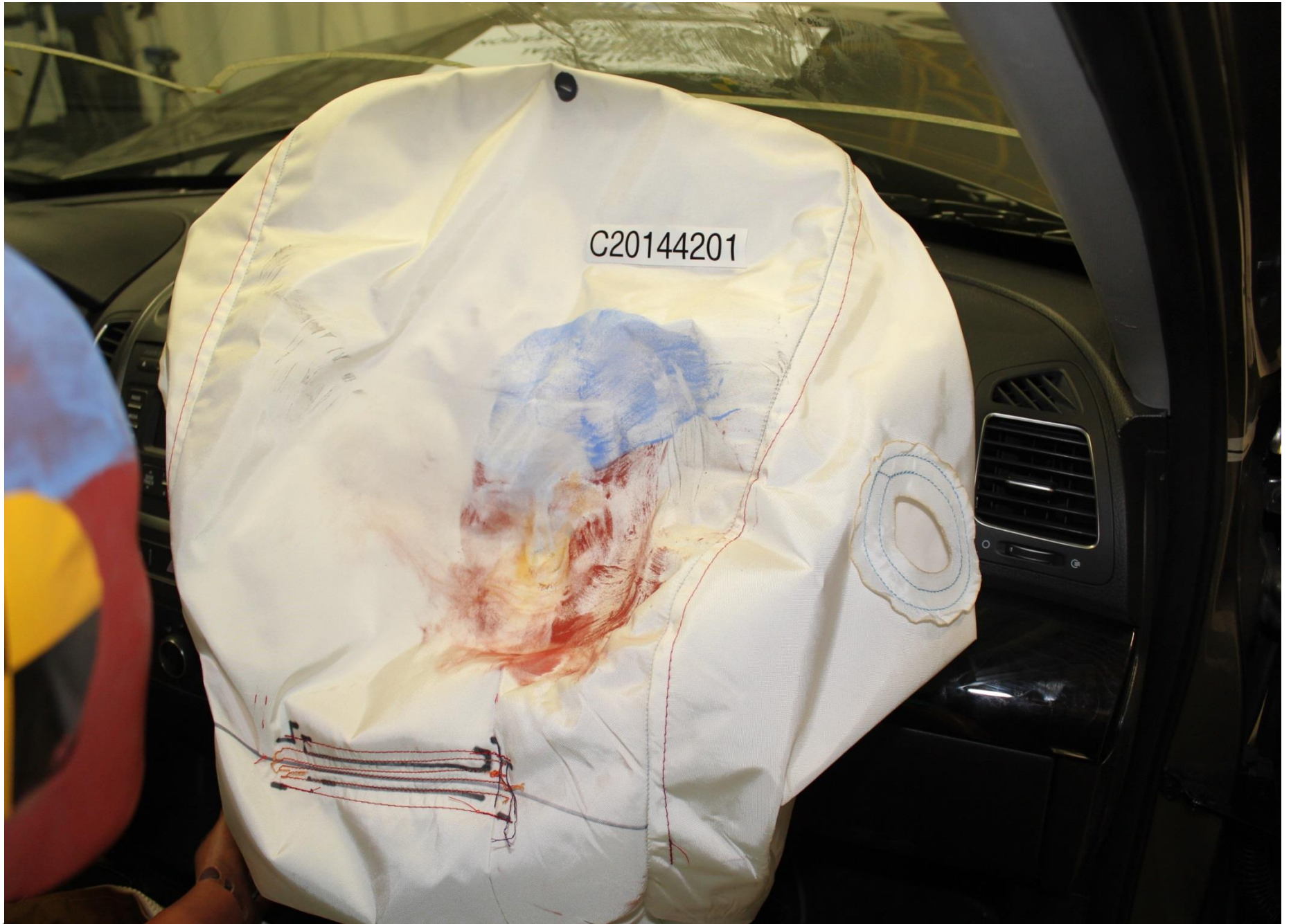
Post-Test Passenger Dummy Airbag Contact
