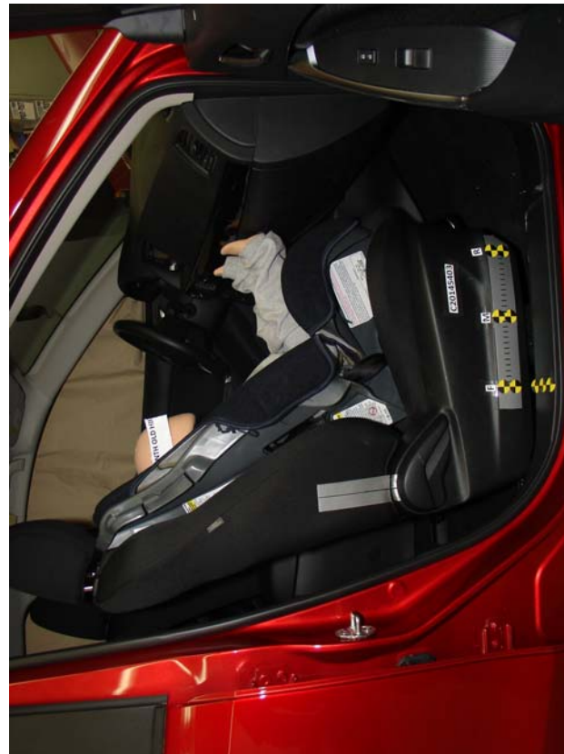
Cosco High Back Booster Forward Facing Unbelted, Forward Seat Track
