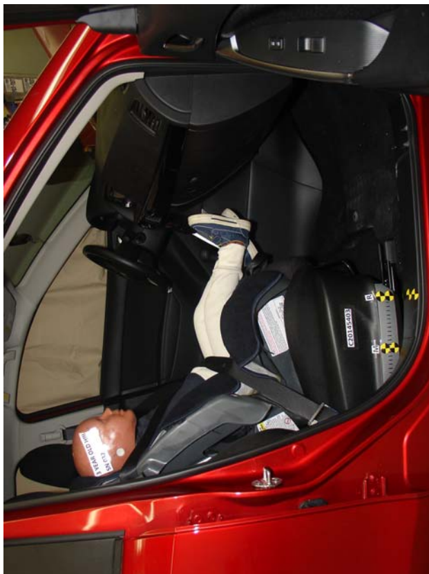
3-Year-Old Forward Facing Cosco High Back Booster Belted, Rearward Seat Track
