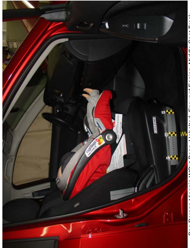
Peg Perego Viaggio WOut Base, Unbelted, Forward Facing, Middle Seat Track
