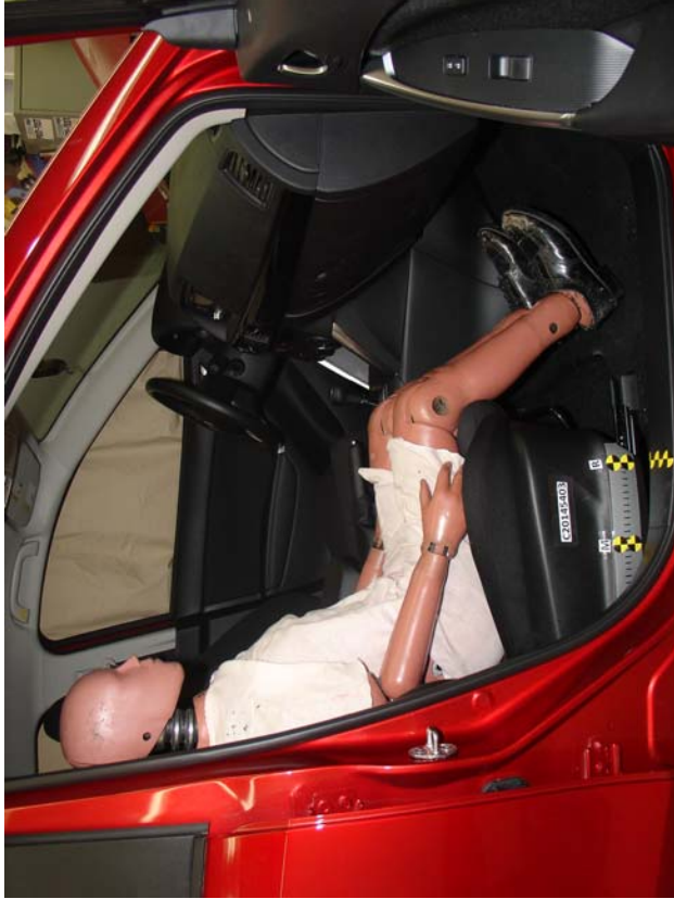
Unbelted 5th Percentile Female Dummy Reaction, Rearward Seat Track
