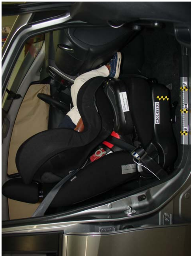
3-Year-Old Forward Facing Graco Toddler SafeSeat Step 2 Belted, Forward Seat Track
