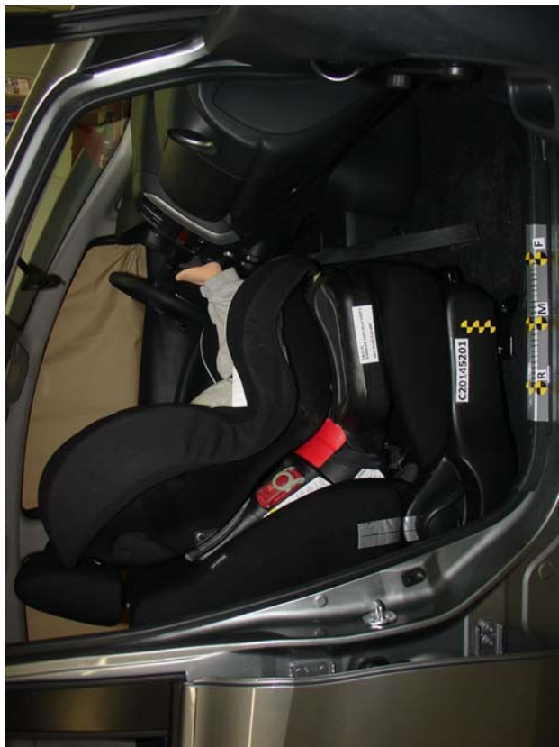
Graco Toddler SafeSeat Step 2 Forward Facing Unbelted, Middle Seat Track
