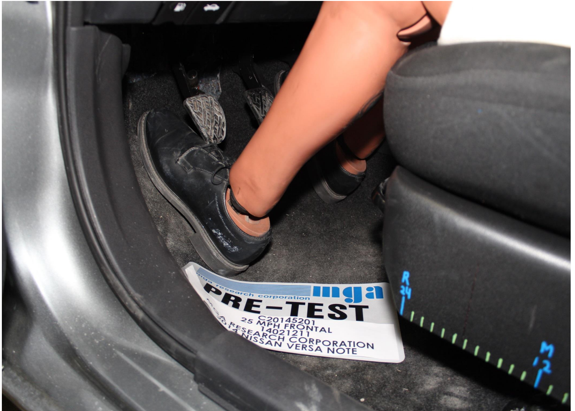
Pre-Test Driver Dummy Feet Position
