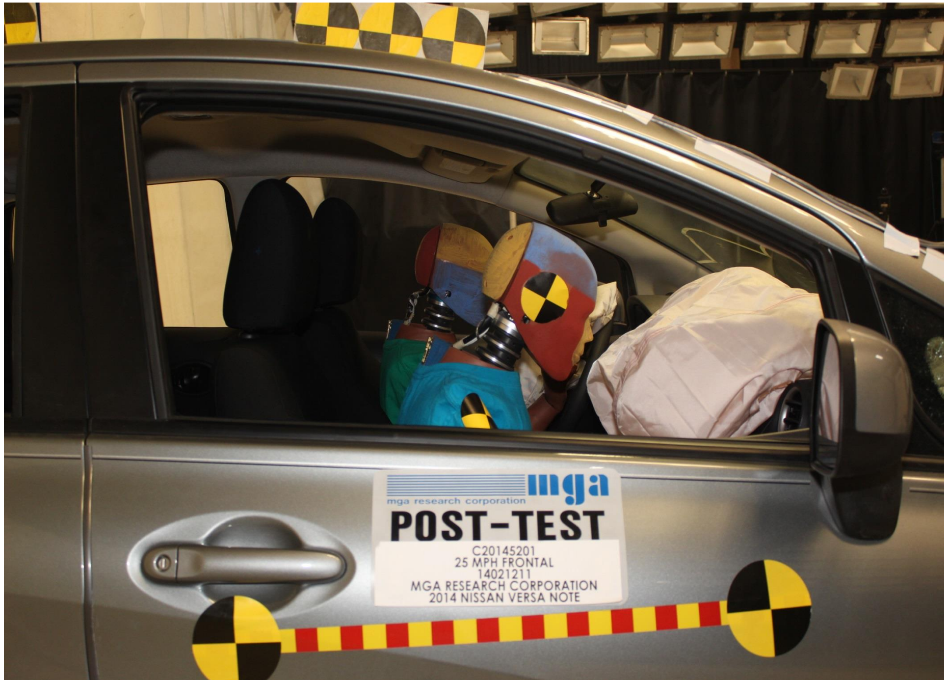
Post-Test Passenger Dummy Position Right Side View
