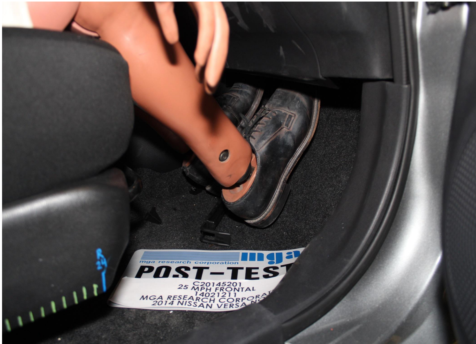
Post-Test Passenger Dummy Feet Position
