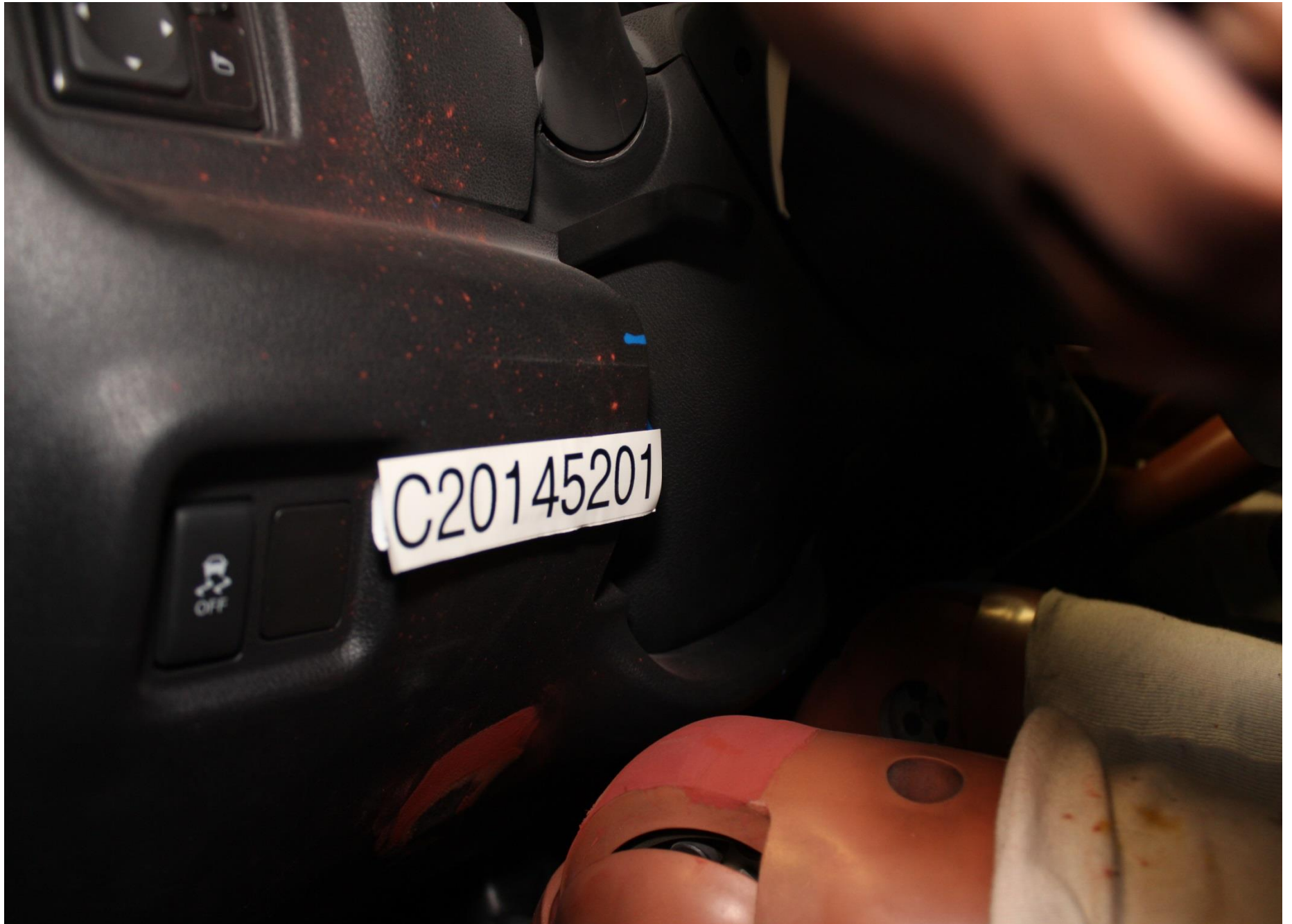
Post-Test Driver Dummy Knee Contact
