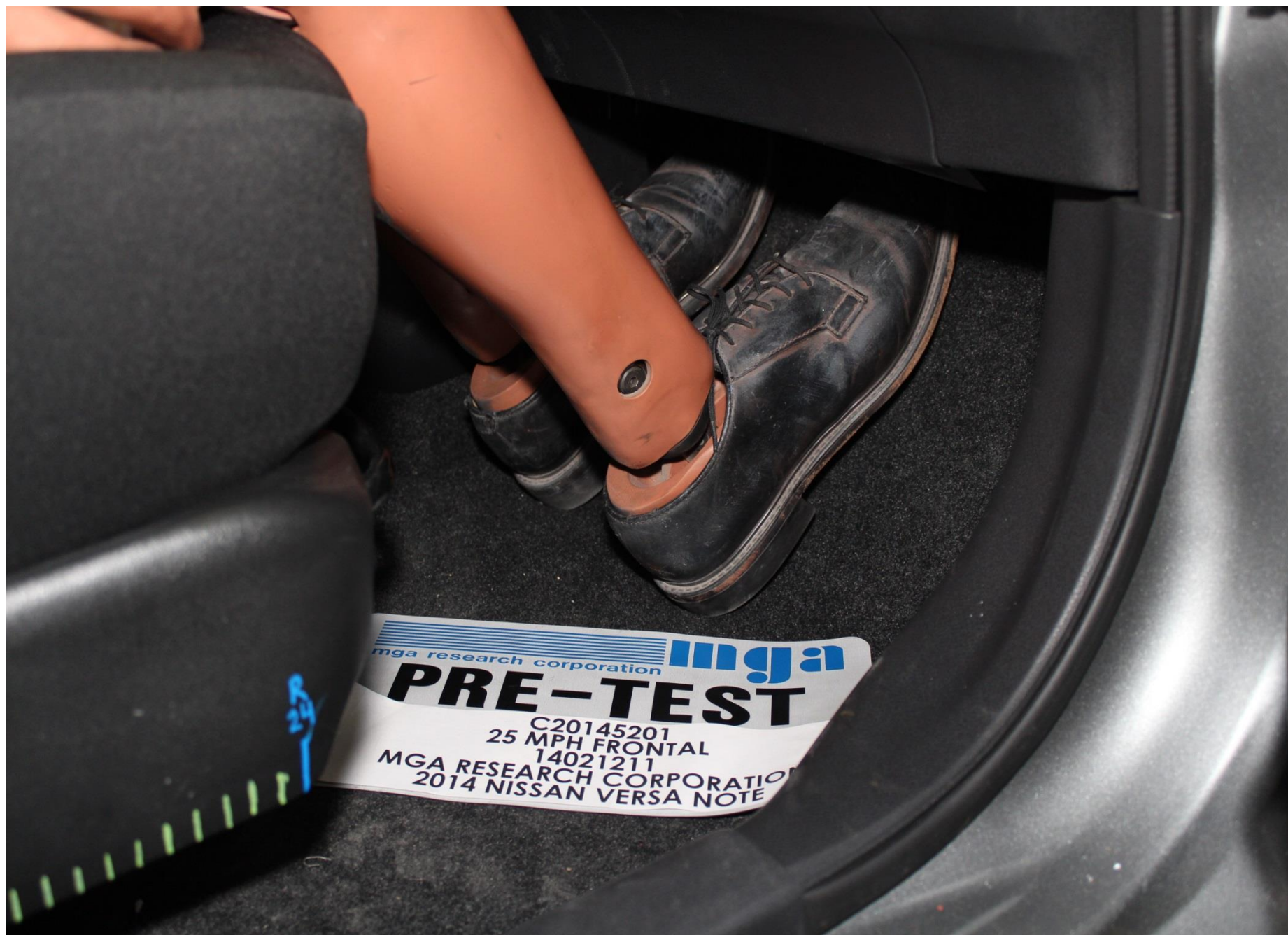
Pre-Test Passenger Dummy Feet Position
