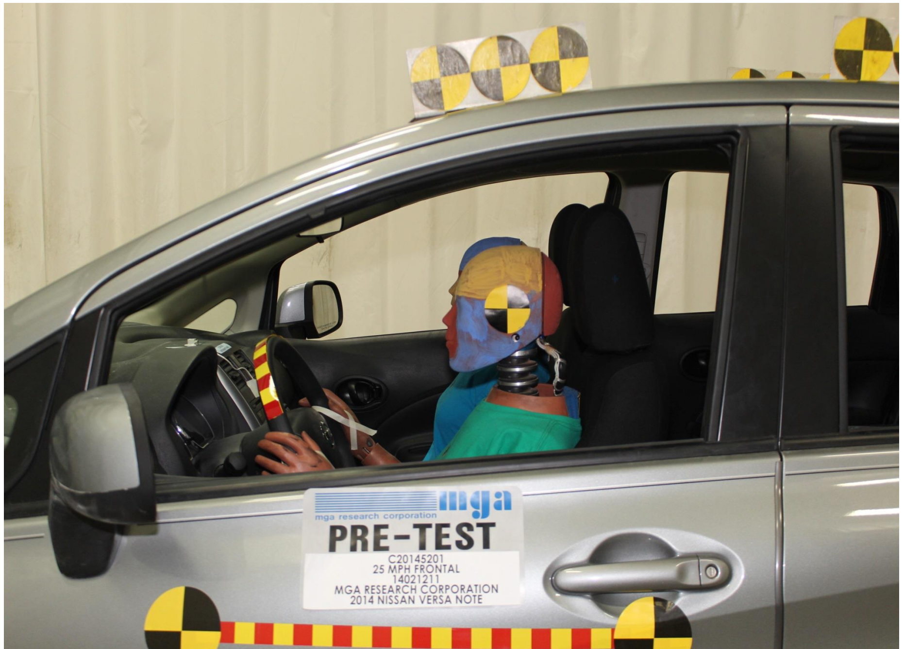
Pre-Test Driver Dummy Position Left Side View
