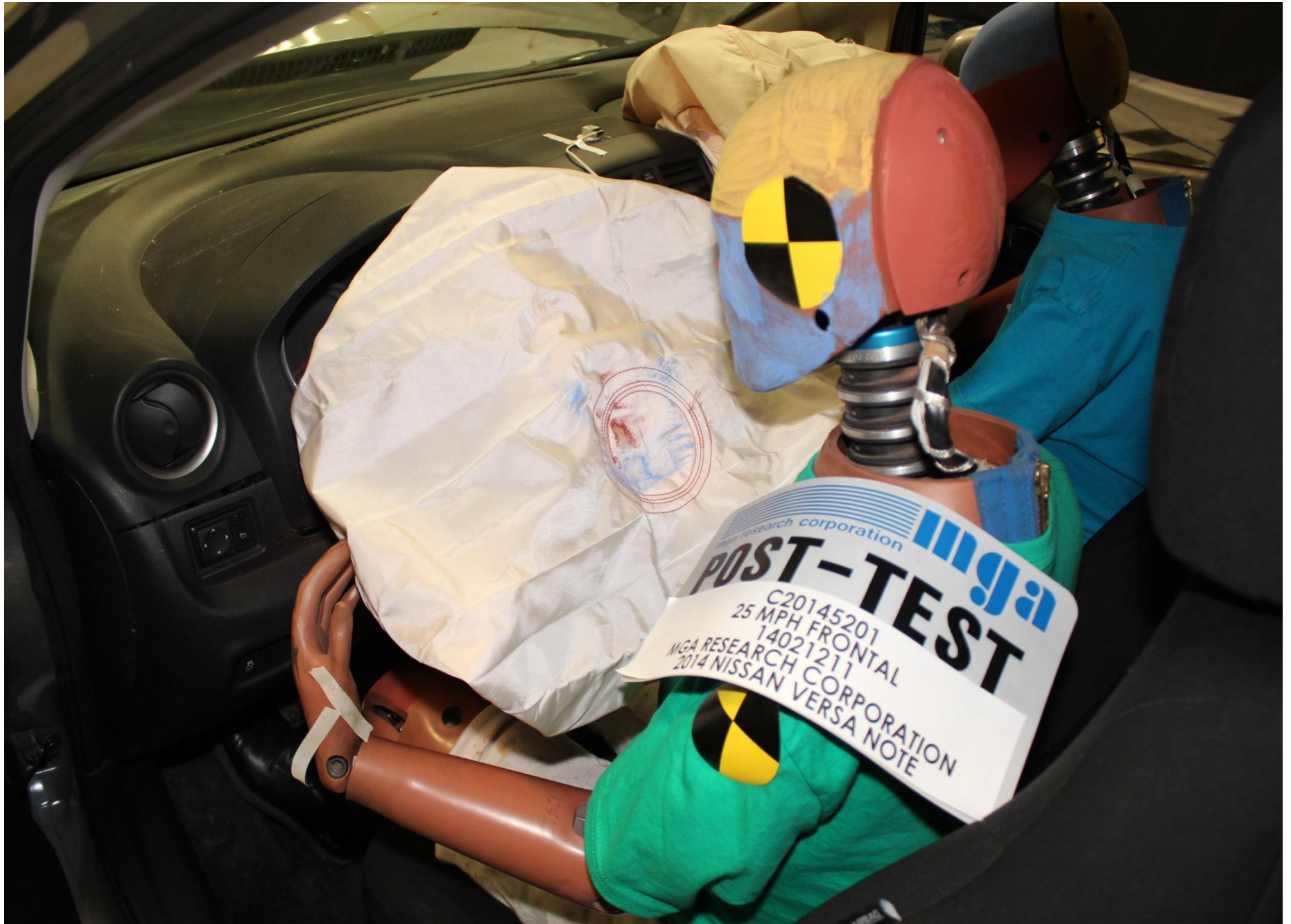
Post-Test Driver Dummy Airbag Contact
