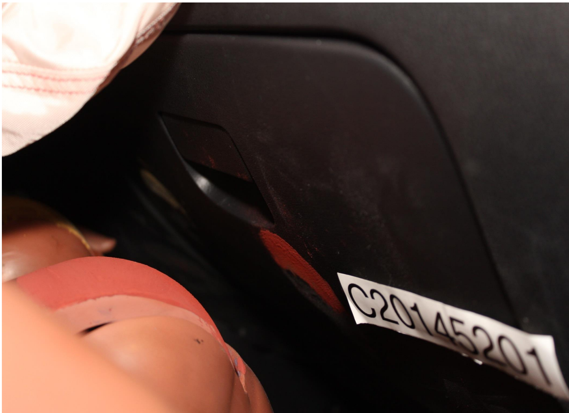
Post-Test Passenger Dummy Knee Contact
