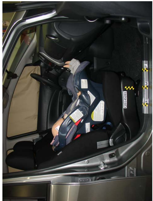
Graco Snuggly WOut Base, Unbelted, Forward Facing, Middle Seat Track
