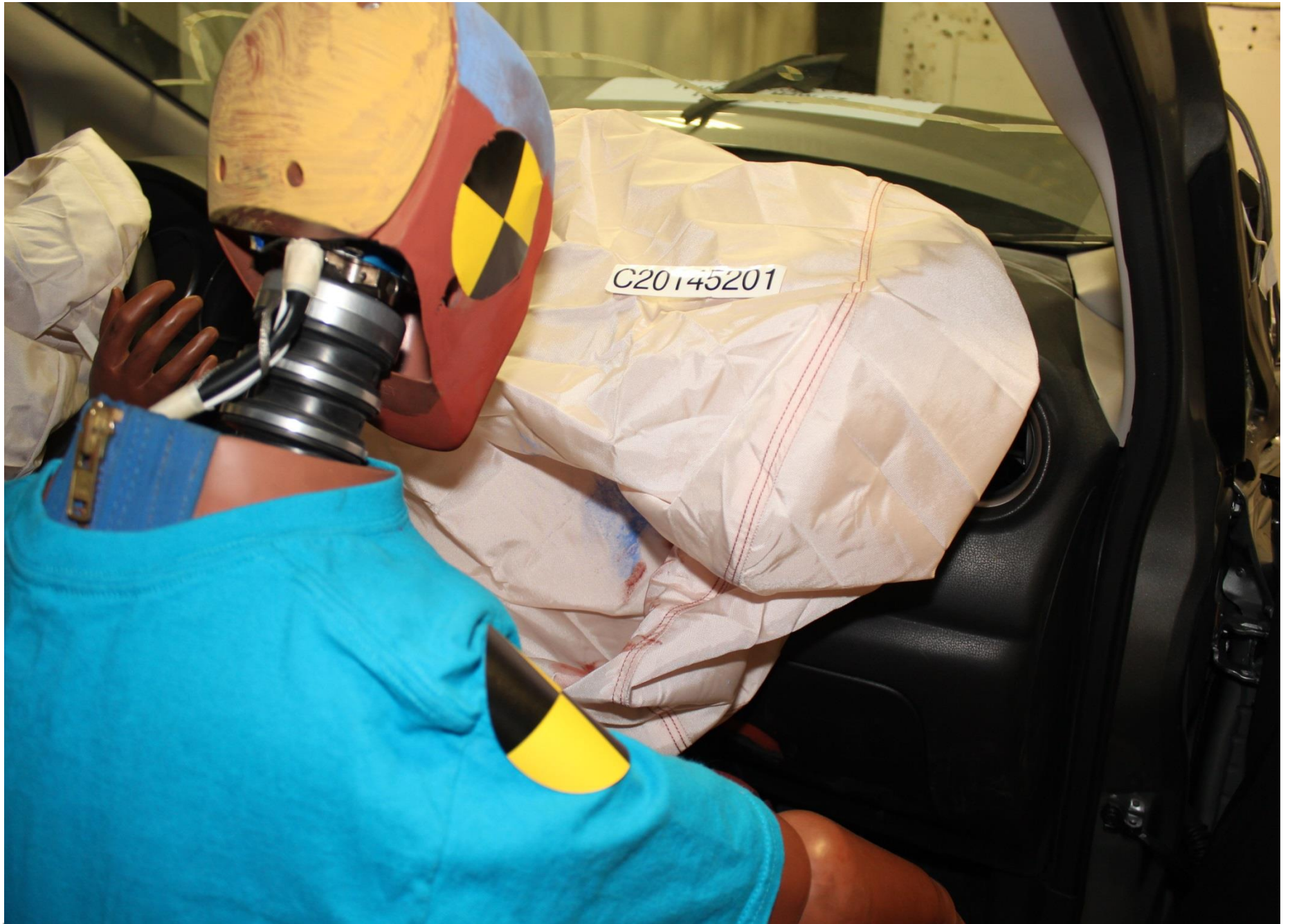
Post-Test Passenger Dummy Airbag Contact
