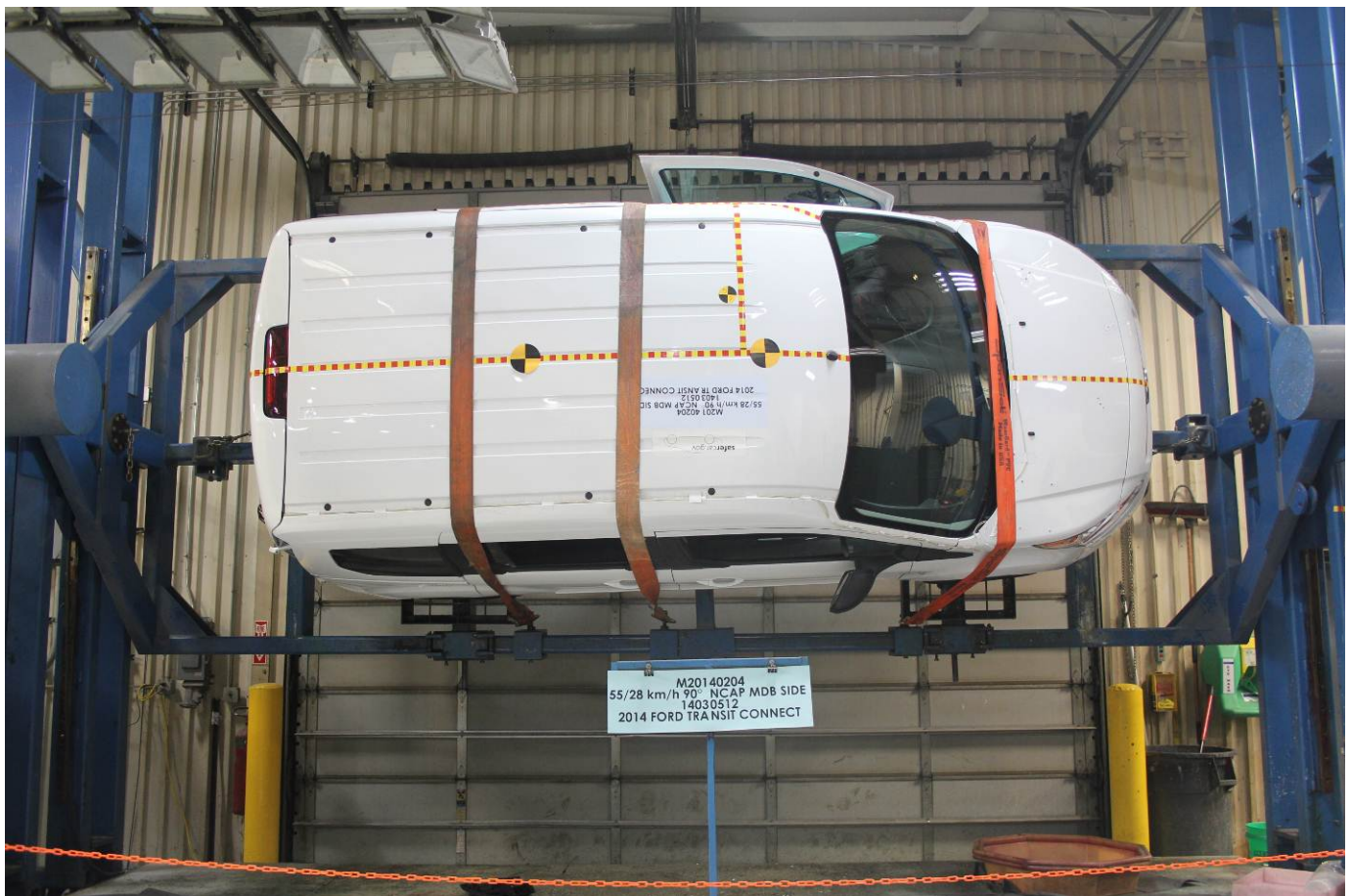
FMVSS No. 301 Static Rollover 90 Degrees
