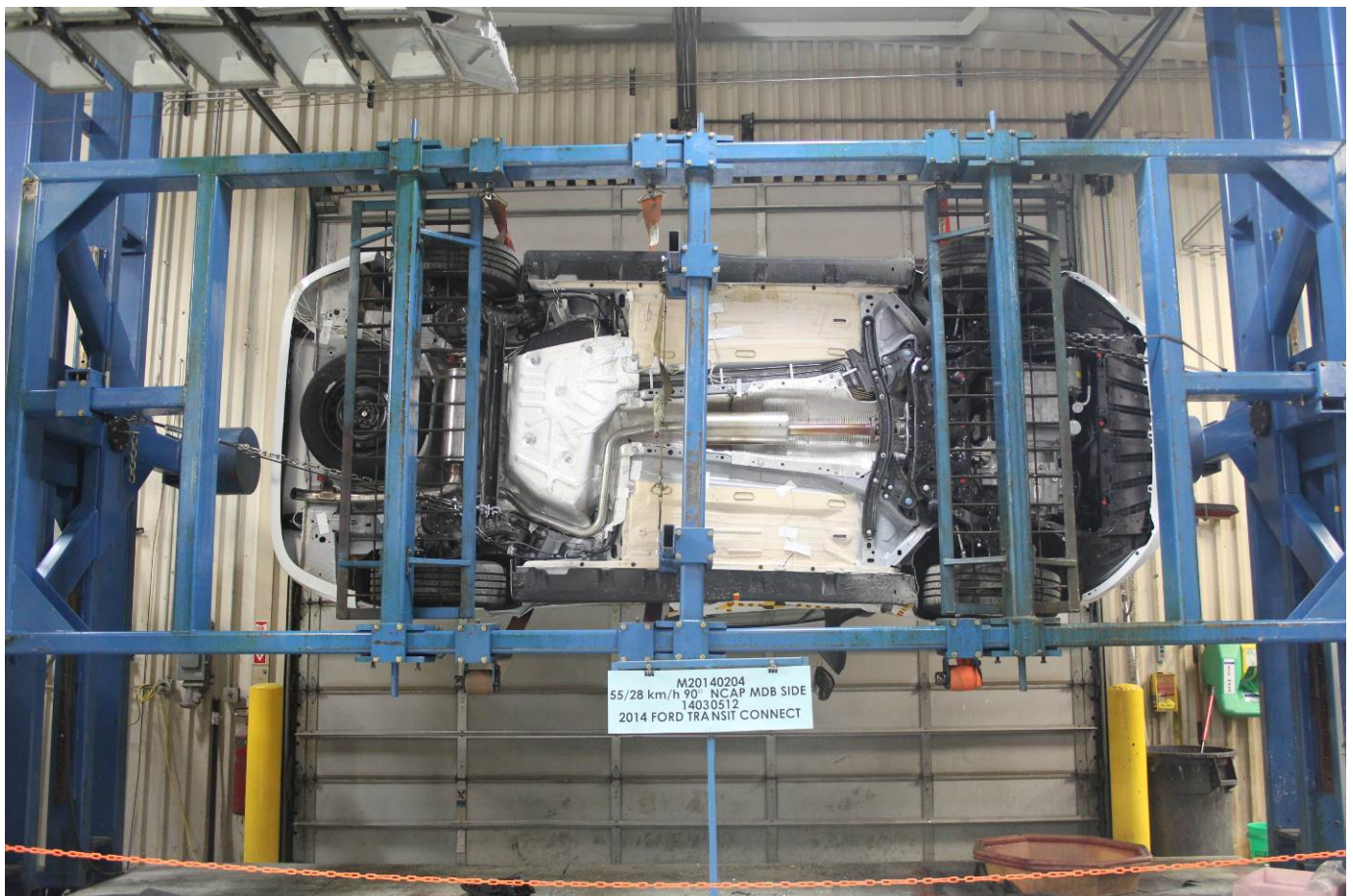
FMVSS No. 301 Static Rollover 270 Degrees
