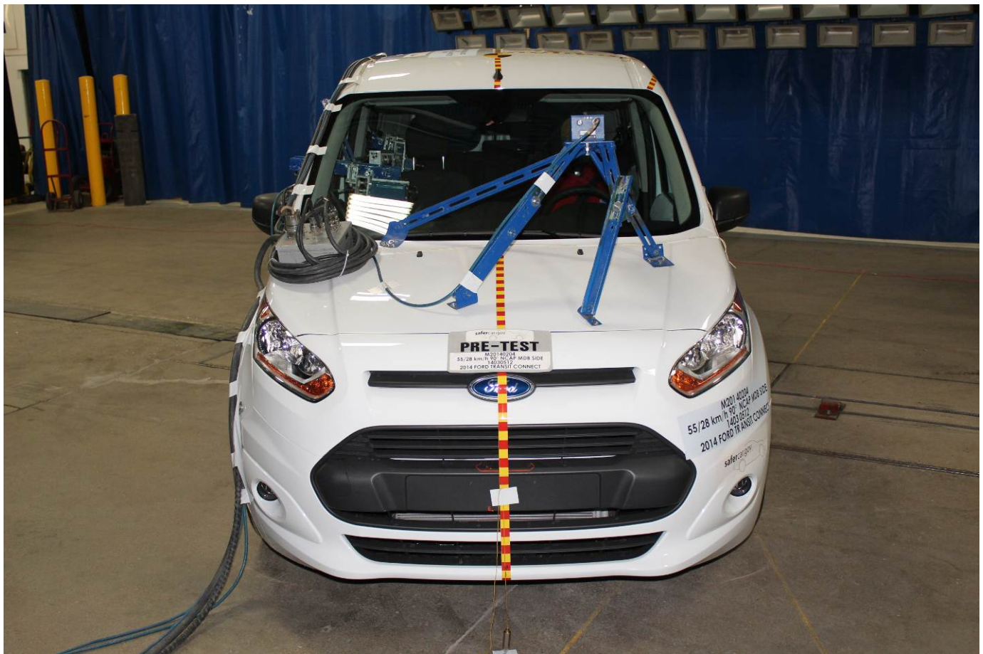
Pre-Test Frontal View of Test Vehicle
