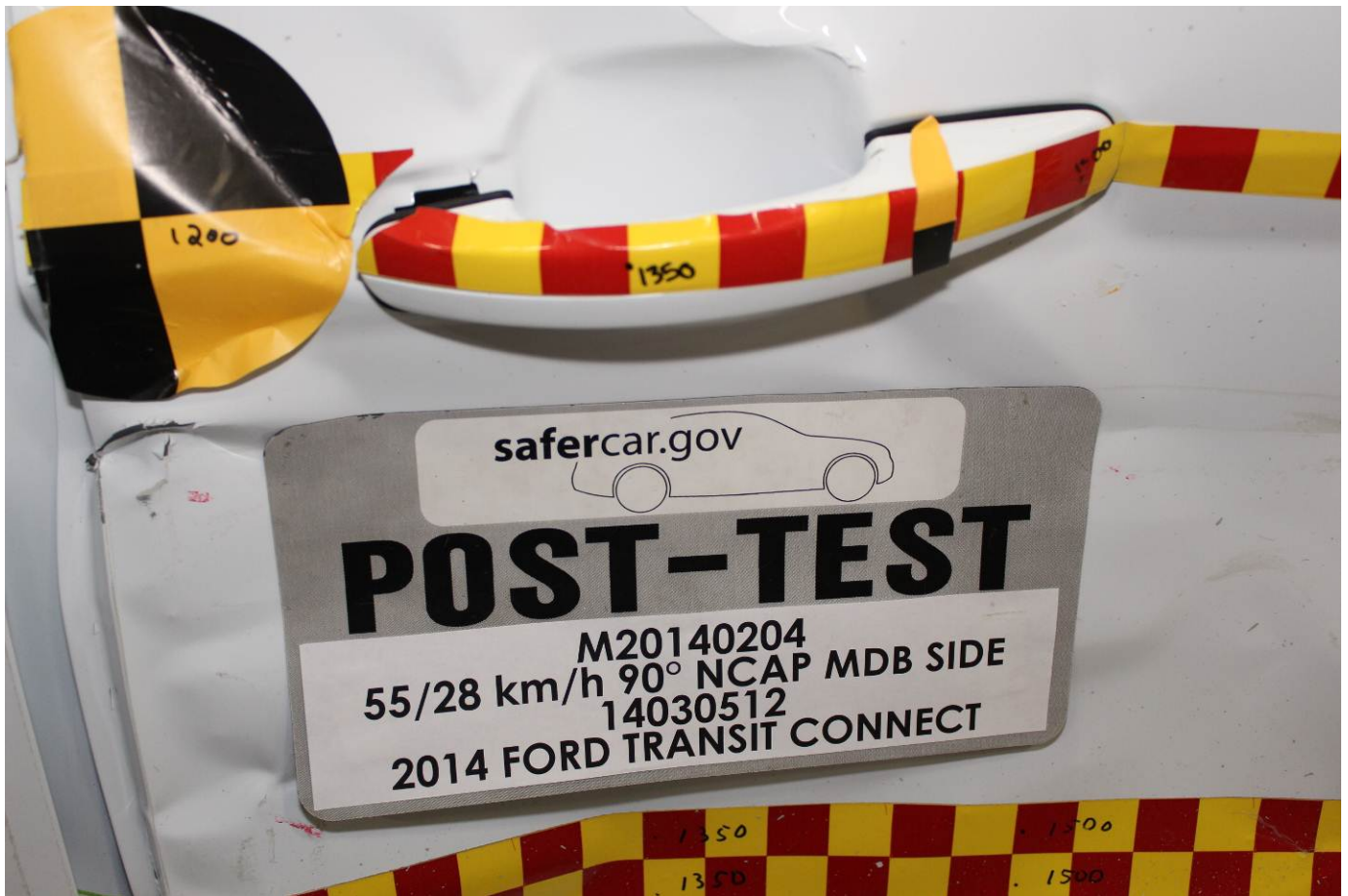
Post-Test Left Rear Door Latch Close-Up
