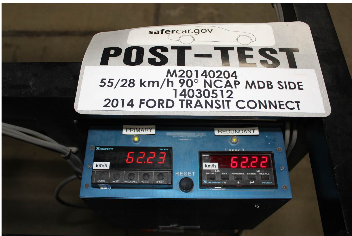
Post-Test Primary and Redundant Speed Trap Read-Out
