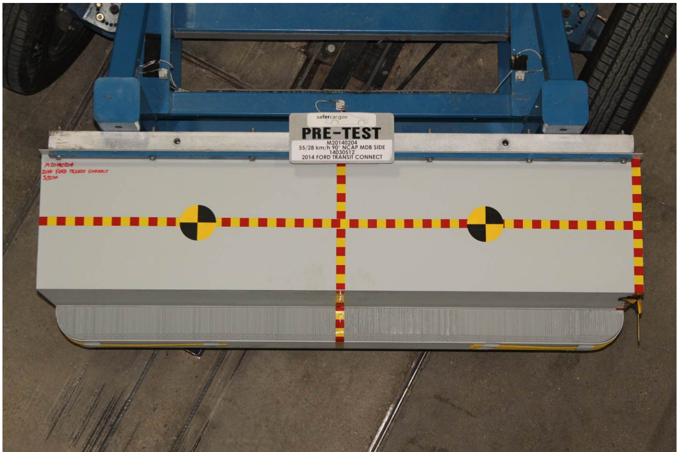
Pre-Test Top View of MDB Impactor Face
