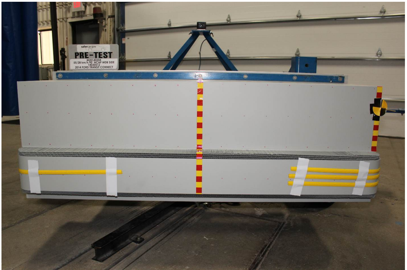
Pre-Test Front View of MDB Impactor Face
