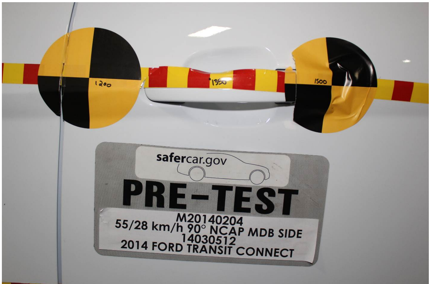
Pre-Test Left Rear Door Latch Close-Up
