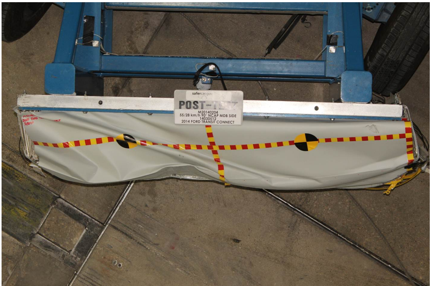
Post-Test Top View of MDB Impactor Face
