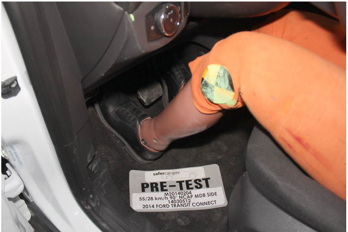
Pre-Test Placement of Driver Dummy's Feet
