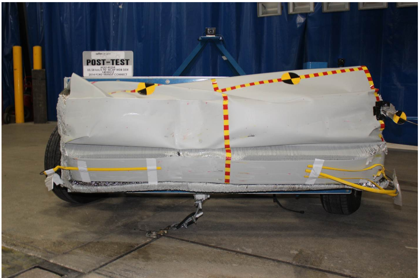
Post-Test Front View of MDB Impactor Face
