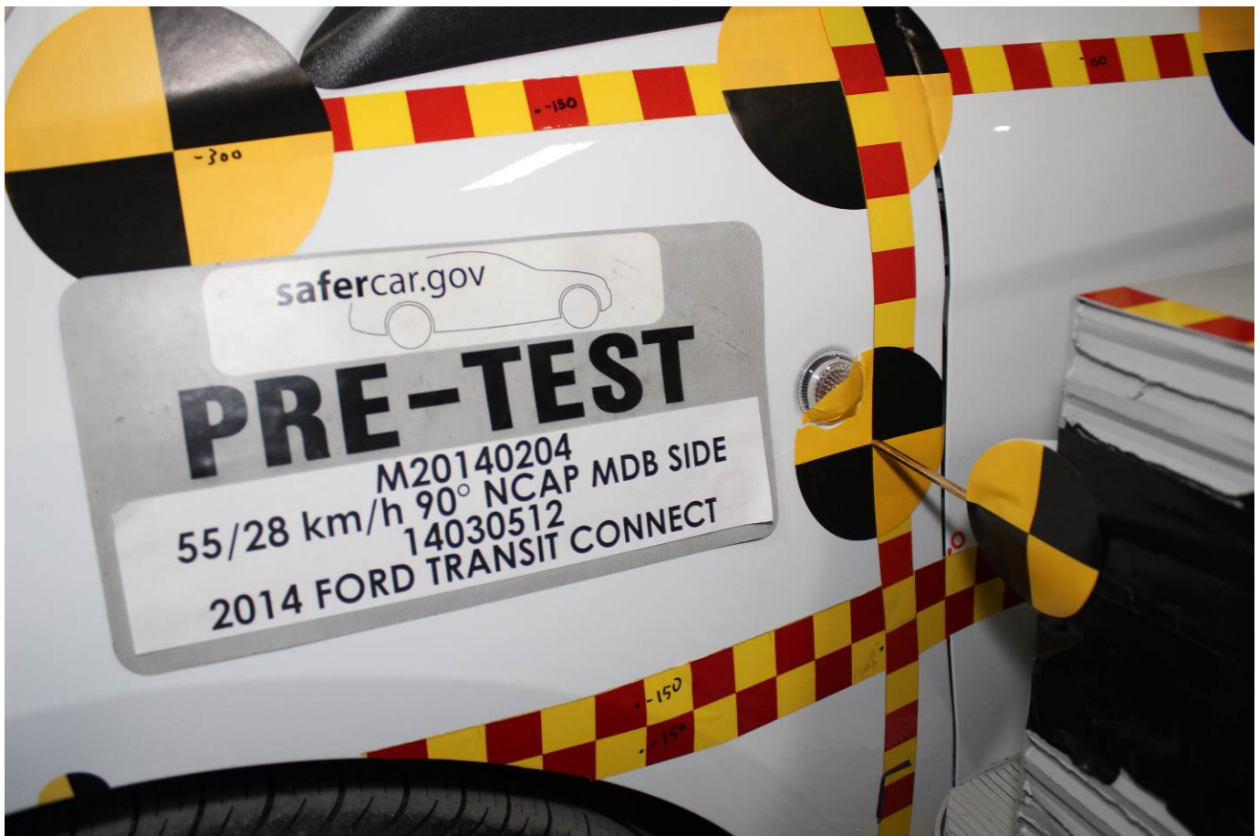
Pre-Test Close-Up View of Impact Point Target
