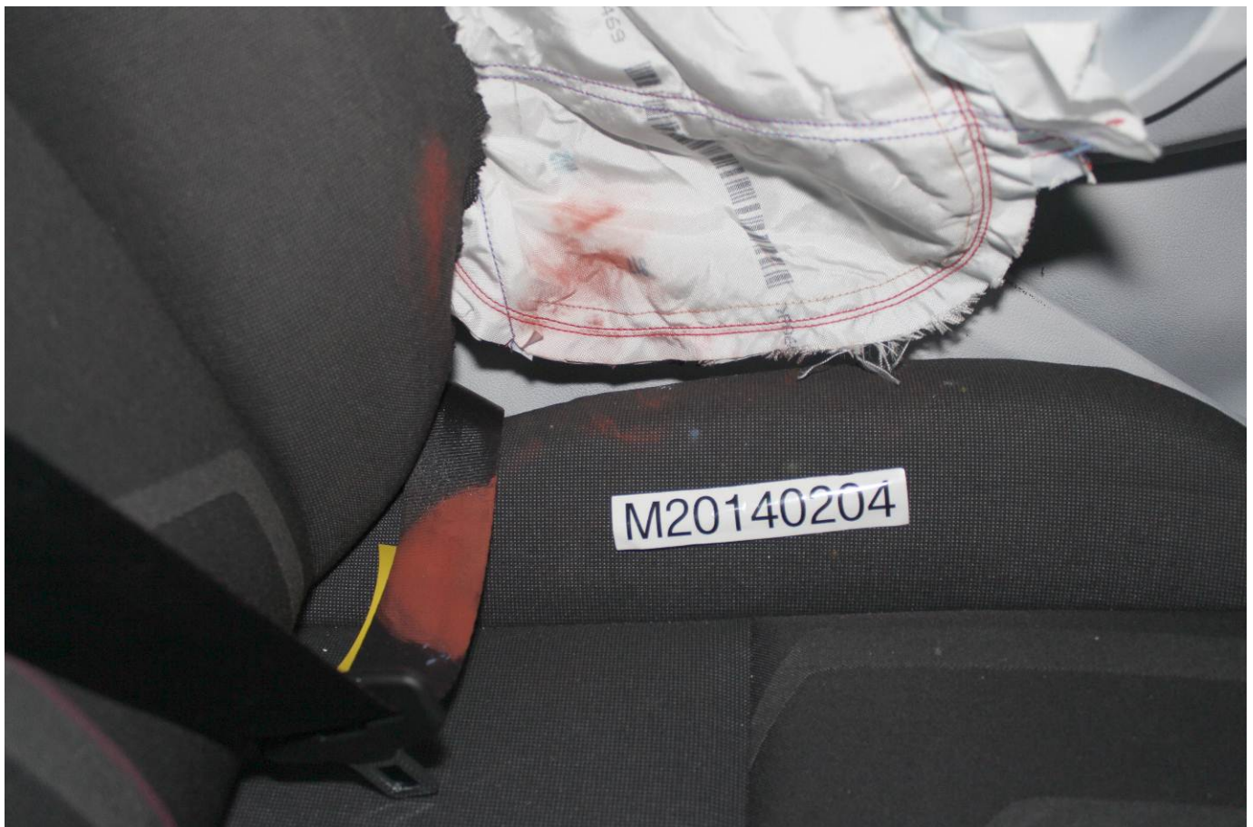
Post-Test Driver Dummy Close-up Pelvis Contact with Side Airbag View
