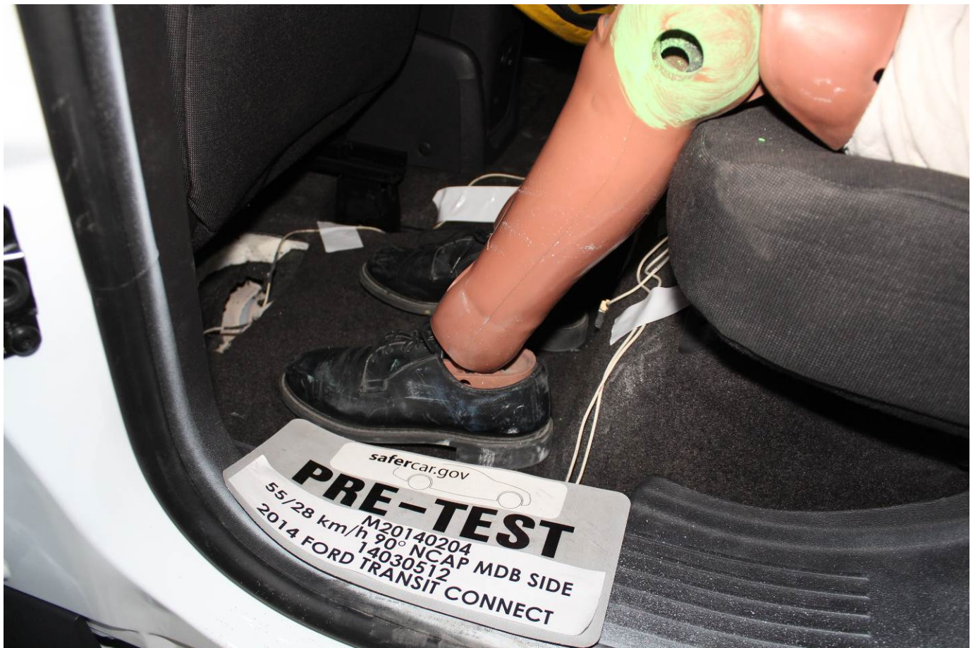
Pre-Test Placement of Rear Passenger Dummy's Feet
