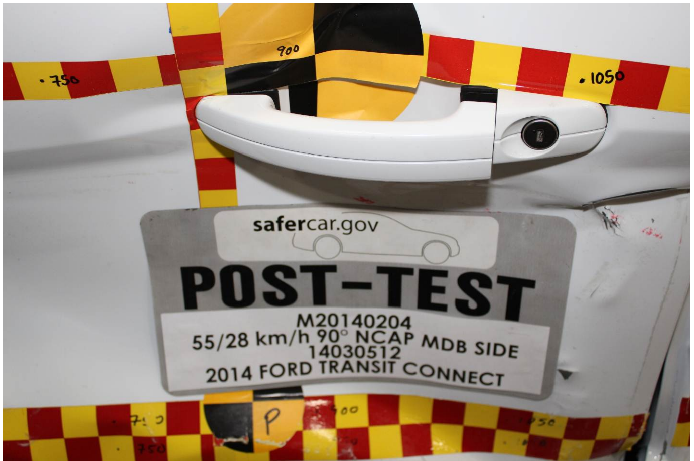
Post-Test Left Front Door Latch Close-Up
