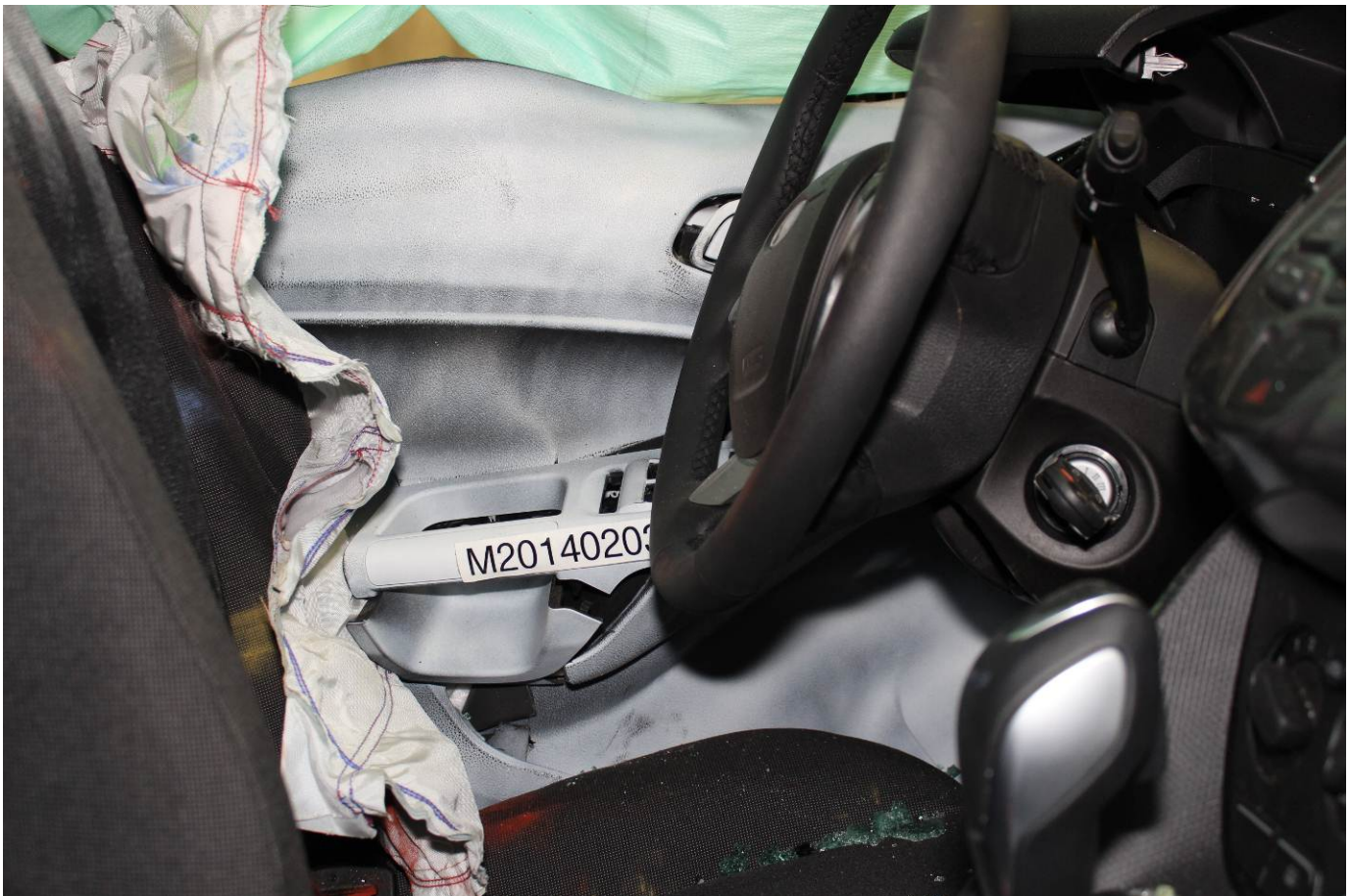
Post-Test View of Shattered Vehicle Inner Door Panel
