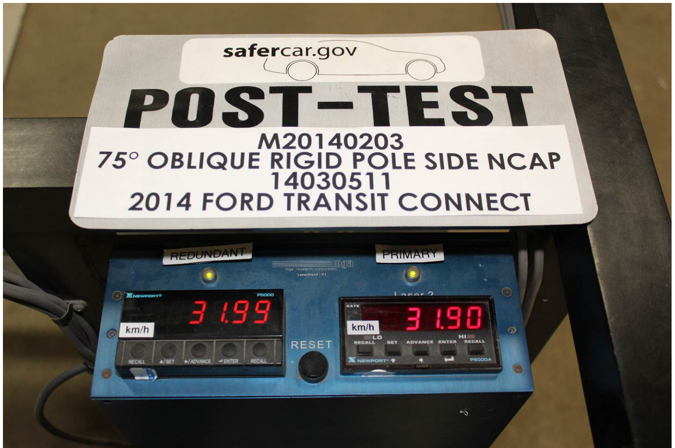
Post-Test Primary and Redundant Speed Trap Read-Out
