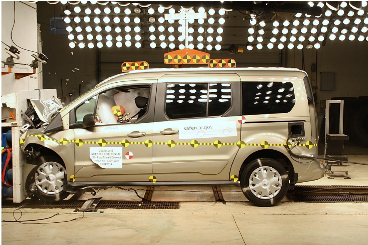
Figure A-77: 2014 Ford Transit Connect Frontal Impact Event
