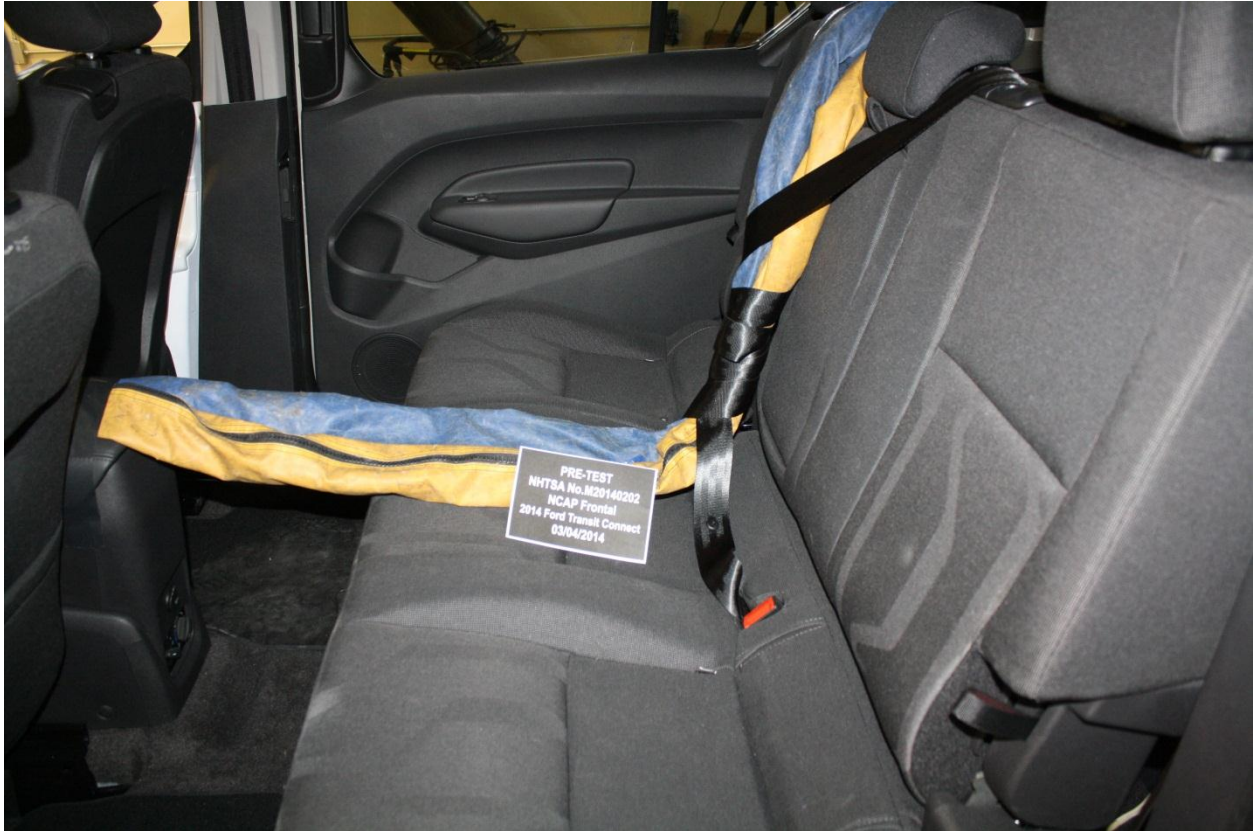
Figure A-27: Pre-Test Dummy Cable Routing
