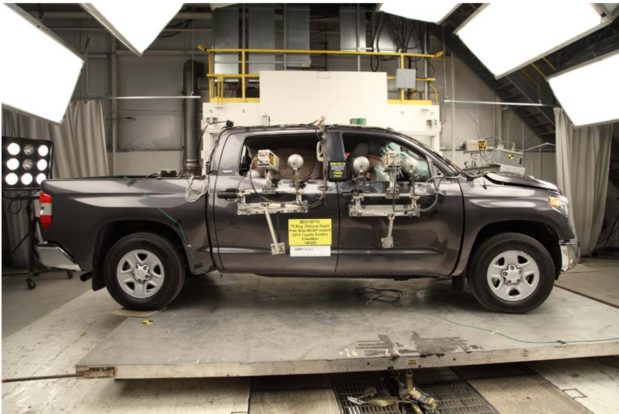
014 Post-Test Right Side View of Test Vehicle
