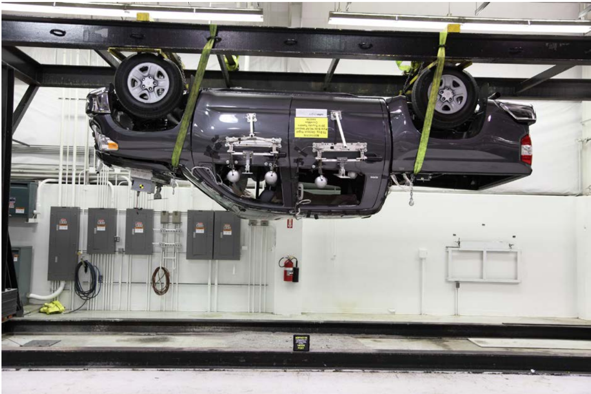
065 FMVSS No. 301 Static Rollover 180 Degrees
