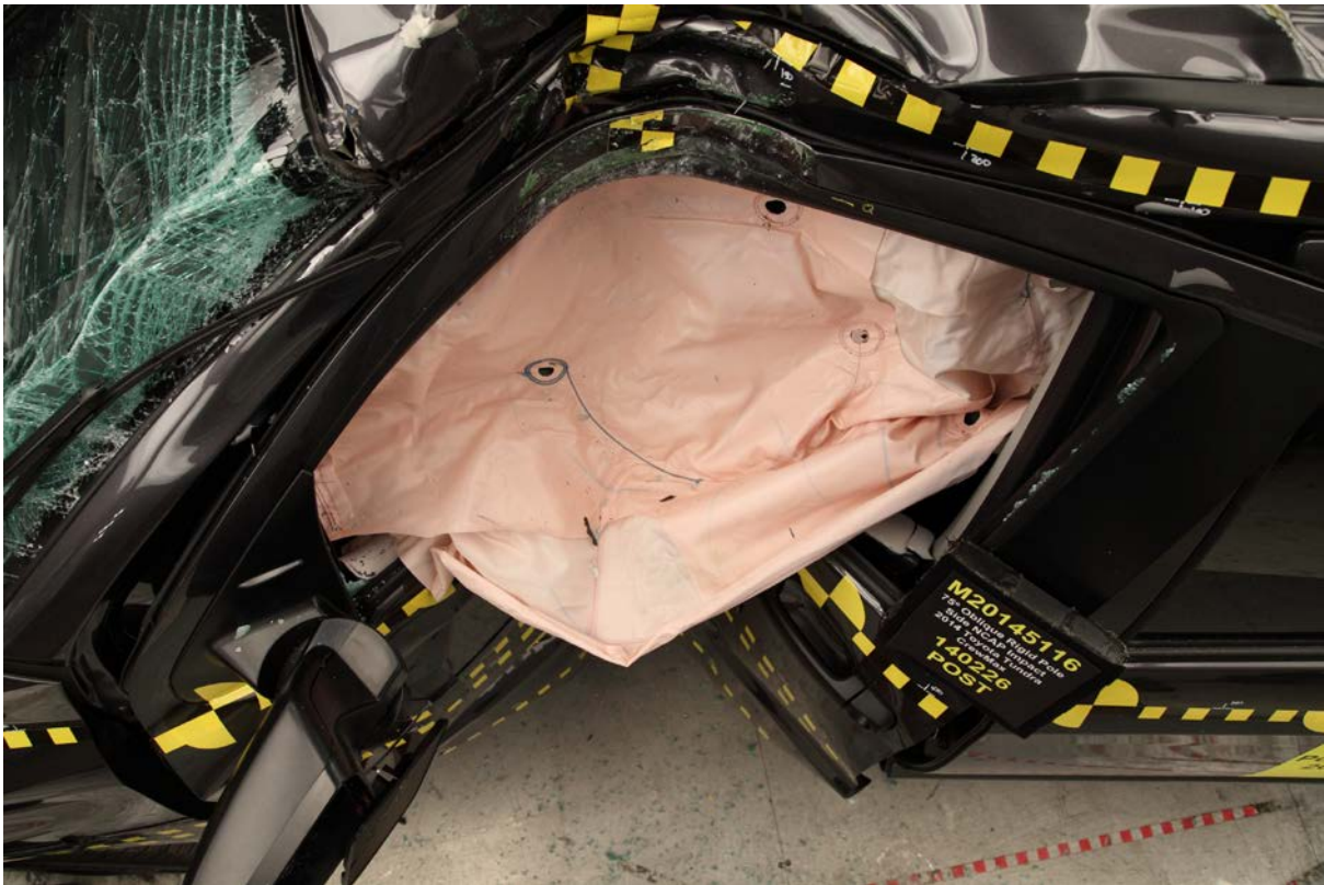
041 Post-Test Dummy and Door Clearance View
