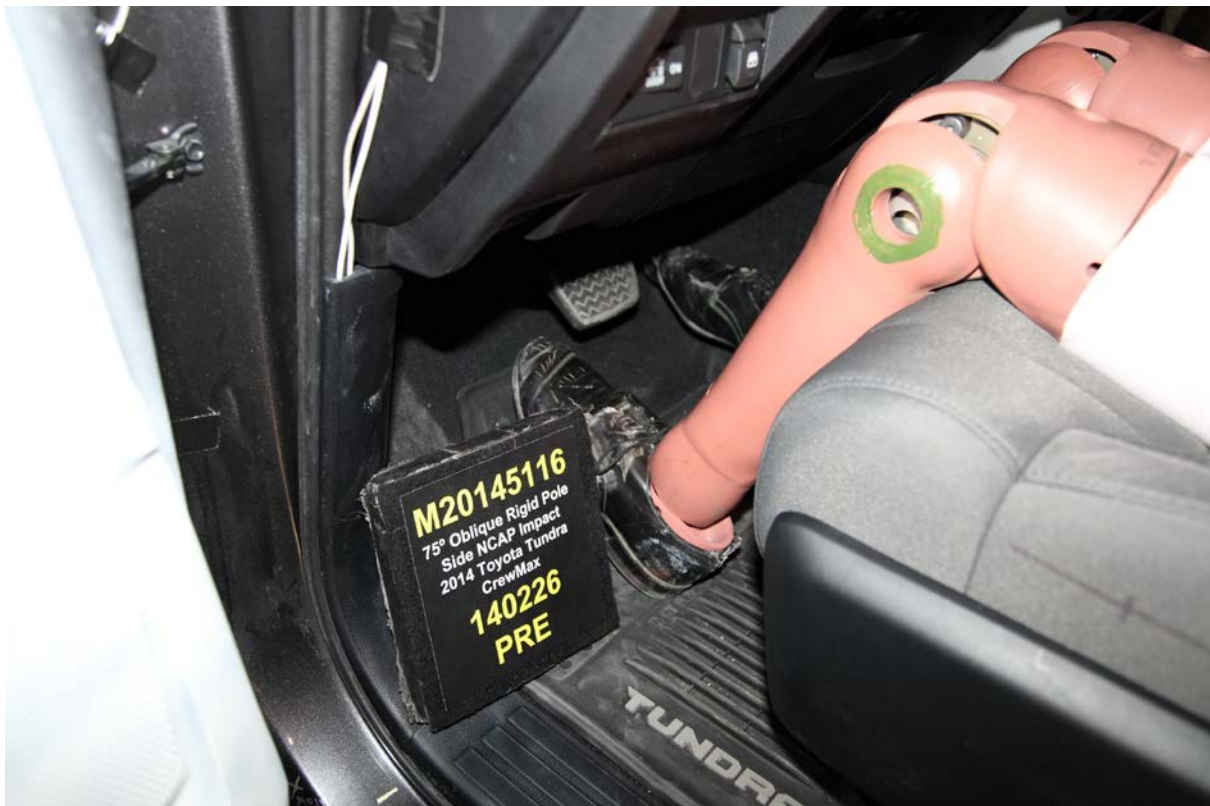
032 Pre-Test Placement of Dummy Feet
