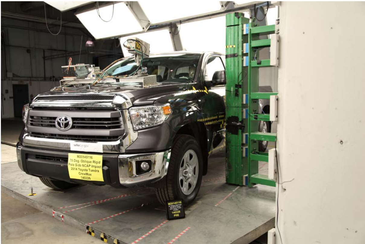
005 Pre-Test Left Front 3-4 View of Test Vehicle
