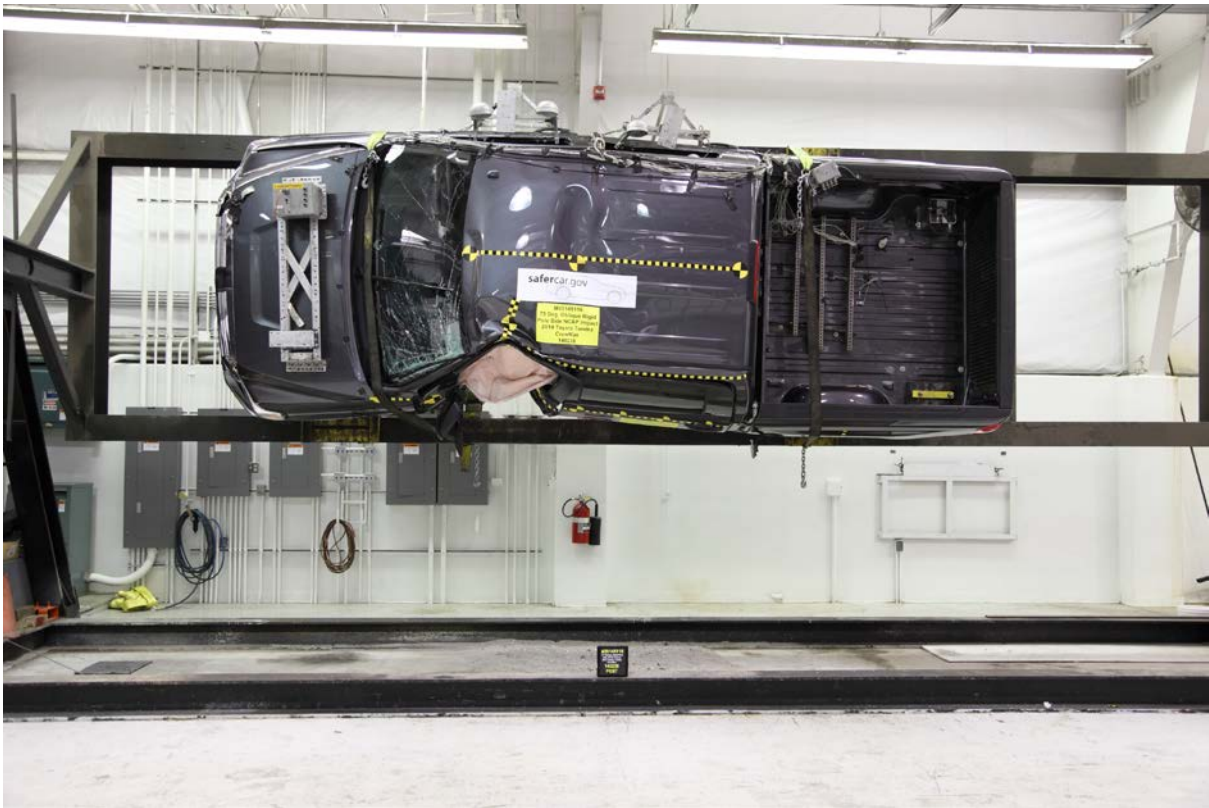
064 FMVSS No. 301 Static Rollover 90 Degrees
