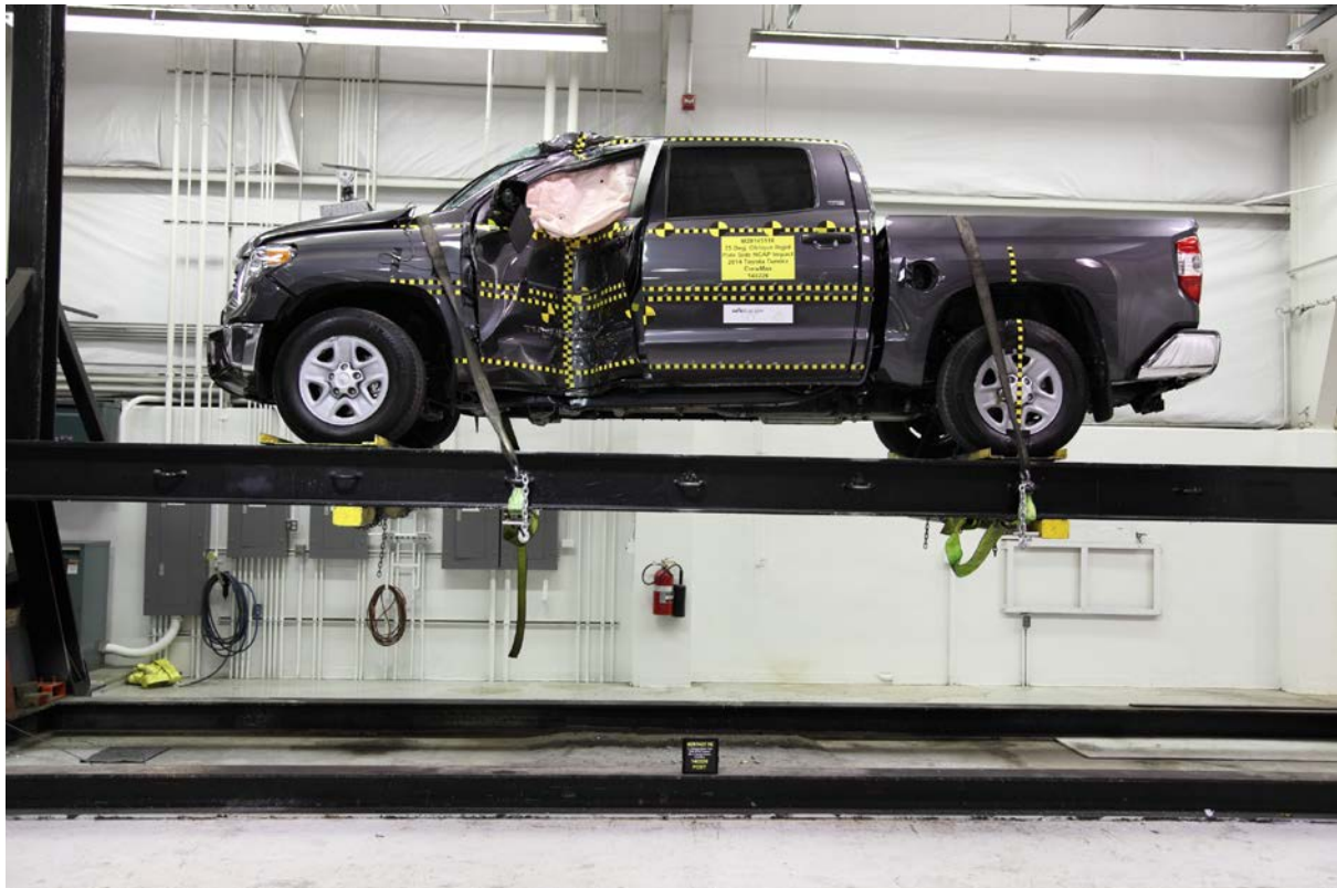
063 FMVSS No. 301 Static Rollover 0 Degrees
