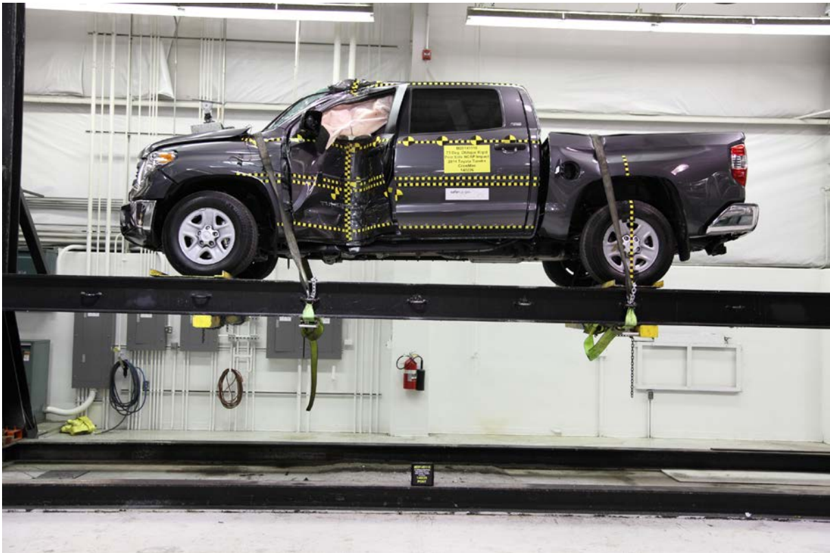
067 FMVSS No. 301 Static Rollover 360 Degrees
