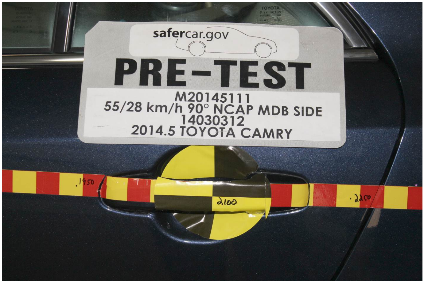
Pre-Test Left Rear Door Latch Close-Up
