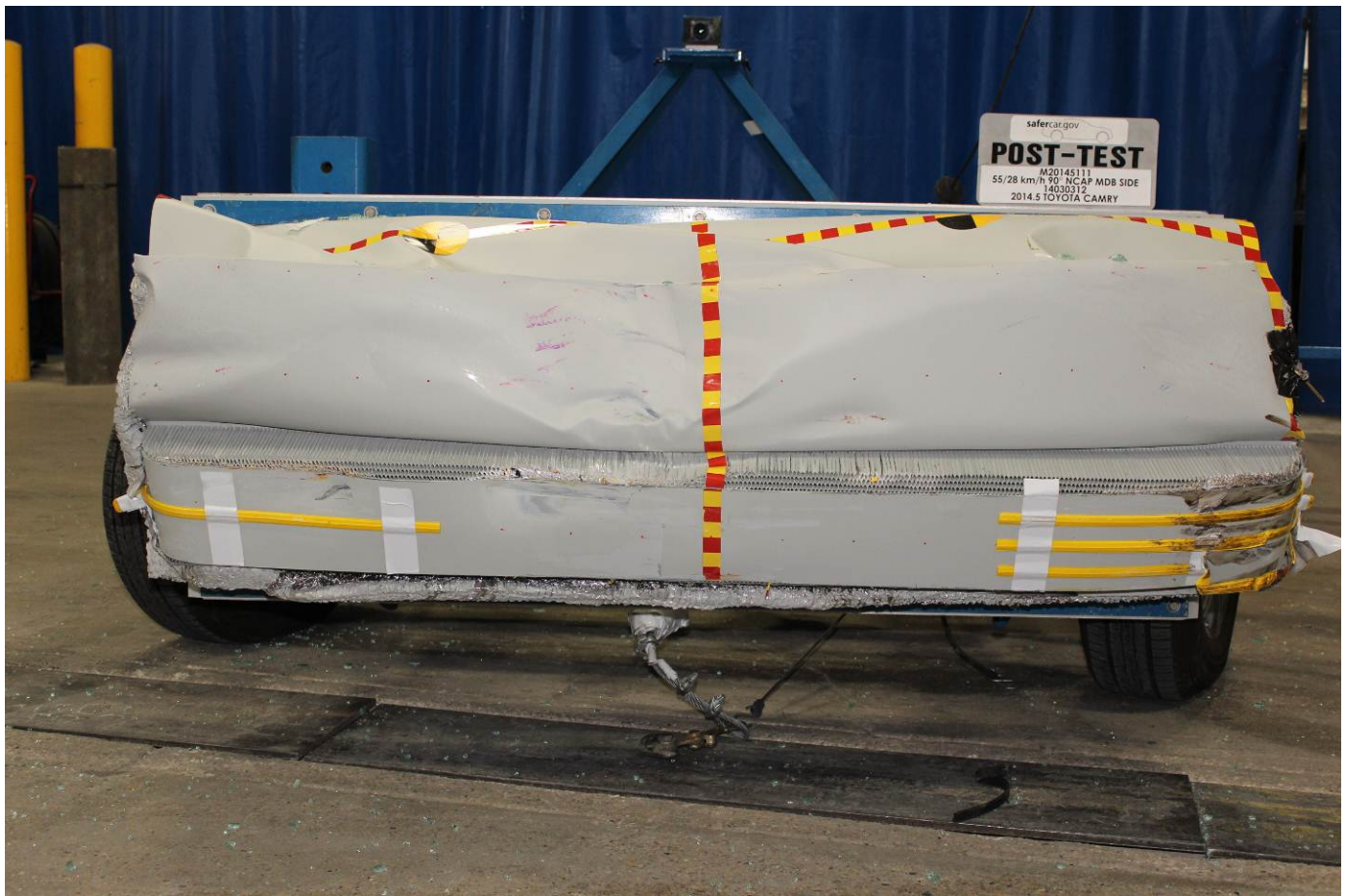
Post-Test Front View of MDB Impactor Face
