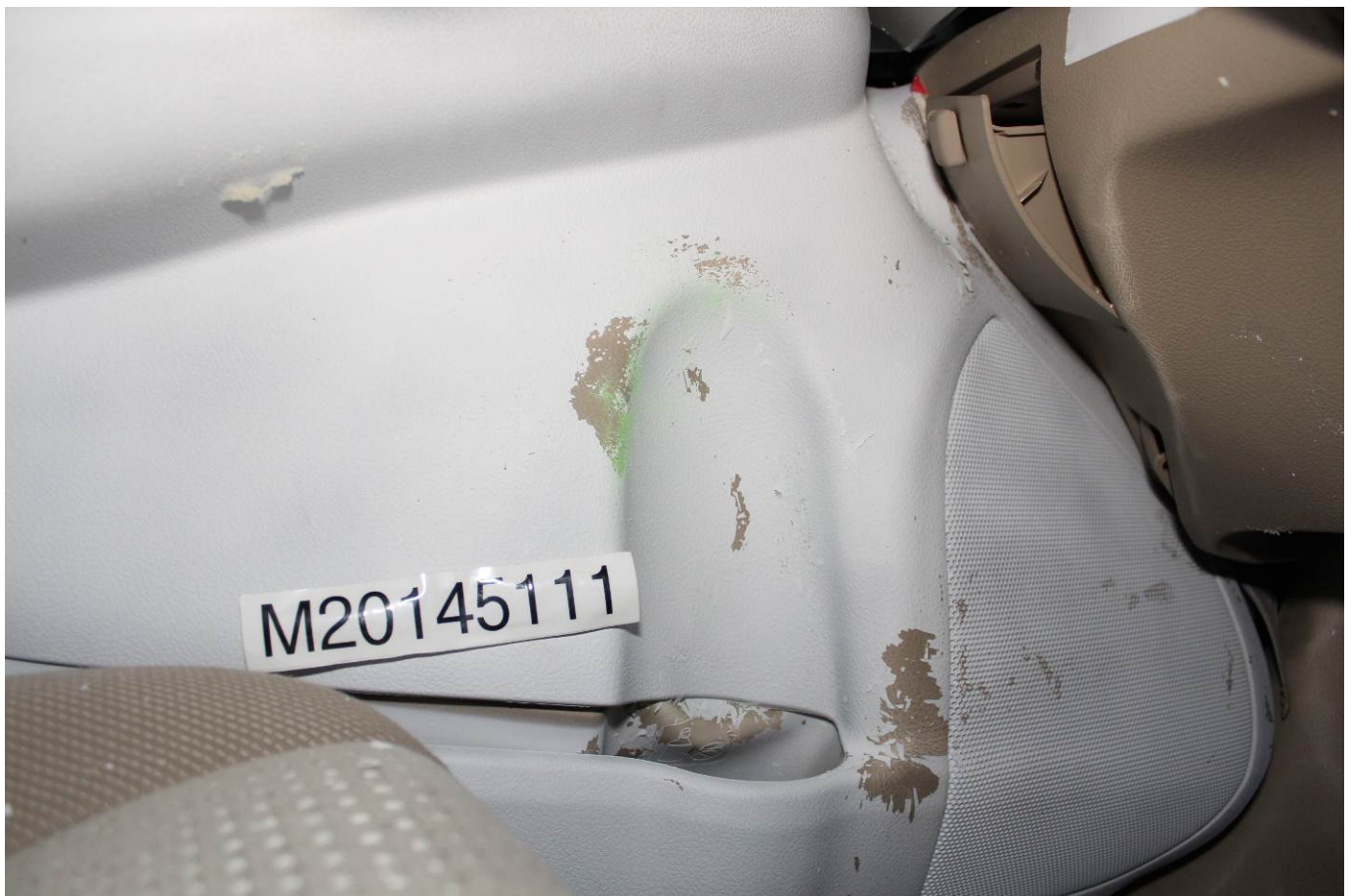
Post-Test Driver Dummy Close-up Knee Contact View
