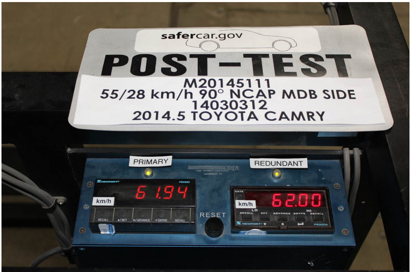
Post-Test Primary and Redundant Speed Trap Read-Out
