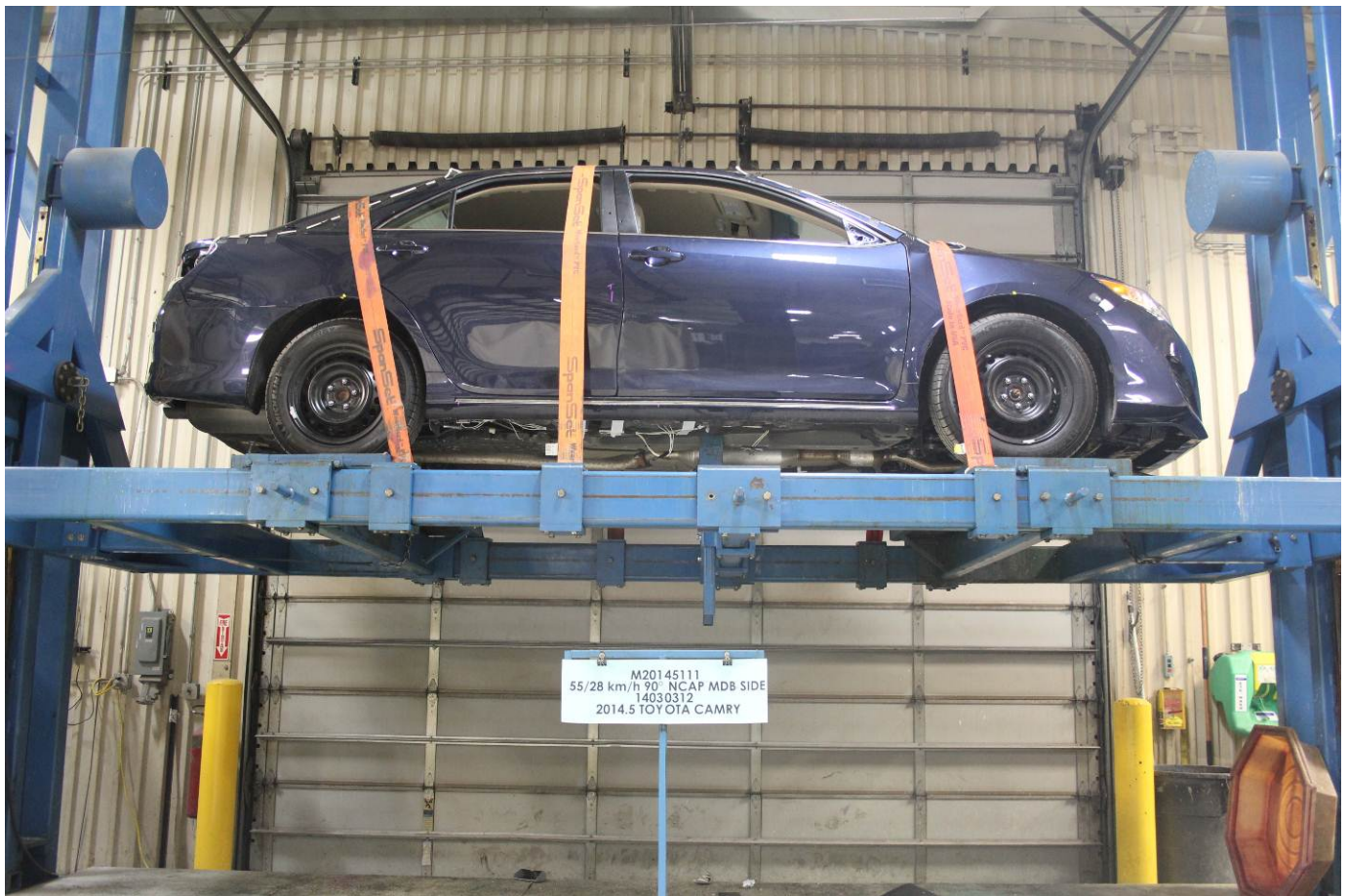
FMVSS No. 301 Static Rollover 0 Degrees
