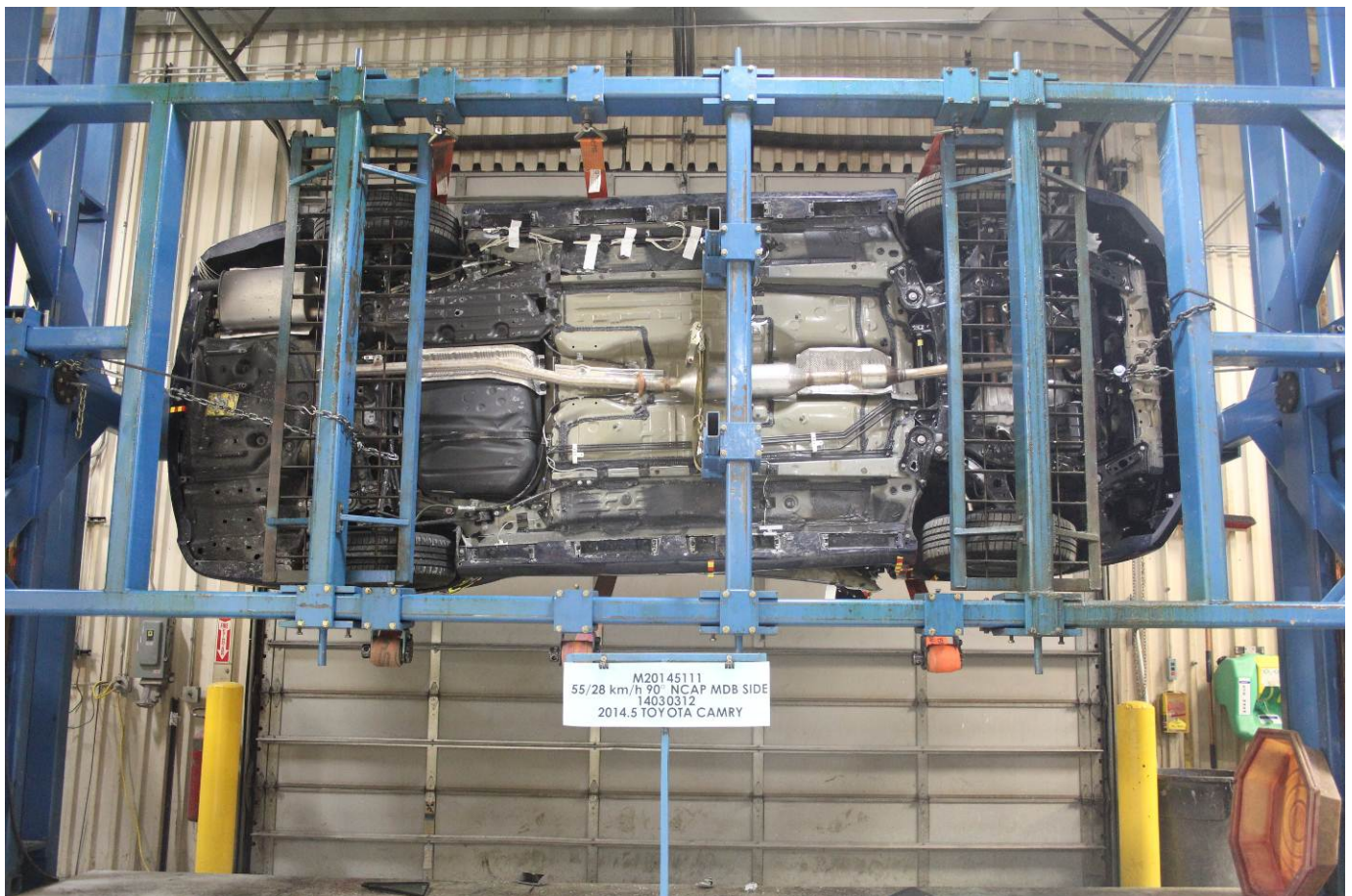
FMVSS No. 301 Static Rollover 90 Degrees
