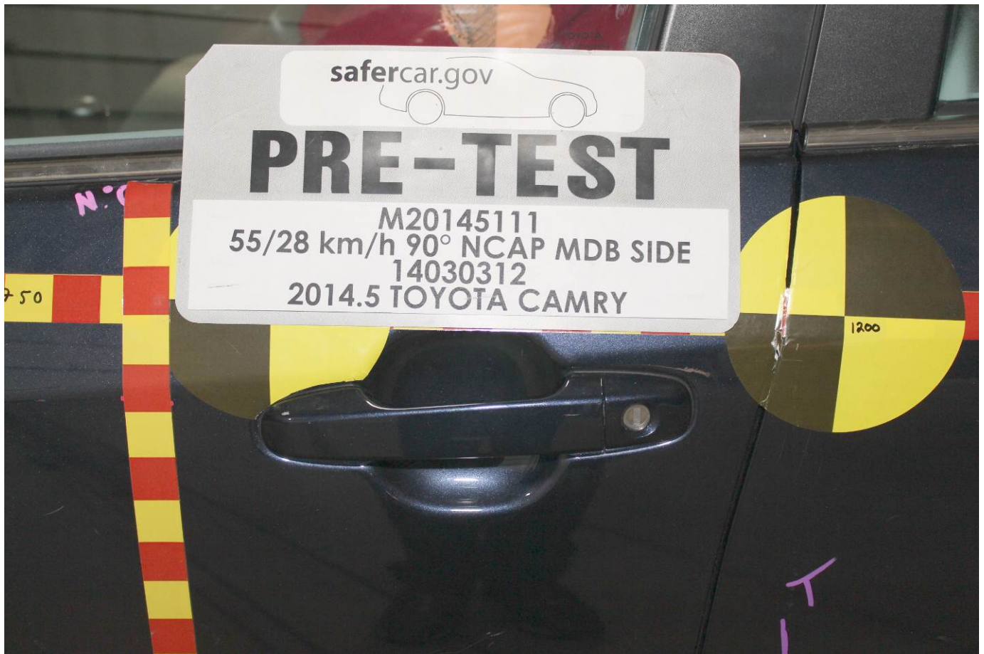
Pre-Test Left Front Door Latch Close-Up
