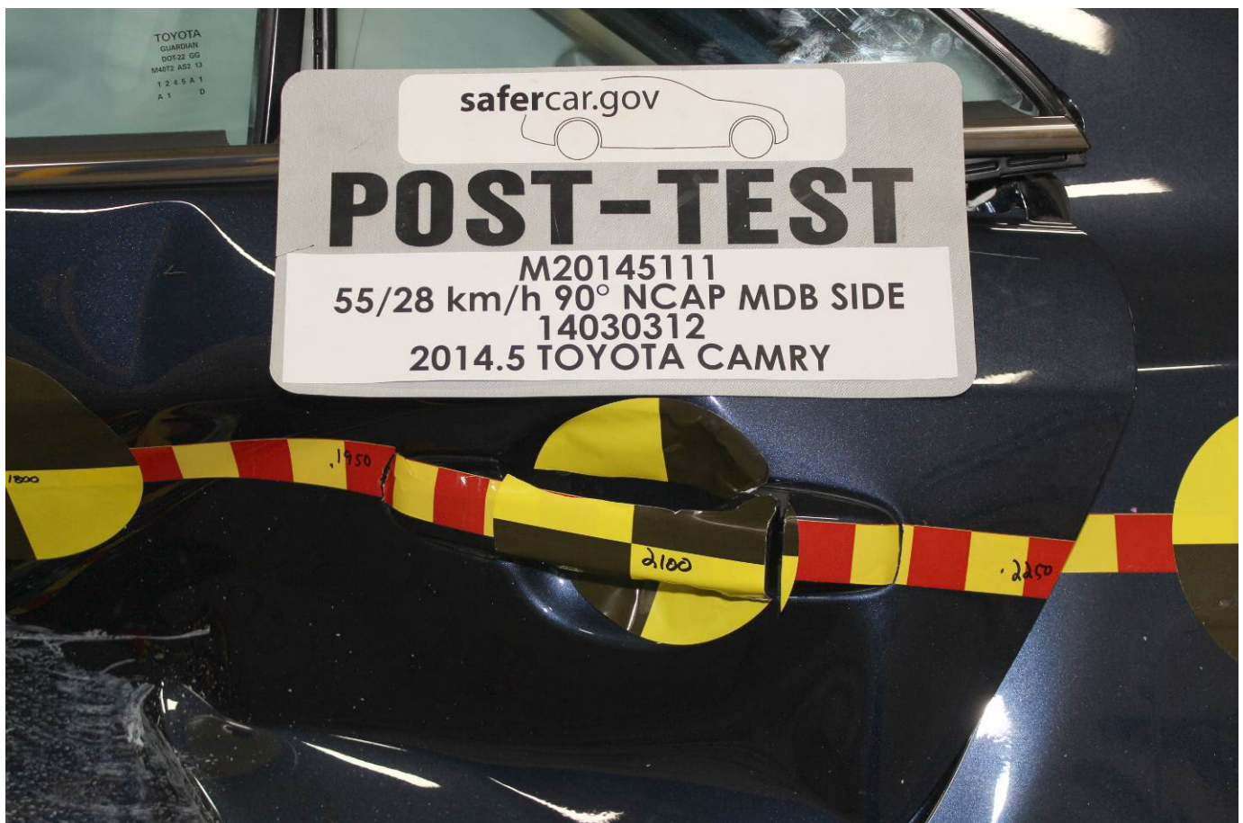
Post-Test Left Rear Door Latch Close-Up
