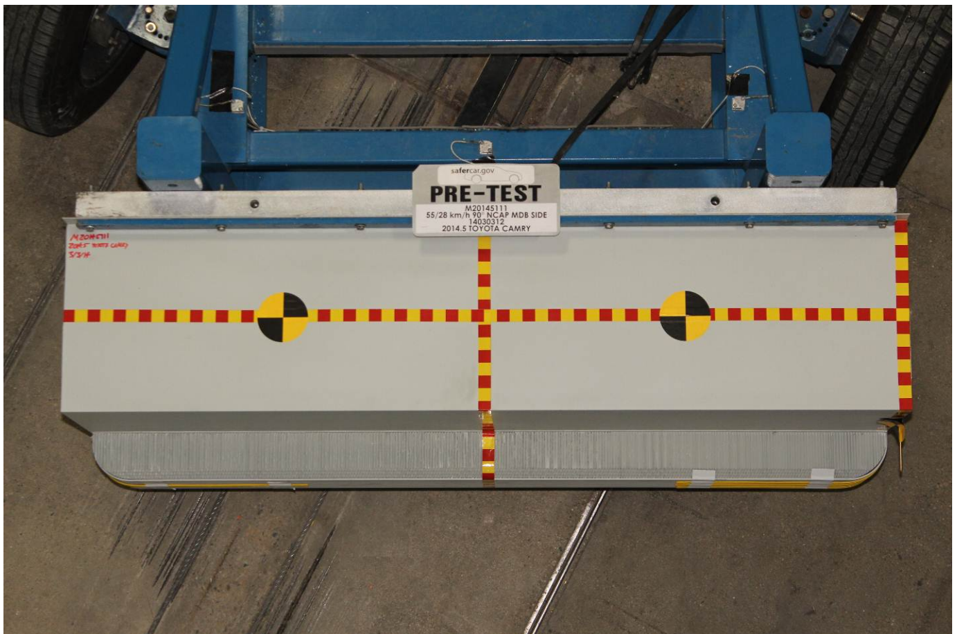
Pre-Test Top View of MDB Impactor Face
