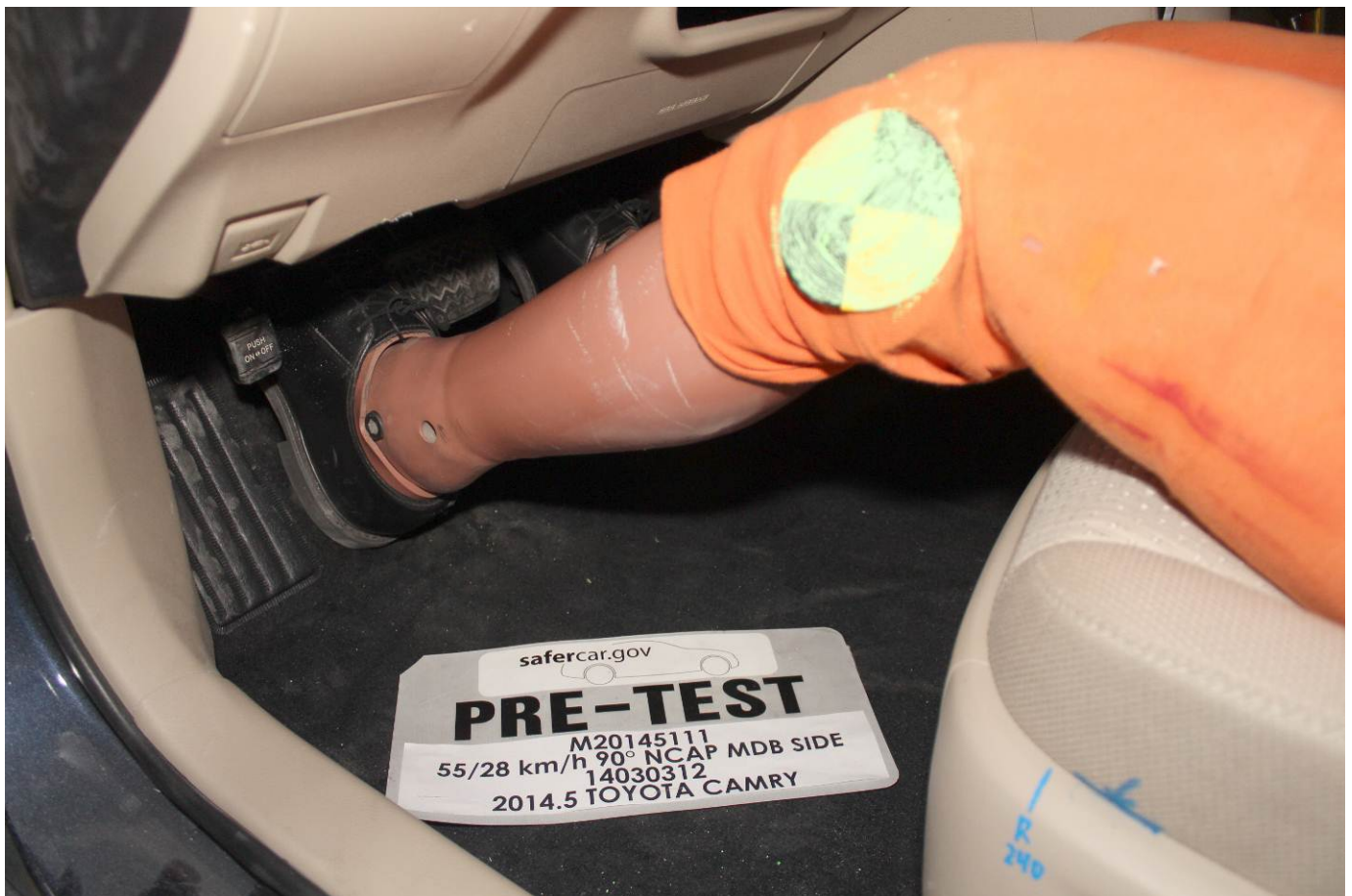
Pre-Test Placement of Driver Dummy's Feet
