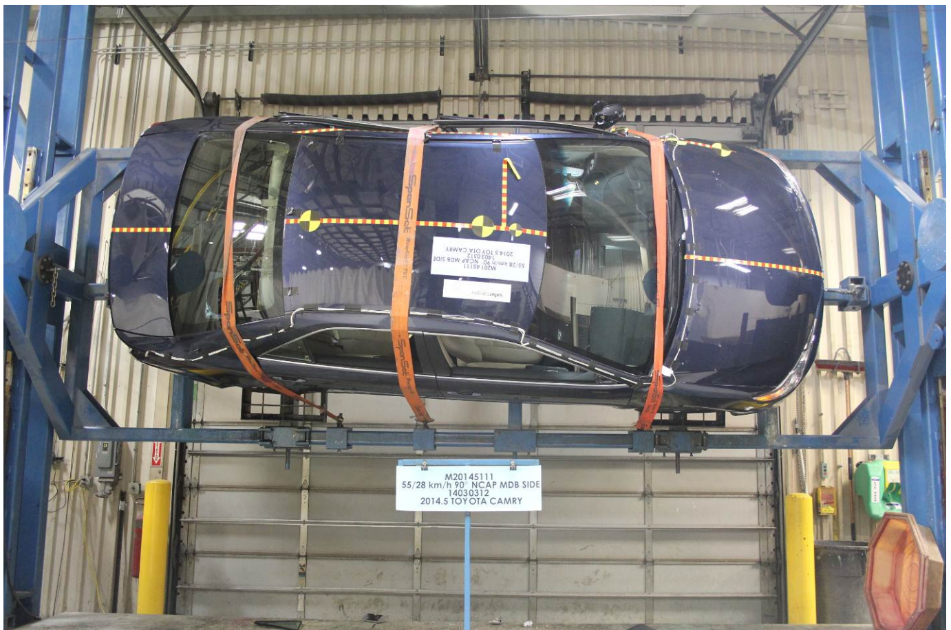
FMVSS No. 301 Static Rollover 270 Degrees
