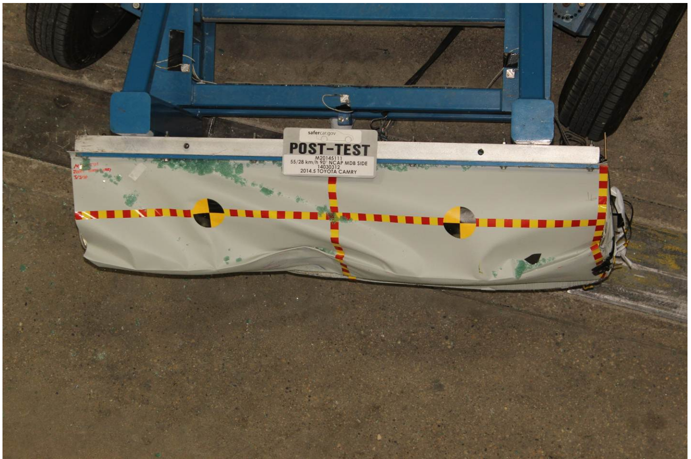
Post-Test Top View of MDB Impactor Face
