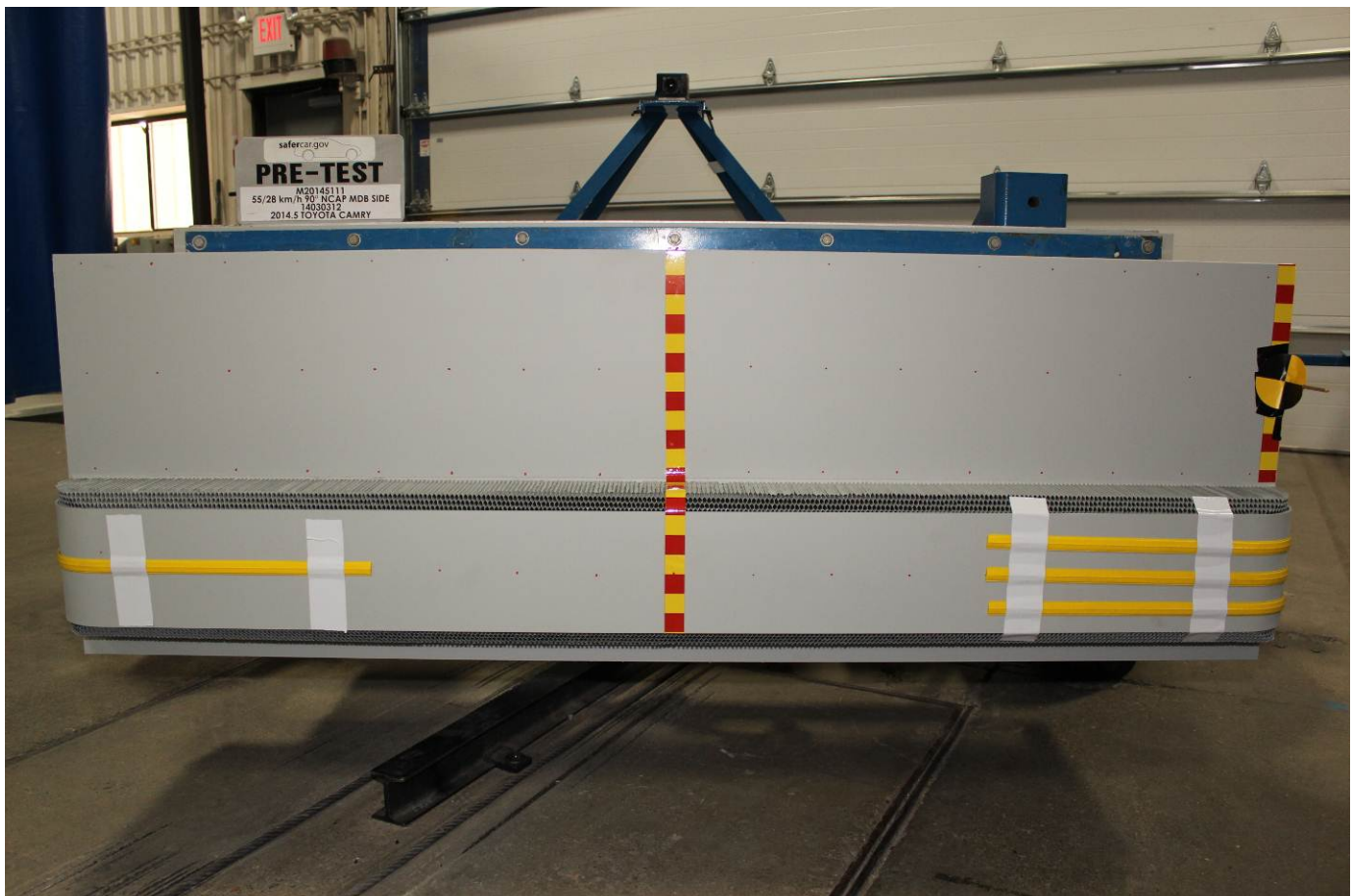
Pre-Test Front View of MDB Impactor Face
