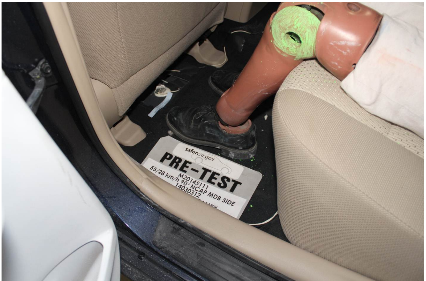
Pre-Test Placement of Rear Passenger Dummy's Feet
