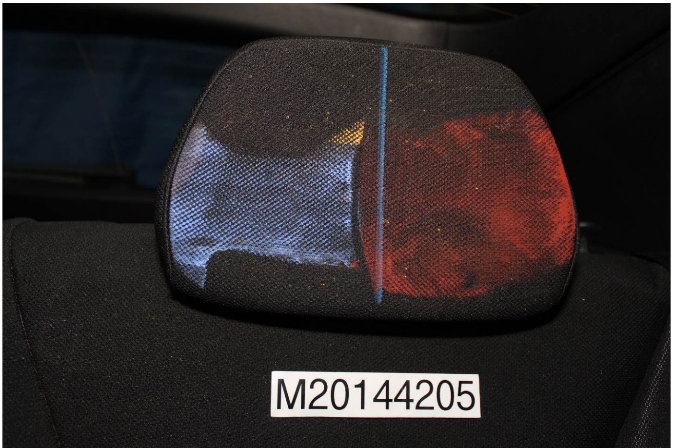
Post-Test Rear Passenger Dummy Close-up Head Contact with Vehicle Interior View
