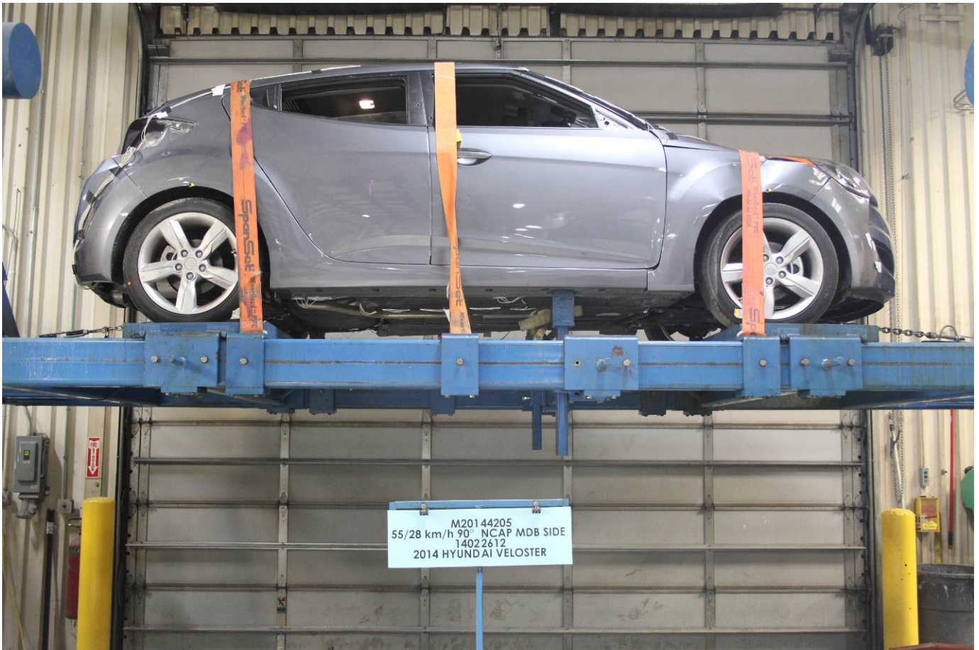
FMVSS No. 301 Static Rollover 360 Degrees
