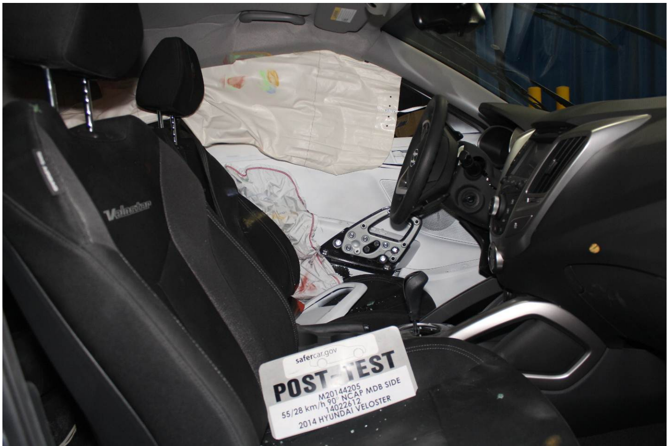
Post-Test Driver Inner Door Panel View
