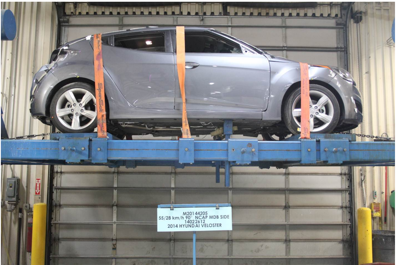
FMVSS No. 301 Static Rollover 0 Degrees
