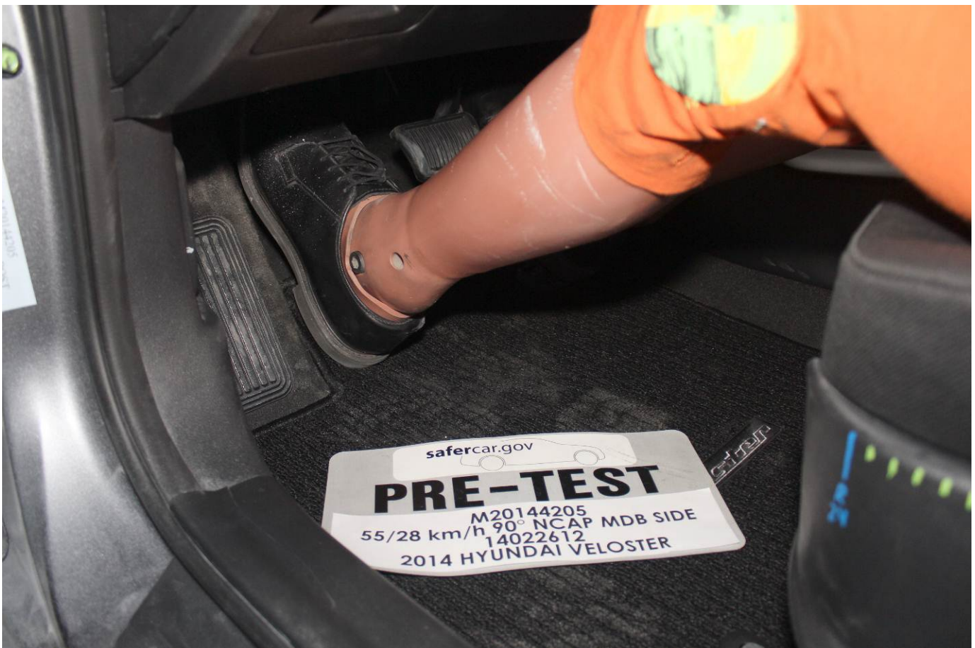
Pre-Test Placement of Driver Dummy's Feet
