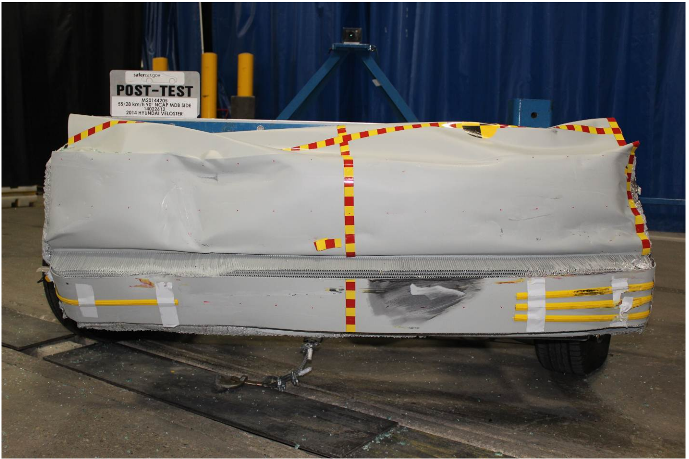
Post-Test Front View of MDB Impactor Face
