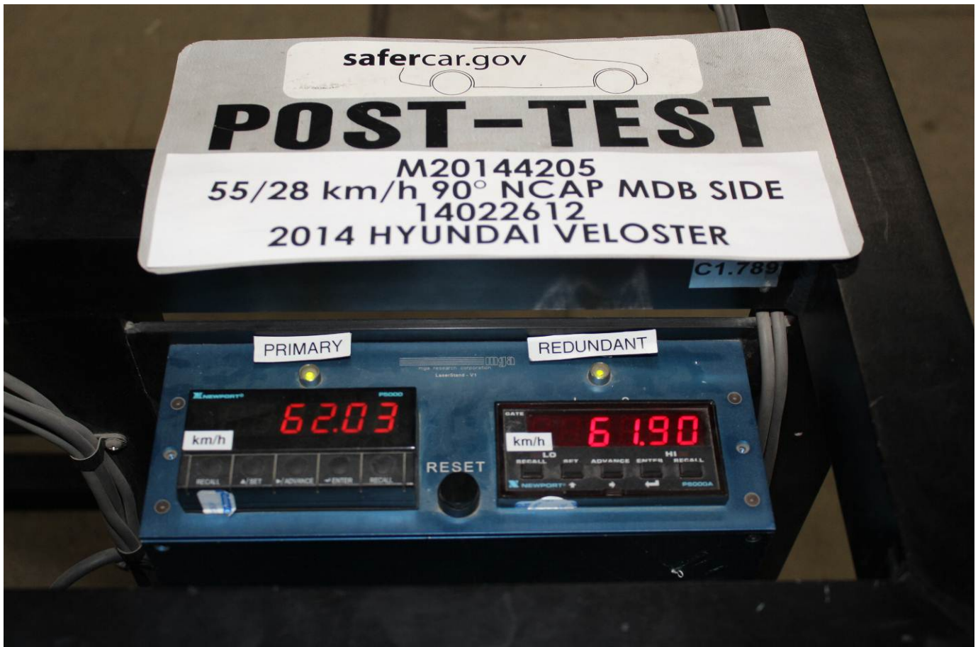
Post-Test Primary and Redundant Speed Trap Read-Out
