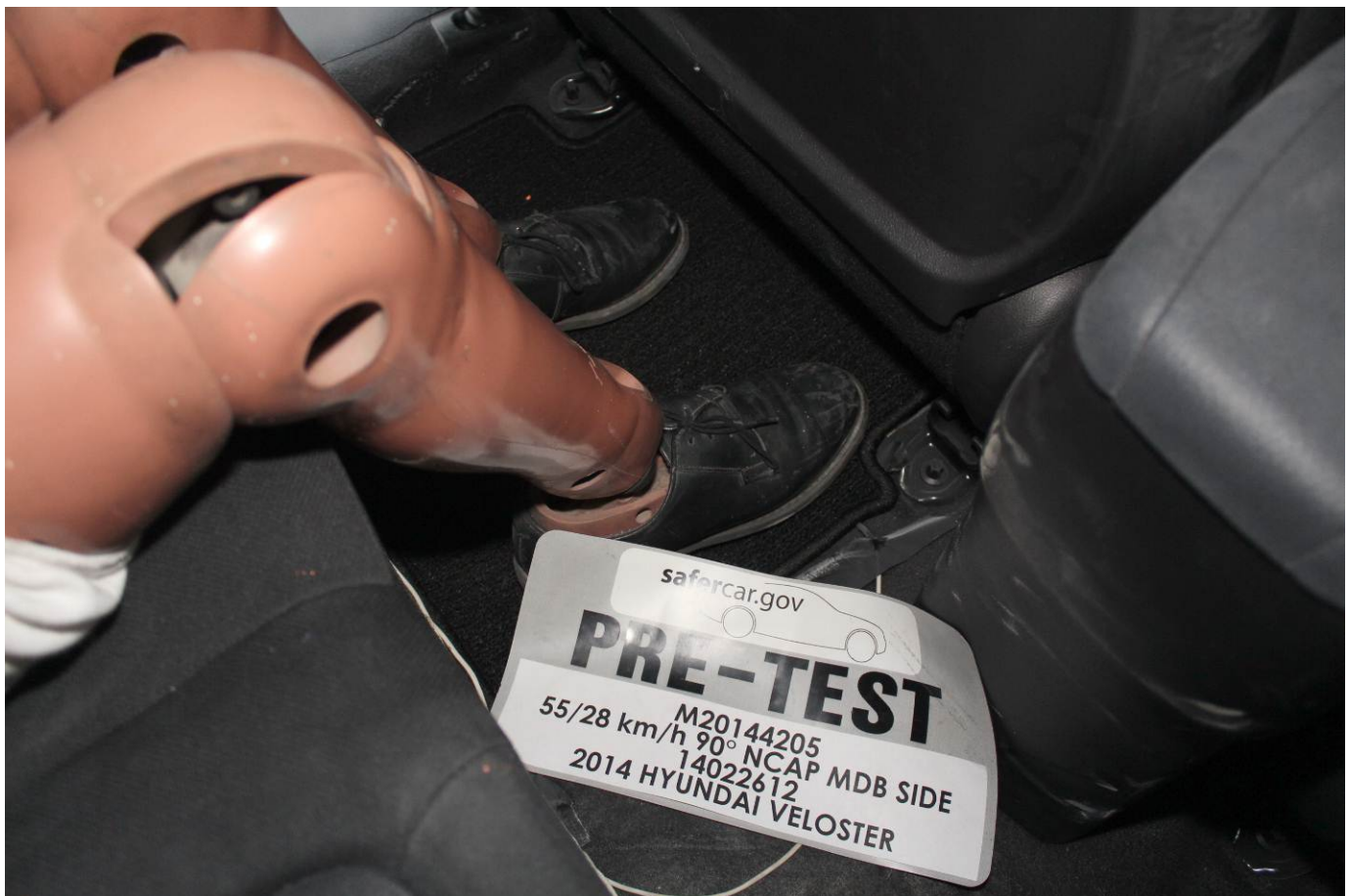
Pre-Test Placement of Rear Passenger Dummy's Feet
