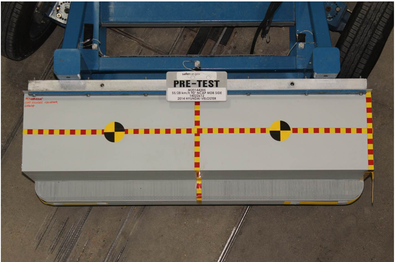
Pre-Test Top View of MDB Impactor Face
