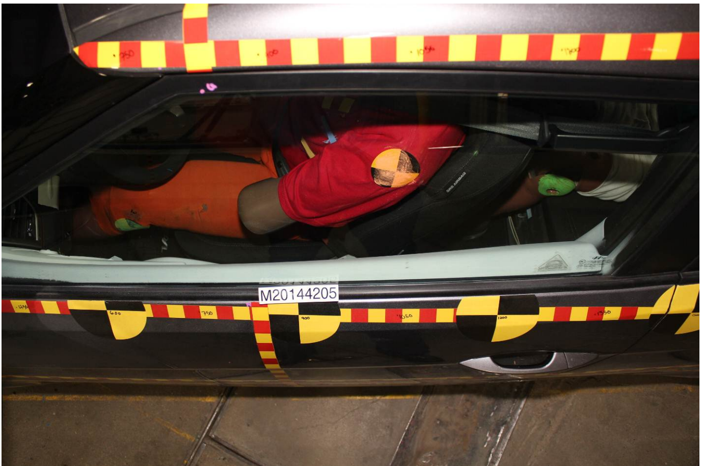
Pre-Test Driver Dummy and Door Clearance View
