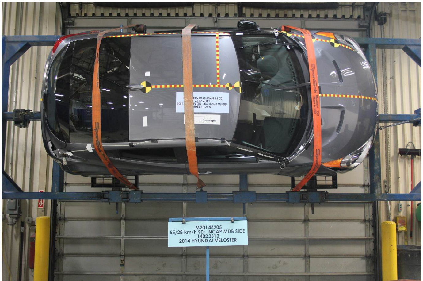
FMVSS No. 301 Static Rollover 270 Degrees
