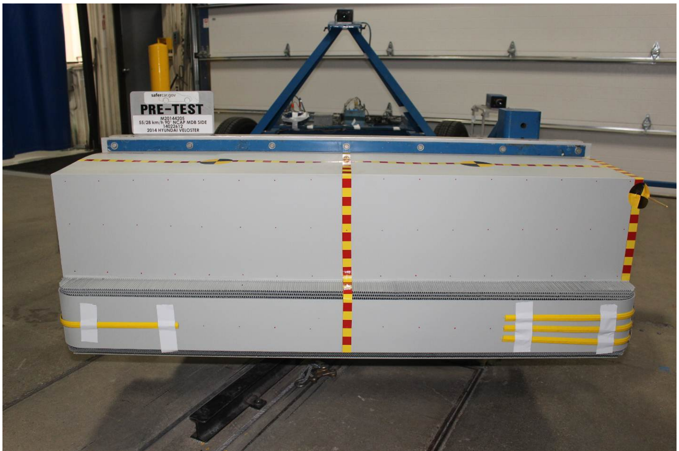
Pre-Test Front View of MDB Impactor Face
