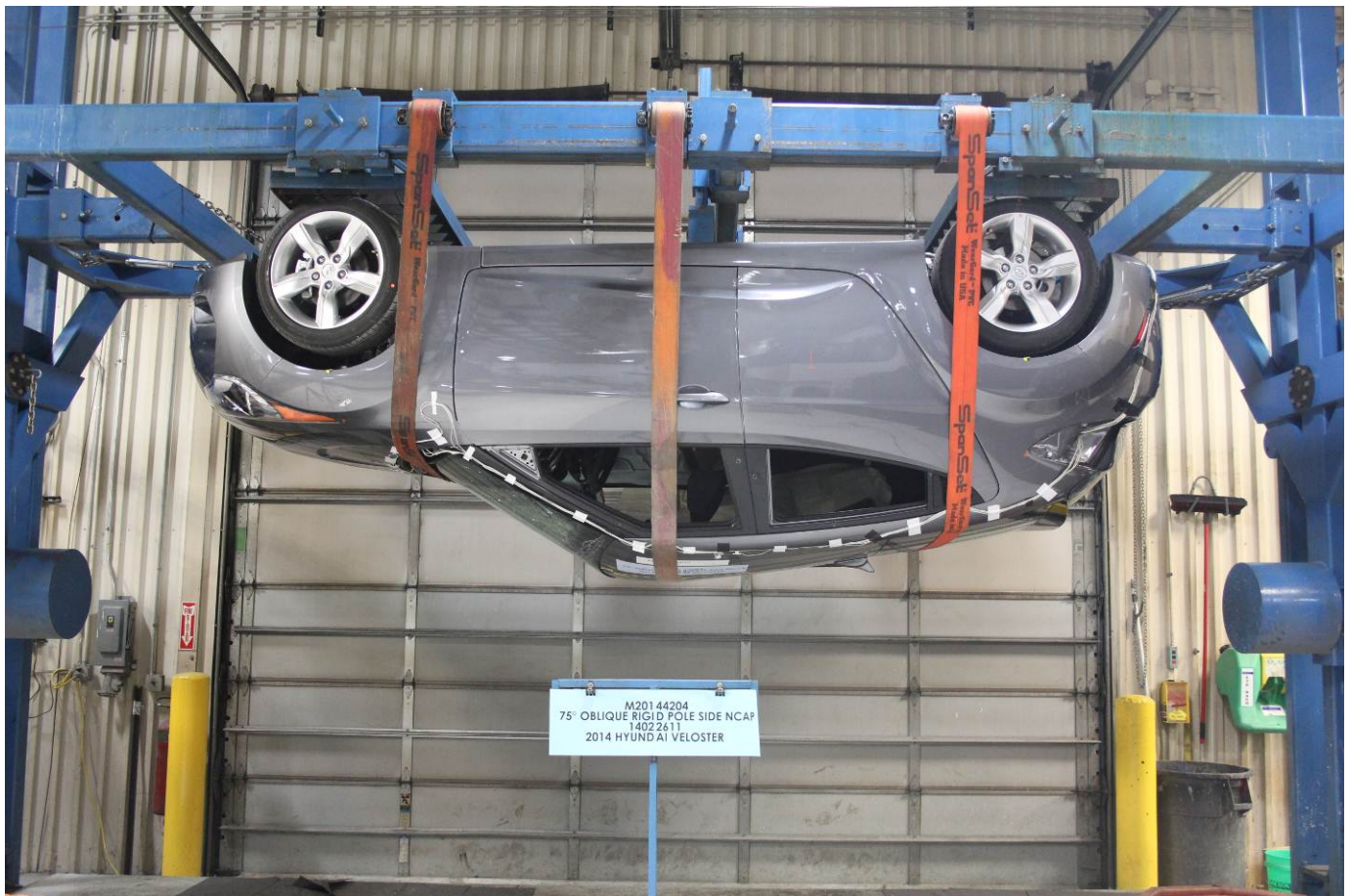
FMVSS No. 301 Static Rollover 180 Degrees
