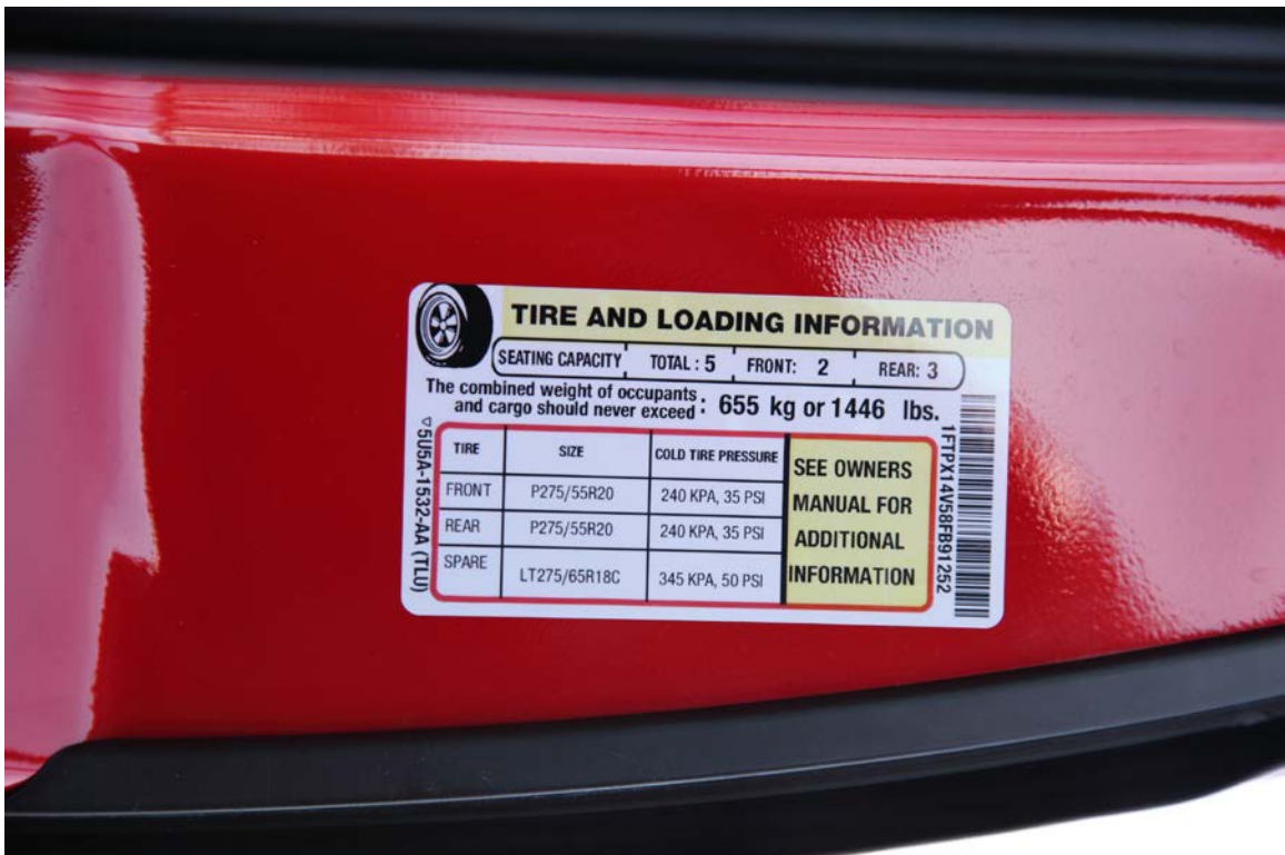
Figure A-51 Close-Up View of Bullet Vehicle Tire Information Placard or Label
