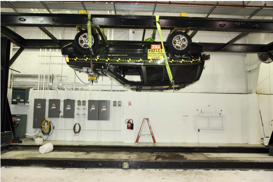
Figure A-60 Target Vehicle at 180° on Static Rollover Device
