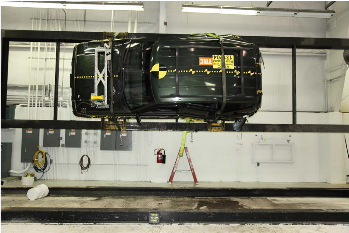
Figure A-59 Target Vehicle at 90° on Static Rollover Device
