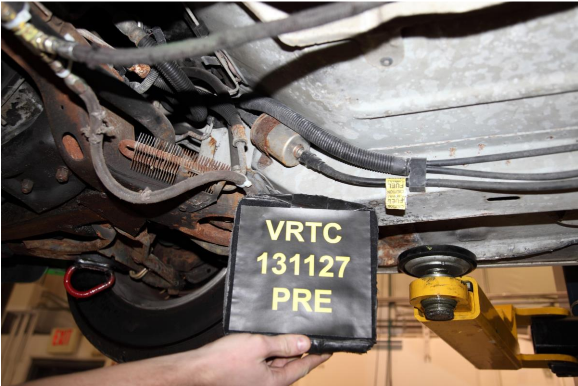
Figure A-46 Pre-Test Bullet Vehicle Fuel Line Close-up View
