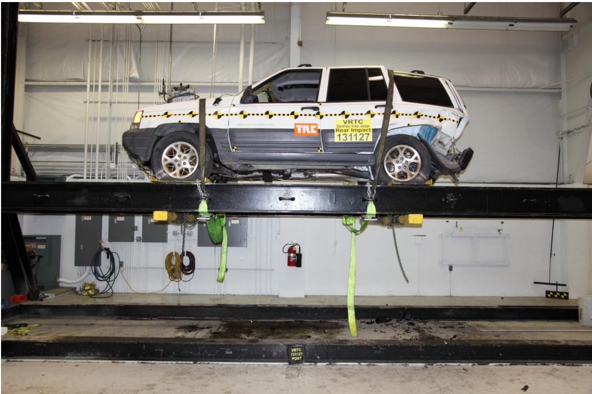
Figure A-62 Target Vehicle at 360° on Static Rollover Device
