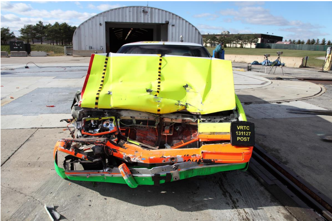
Figure A-29 Post-Test Bullet Vehicle Frontal View
