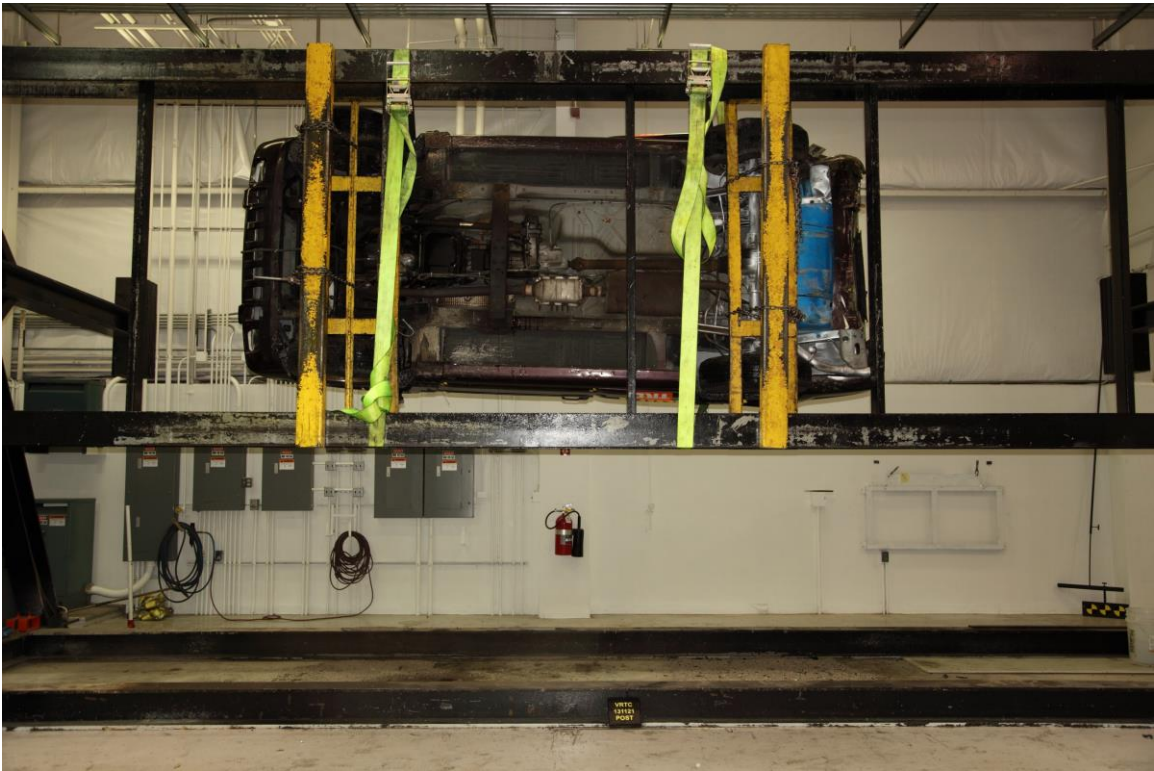
Figure A-61 Target Vehicle at 270° on Static Rollover Device
