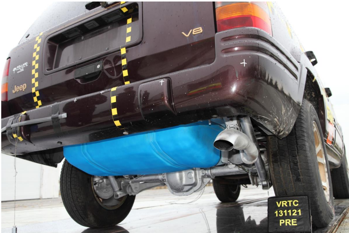
Figure A-19 Pre-Test Target Vehicle Fuel Tank Close-up View
