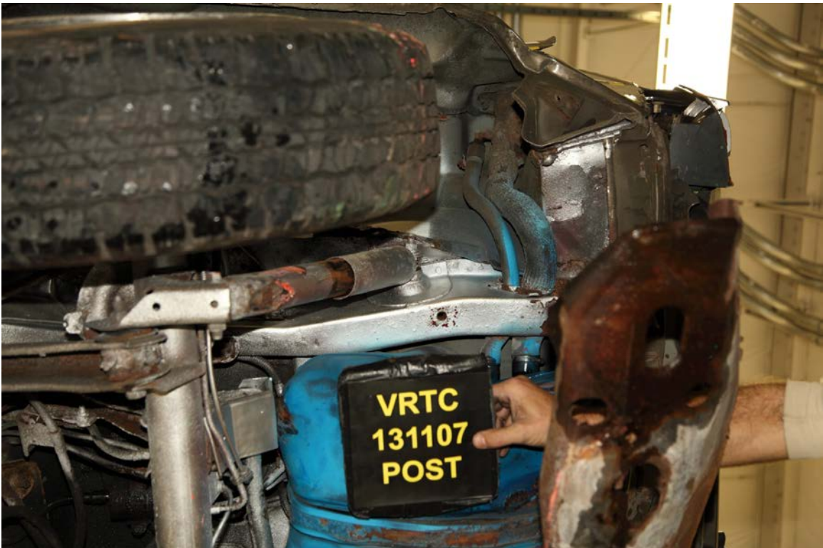
Figure A-24 Post-Test Target Vehicle Fuel Filler Close-up View
