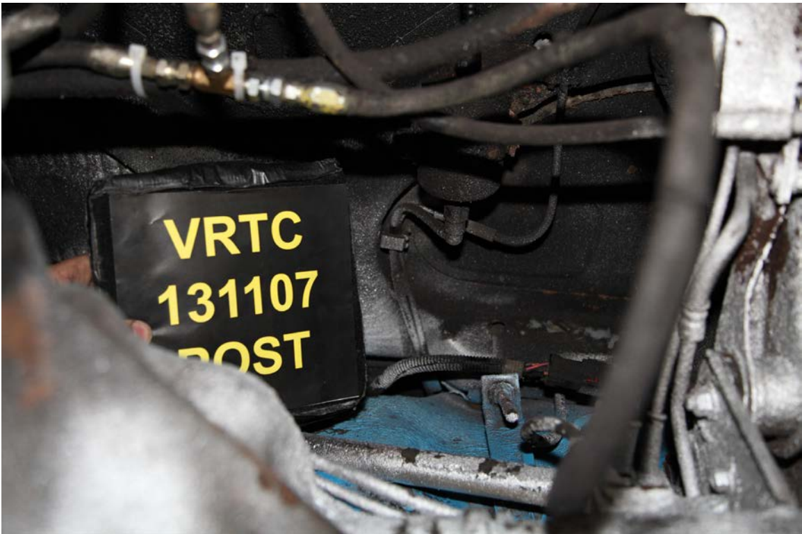
Figure A-22 Post-Test Target Vehicle Fuel Line Close-up View
