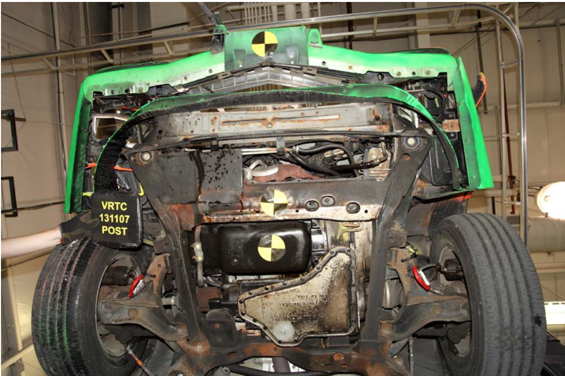
Figure A-41 Post-Test Bullet Vehicle Front Underbody View
