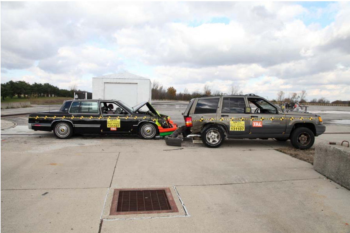
Figure A-55 Post-Test Bullet and Target Vehicles Overall Right Side View
