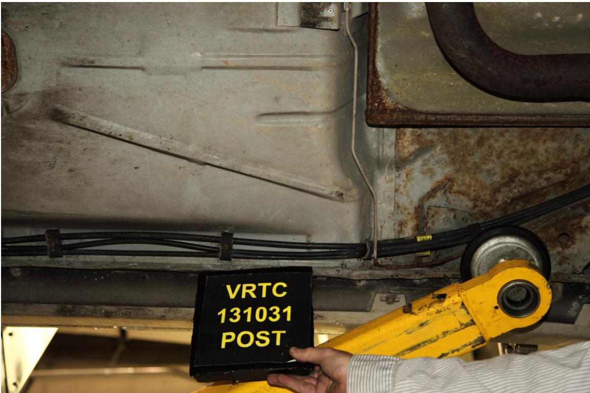
Figure A-48 Post-Test Bullet Vehicle Fuel Line Close-up View
