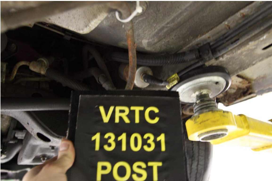
Figure A-50 Post-Test Bullet Vehicle Fuel Filter Close-up View
