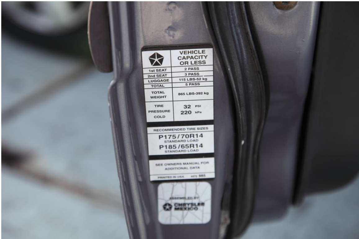
Figure A-55 Close-Up View of Bullet Vehicle Tire Information Placard or Label
