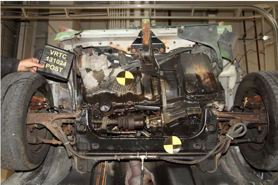
Figure A-45 Post-Test Bullet Vehicle Front Underbody View
