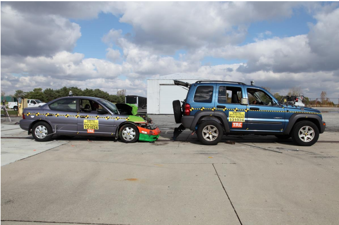
Figure A-59 Post-Test Bullet and Target Vehicles Overall Right Side View
