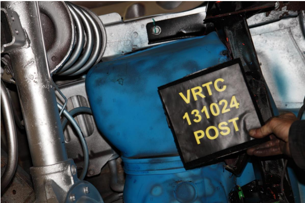
Figure A-26 Post-Test Target Vehicle Fuel Filter Close-up View
