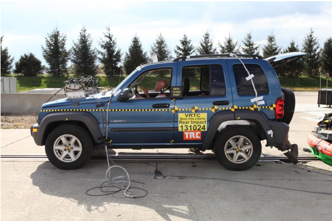
Figure A-6 Post-Test Target Vehicle Left Side View
