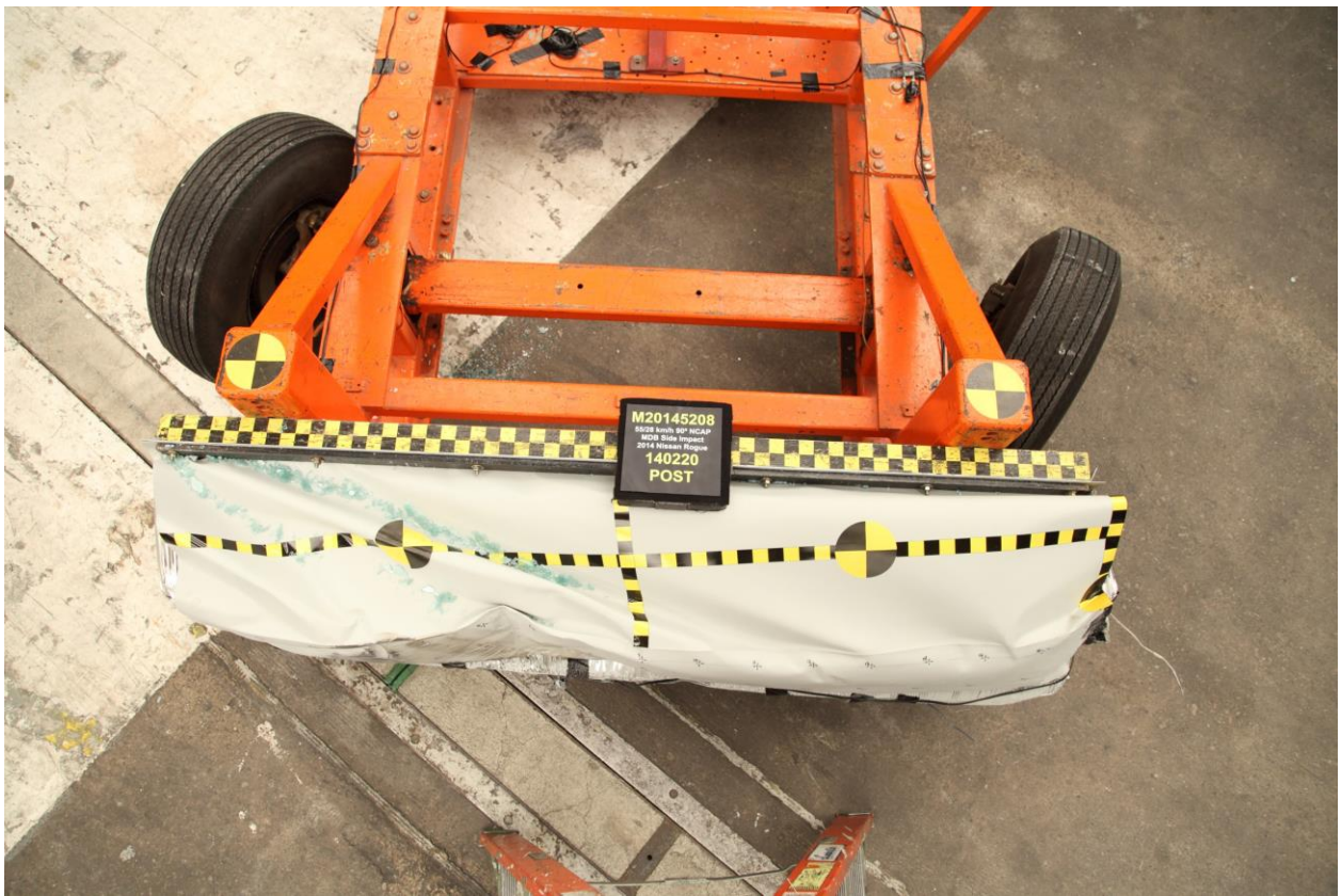
087 Post-Test Top View of MDB Impactor Face
