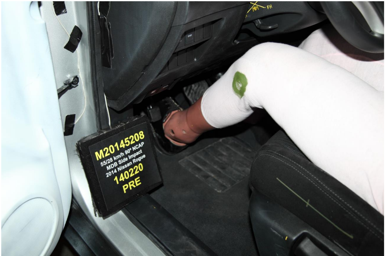
034 Pre-Test Placement of Driver Dummy Feet
