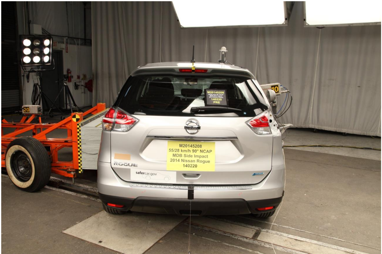
011 Pre-Test Rear View of Test Vehicle
