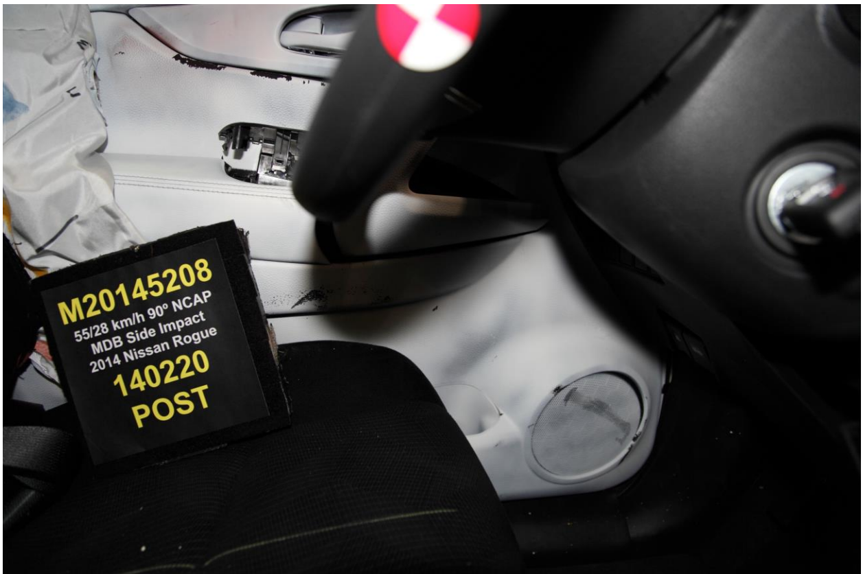
054 Post-Test Driver Dummy Close-Up Knee Contact View
