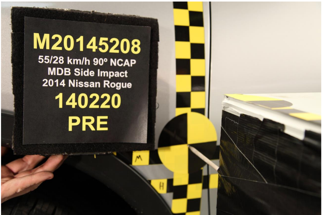
019 Pre-Test Close-up View of Impact Point Target
