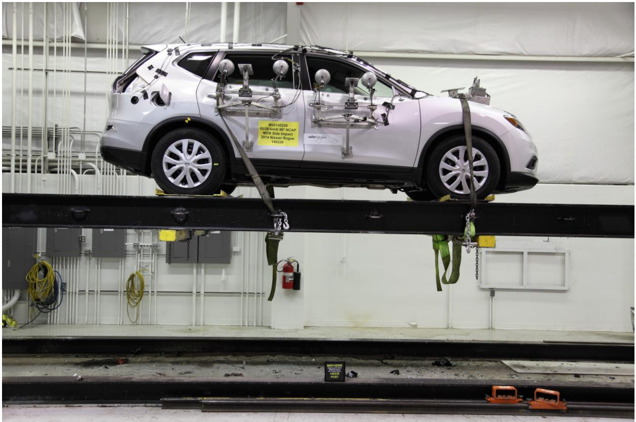
096 FMVSS No. 301 Static Rollover 0 Degrees
