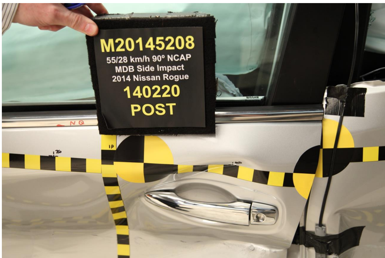
022 Post-Test Left Front Door Latch Close-up
