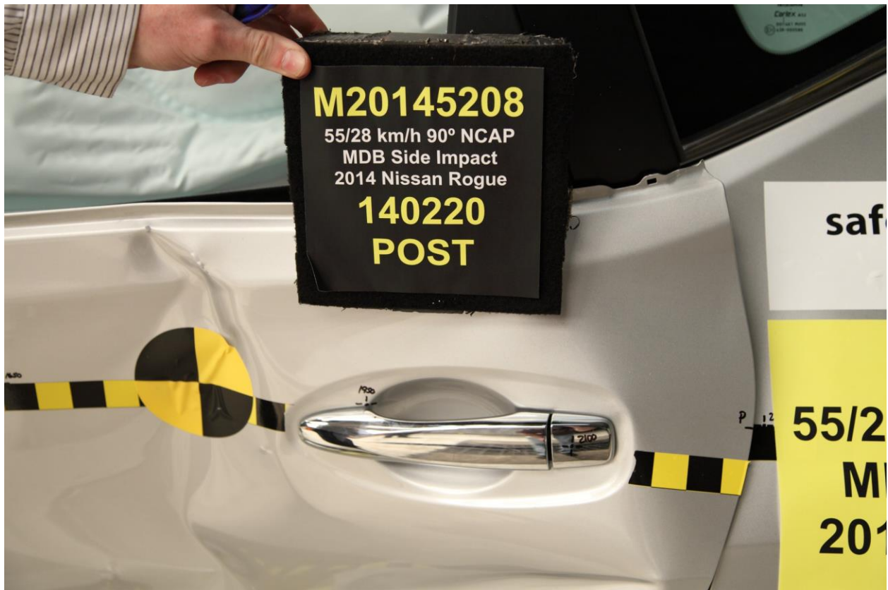
024 Post-Test Left Rear Door Latch Close-up
