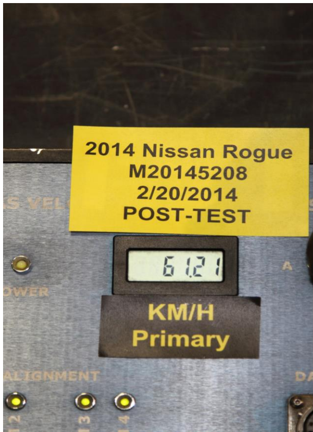
095 Post-Test Primary Speed Trap Read-Out
