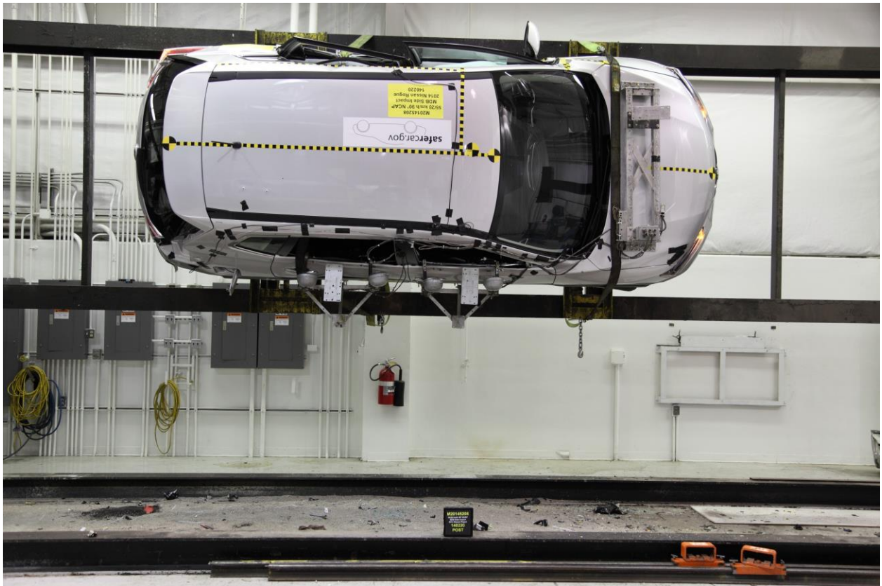
097 FMVSS No. 301 Static Rollover 90 Degrees
