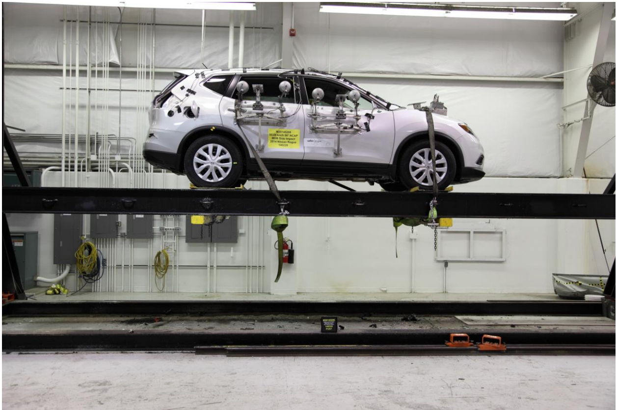
100 FMVSS No. 301 Static Rollover 360 Degrees
