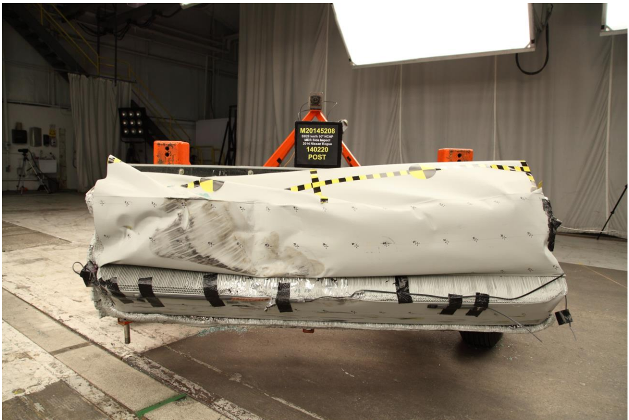
085 Post-Test Front View of MDB Impactor Face
