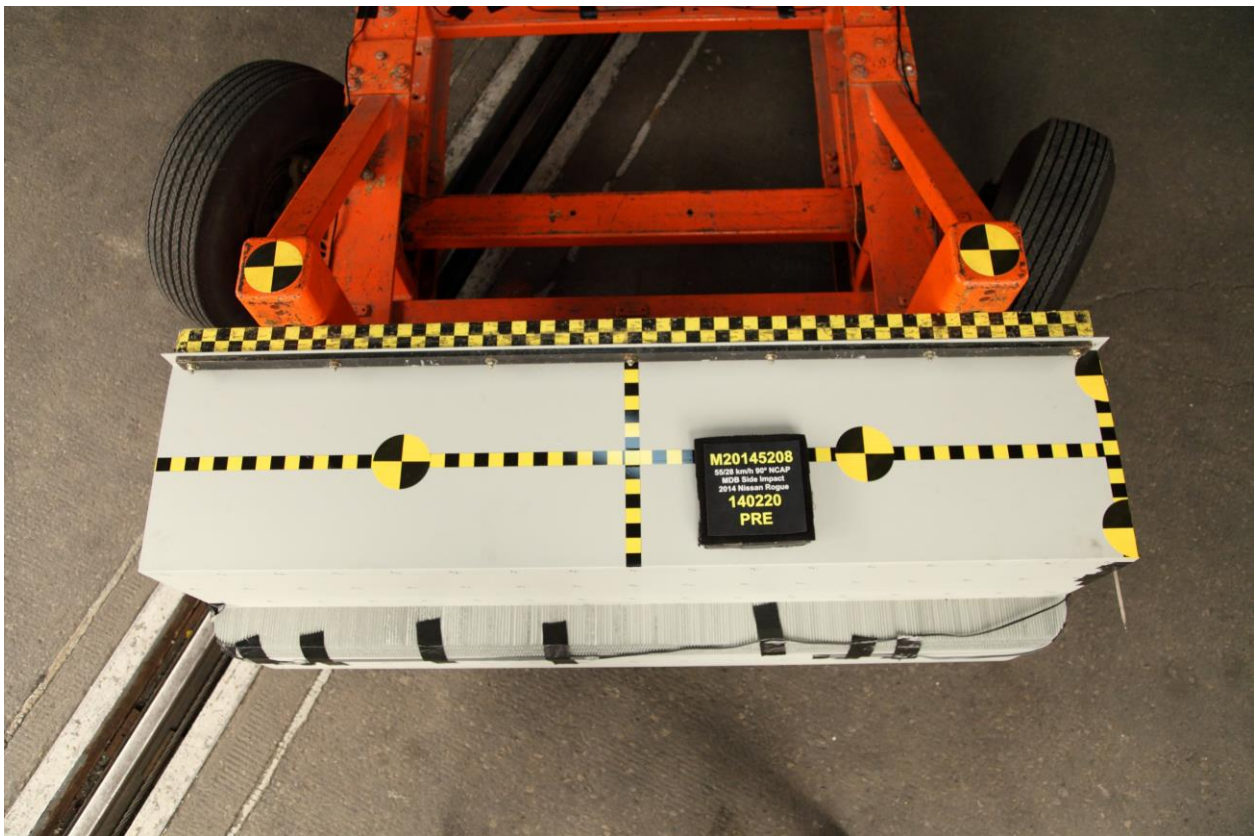
086 Pre-Test Top View of MDB Impactor Face
