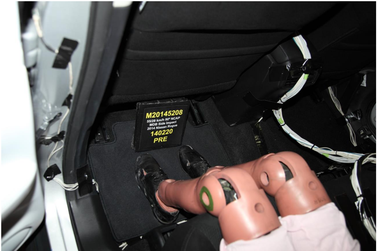
064 Pre-Test Placement of Rear Passenger Dummy Feet
