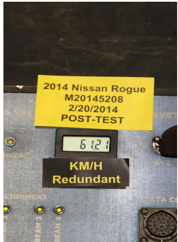
095 Post-Test Primary Speed Trap Read-Out
