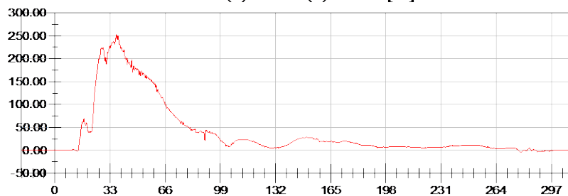
Driver Posterior Abdominal Force (Y) vs. Time (N) vs. Time [ms]
