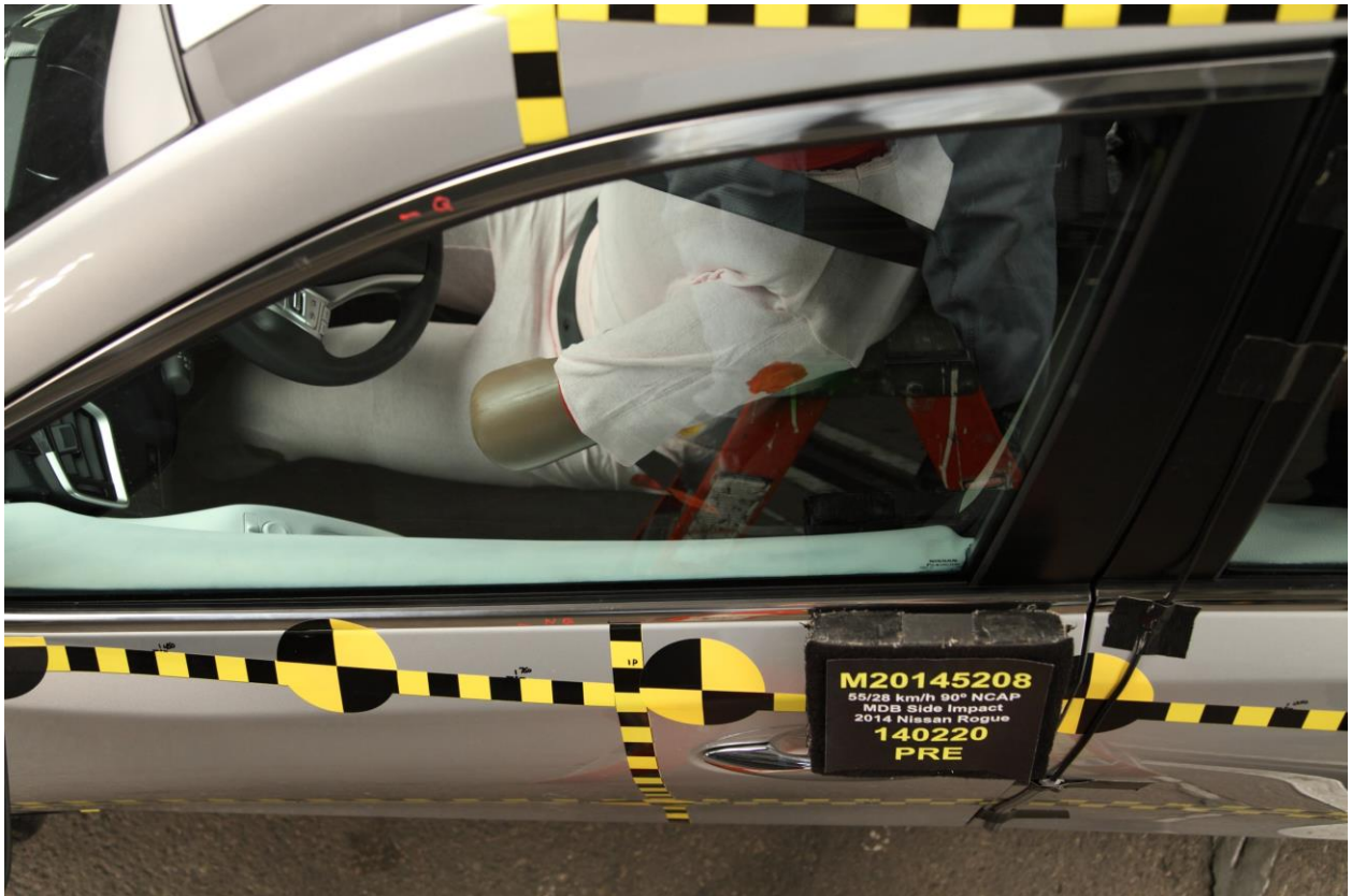
042 Pre-Test Driver Dummy and Door Clearance View
