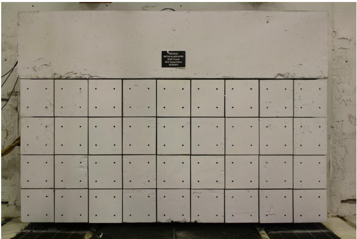
Figure A-2: Load Cell Wall
