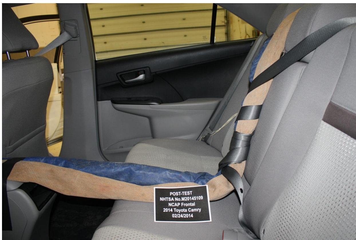
Figure A-28: Post-Test Dummy Cable Routing
