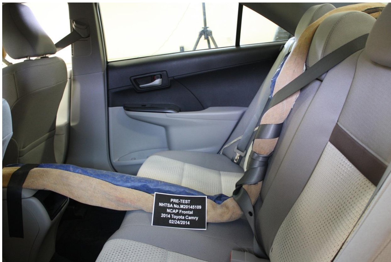
Figure A-27: Pre-Test Dummy Cable Routing
