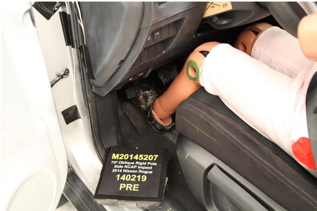
032 Pre-Test Placement of Dummy Feet
