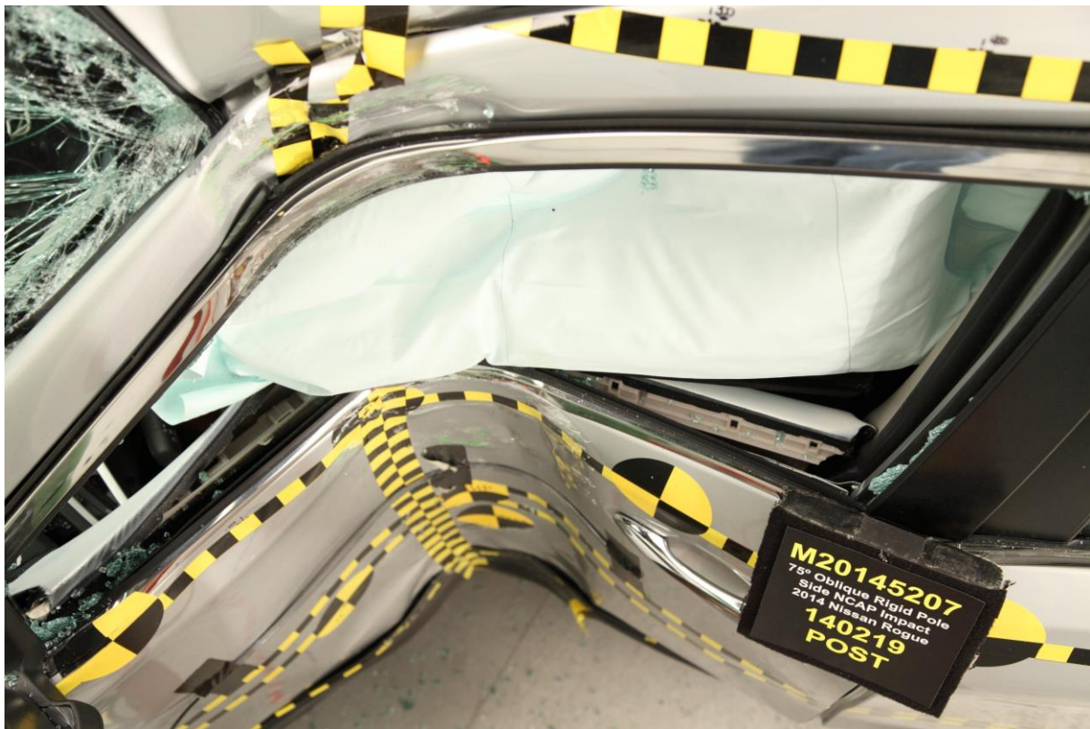
041 Post-Test Dummy and Door Clearance View
