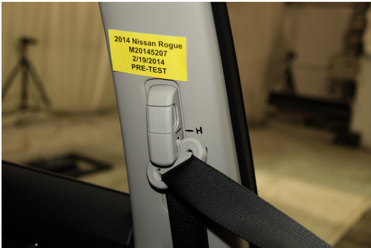
033 Pre-Test View of Belt Anchorage for Dummy
