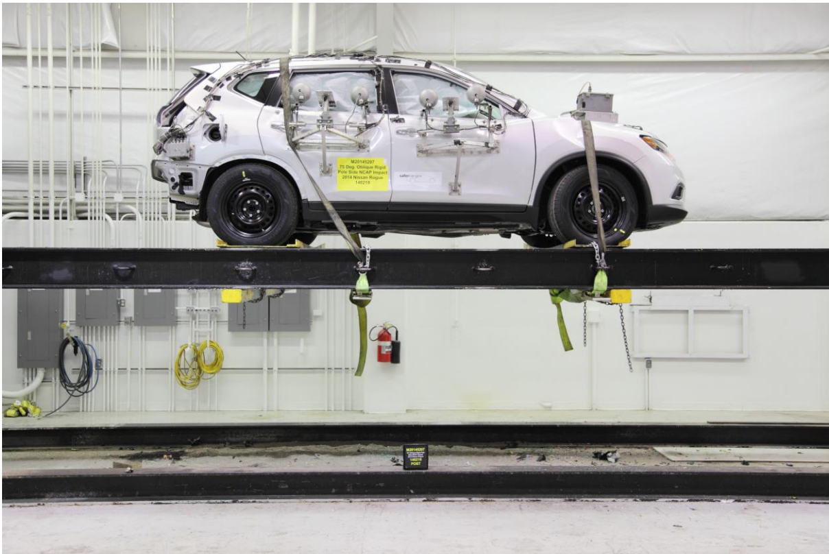
067 FMVSS No. 301 Static Rollover 360 Degrees
