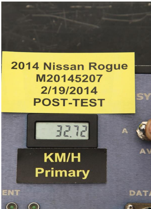
062 Post-Test Primary and Redundant Speed Trap Read-Out
