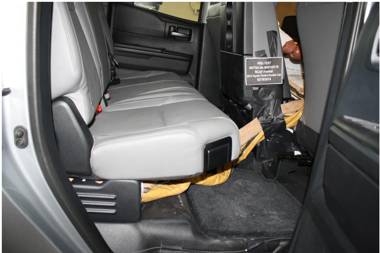
Figure A-27: Pre-Test Dummy Cable Routing
