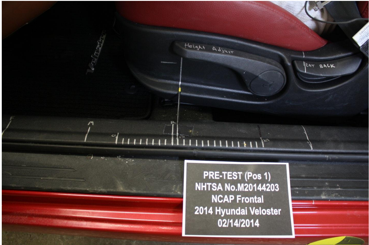
Figure A-35: Pre-Test Driver's Seat Fore-Aft Markings
