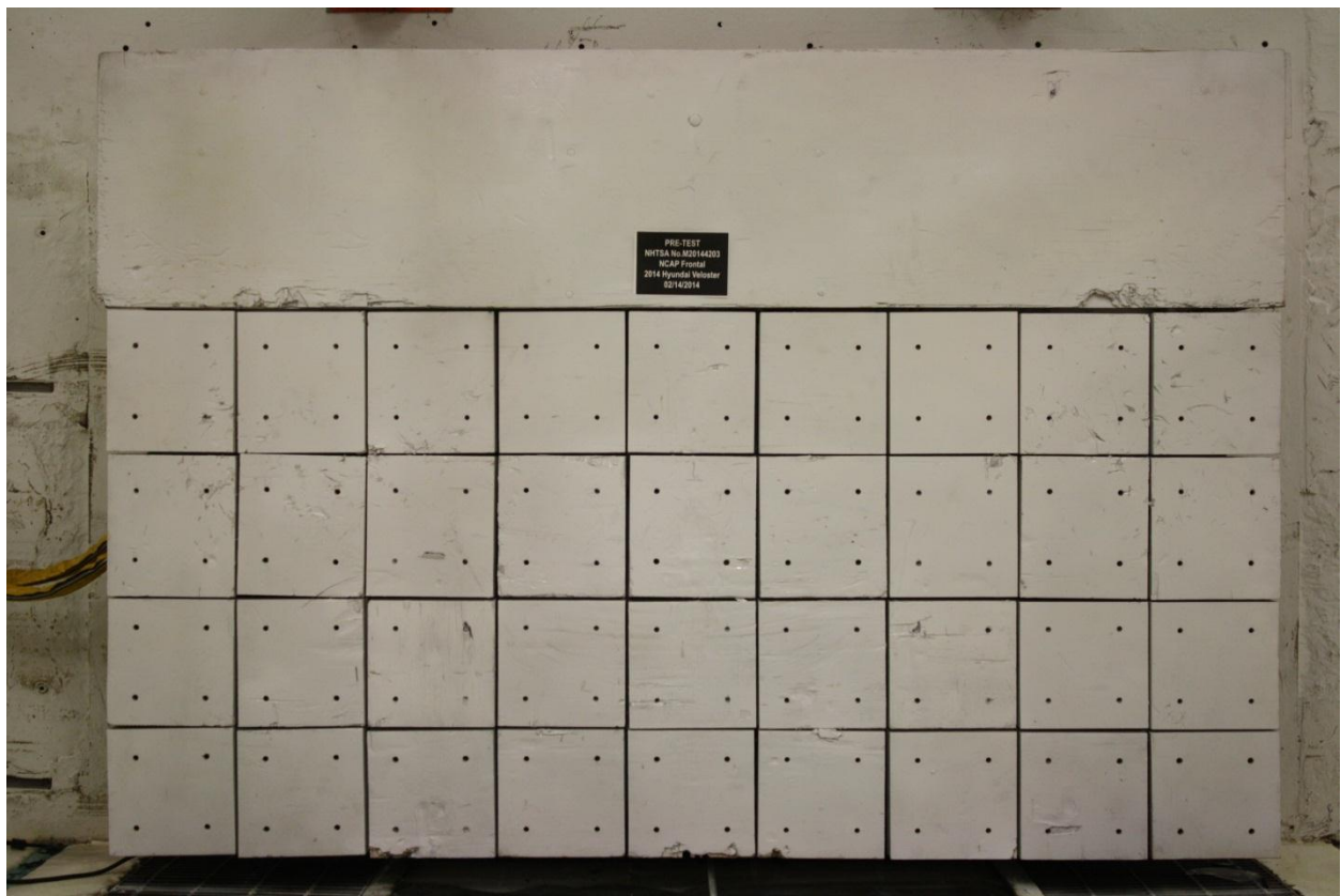
Figure A-2: Load Cell Wall
