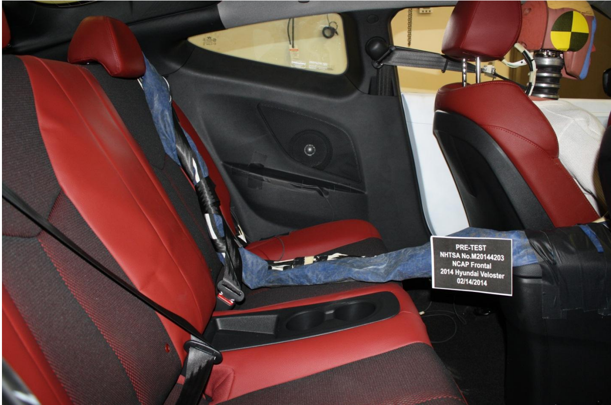
Figure A-27: Pre-Test Dummy Cable Routing
