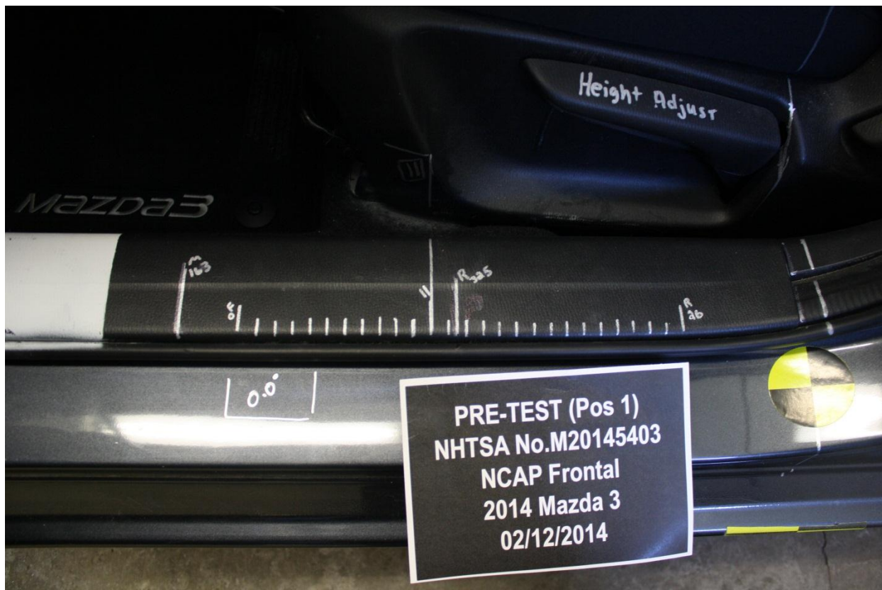
Figure A-35: Pre-Test Driver's Seat Fore-Aft Markings
