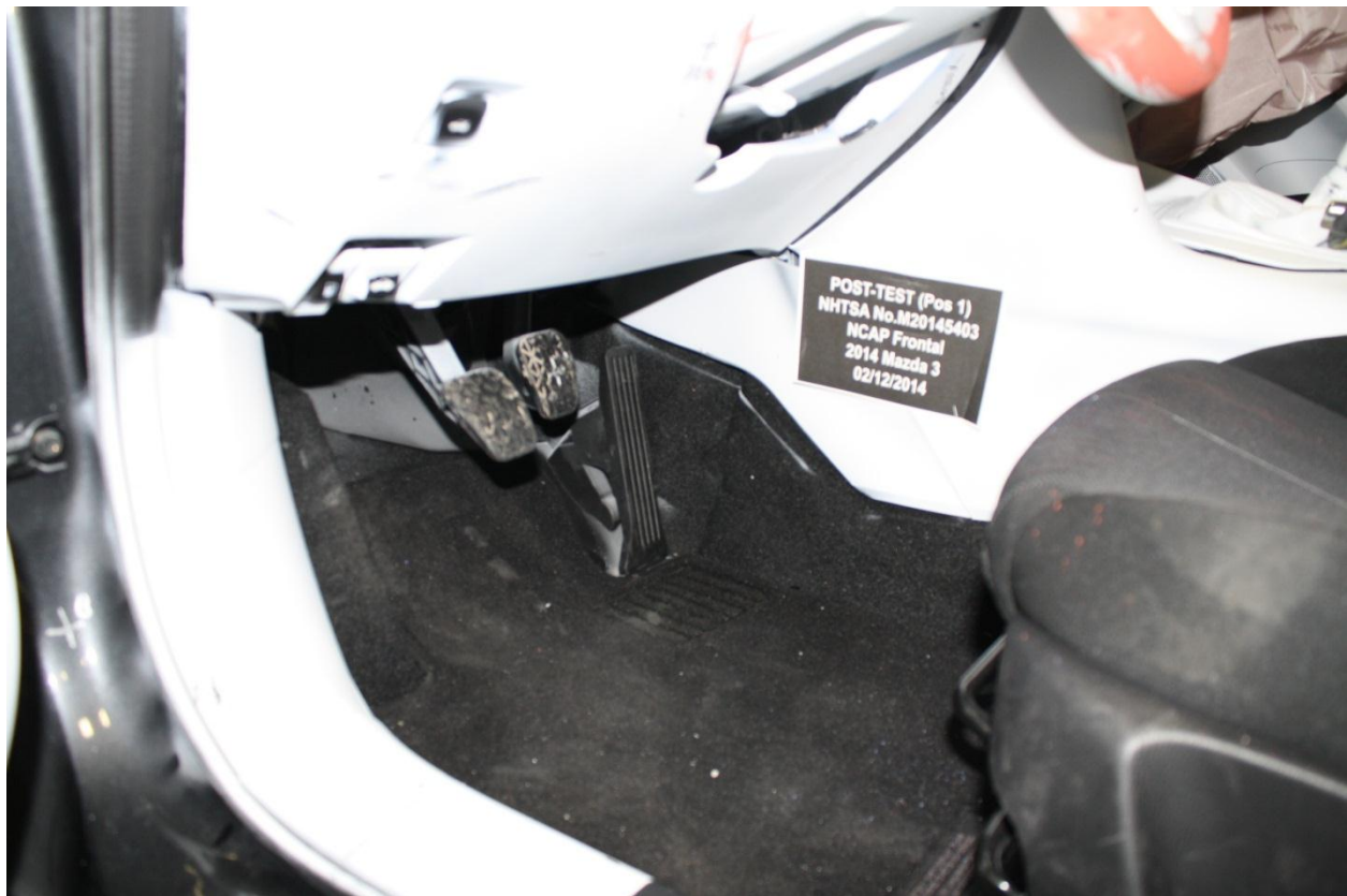
Figure A-44: Post-Test Driver's Side Floorpan
