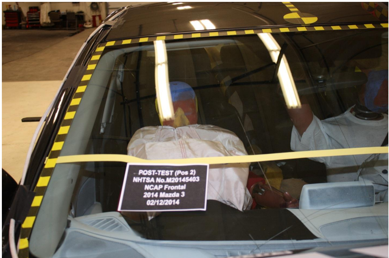
Figure A-51: Post-Test Passenger Dummy Front View
