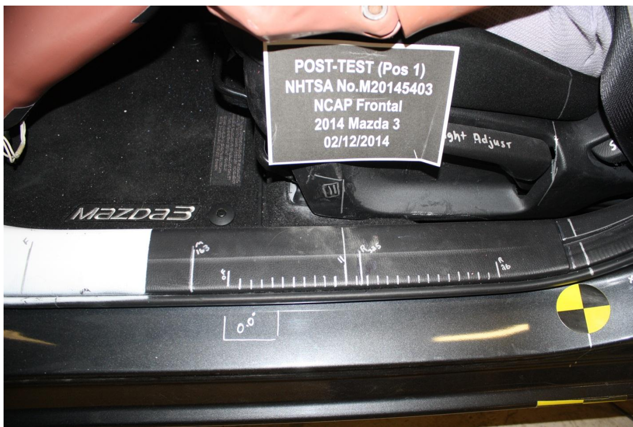
Figure A-36: Post-Test Driver's Seat Fore-Aft Markings
