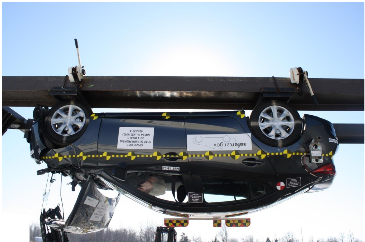
Figure A-74: Vehicle at 180° on Static Rollover Device
