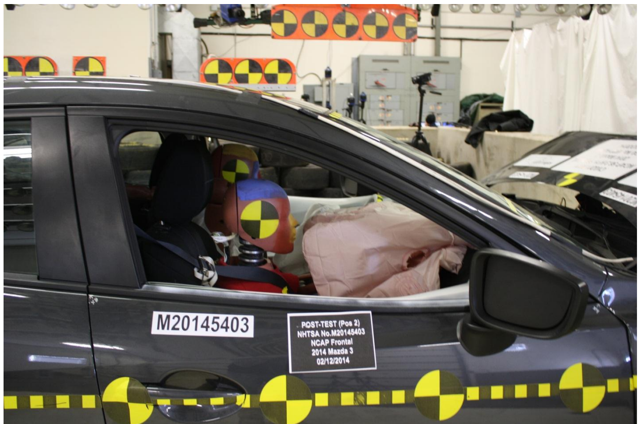
Figure A-53: Post-Test Passenger Dummy Window View
