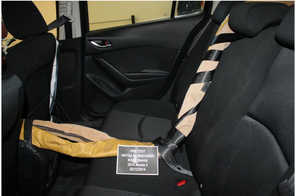
Figure A-27: Pre-Test Dummy Cable Routing
