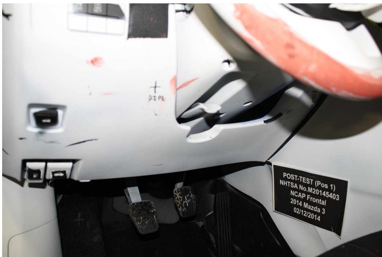
Figure A-42: Post-Test Driver's Side Knee Bolster
