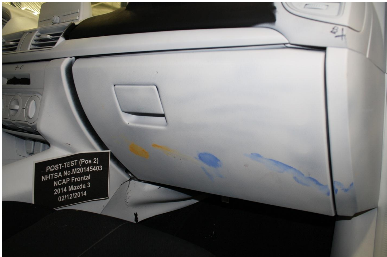
Figure A-63: Post-Test Passenger's Side Knee Bolster
