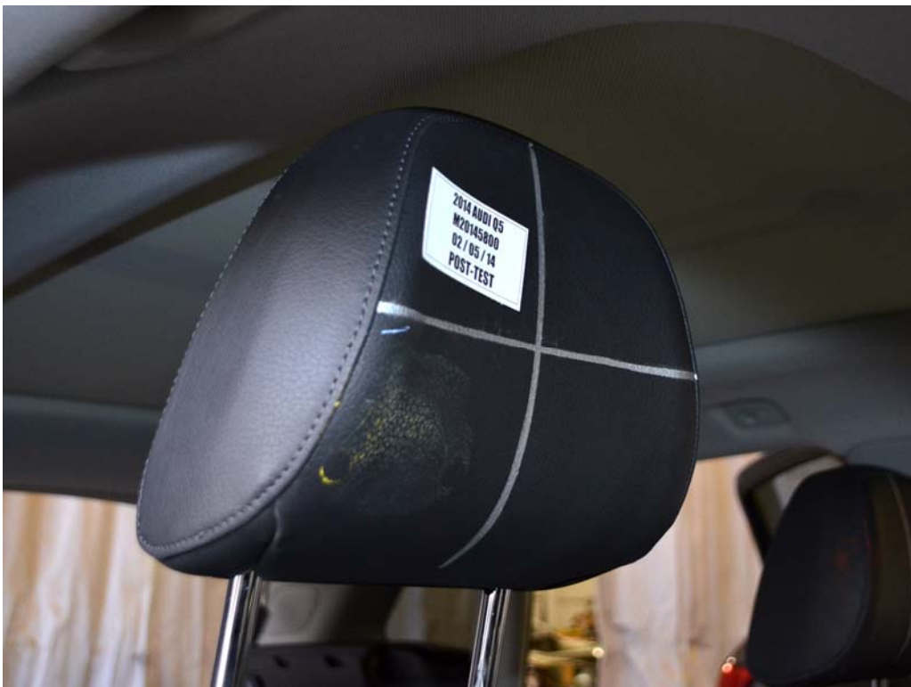
FIGURE 68. Post-Test Passenger Dummy Contact with Headrest
