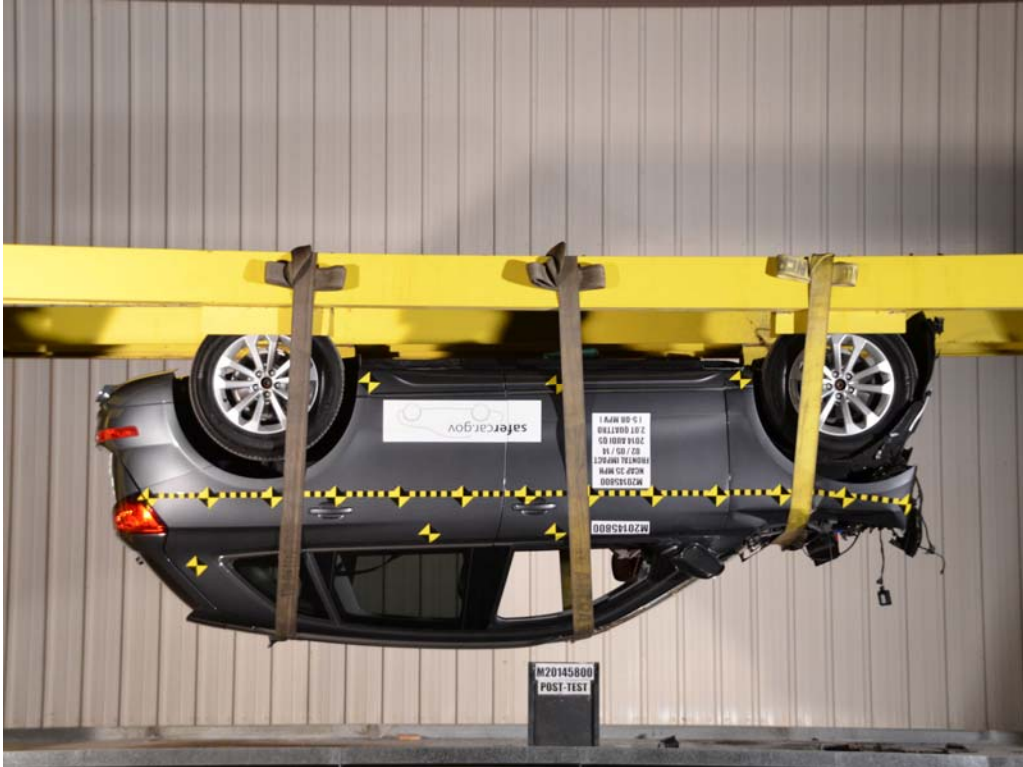
FIGURE 74. Vehicle at 180° on Static Rollover Device
