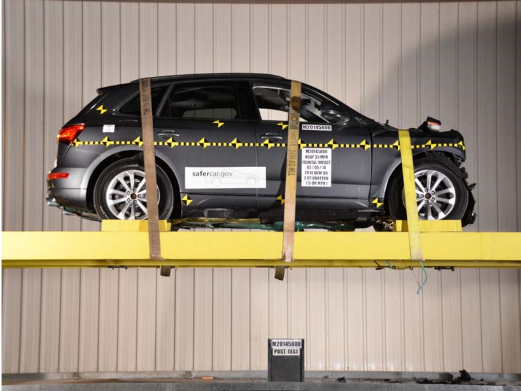
FIGURE 76. Vehicle at 360° on Static Rollover Device
