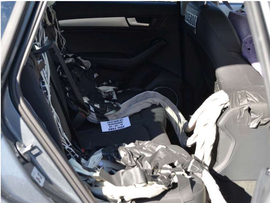
FIGURE 28. Post-Test Dummy Cable Routing
