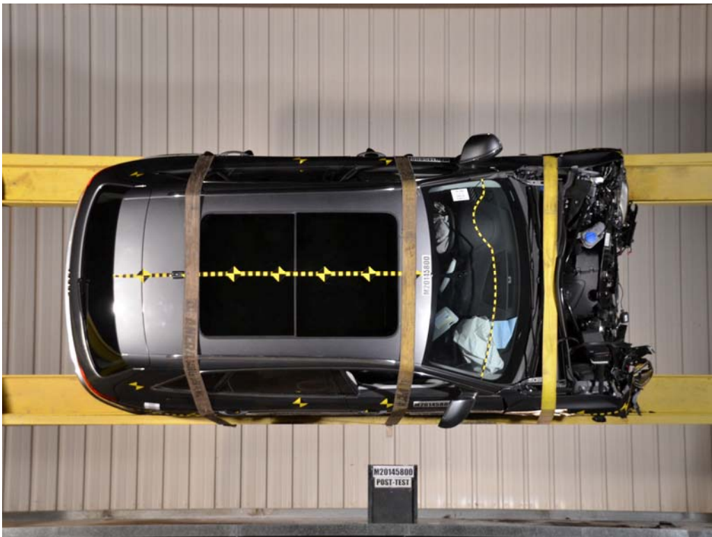
FIGURE 73. Vehicle at 90° on Static Rollover Device
