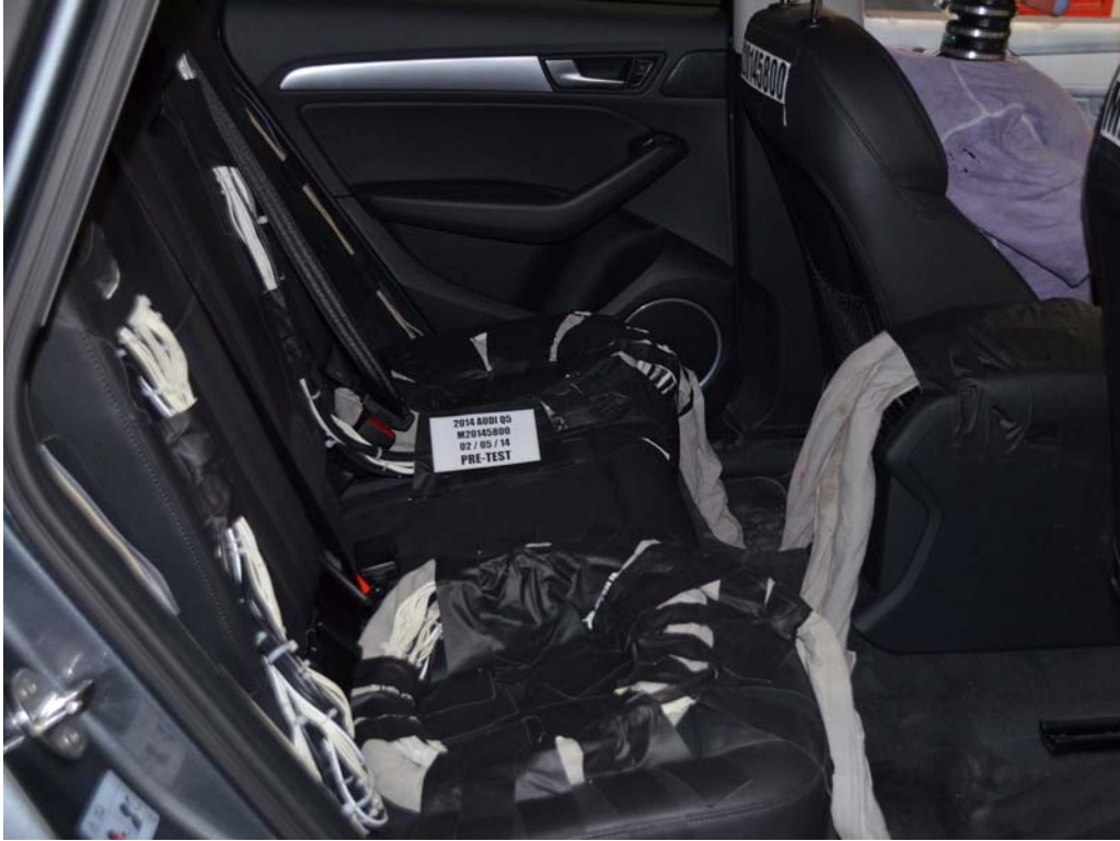
FIGURE 27. Pre-Test Dummy Cable Routing
