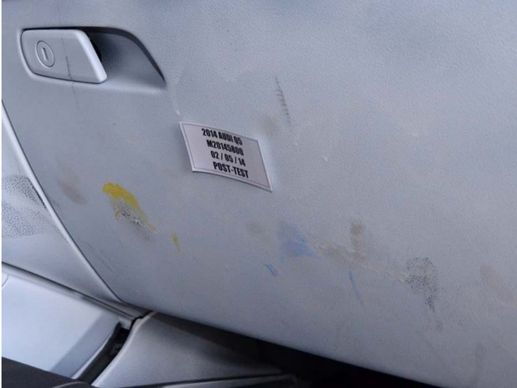
FIGURE 68a. Post-Test Passenger Dummy Contact with Glovebox
