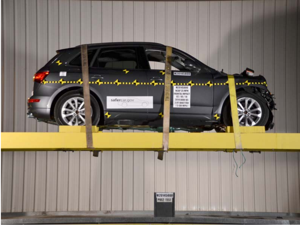
FIGURE 72. Vehicle at 0° on Static Rollover Device
