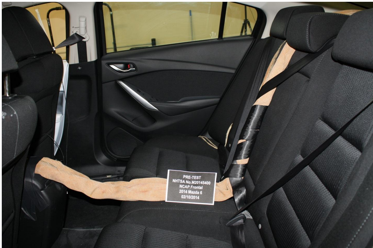
Figure A-27: Pre-Test Dummy Cable Routing
