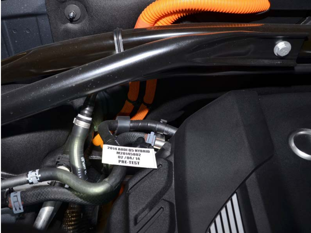
FIGURE 18c. Pre-Impact View of High Voltage Interconnect(s)
