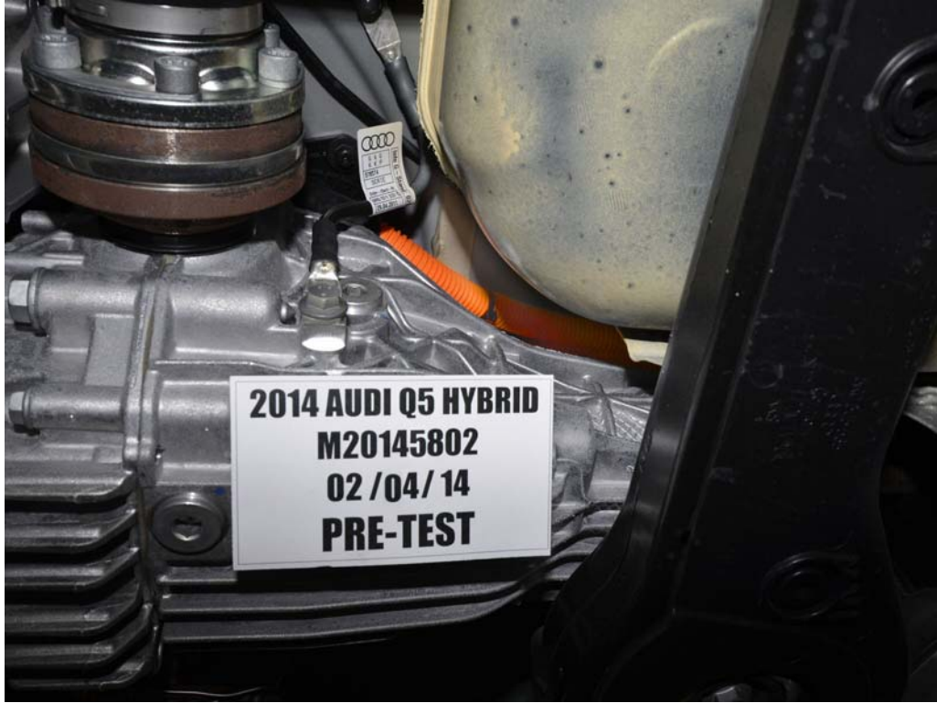
FIGURE 18a. Pre-Impact View of High Voltage Interconnect(s)
