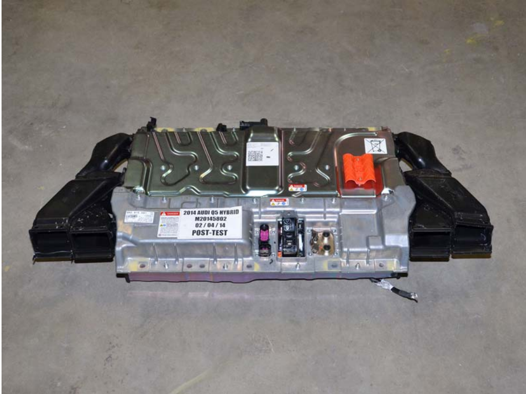
FIGURE 13b. Post-Impact View of Battery Box(s) or Container(s) Which Holds Individual Battery Modules
