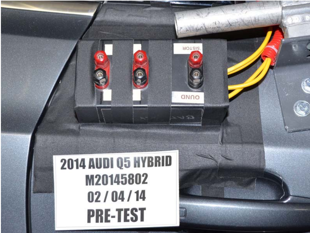
FIGURE 24. Pre-Impact View of Installed Test Interface Port
