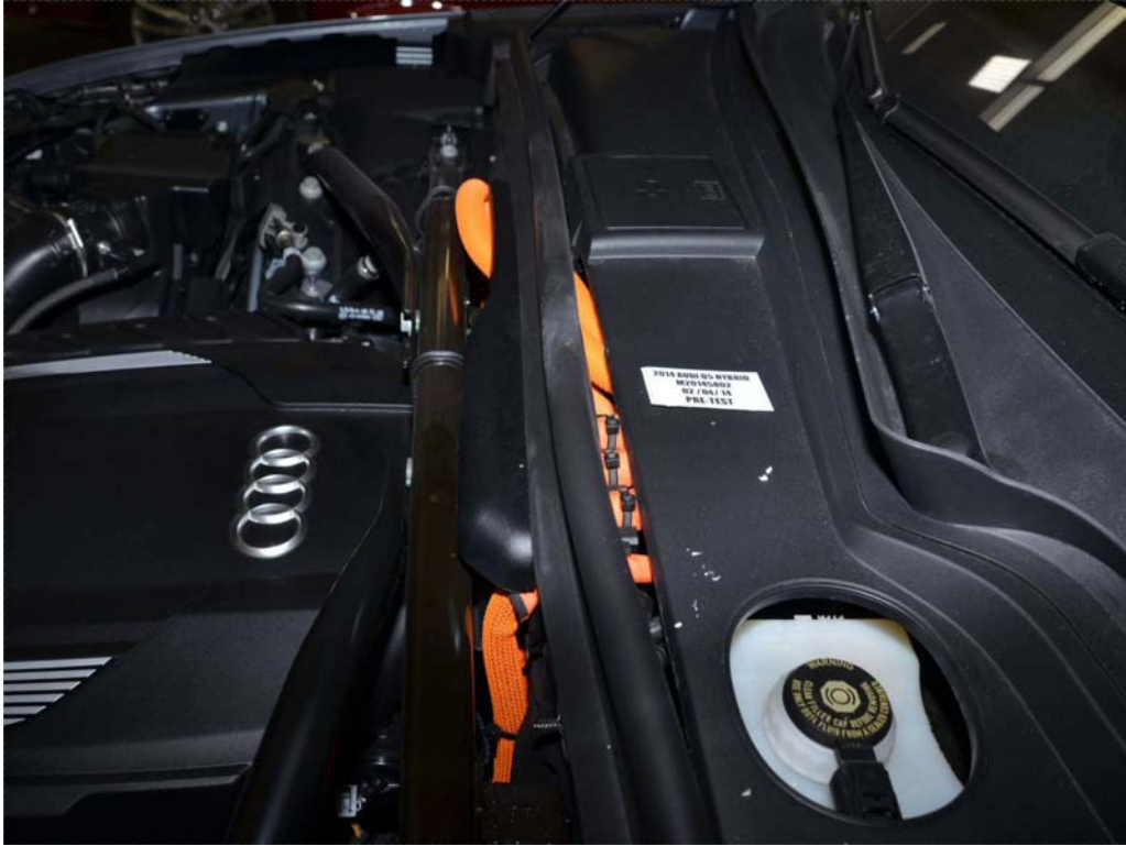
FIGURE 18e. Pre-Impact View of High Voltage Interconnect(s)
