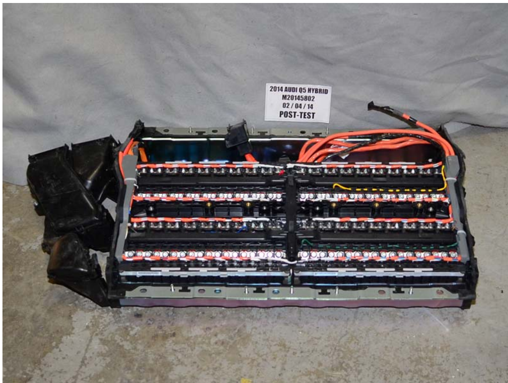
FIGURE 15. Post-Impact View of Propulsion Battery Module(s)
