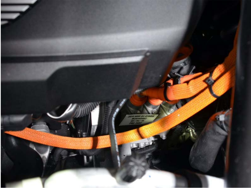
FIGURE 18g. Pre-Impact View of High Voltage Interconnect(s)
