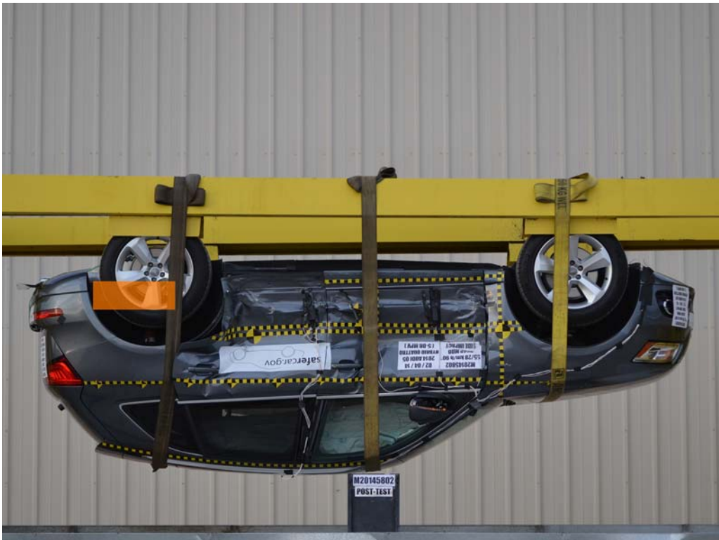
FIGURE 30. FMVSS No. 305 Static Rollover at 180°
