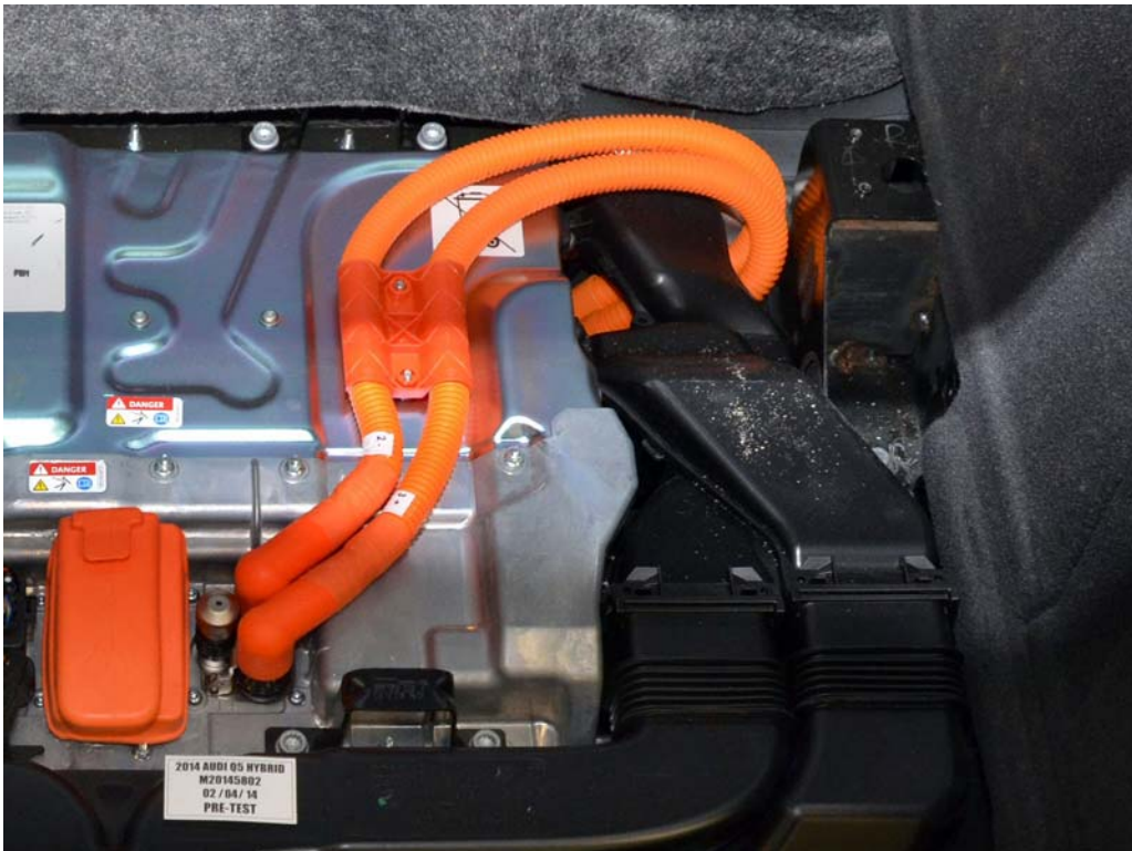
FIGURE 18. Pre-Impact View of High Voltage Interconnect(s)
