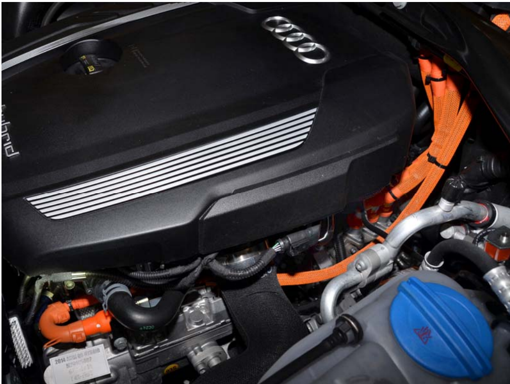
FIGURE 18f. Pre-Impact View of High Voltage Interconnect(s)
