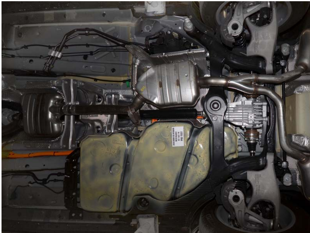
FIGURE 18b. Pre-Impact View of High Voltage Interconnect(s)
