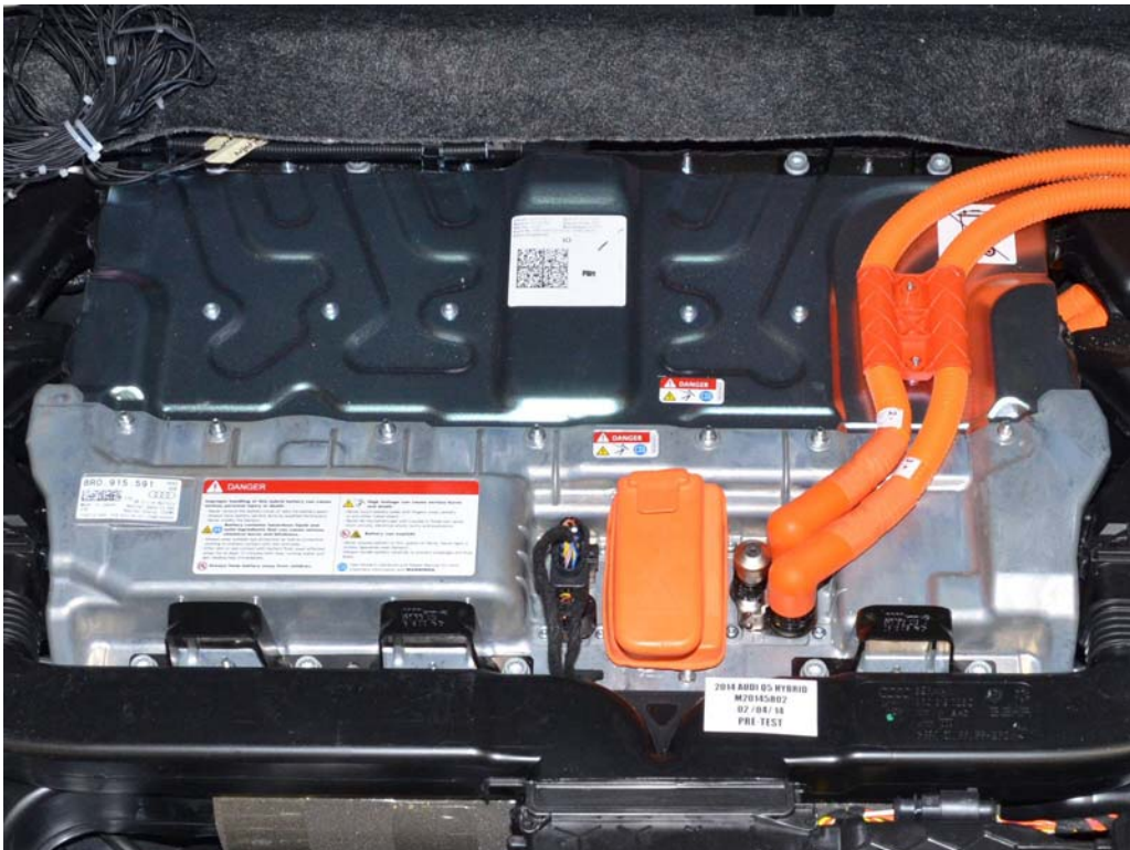
FIGURE 12. Pre-Impact View of Battery Box(s) or Container(s) Which Holds Individual Battery Modules
