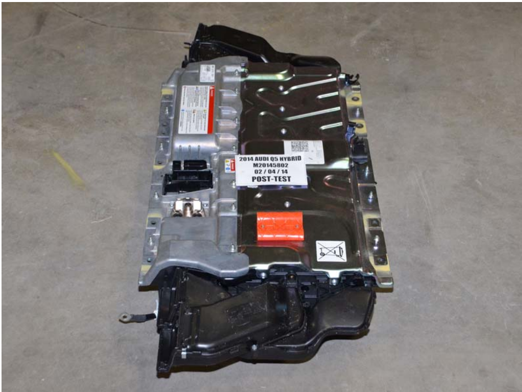
FIGURE 13a. Post-Impact View of Battery Box(s) or Container(s) Which Holds Individual Battery Modules
