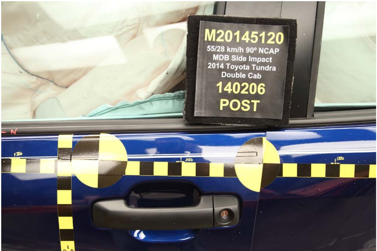
022 Post-Test Left Front Door Latch Close-up
