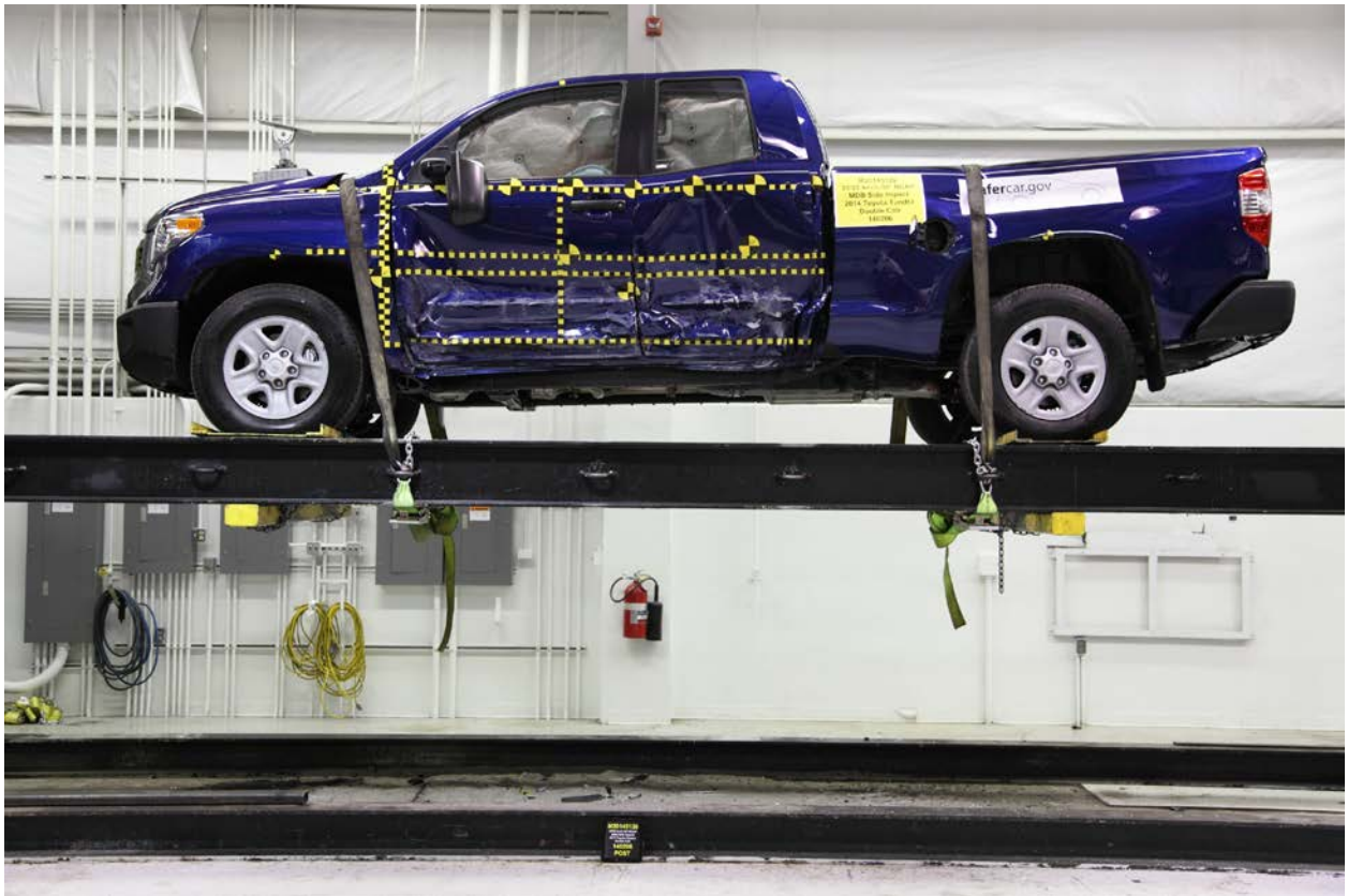
100 FMVSS No. 301 Static Rollover 360 Degrees
