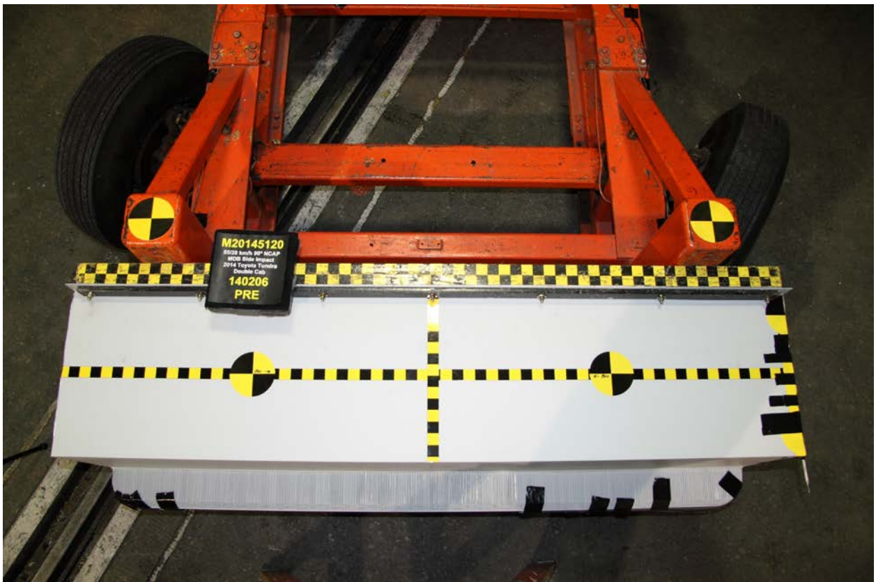
086 Pre-Test Top View of MDB Impactor Face
