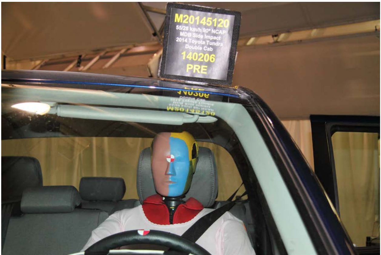
025 Pre-Test Front Close-up View of Driver Dummy
