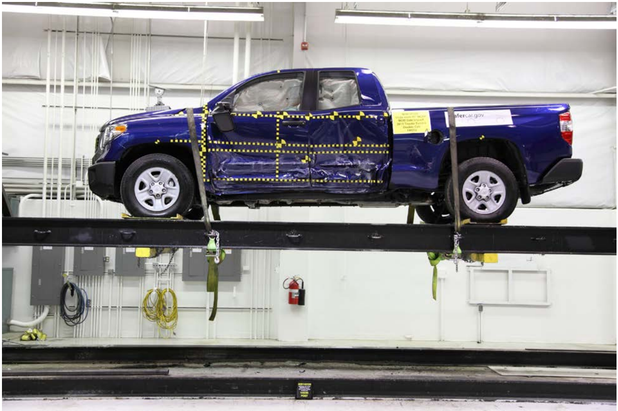
096 FMVSS No. 301 Static Rollover 0 Degrees
