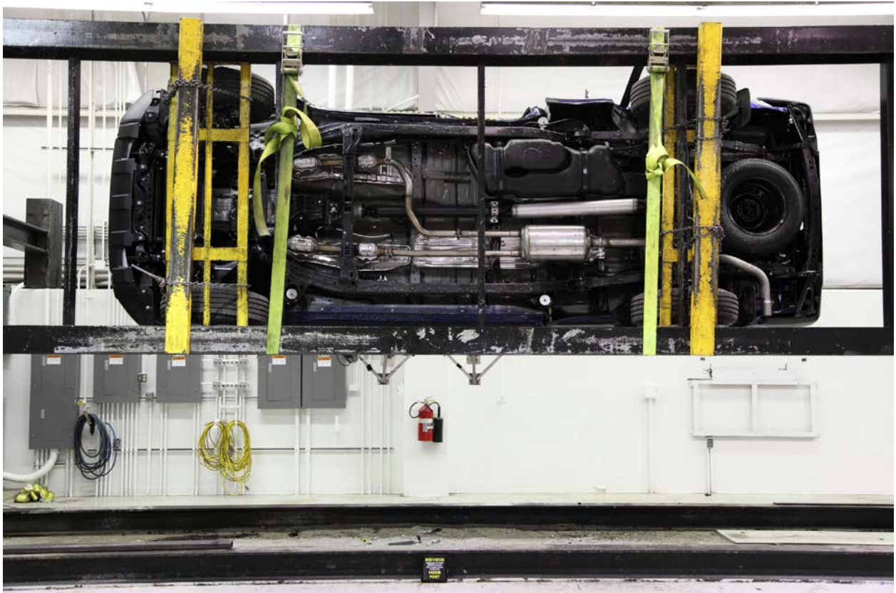
099 FMVSS No. 301 Static Rollover 270 Degrees
