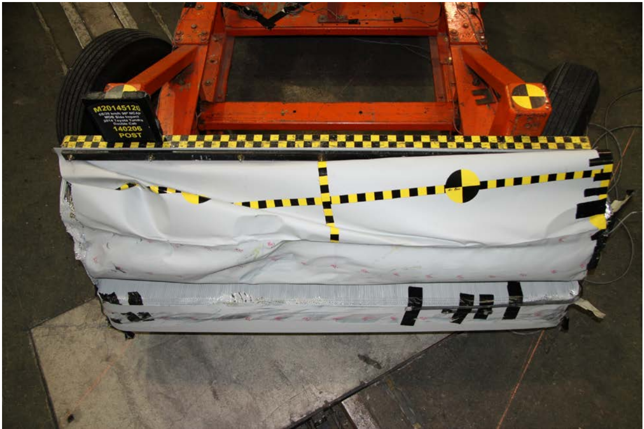
087 Post-Test Top View of MDB Impactor Face
