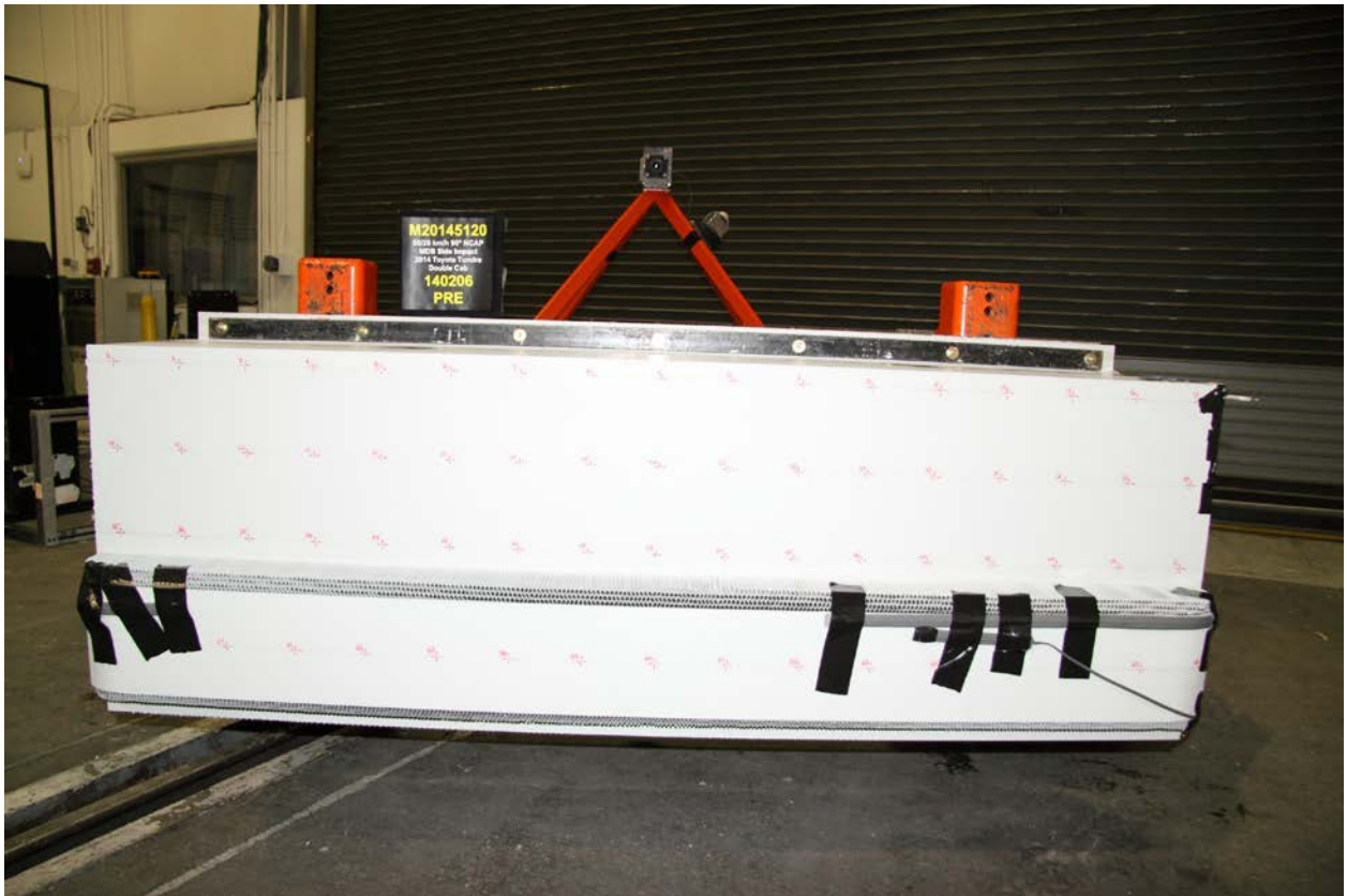
084 Pre-Test Front View of MDB Impactor Face
