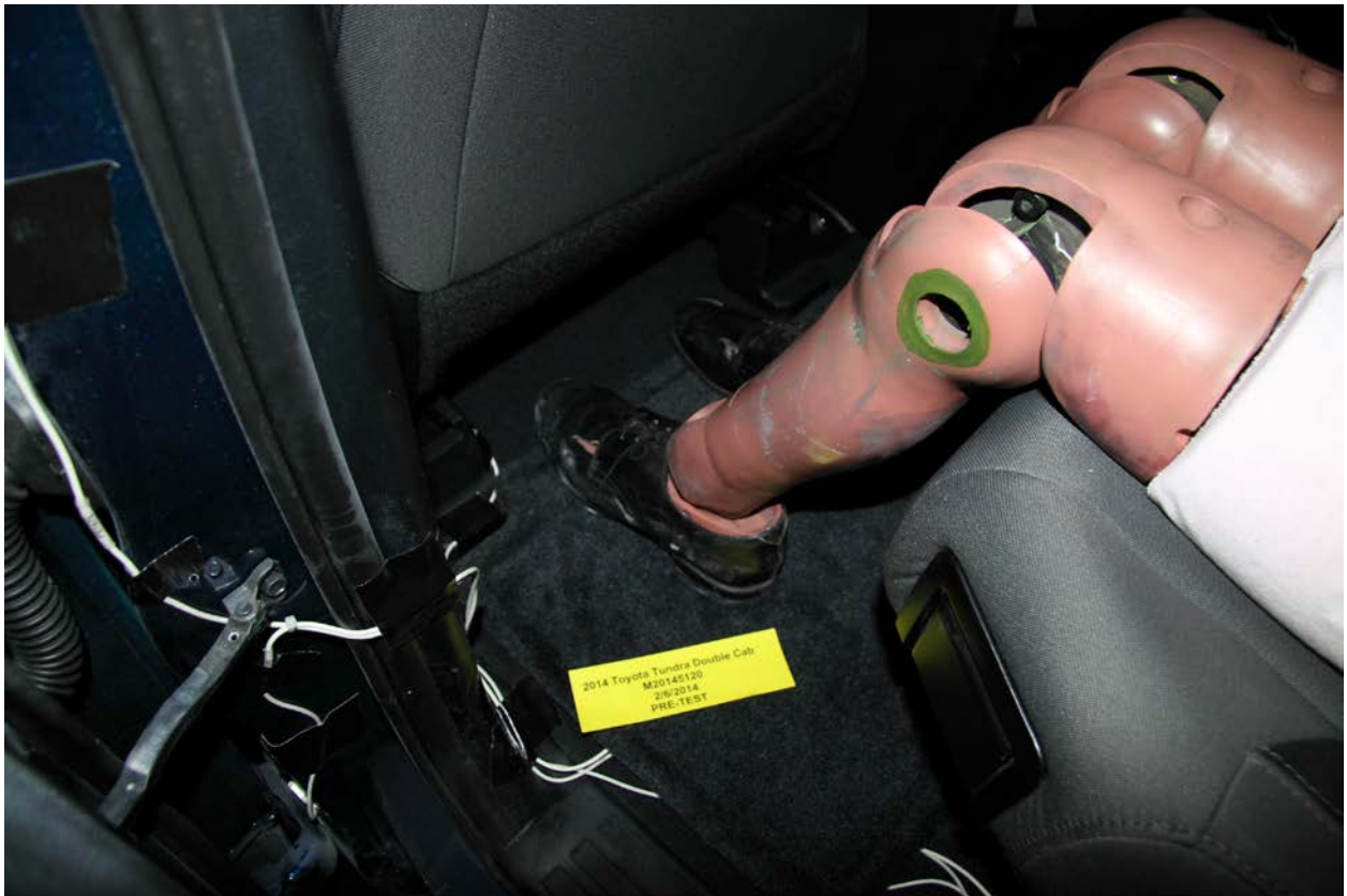
064 Pre-Test Placement of Rear Passenger Dummy Feet
