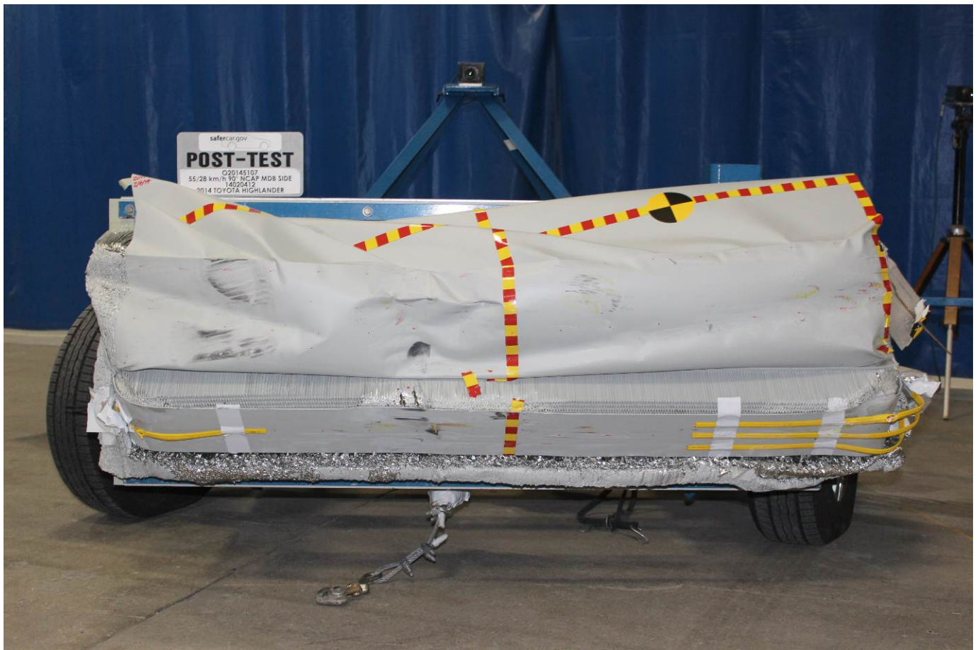
Post-Test Front View of MDB Impactor Face
