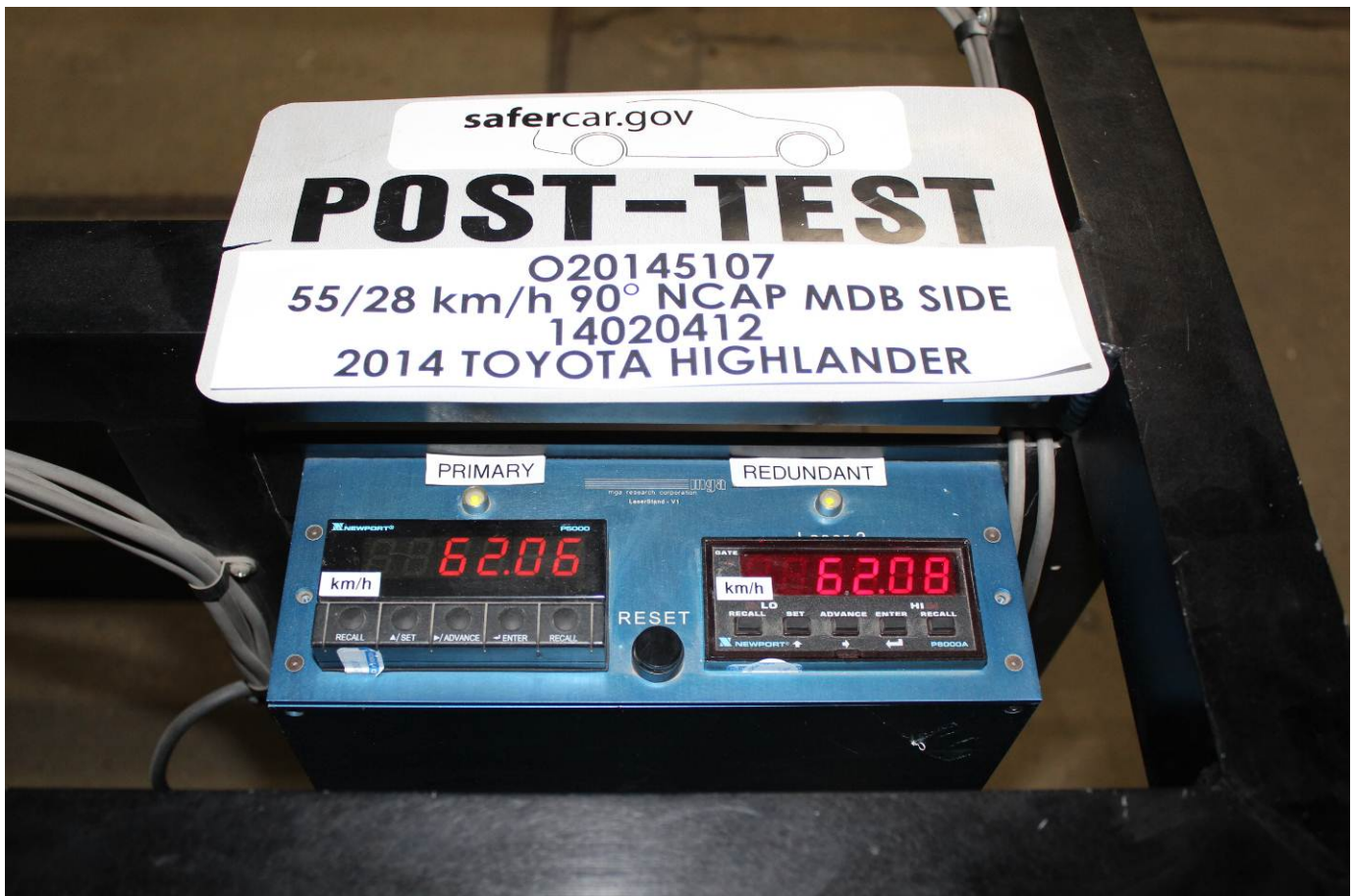
Post-Test Primary and Redundant Speed Trap Read-Out
