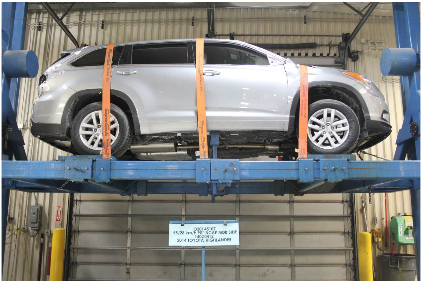
FMVSS No. 301 Static Rollover 0 Degrees
