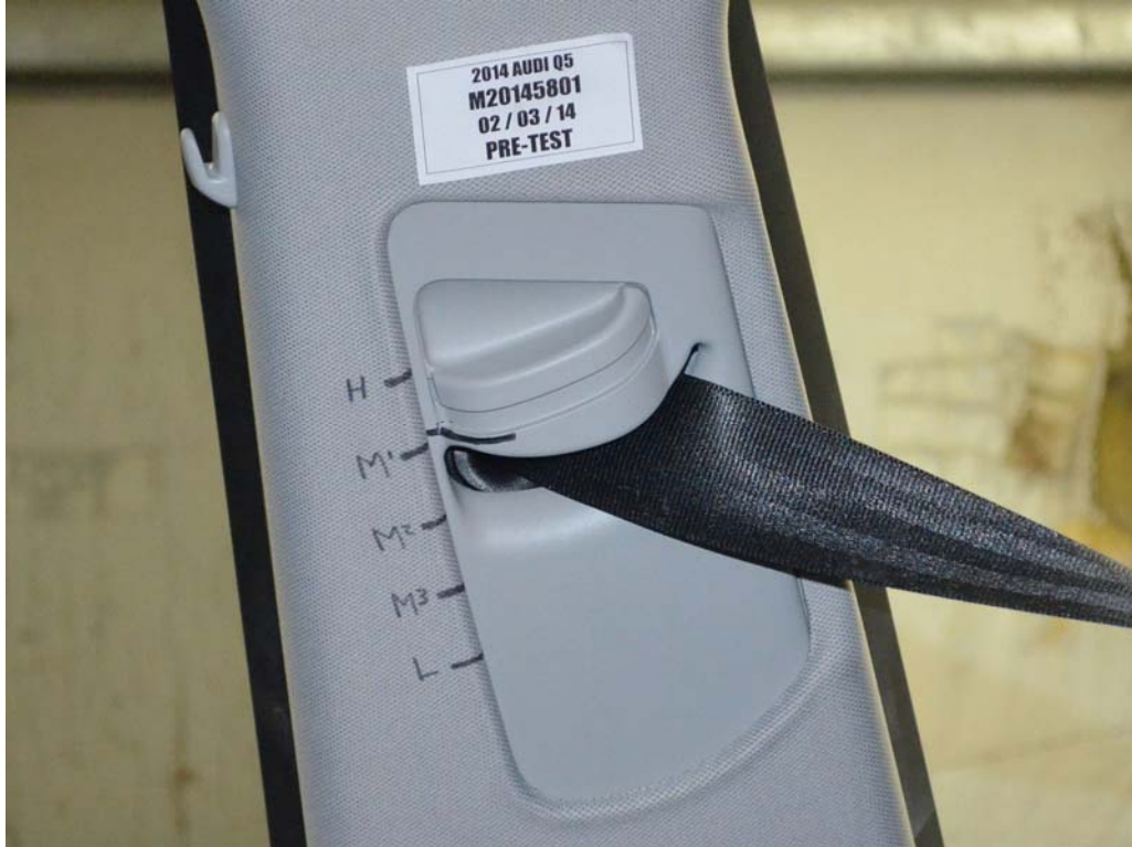
FIGURE 33. Pre-Test View of Belt Anchorage for Dummy
