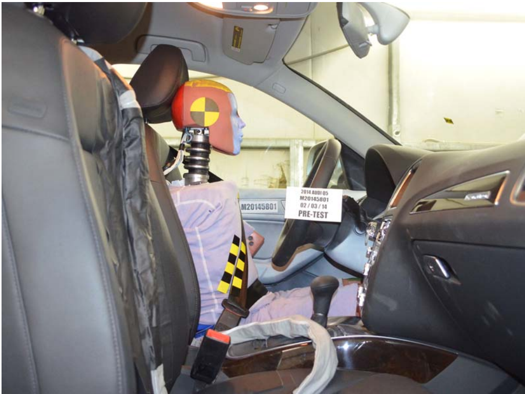
FIGURE 42. Pre-Test Right Side View of Dummy and Front Seat of Occupant Compartment
