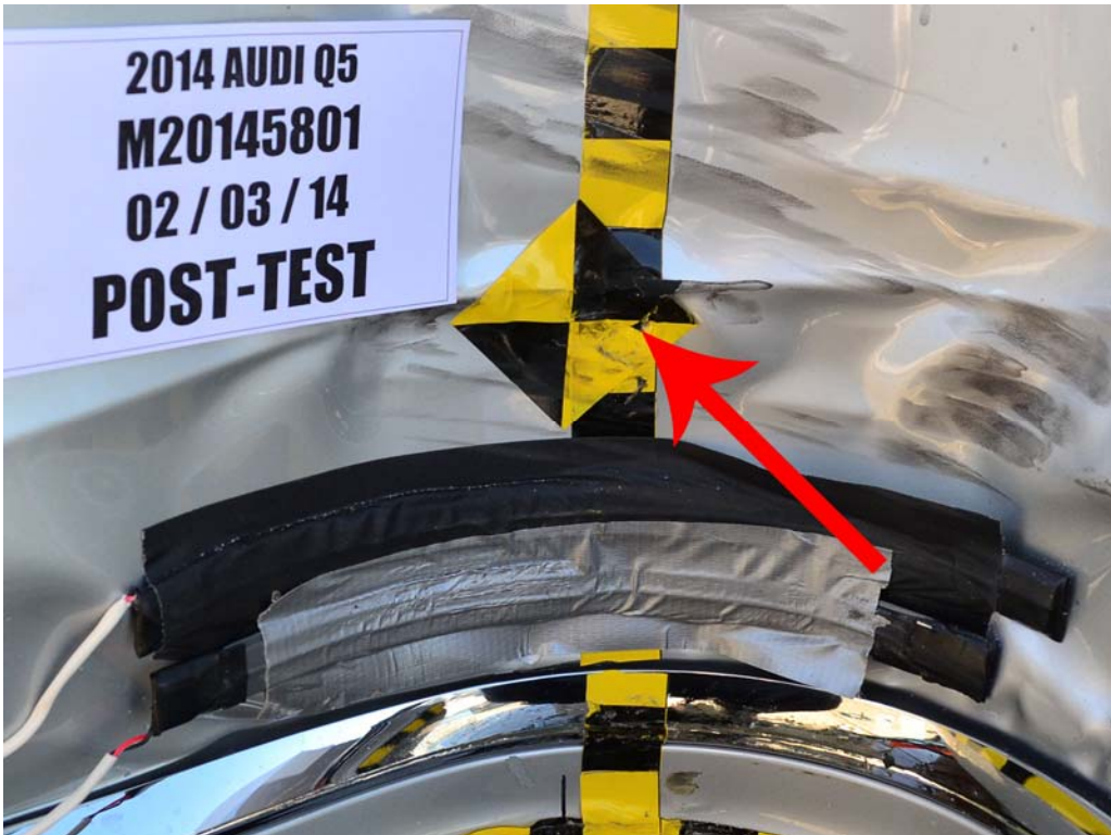
FIGURE 20. Post-Test Close-Up View of Impact Point Target Showing Impact Location
