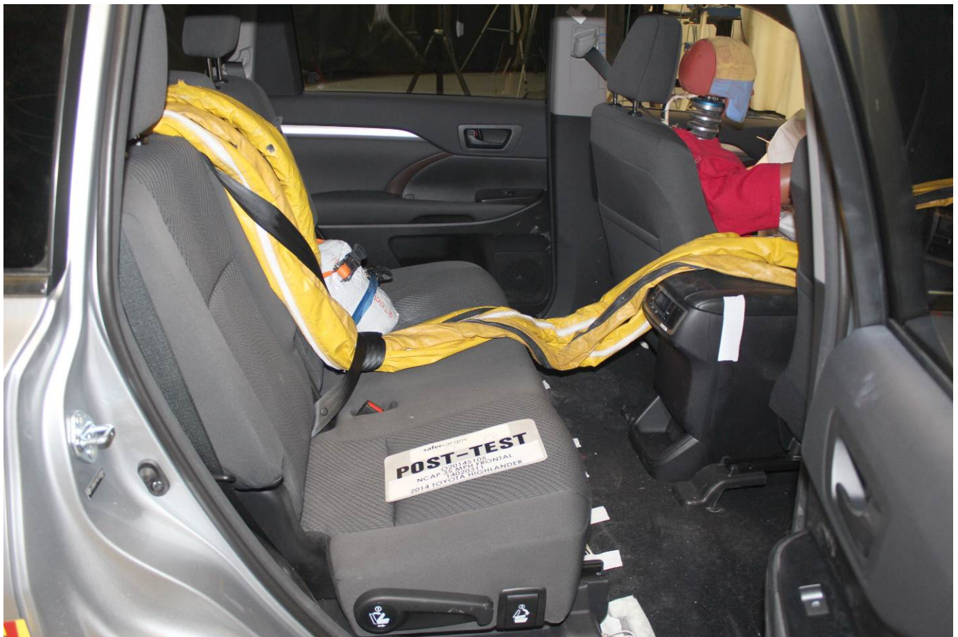
Post-Test Dummy Cable Routing
