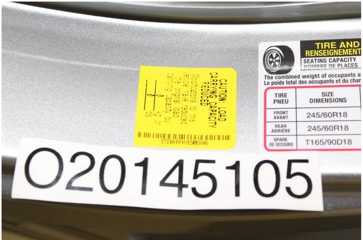
Load Carrying Capacity Reduced Label
