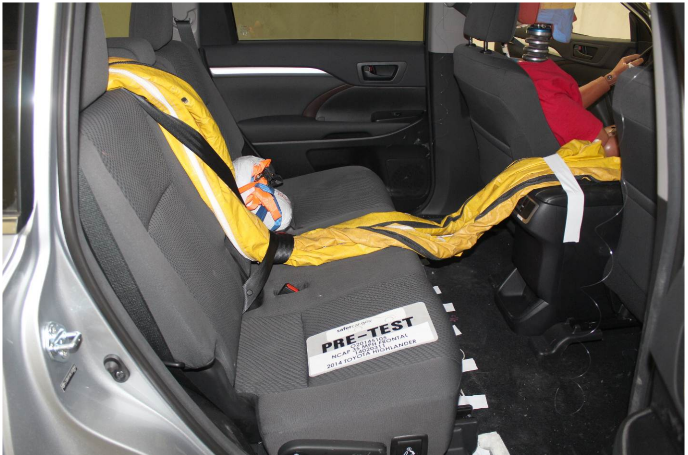
Pre-Test Dummy Cable Routing
