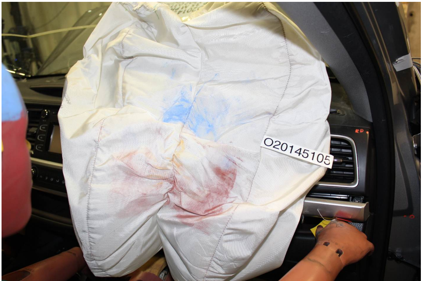
Post-Test Passenger Dummy Contact with Airbag
