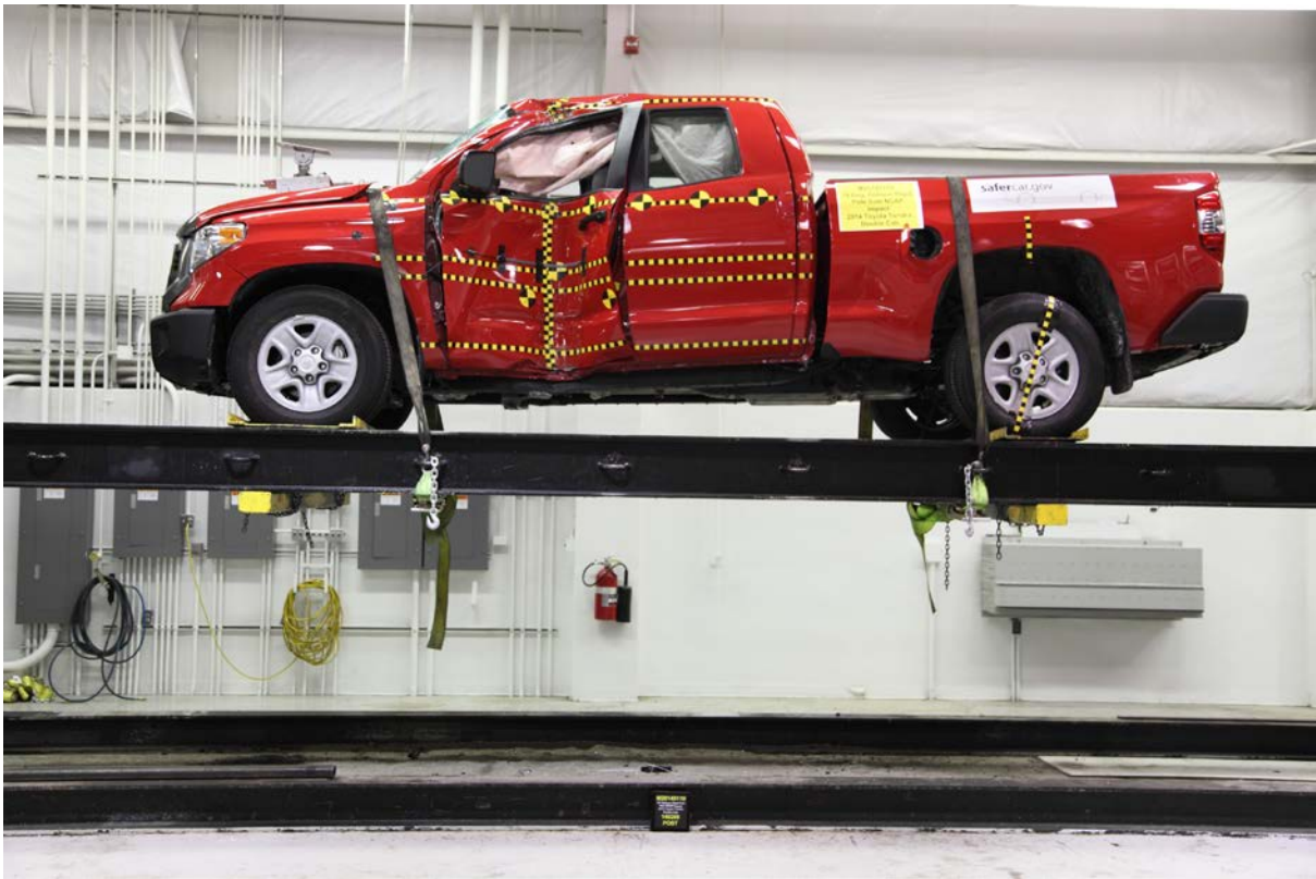
063 FMVSS No. 301 Static Rollover 0 Degrees
