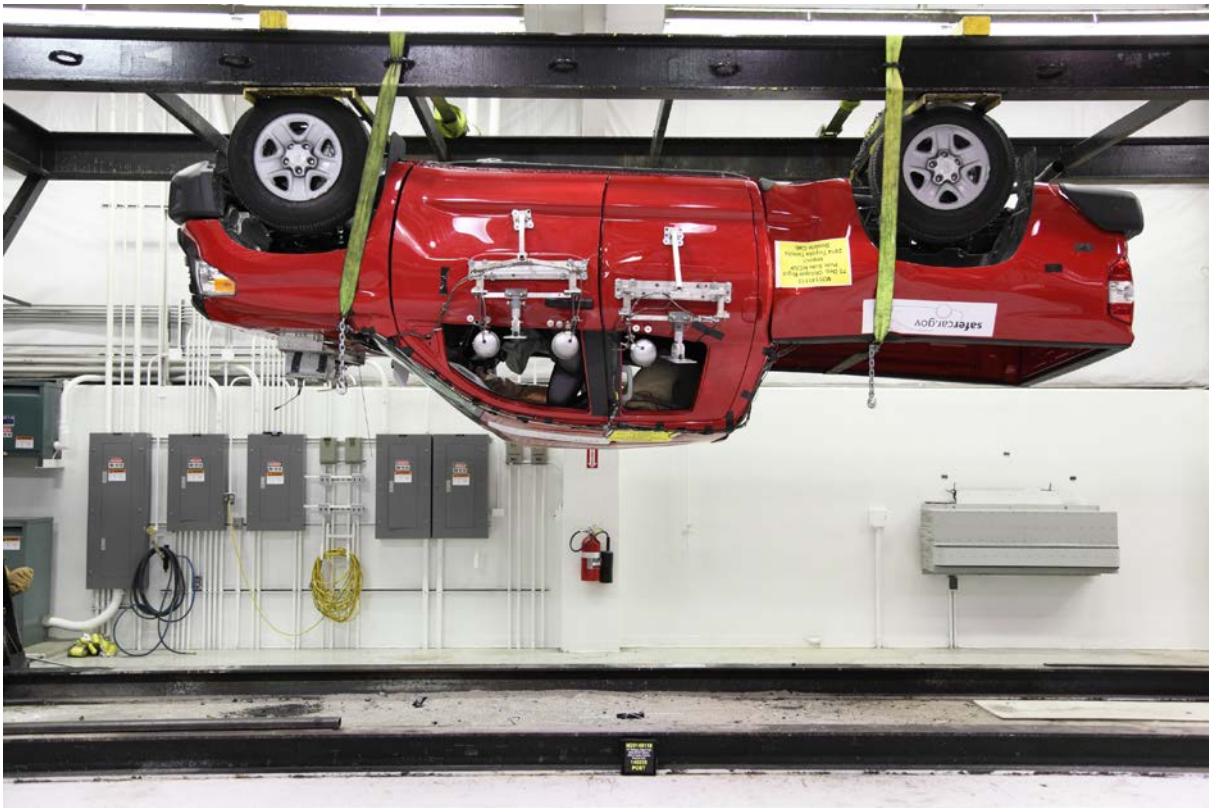
065 FMVSS No. 301 Static Rollover 180 Degrees
