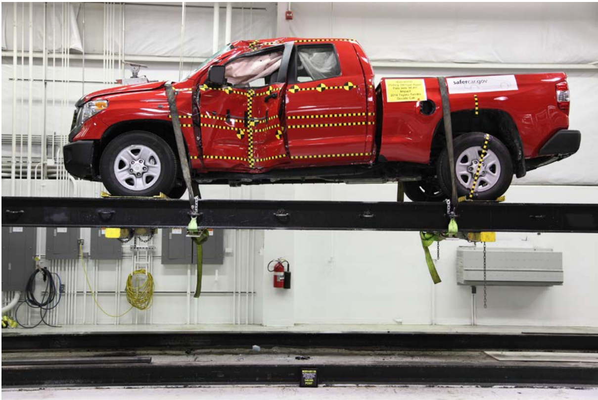
067 FMVSS No. 301 Static Rollover 360 Degrees
