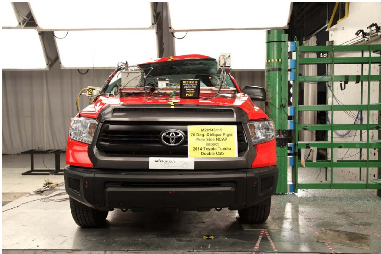
004 Post-Test Frontal View of Test Vehicle
