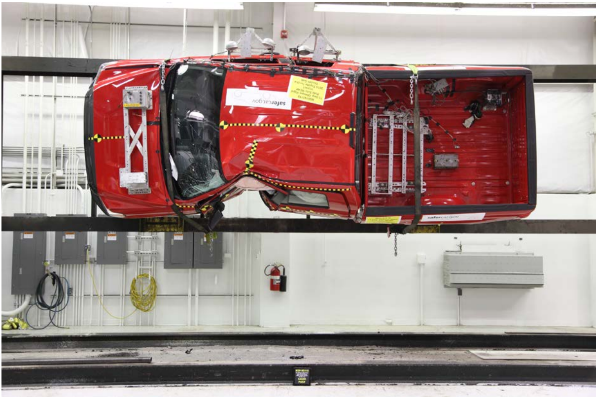
064 FMVSS No. 301 Static Rollover 90 Degrees
