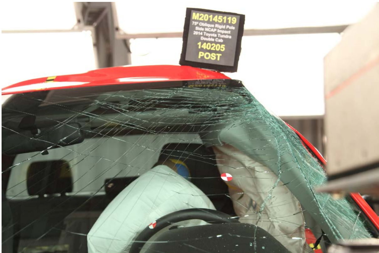
022 Post-Test Front Close-Up View of Dummy
