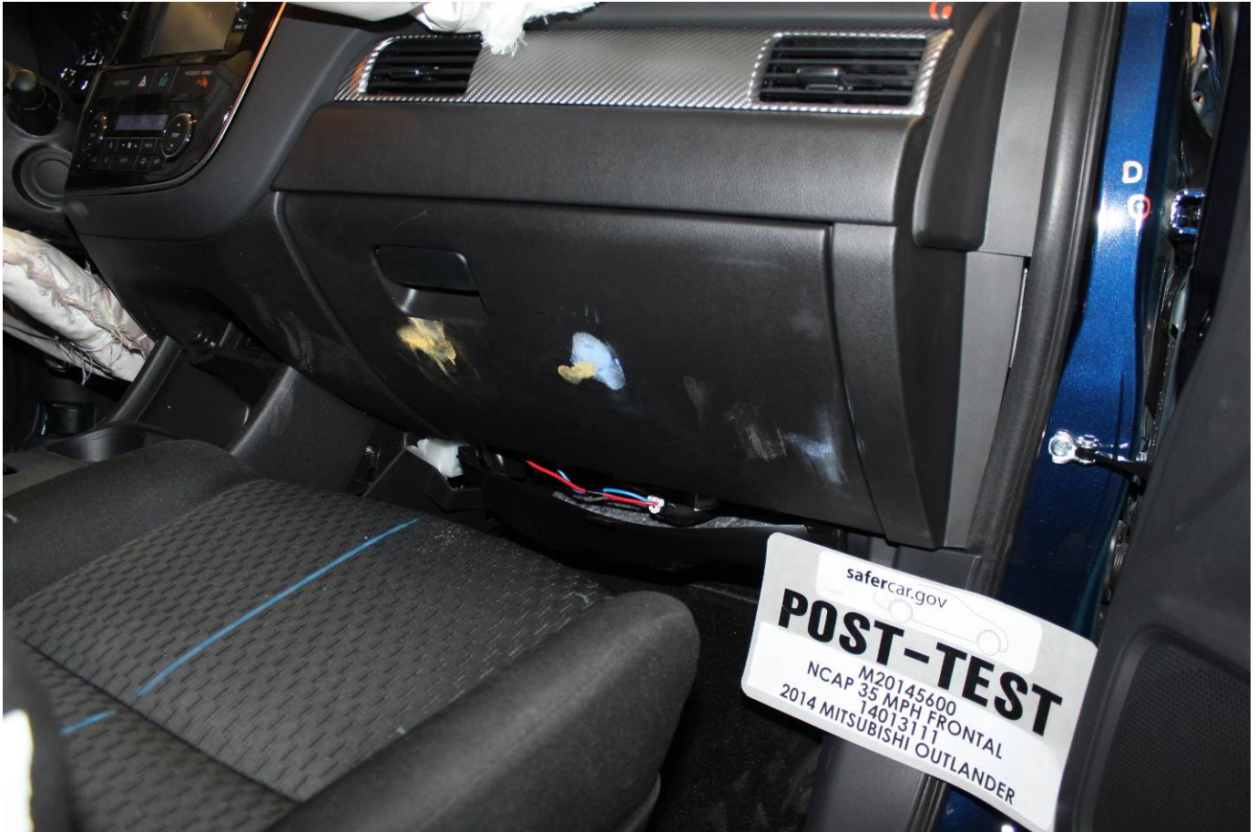
Post-Test Passenger's Side Knee Bolster (without dummy)
