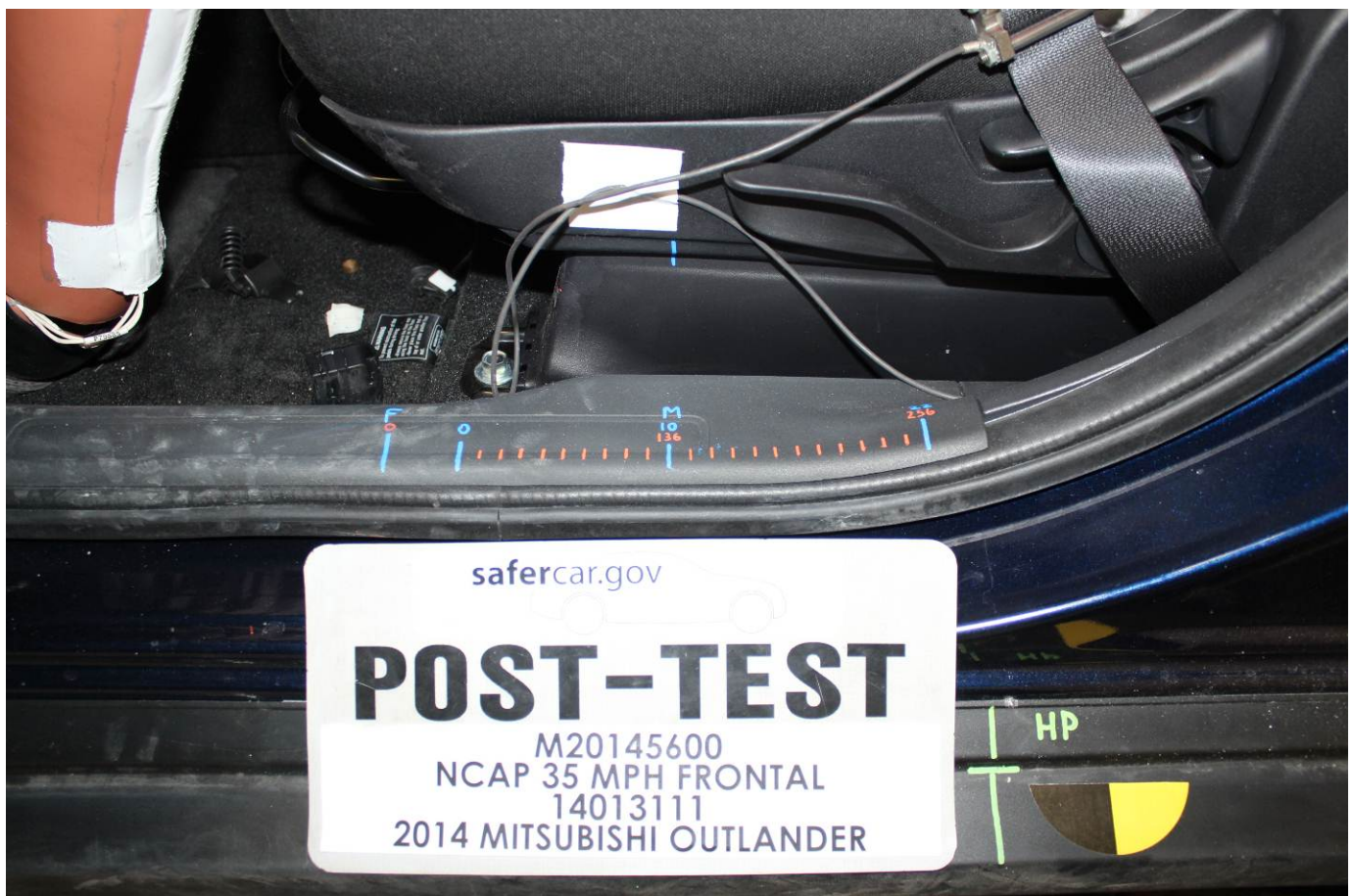
Post-Test Driver's Seat Fore-Aft Markings
