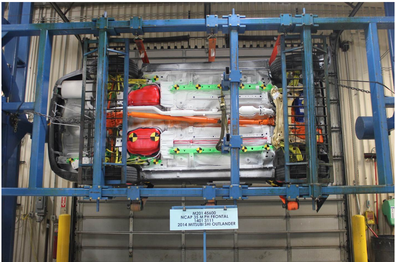
Vehicle at 0 Degree on Static Rollover Device
