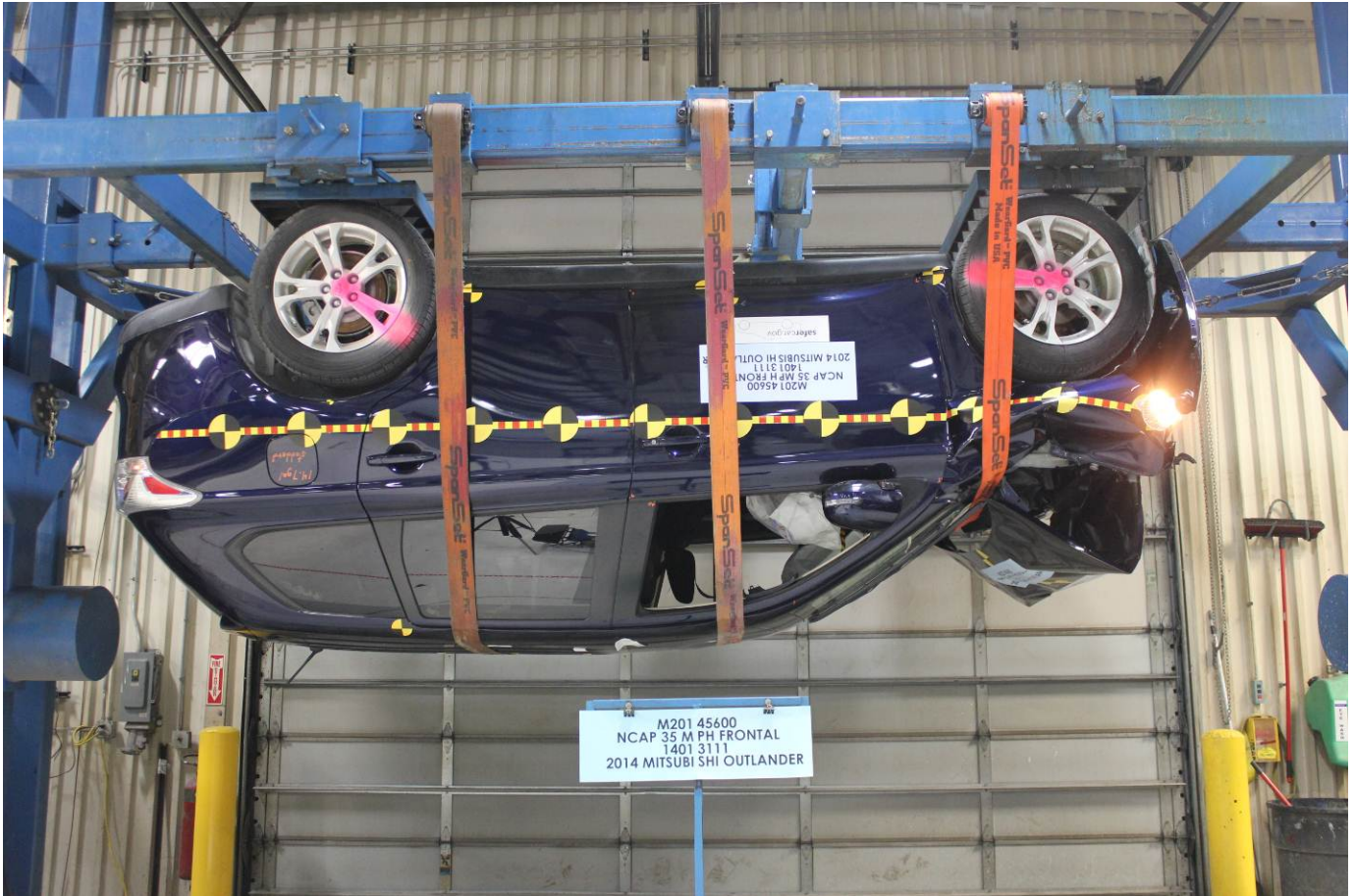
Vehicle at 180 Degrees on Static Rollover Device
