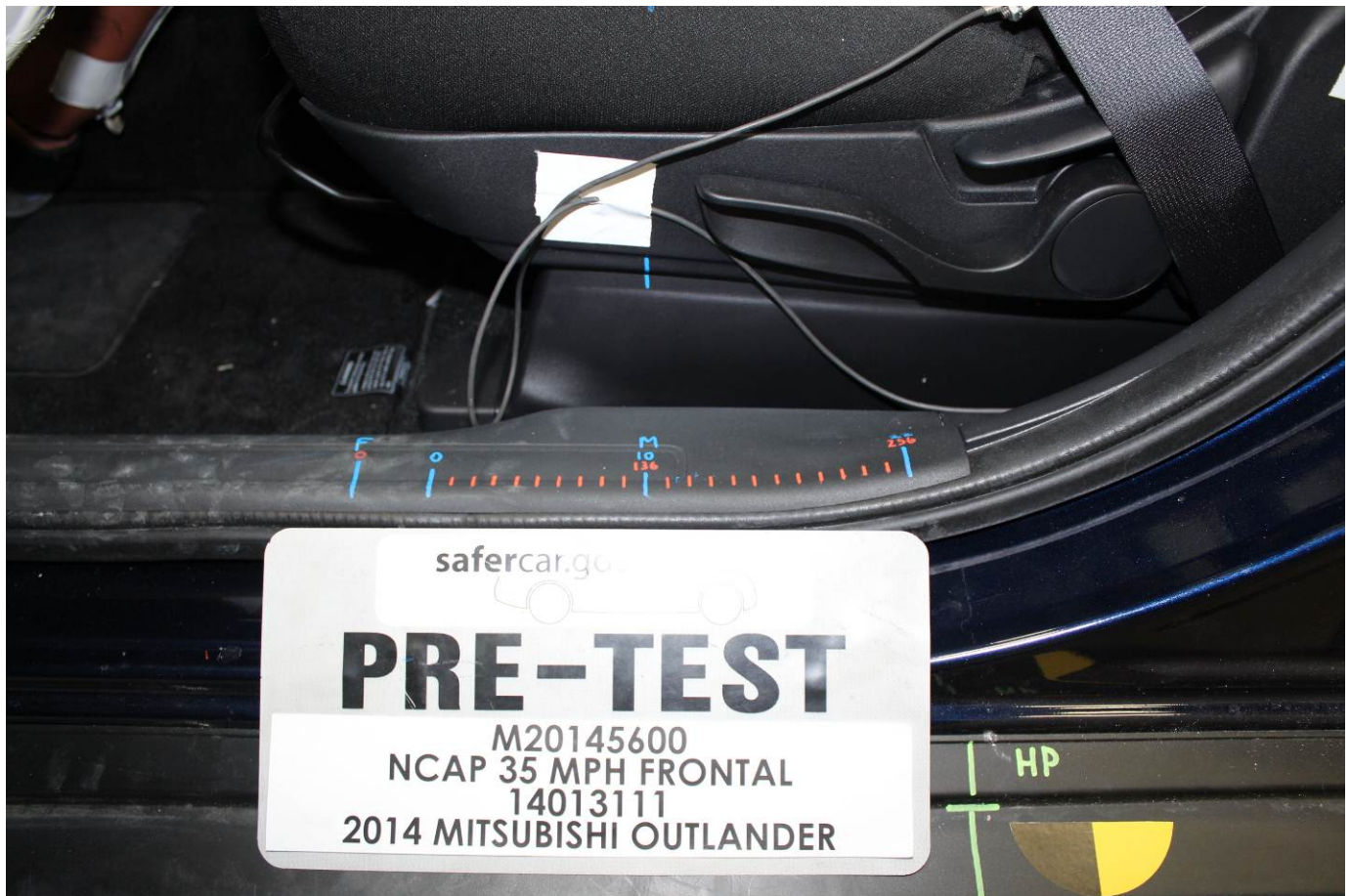
Pre-Test Driver's Seat Fore-Aft Markings
