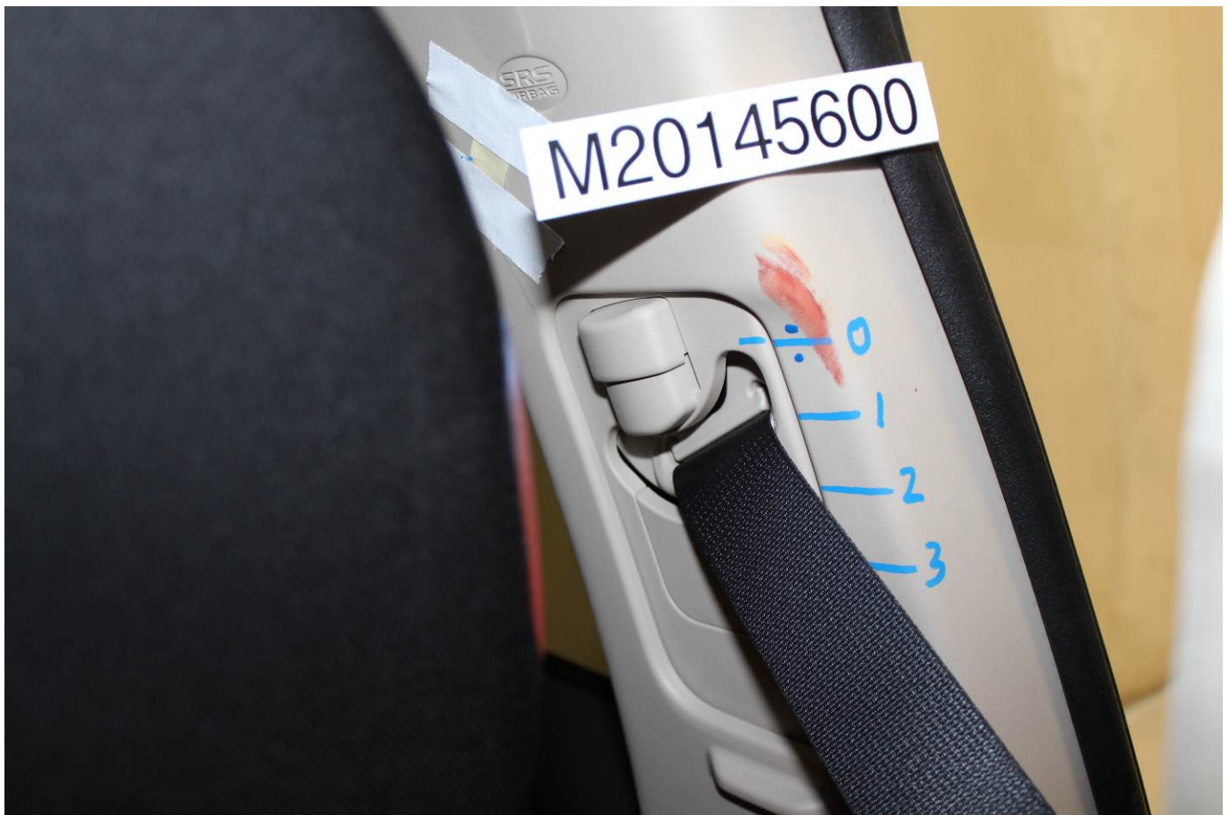
Post-Test Driver Dummy Contact with B-Post
