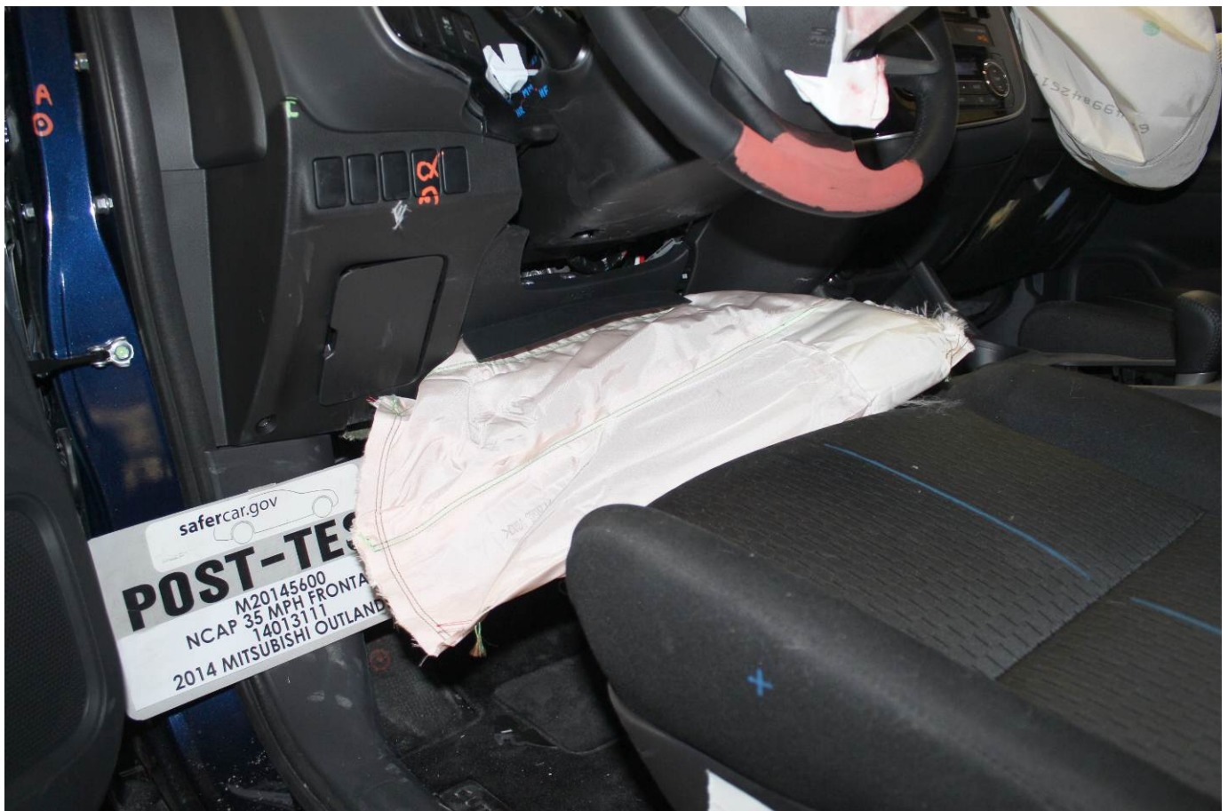
Post-Test Driver's Side Knee Bolster (without dummy)
