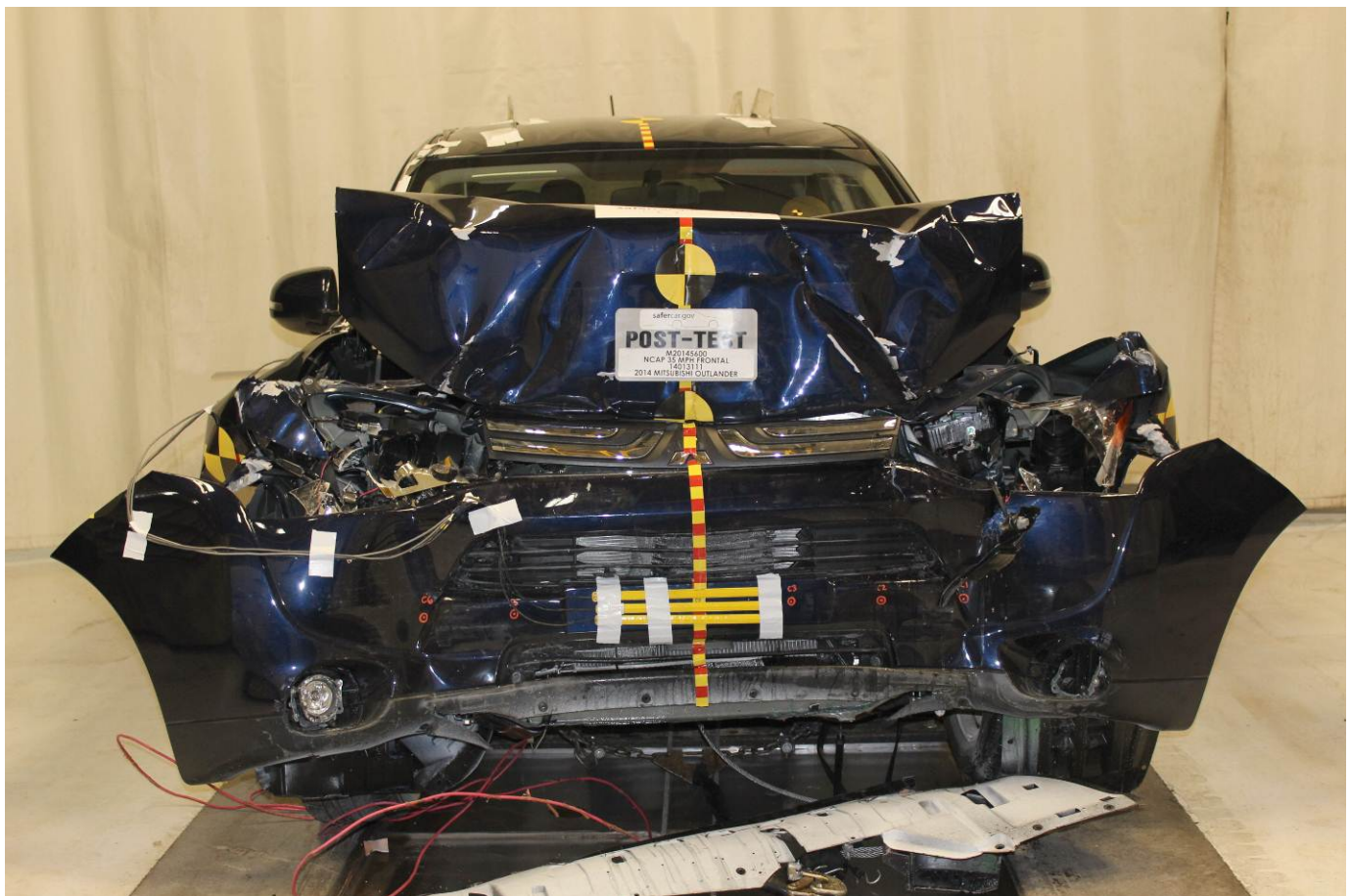
Post-Test Front View of Test Vehicle
