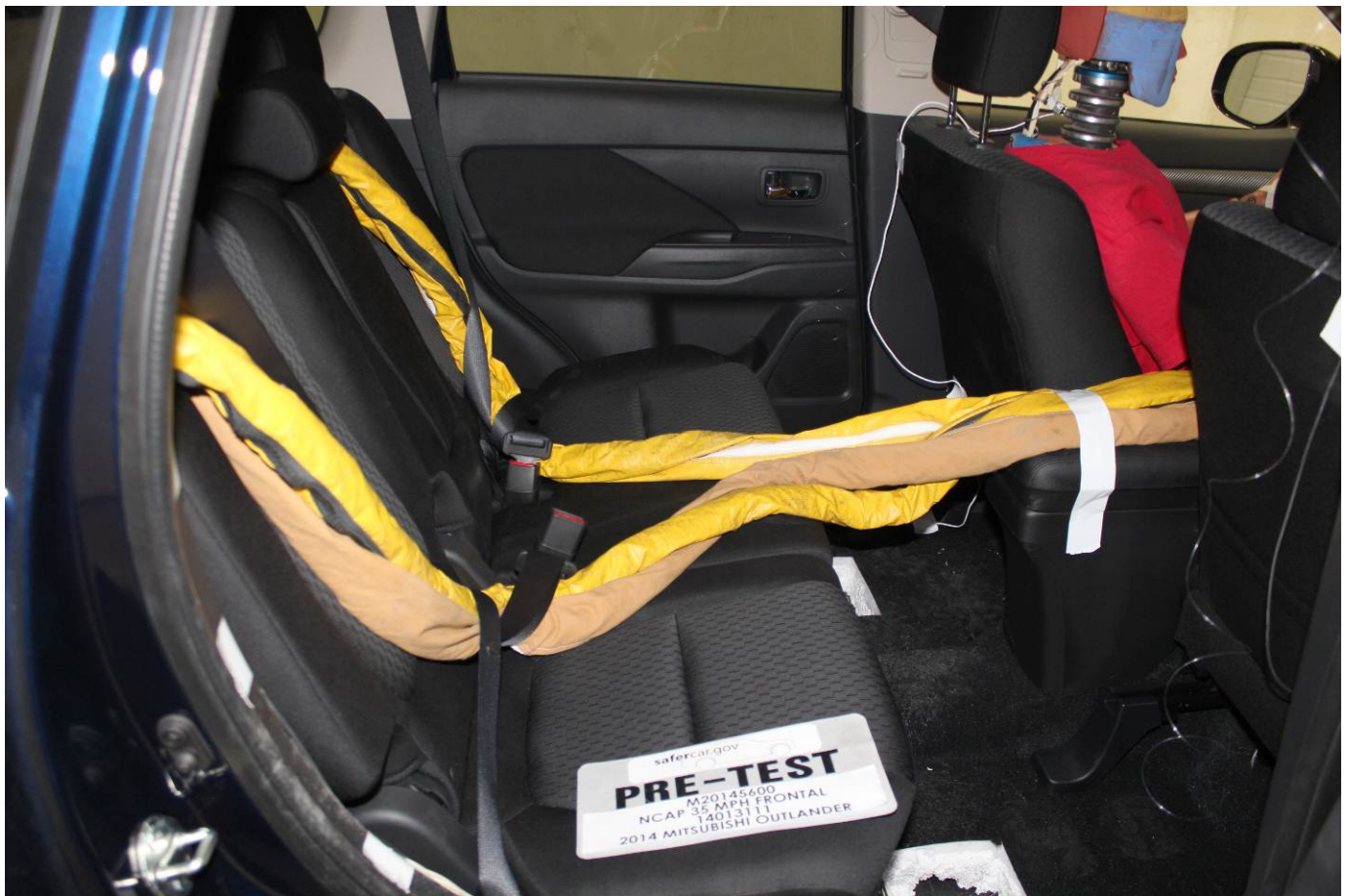
Pre-Test Dummy Cable Routing
