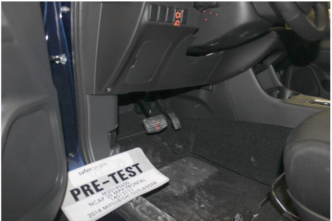
Pre-Test Driver's Side Knee Bolster (without dummy)
