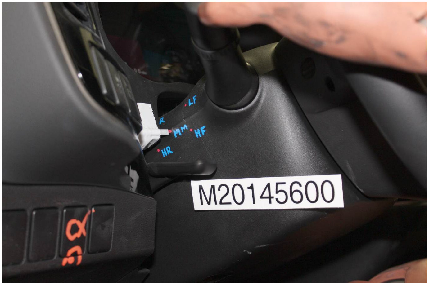
Post-Test Driver Dummy Contact with Knee Airbag
