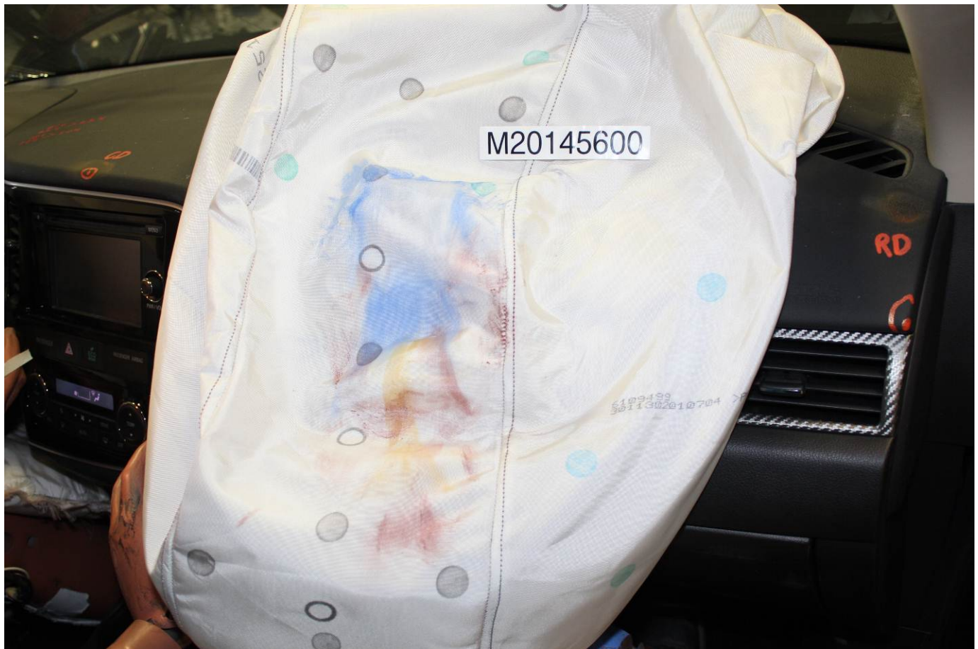
Post-Test Passenger Dummy Contact with Airbag
