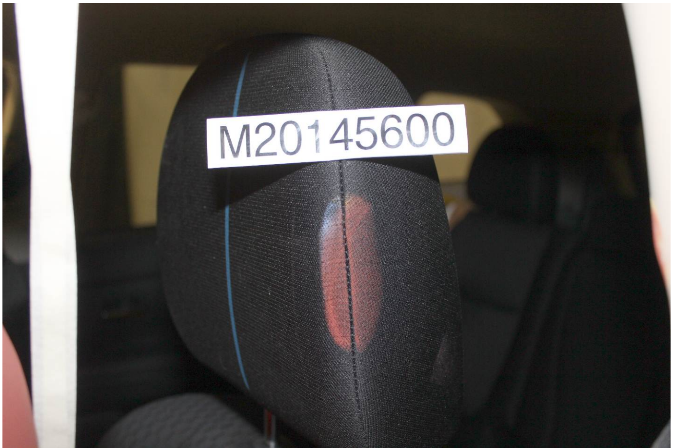
Post-Test Driver Dummy Contact with Headrest
