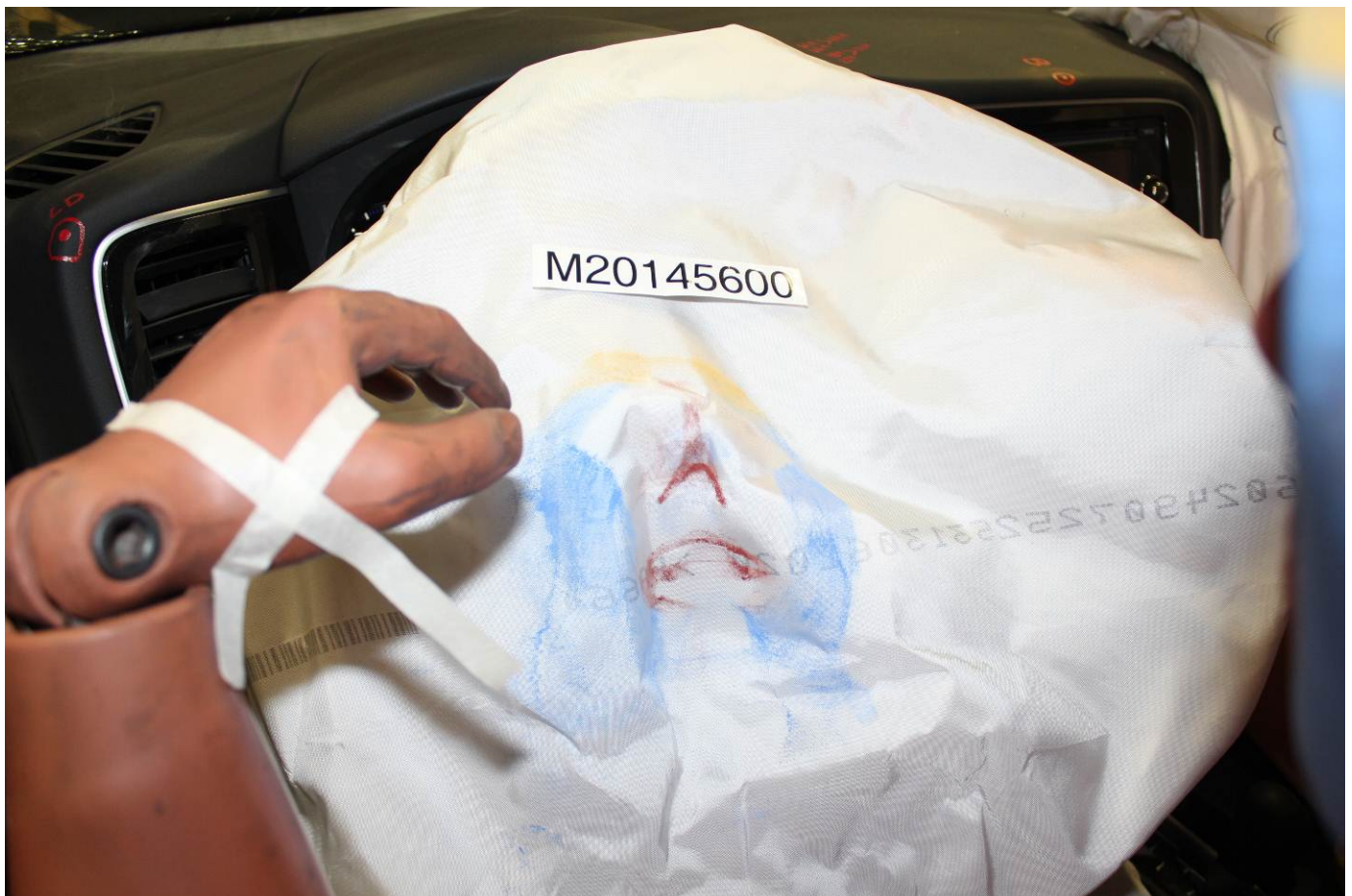
Post-Test Driver Dummy Contact with Airbag
