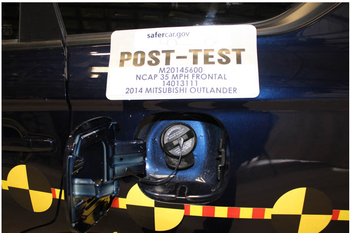
Post-Test Fuel Filler Cap View
