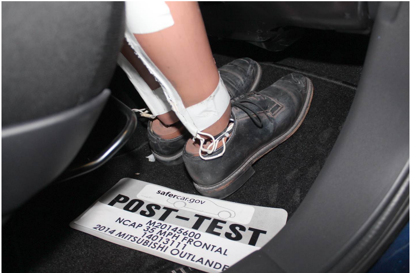
Post-Test Passenger Dummy Feet
