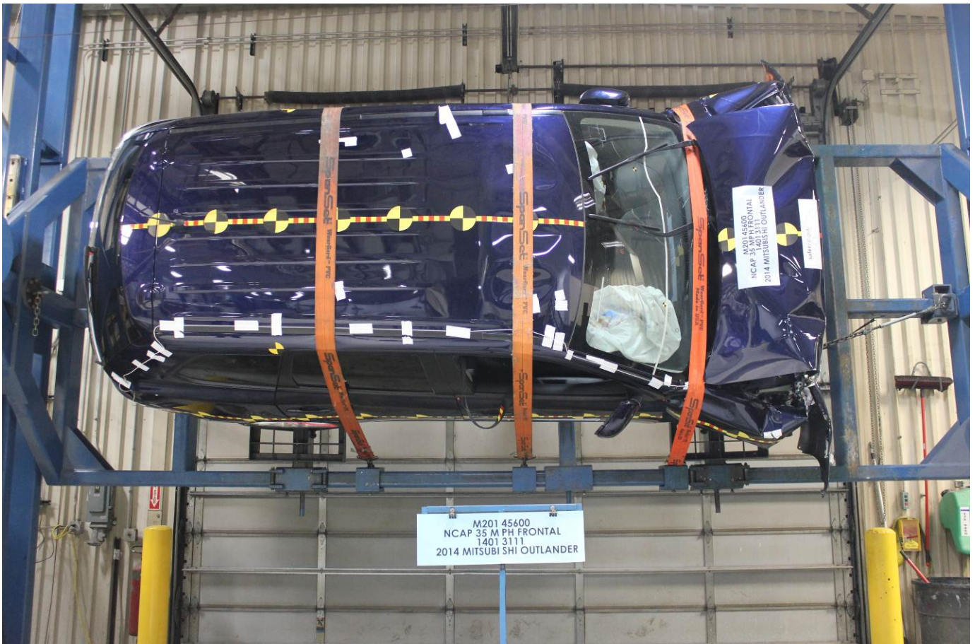
Vehicle at 180 Degrees on Static Rollover Device
