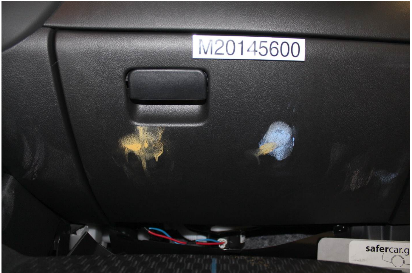
Post-Test Passenger Dummy Contact with Glovebox
