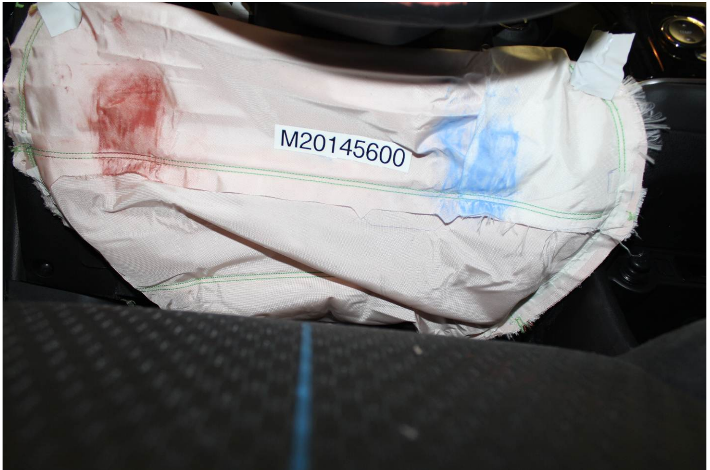
Post-Test Driver Dummy Contact with Knee Airbag
