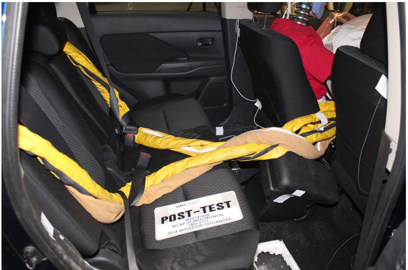
Post-Test Dummy Cable Routing
